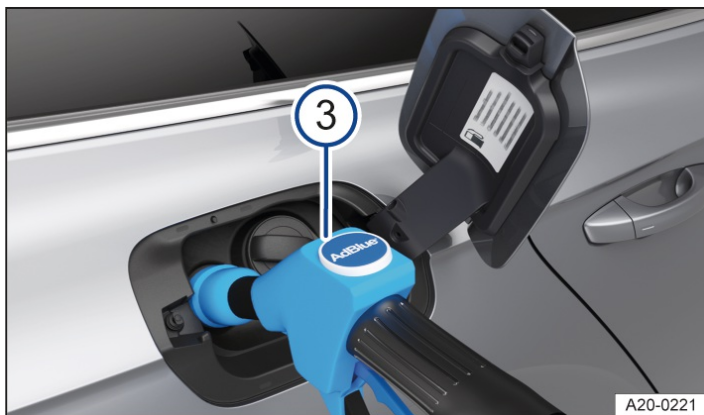
Fig. 3 Behind the fuel filler flap: refuel AdBlue with the fuel pump nozzle (general example).
