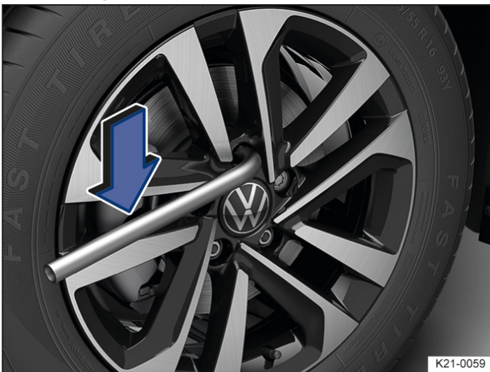
Fig. 1 Wheel change: removing wheel bolts with the lug wrench.
