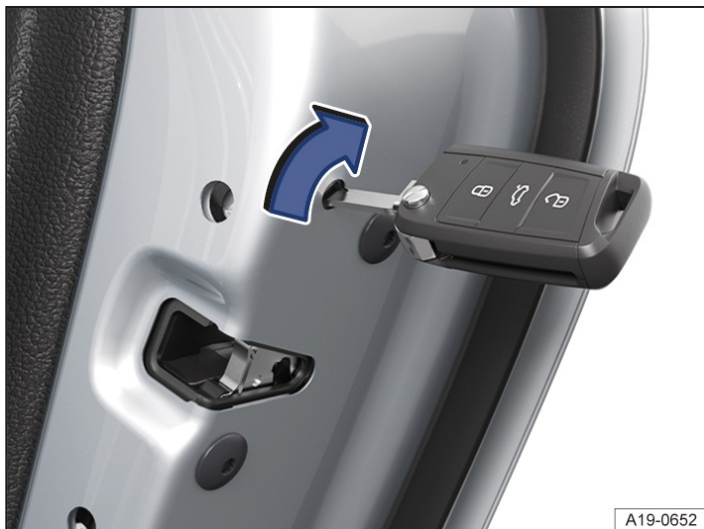
Fig. 1 On the front of the right rear door: emergency locking the vehicle with the vehicle key (general example).
