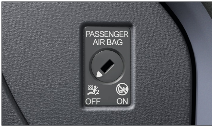
Fig. 1 In the instrument panel on the front passenger side: Key-operated switch to turn on and off the front passenger's front airbag.
