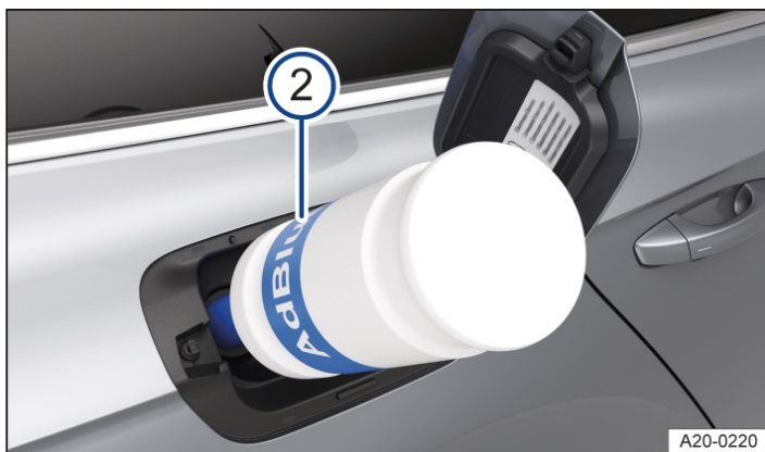
Fig. 2 Behind the fuel filler flap: filling up AdBlue with the refiller bottle (general example).
