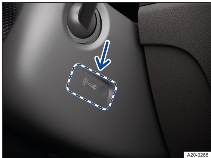
Fig. 1 On the right side of the steering column: emergency start function on vehicles with Keyless Access with push-button start.
