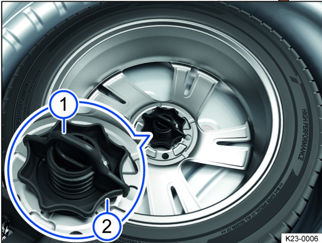
Fig. 222 Under the luggage compartment floor: handwheel to secure the spare wheel.
