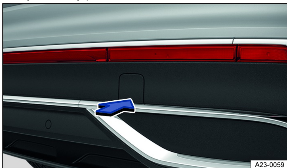
Fig. 202 In the right rear bumper: Remove the cover, variant 1.
