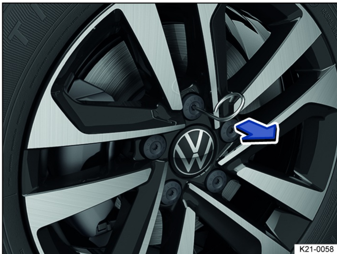
Fig. 224 Remove the caps from the wheel bolts.
