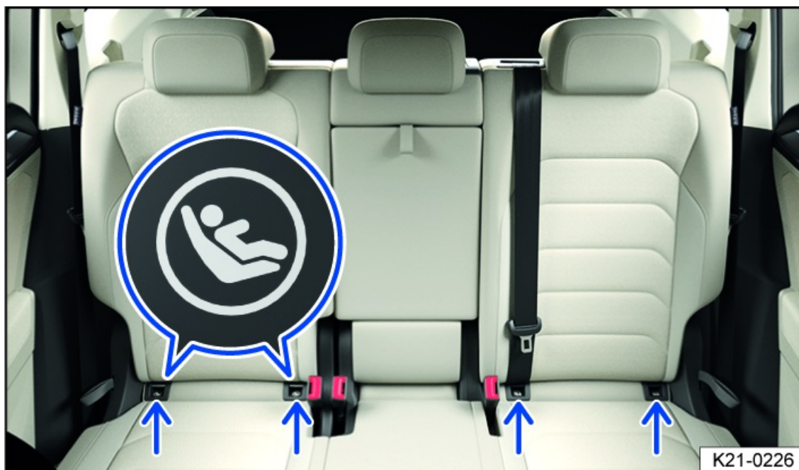
Fig. 43 On the outer seats in the second row: Designation and symbol showing the ISOFIX/lower LATCH anchorage points for child restraints.
