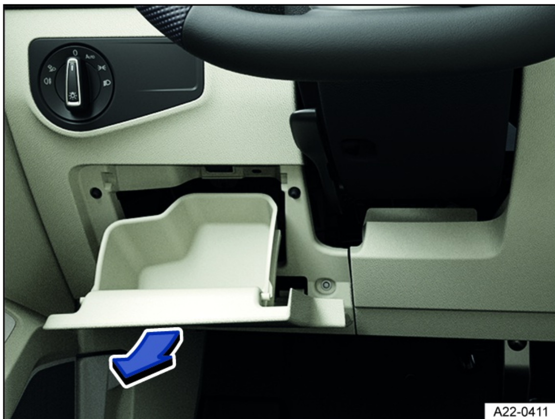
Fig. 193 To the left of the steering wheel: Fuse box cover in the instrument panel (left-hand drive vehicles).
