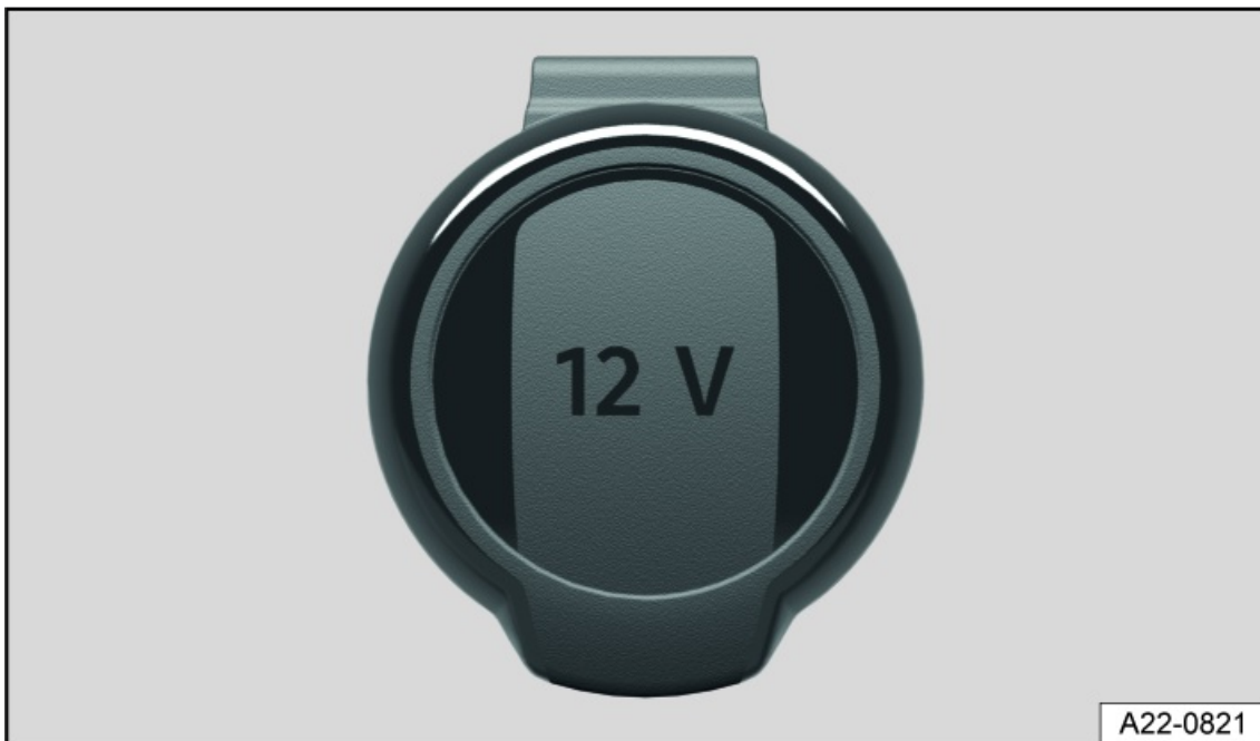
Fig. 165 In the storage compartment in the front center console, in the rear center console or in the luggage compartment on the left-hand side: folding 12-volt socket (general example).
