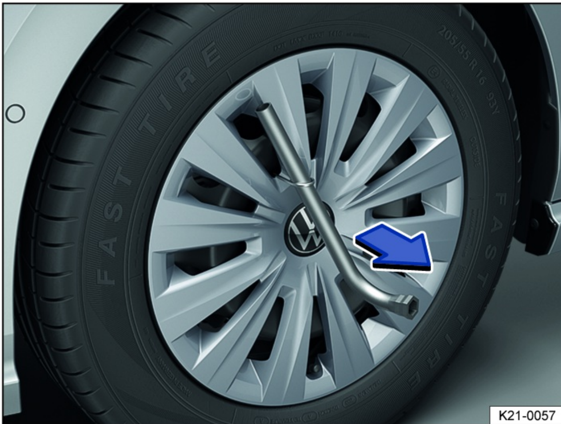
Fig. 223 Remove the wheel hub cover.
