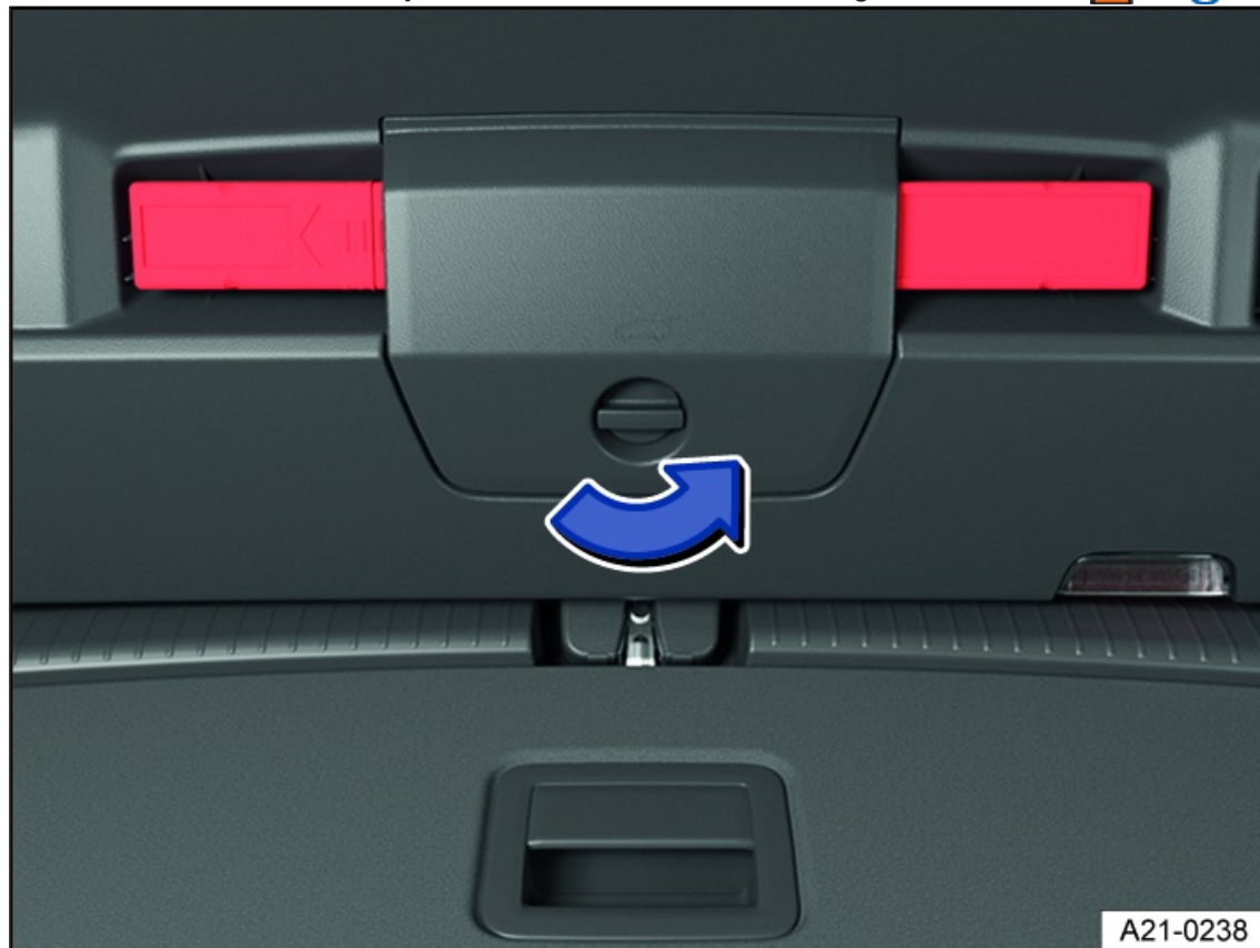
Fig. 70 In the trunk lid: open the holder for the warning triangle.
