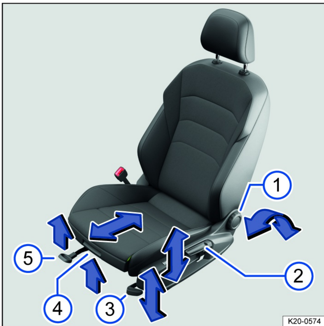
Fig. 77 On the driver seat: Controls (variant 2).
