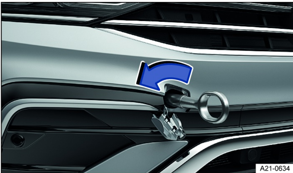
Fig. 201 In the right front bumper: Screw in towing eye.
