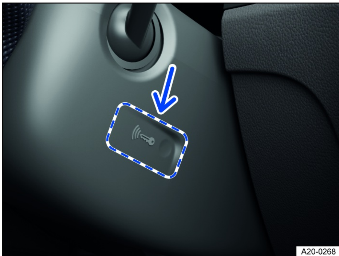
Fig. 120 On the right side of the steering column: emergency start function on vehicles with Keyless Access with push-button start.
