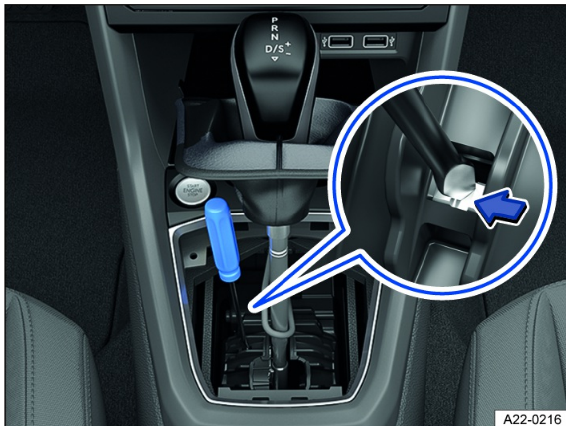
Fig. 124 In the center console: manually release the Automatic Shift Lock (ASL) (variant 1).
