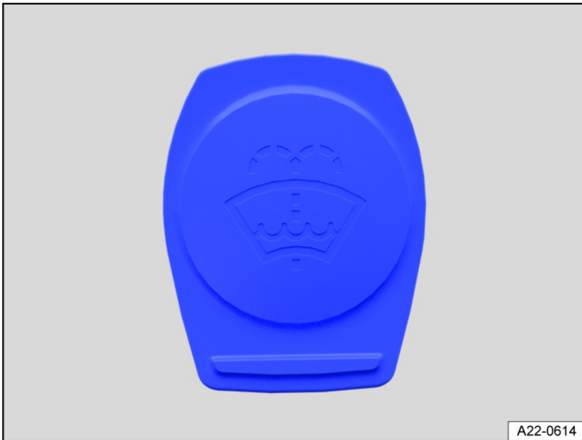
Fig. 208 In the engine compartment: Cap on the washer fluid reservoir (general example).
