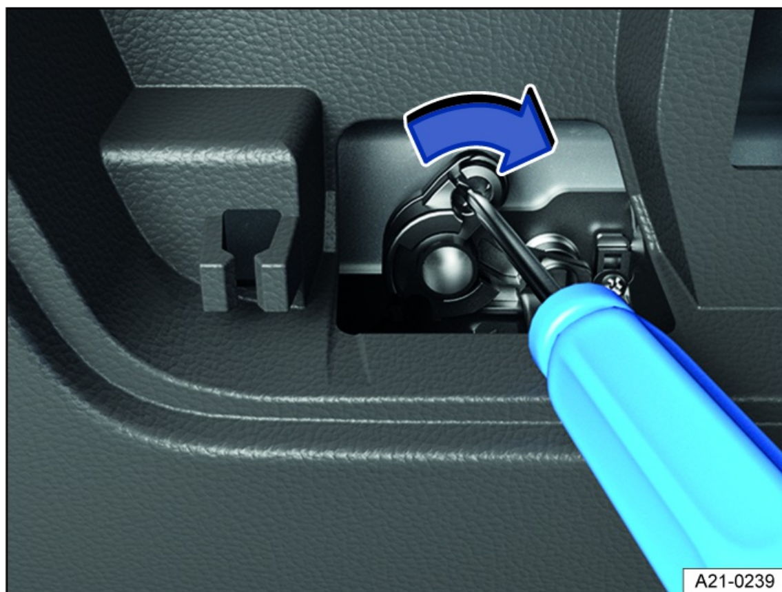
Fig. 71 In the trunk lid: emergency release for the trunk lid.
