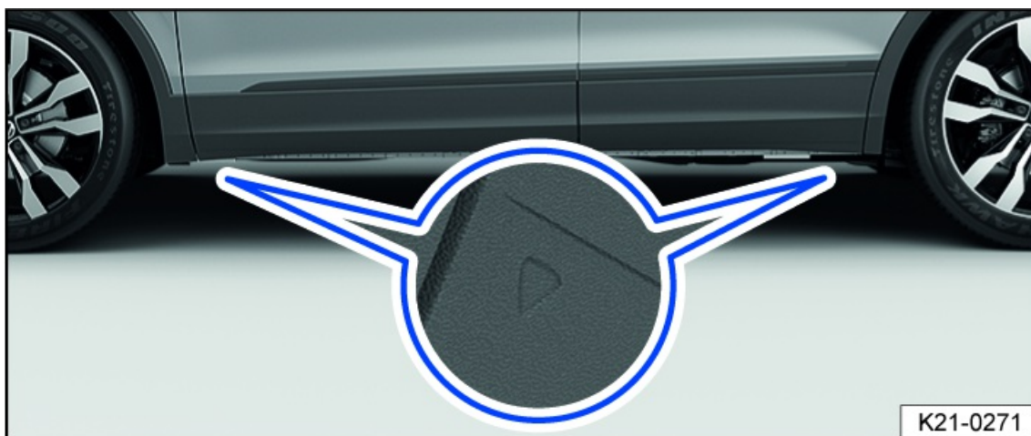
Fig. 226 On the side sill: markings for the jack lift points.
