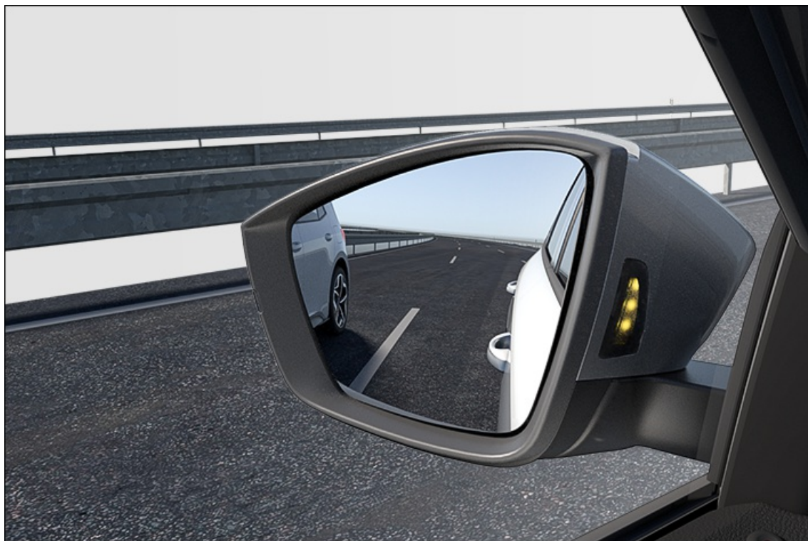
Fig. 147 In the housing of the outside mirrors: Side Assist indicators.
