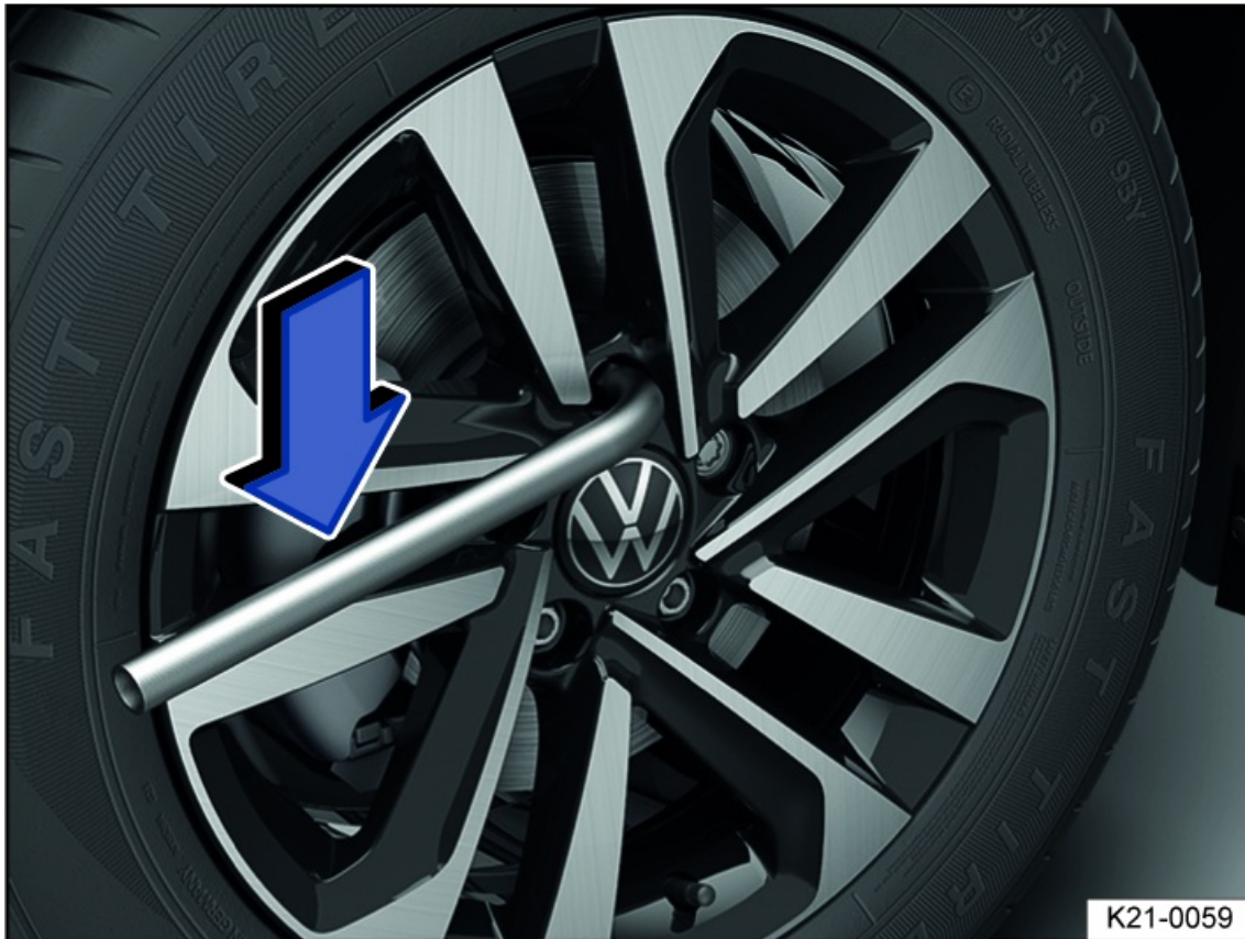
Fig. 229 Removing wheel bolts with the lug wrench.
