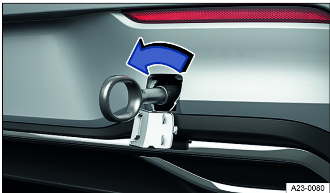
Fig. 203 In the right rear bumper: Remove the cover, variant 2.
