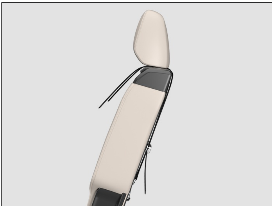
Fig. 46 On the back of the second-row seats: attached top tether safety belt.
