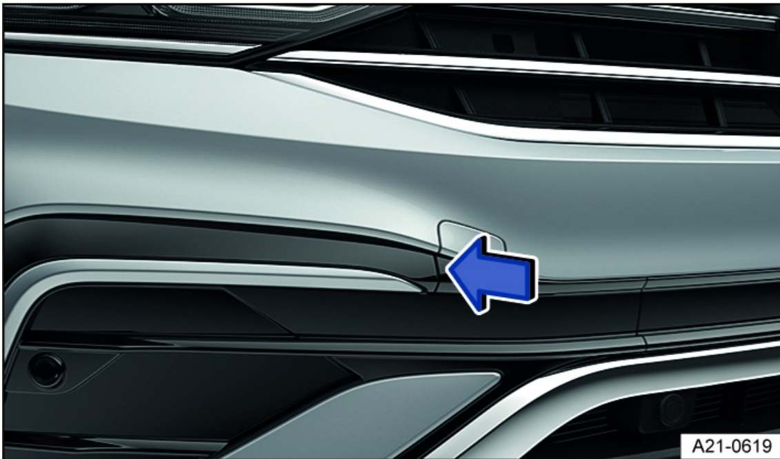
Fig. 200 In the right front bumper: Remove cover.
