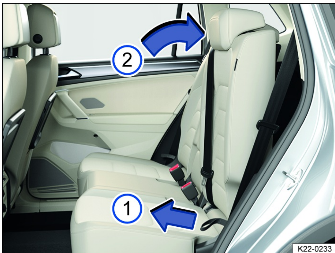
Fig. 83 Rear bench seat: adjust the rear seat backrest.
