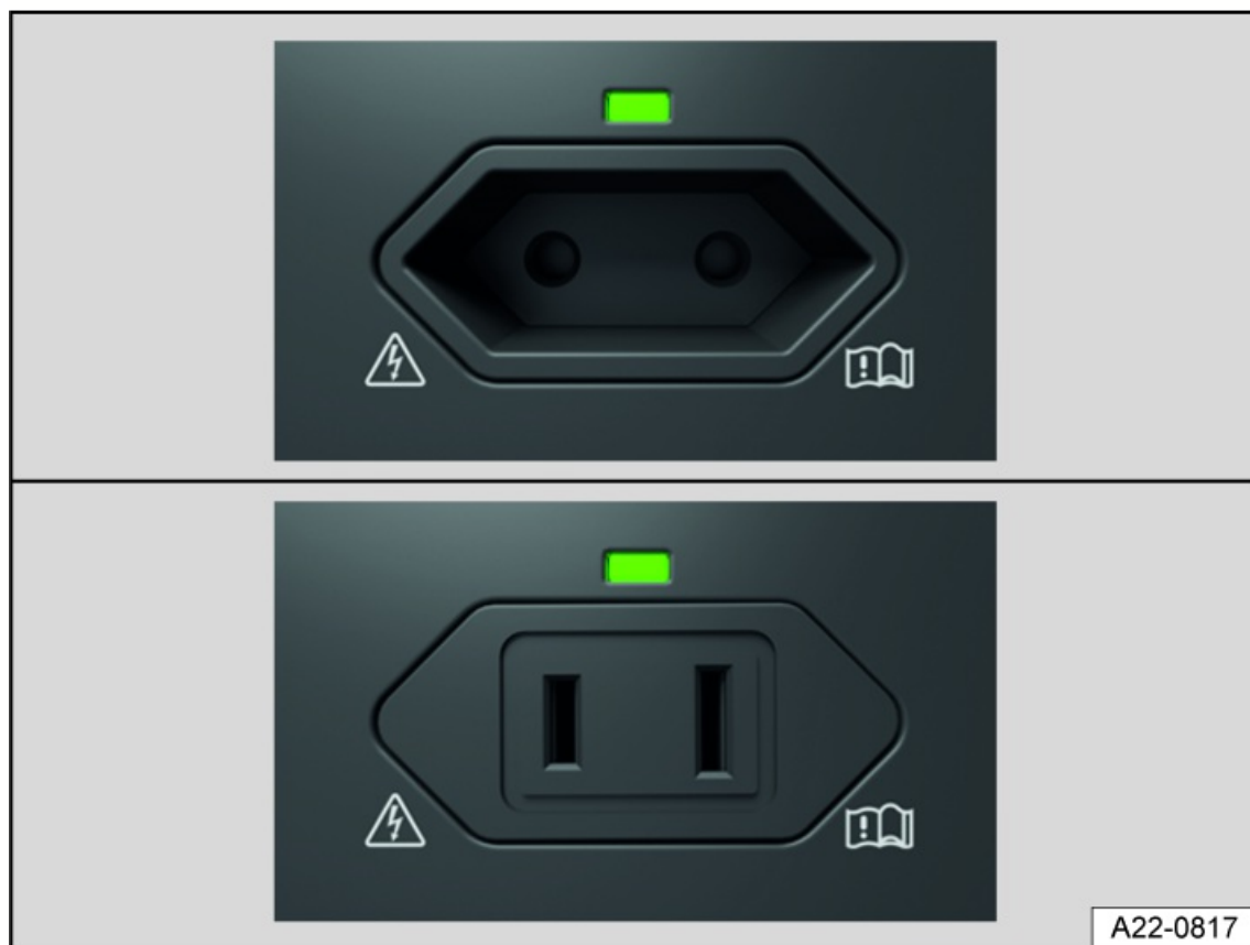
Fig. 166 In the luggage compartment on the left-hand side: 230-volt socket, 115-volt socket or 100-volt socket (depending on the vehicle equipment).
