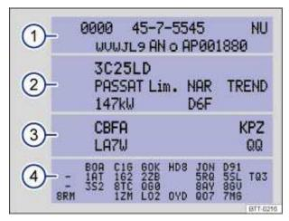
Fig. 17 Vehicle identification label: shown in the example with engine identification code CBFA 3.
