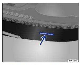
Fig. 18 Vehicle identification number (VIN).
