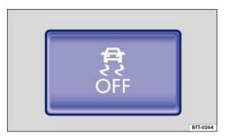
Fig. In the center console: Button to manually switch ASR on and off.
