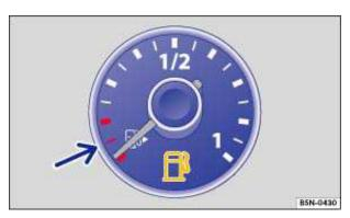
Fig. In the instrument cluster: Fuel gauge.
