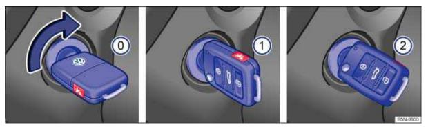
Fig. In the ignition switch: Vehicle key positions.
