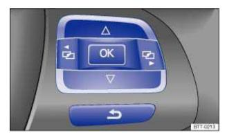
Fig. 16 Premium version (vehicles with menu control multi-function steering wheel): buttons on the right side of the steering wheel.
