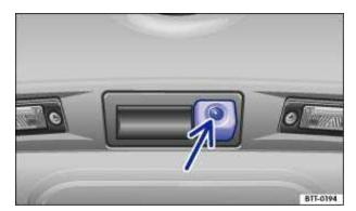
Fig. In the rear hatch: Location of the Rear Assist camera.
