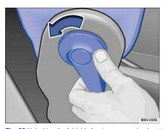
Fig. 55 Unlocking the foldable front passenger backrest.
