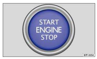
Fig. In the center console: Starter button of the Keyless Access locking and starting system.
