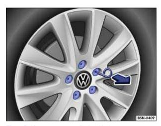
Fig. Pulling cover caps off wheel bolts.
