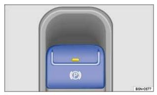
In the lower center console: Button for the electronic parking brake.
