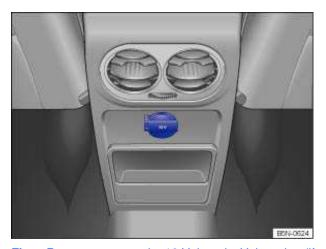
Fig. Rear center console: 12 Volt and Volt socket (if equipped).
