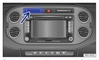
**Fig.** In the upper part of the center console: Card holder.
