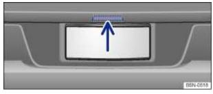
Fig. 31 Opening rear hatch from the outside.
