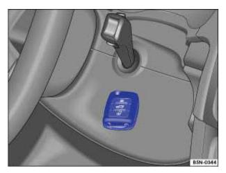
Fig. Emergency starting feature on vehicles with Keyless Access.
