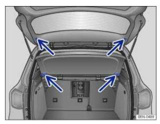
Fig. 99 Installing and removing the luggage compartment cover.
