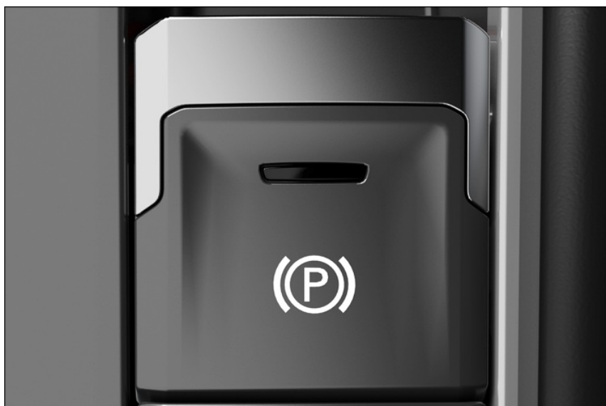
Fig. 113 In the center console: button for the electronic parking brake.
