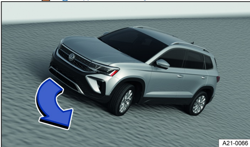
Fig. 100 General example: steering downhill along the fall line.
