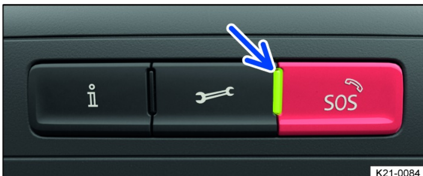
Fig. 39 In the roof console: controls for call services.
