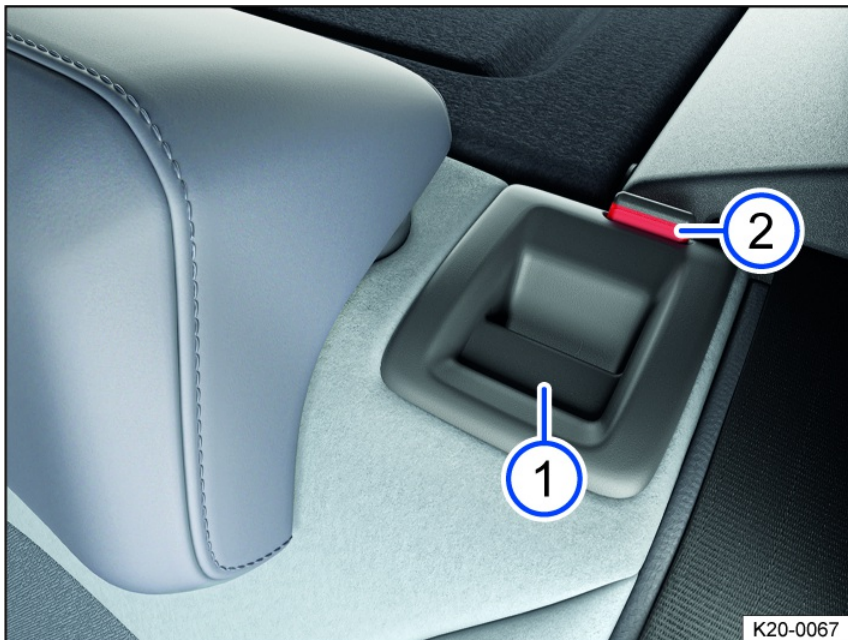
Fig. 64 In the rear seat backrest: release button.
