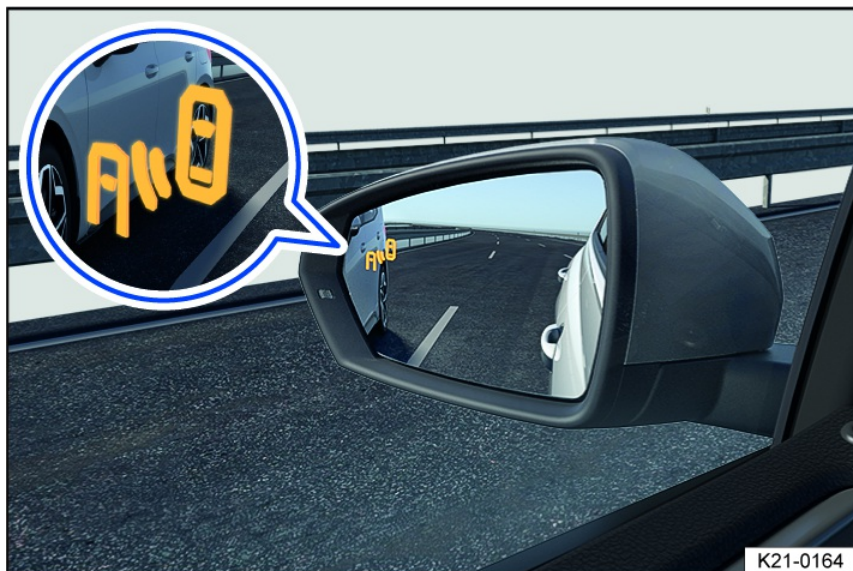
Fig. 112 In the outside mirrors: Blind Spot Monitor indicator.
