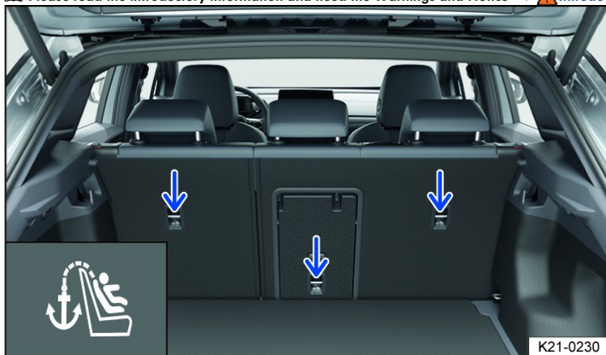
Fig. 35 On the rear side of the rear bench seat: Top tether anchorages for the top tether safety belt.
