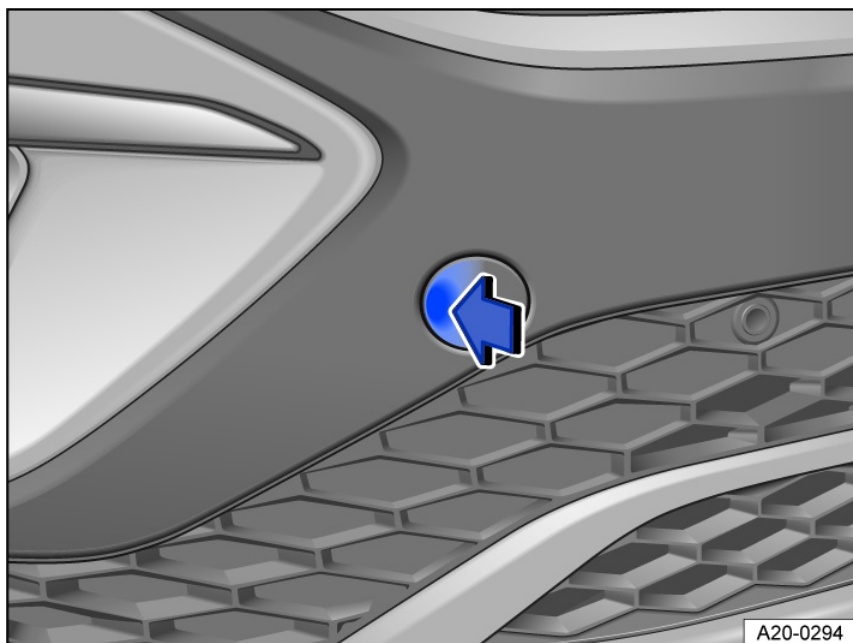
Fig. 144 In the right front bumper: Remove cover.
