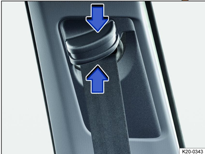
Fig. 25 Next to the front seats: safety belt height adjuster.
