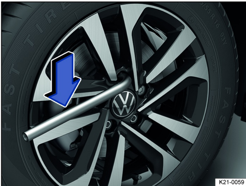
Fig. 168 Changing a tire: loosening the wheel bolts.
