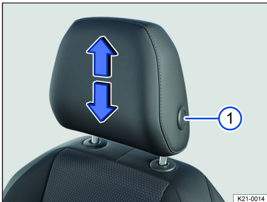
Fig. 65 General example: adjusting the front head restraint.
