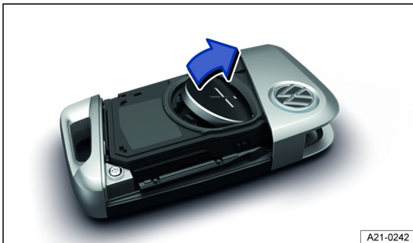
Fig. 45 Vehicle key: replacing the button cell battery
