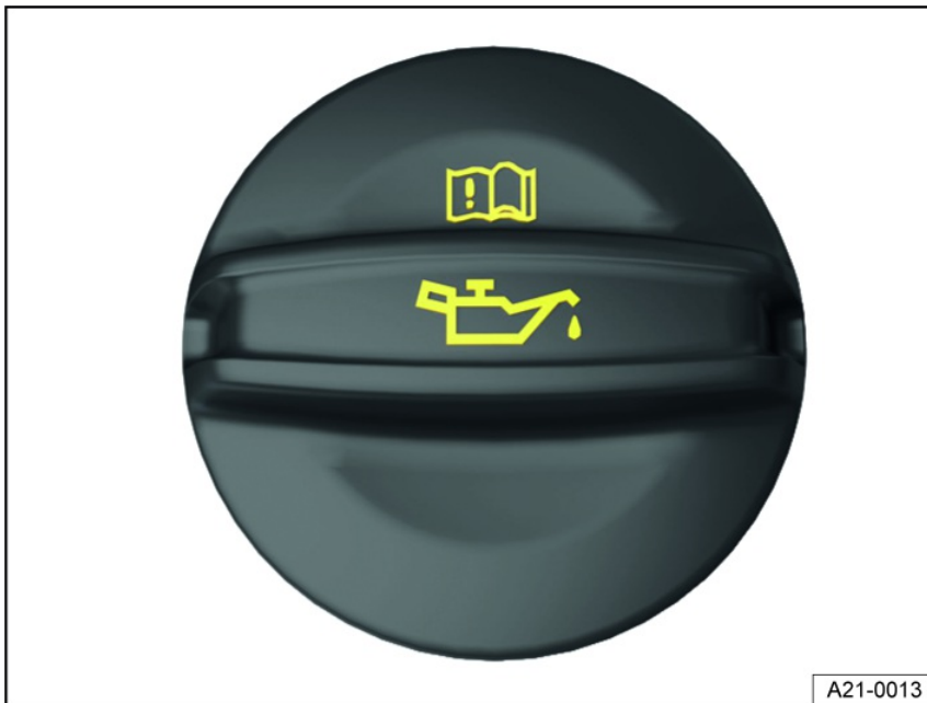
Fig. 154 In the engine compartment: engine oil filler cap (general example).
