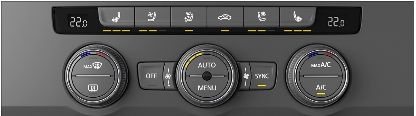
Fig. 83 In the upper section of the center console: Climate control bar for the Climatronic system.
