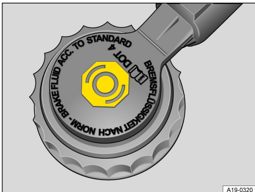
Fig. 158 In the engine compartment: cap on the brake fluid reservoir (version 1).
