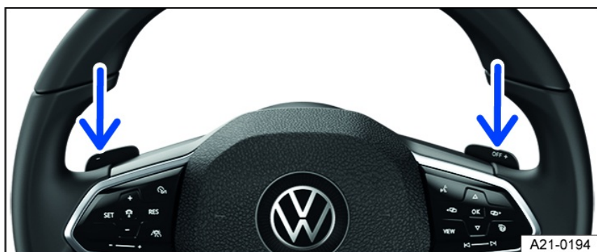
Fig. 93 Steering wheel with shift paddles for Tiptronic.
