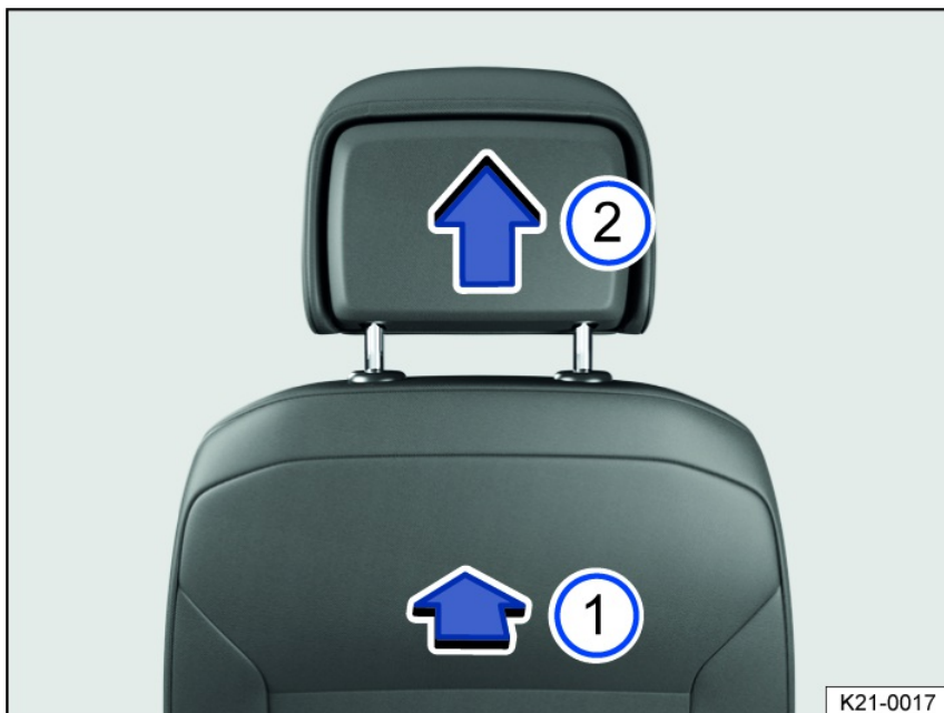
Fig. 67 General example: removing the front head restraint.
