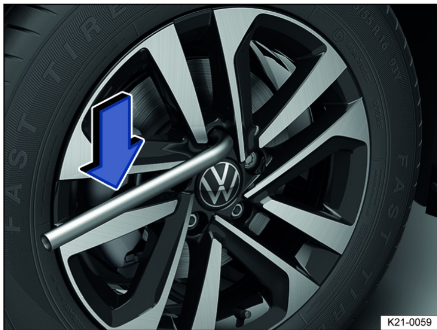
Fig. 176 Wheel change: removing wheel bolts with the lug wrench.
