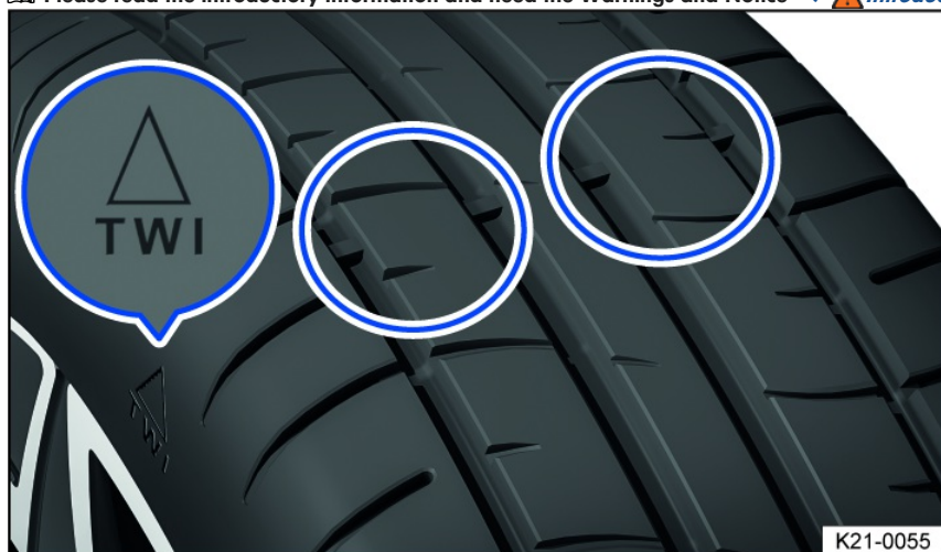
Fig. 163 Tire tread: tread wear indicator.
