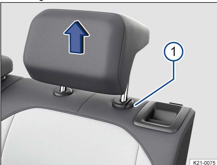
Fig. 2 Removing a rear head restraint (illustration).
