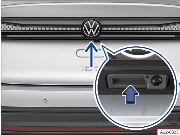
Fig. 1 In the boot lid: button for opening the boot lid (illustration).
