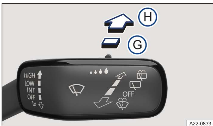
Fig. 2 On the right-hand side of the steering column: operating the rear window wiper.
