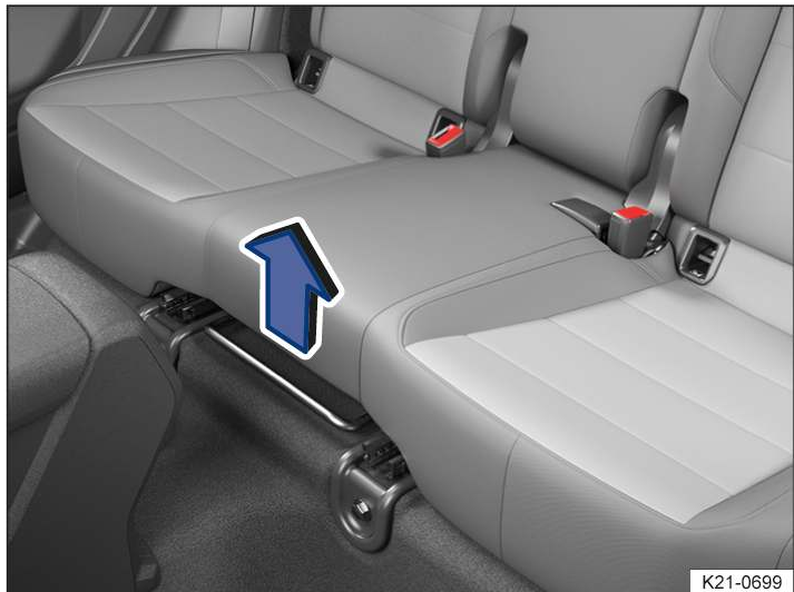
Fig. 1 Under the seat cushion of the rear bench seat: adjusting lever.
