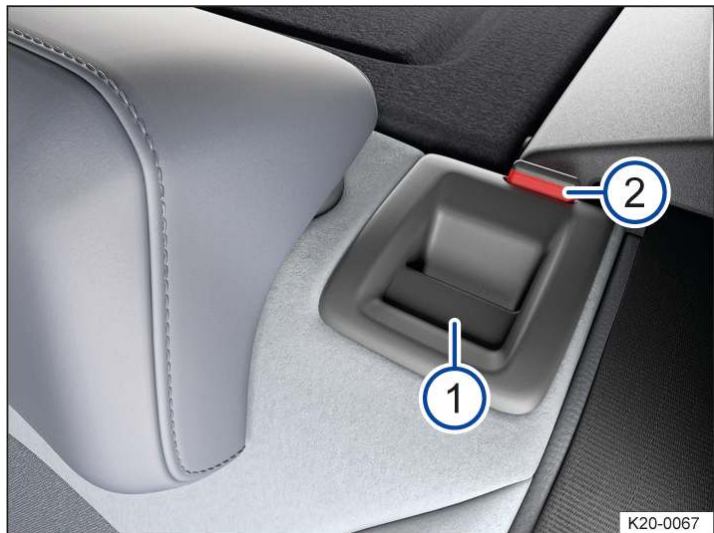
Fig. 1 In the rear seat backrest: release button.
