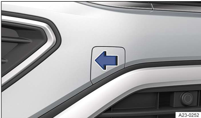
Fig. 1 In the front bumper on the right: removing the cover.
