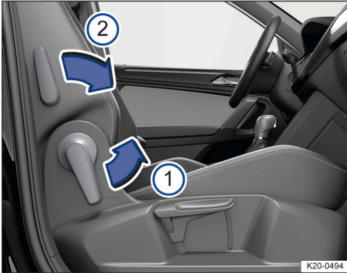
Fig. 1 Front passenger seat: folding backrest forwards.
