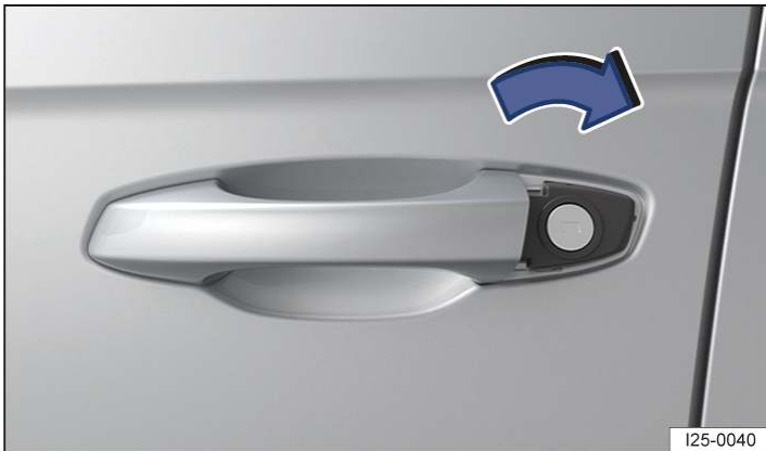
Fig. 2 Driver's door handle: manual closing.
