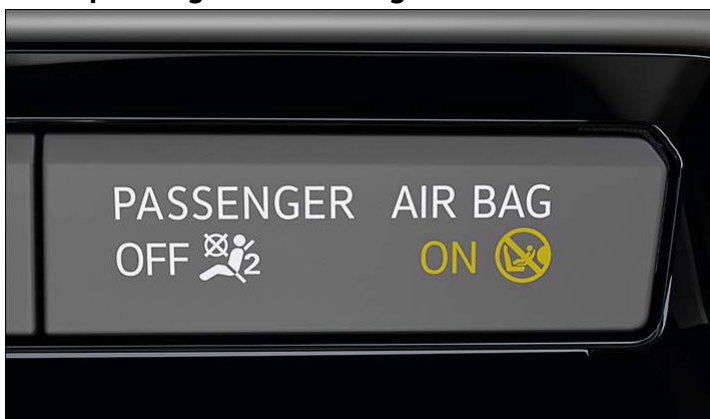
Fig. 2 In the centre console: indicator lamp for activated front passenger front airbag.
