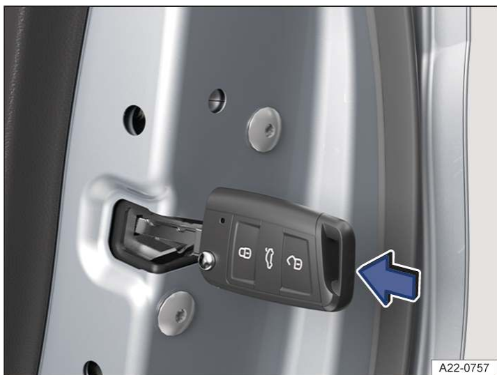
Fig. 2 In the front edge of the rear door: locking the vehicle manually with the key bit or manual key (variant 2).
