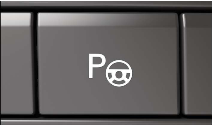
Fig. 1 In the upper section of the centre console: button for Park Assist.
