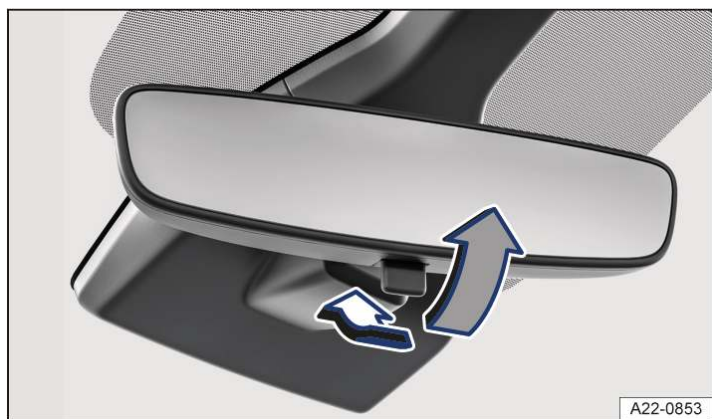
Fig. 2 On the windscreen: manual anti-dazzle interior mirror.
