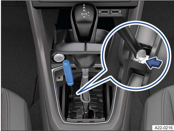
Fig. 1 In the centre console: releasing the selector lever lock manually.
