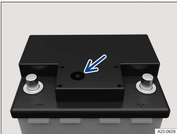
Fig. 1 On the top of the 12-volt vehicle battery: battery window (illustration).
