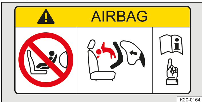
Fig. 3 On the sun visor: airbag label (illustration).
