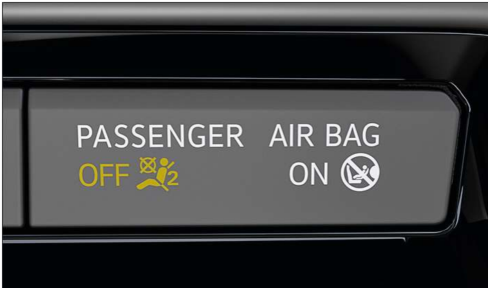
Fig. 3 In the centre console: indicator lamp for deactivated front passenger front airbag.
