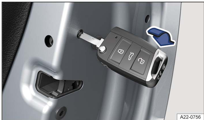
Fig. 1 In the front edge of the rear door: locking the vehicle manually with the key bit or manual key (variant 1).
