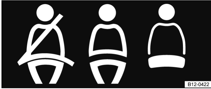
Fig. 1 On the instrument cluster display: fasten seat belt prompt for the rear seats (version 1).
