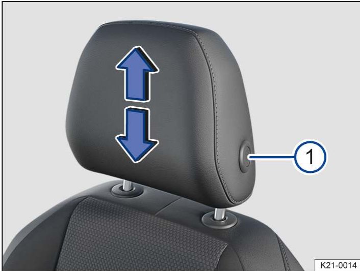
Fig. 1 Adjusting a front head restraint (illustration).
