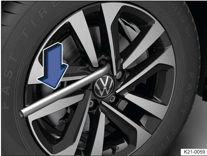
Fig. 1 Loosening wheel bolts.
