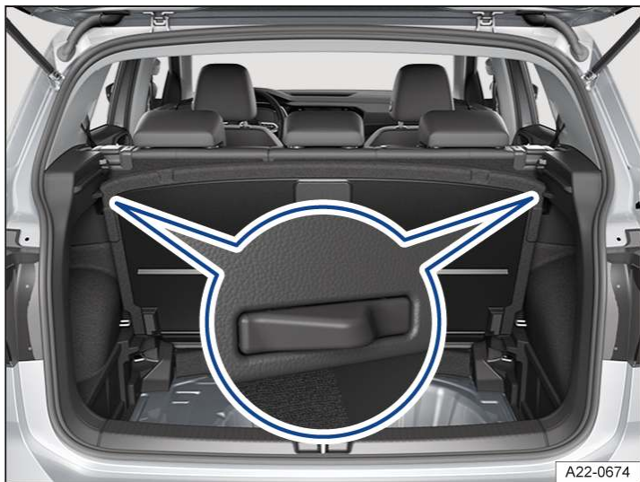
Fig. 2 In the luggage compartment: locking the variable luggage compartment floor in position.
