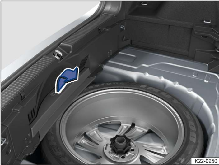
Fig. 1 Under the luggage compartment floor: cover over the spare wheel.
