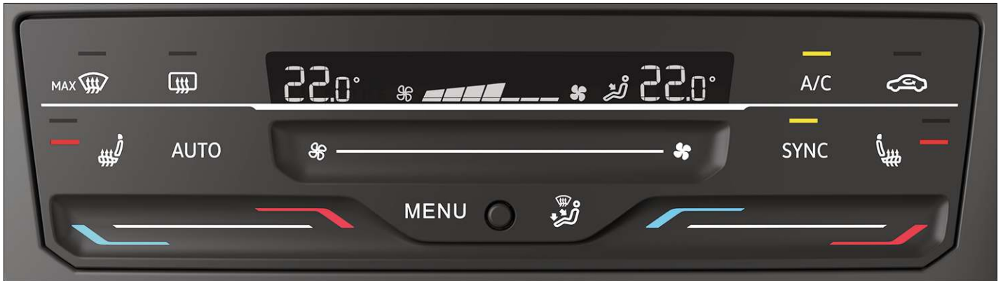
Fig. 1 In the upper part of the centre console: Climatronic air conditioning block.
