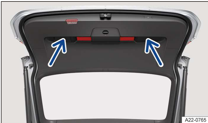
Fig. 2 In the open boot lid: handle recesses for closing the boot lid (illustration).
