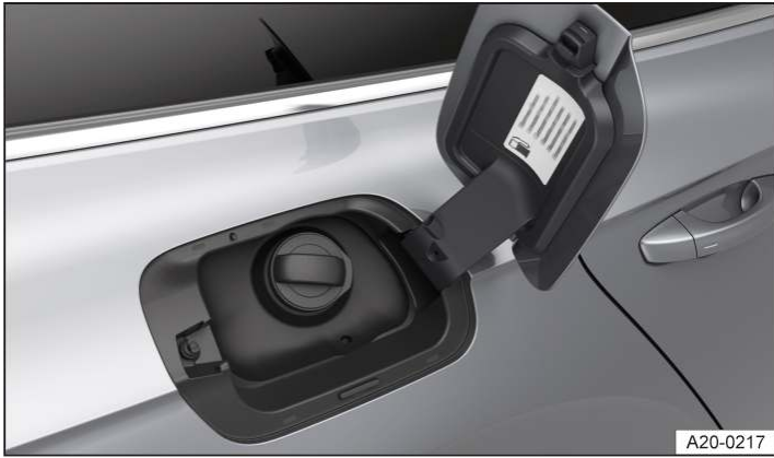
Fig. 1 Behind the tank flap: tank cap (illustration).
