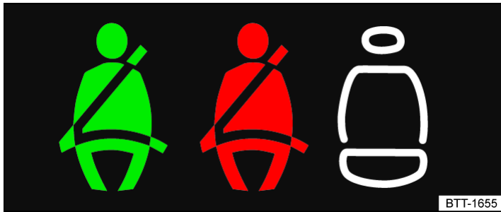
Fig. 2 On the instrument cluster display: fasten seat belt prompt for the rear seats (version 2).
