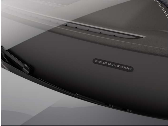
Fig. 1 In the windscreen: vehicle identification number.
