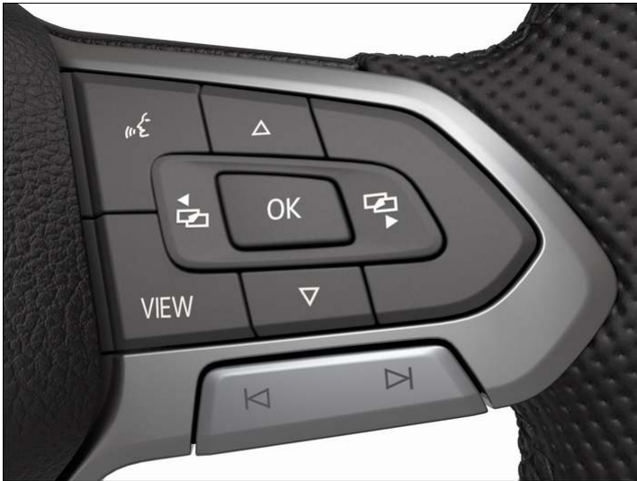
Fig. 1 Right side of the multifunction steering wheel: operating the digital instrument cluster Pro (illustration).
