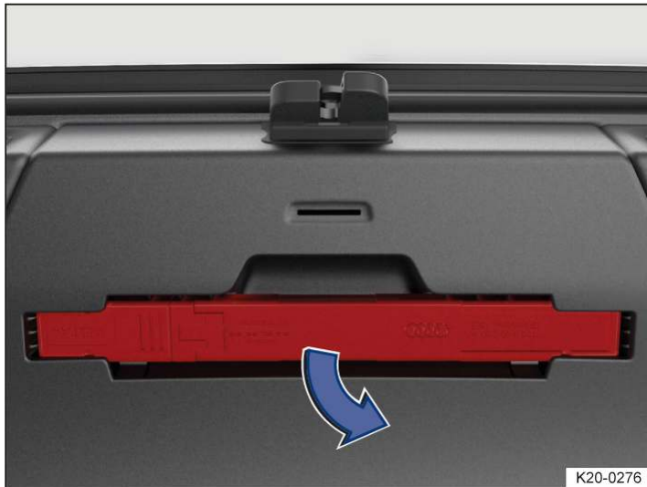
Fig. 1 In the boot lid: holder for the warning triangle.
