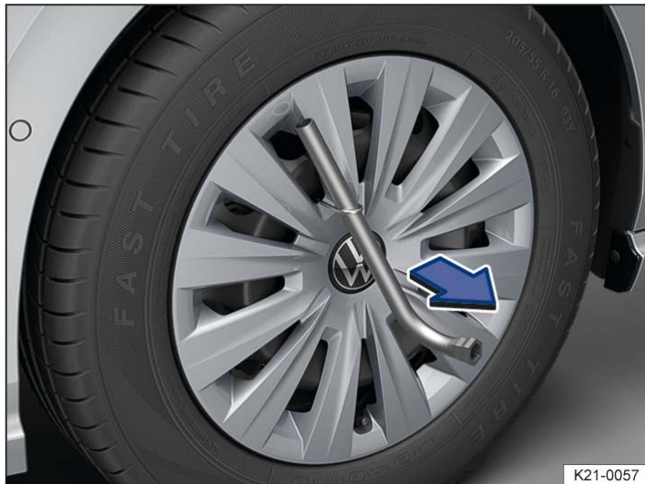
Fig. 1 Removing the wheel cover.
