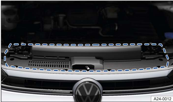
Fig. 1 Area for the engine oil sticker (illustration).
