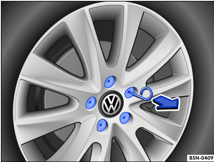
Fig. 1 Removing the wheel bolt caps.
