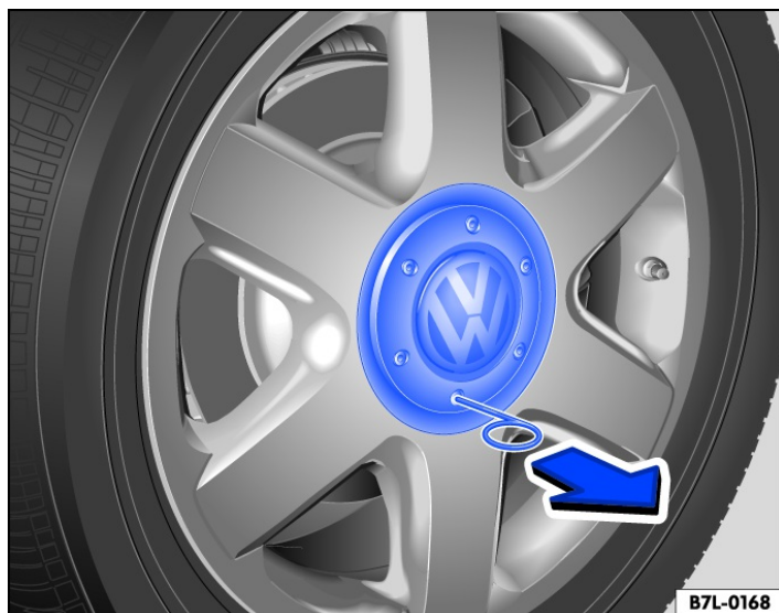
Fig. 1 Removing the centre wheel trim by pulling off.
