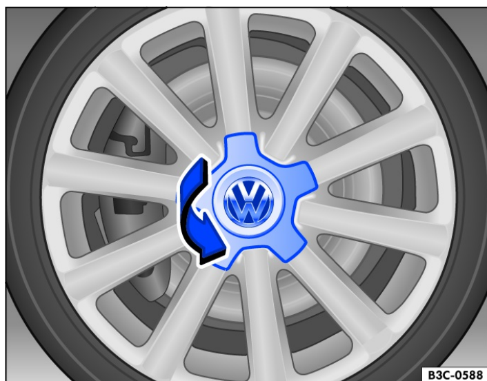
Fig. 2 Removing the centre wheel trim by turning.
