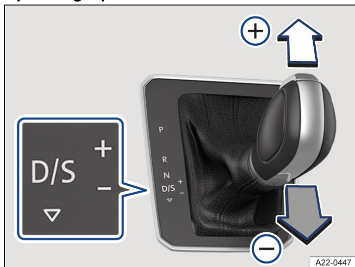
Fig. 1 In the centre console: selector lever in Tiptronic position.
