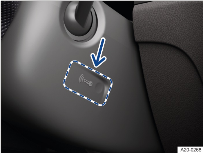
Fig. 1 On the right-hand side of the steering column: emergency start function in vehicles with the keyless locking and starting system Keyless Access.
