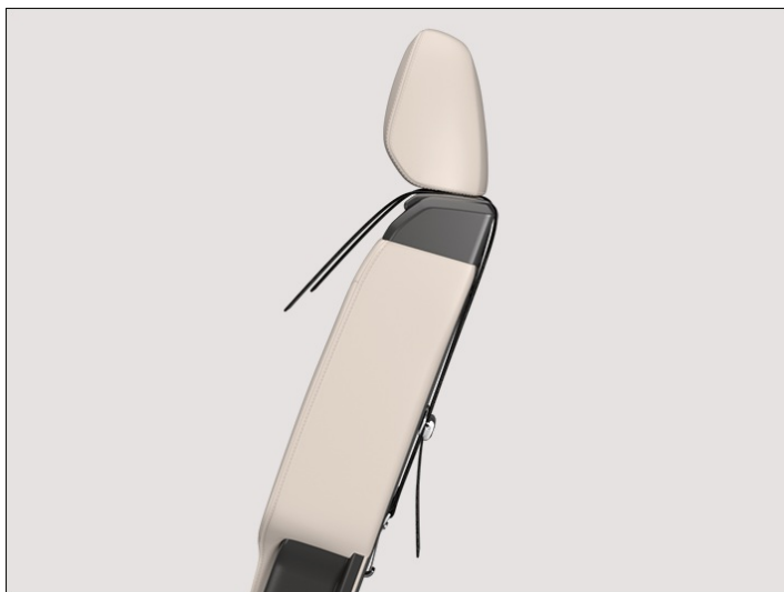
Fig. 4 On the rear of the outer seats of the rear bench seat or front passenger seat: attached top tether.
