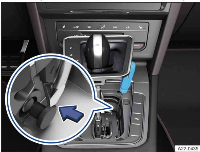
Fig. 1 In the centre console: releasing the selector lever lock manually (variant 1).
