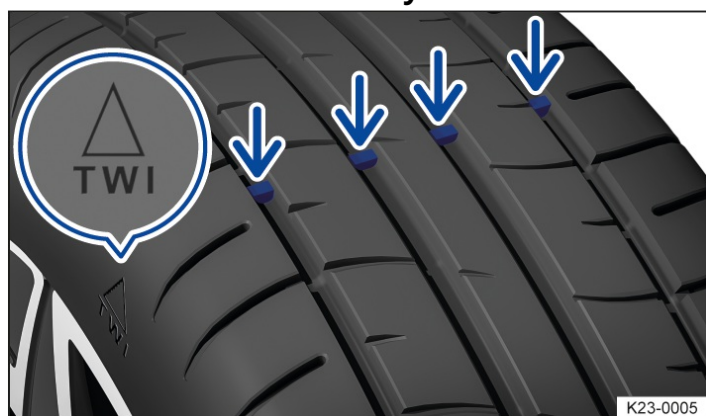
Fig. 1 In the tread grooves: tread wear indicator.
