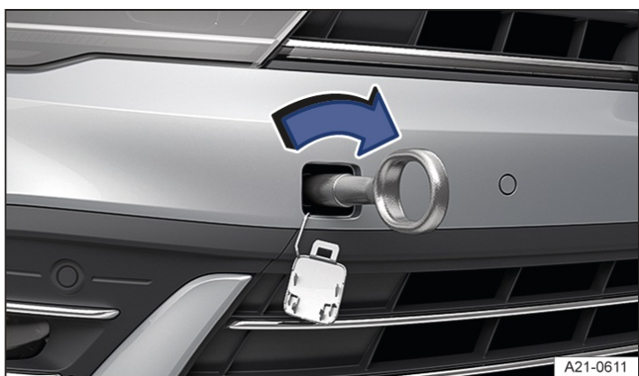
Fig. 3 In the front bumper on the right: screwing in the towing eye, variant 1.
