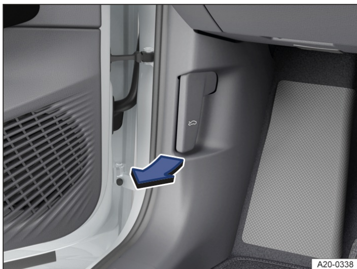
Fig. 1 In the footwell on the driver side: bonnet release lever (schematic diagram).
