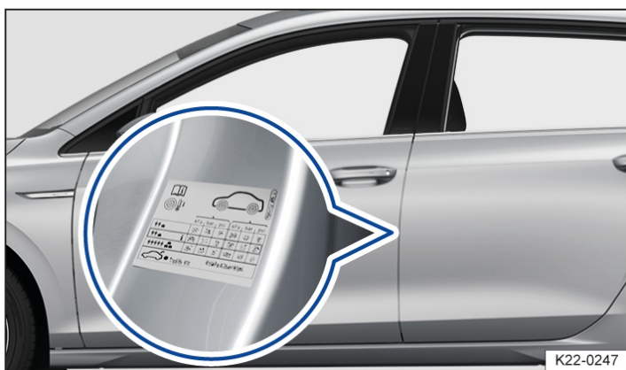
Fig. 2 On the driver door pillar: tyre pressure sticker (alternatively on the inside of the tank flap)
