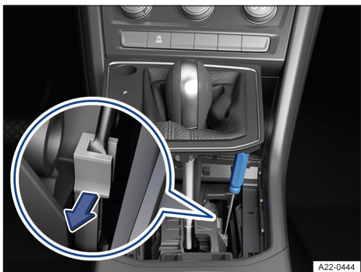
Fig. 2 In the centre console: releasing the selector lever lock manually (variant 2).
