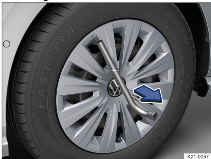
Fig. 1 Removing the wheel cover.
