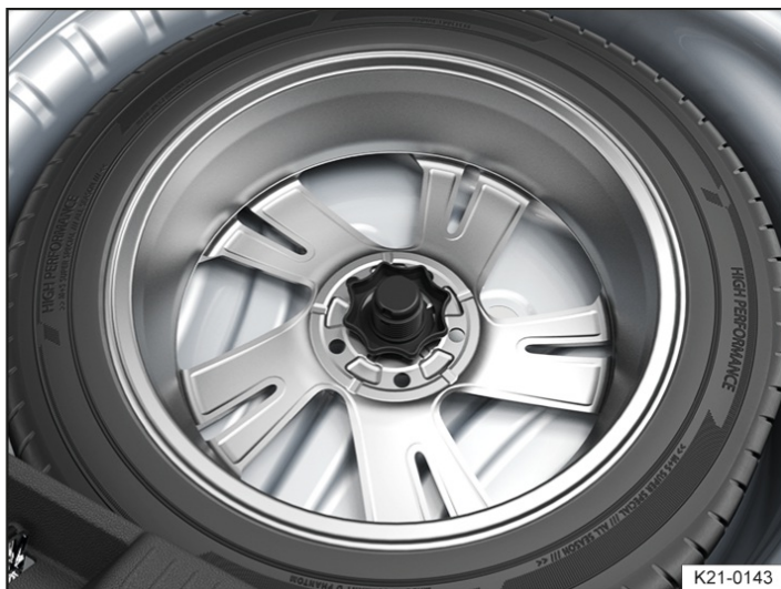
Fig. 1 Under the luggage compartment floor: handwheel for securing the spare wheel or temporary spare wheel.
