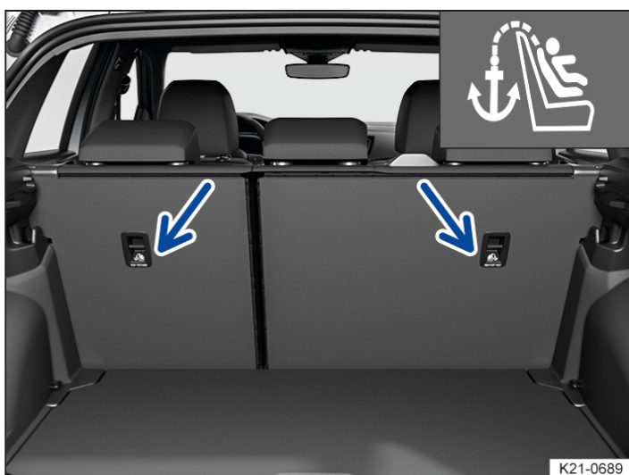
Fig. 1 On the rear of the rear bench seat: top tether anchor points for top tether.
