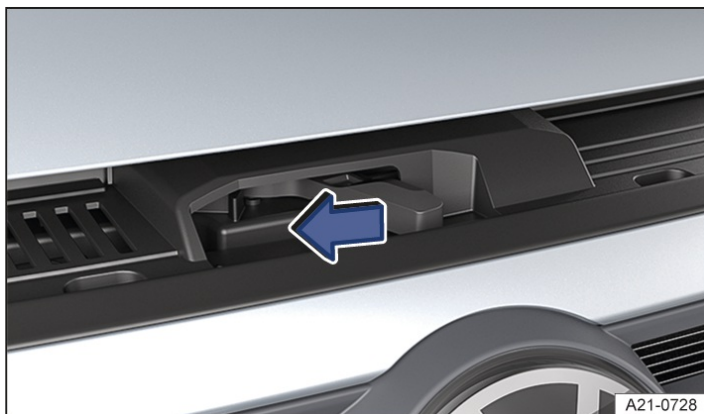
Fig. 2 Above the radiator grille: bonnet control lever.
