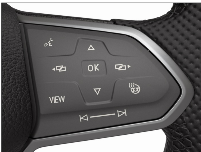
Fig. 2 Right side of the multifunction steering wheel: operating the digital instrument cluster Basic (variant 2).
