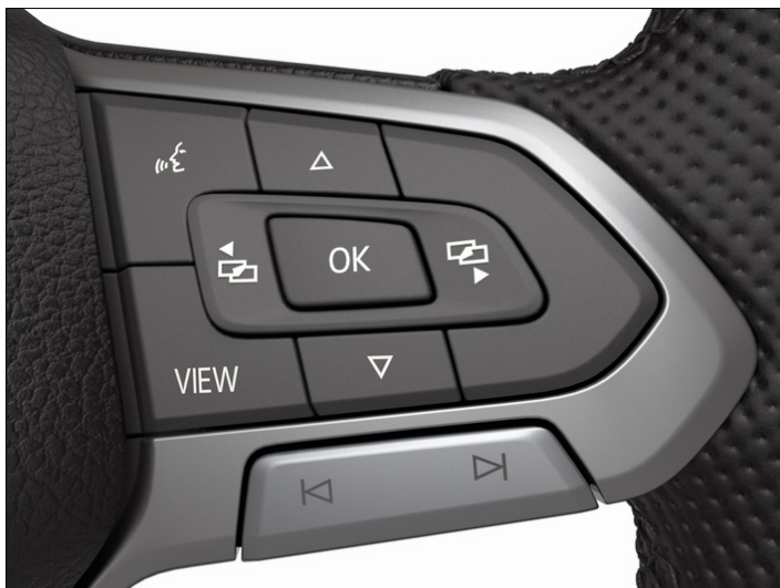
Fig. 1 Right side of the multifunction steering wheel: operating the digital instrument cluster Basic (variant 1).
