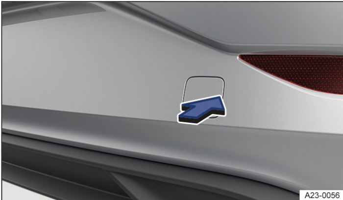
Fig. 1 In the rear bumper on the right: removing the cover.
