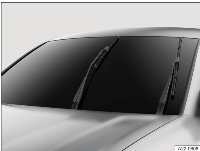
Fig. 1 Wipers in service position (illustration).
