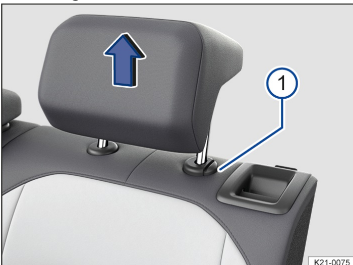
Fig. 2 Removing a rear head restraint (illustration).
