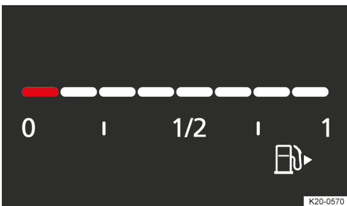
Fig. 2 In the digital instrument cluster Basic: fuel gauge (illustration).
