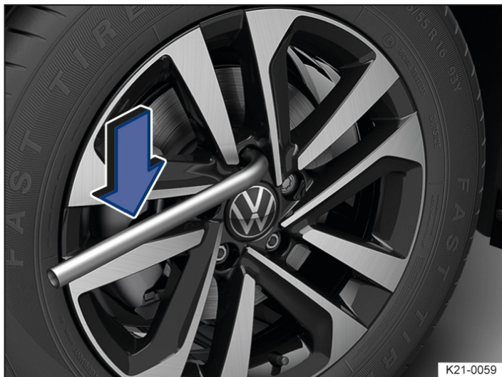
Fig. 1 Loosening wheel bolts.
