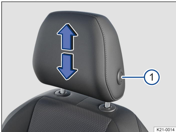
Fig. 1 Adjusting a front head restraint(illustration).
