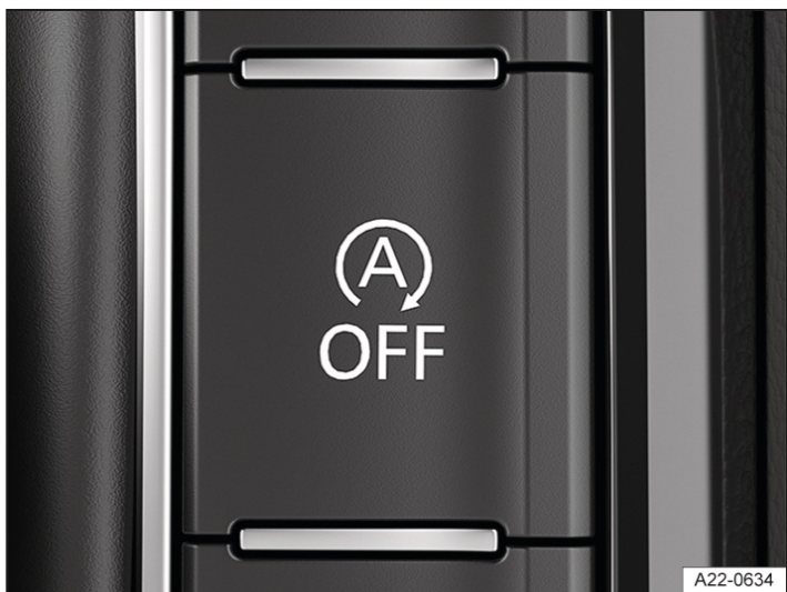
Fig. 1 In the lower part of the centre console or in the Infotainment system (depending on equipment): button for the start/stop system.
