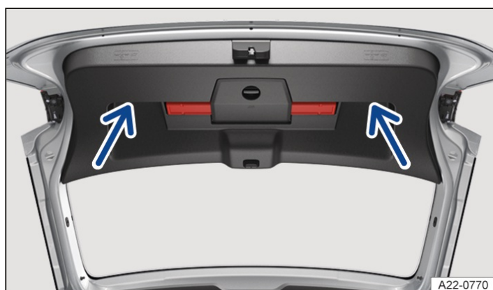
Fig. 1 In the open boot lid: handle recesses for closing the boot lid
