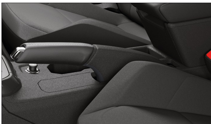
Fig. 1 Between the front seats: handbrake with lock button (illustration).
