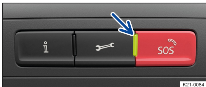
Fig. 1 In the roof console: control for legally required eCall Emergency System and indicator lamp.
