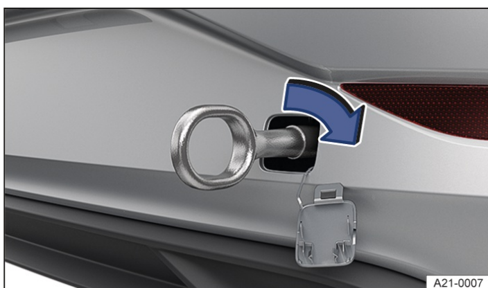
Fig. 2 In the rear bumper on the right: screwing in the towing eye.
