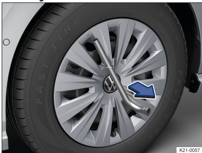
Fig. 1 Removing the wheel cover.
