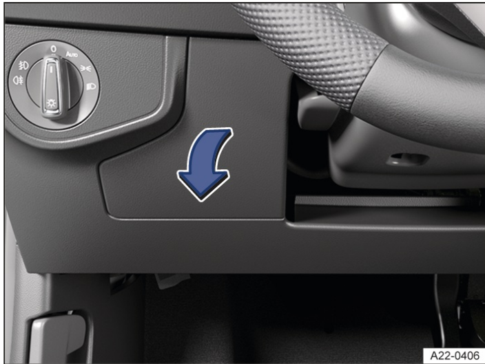
Fig. 1 In the dash panel on the driver side: fuse box cover(left-hand drive vehicle).
