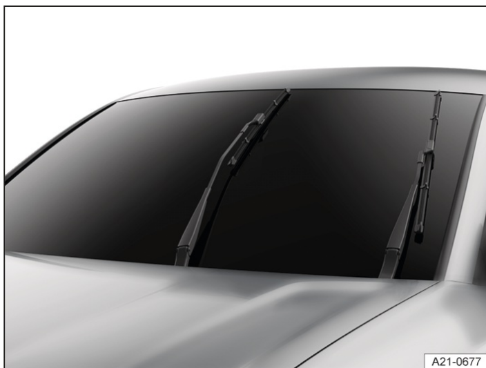
Fig. 1 Wipers in service position (illustration).
