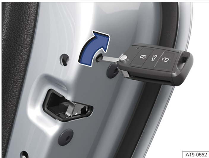
Fig. 1 In the front edge of the rear right-hand door: manually locking the vehicle with the vehicle key (illustration).
