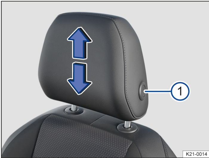
Fig. 1 Adjusting a front head restraint (illustration).
