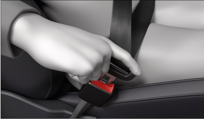
Fig. 1 Inserting the seat belt latch plate into the buckle.
