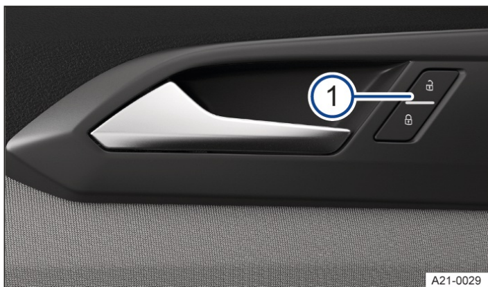
Fig. 1 In the driver door: central locking button (illustration).
