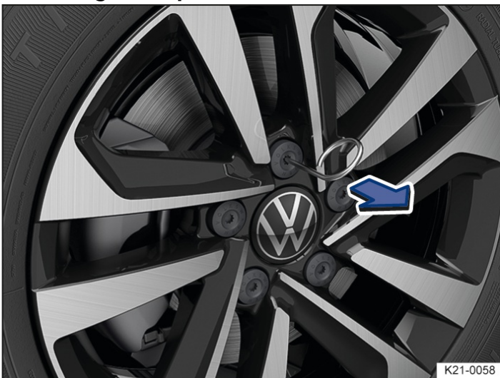
Fig. 1 Removing the wheel bolt caps.
