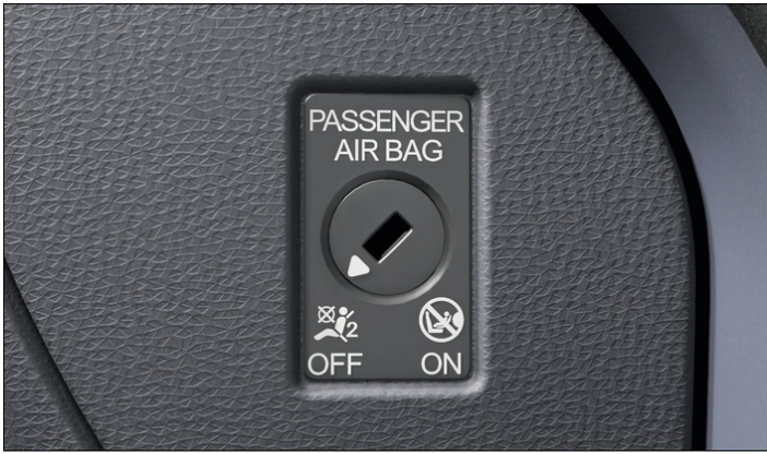
Fig. 1 In the dash panel on the front passenger side: key-operated switch for switching the front airbag on the front passenger side on and off.
