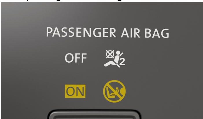
Fig. 2 In the centre console: indicator lamp for activated front passenger front airbag (depending on country).
