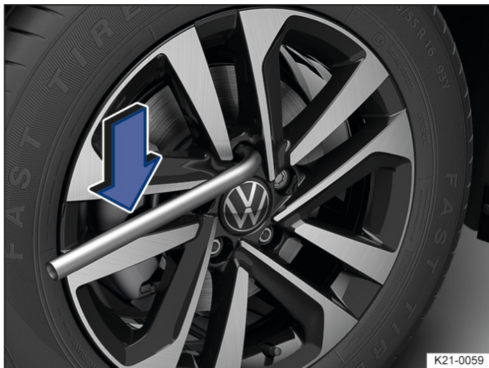
Fig. 1 Changing a wheel: loosening the wheel bolts.
