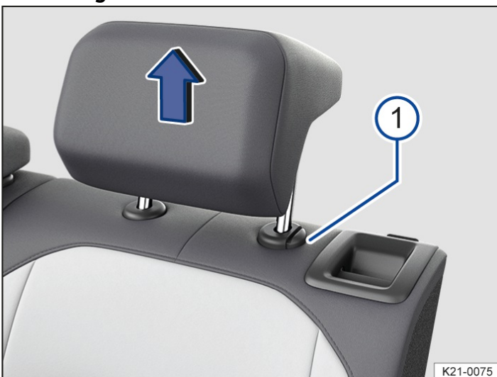
Fig. 2 Removing a rear head restraint(illustration).
