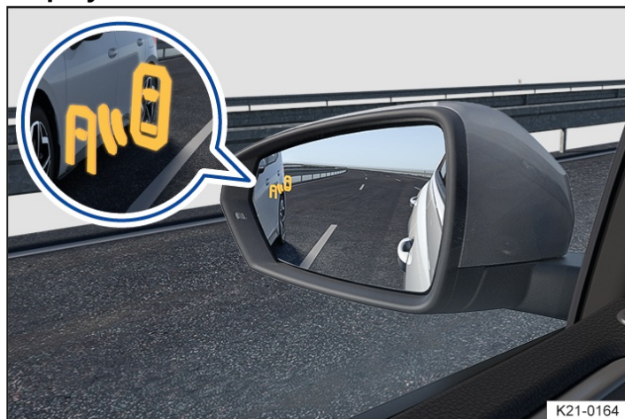
Fig. 1 In the exterior mirrors: Side Assist display.
