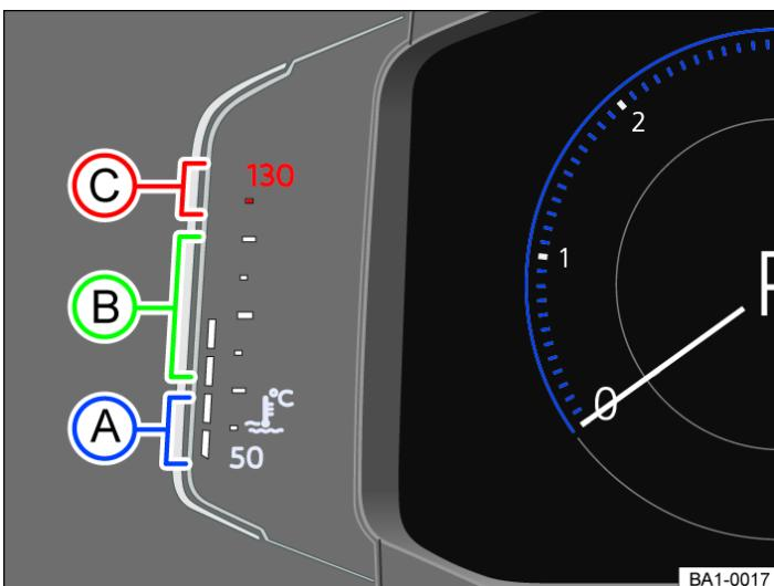
Fig. 2 Coolant temperature gauge in the Active Info Display.
