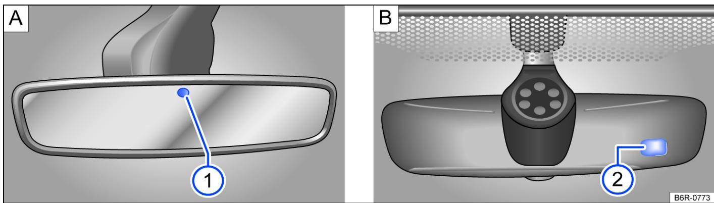
Fig. 1 On the windscreen: automatic anti-dazzle interior mirror.
