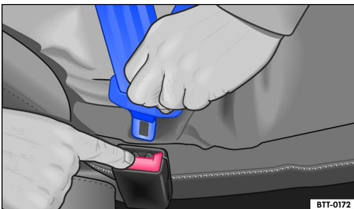
Fig. 2 Removing the latch plate from the buckle.
