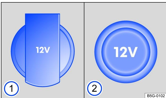
Fig. 1 In the front centre console: fold-open 12-volt socket 1 or 12-volt socket with removable cover 2.
