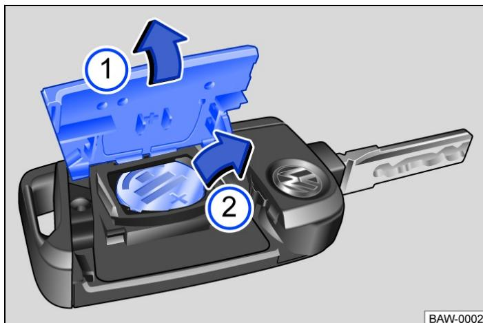
Fig. 1 Vehicle key: replacing the button cell.
