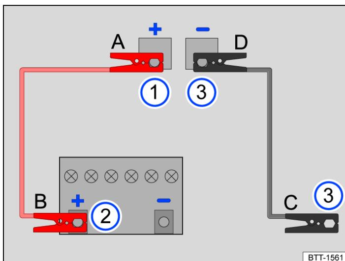
Fig. 2 Diagram showing how to connect jump leads on the vehicle providing the jump start (12-volt battery in luggage compartment).
