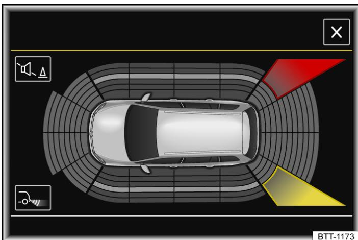
Fig. 2 Infotainment system screen display: Rear Traffic Alert.
