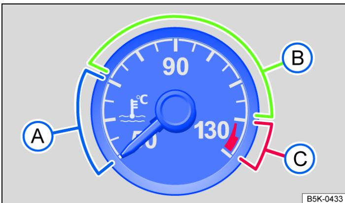
Fig. 1 Coolant temperature display in the analogue instrument cluster.
