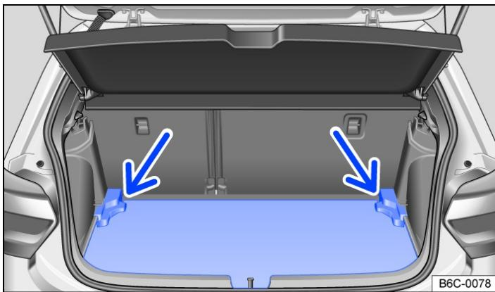
Fig. 2 In the luggage compartment: lowering the luggage compartment floor.
