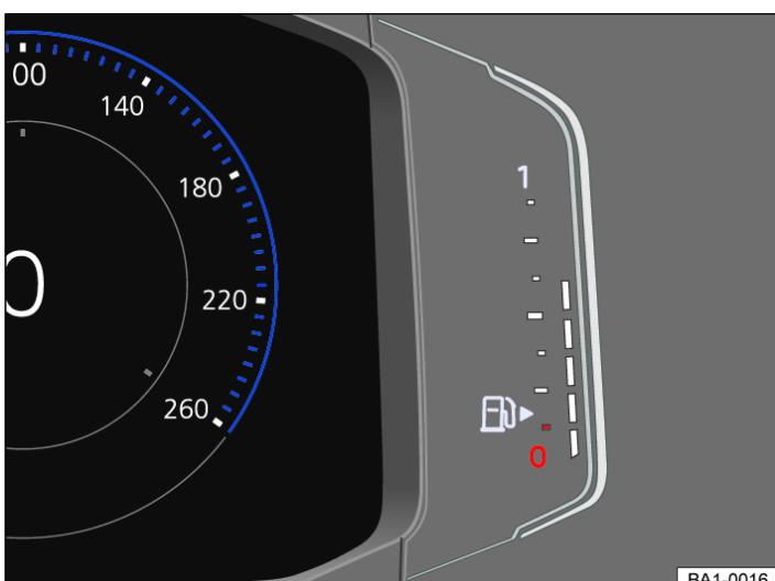
Fig. 4 Fuel gauge in the Active Info Display.
