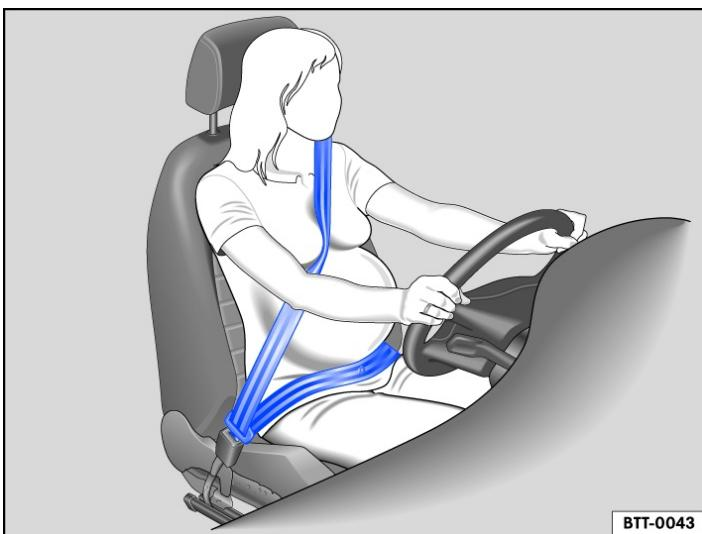
Fig. 2 Correct seat belt routing during pregnancy.
