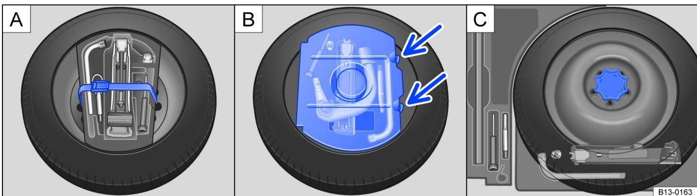
Fig. 1 In the luggage compartment under the floor covering: **A**: spare wheel and vehicle toolkit without ball head (variant 1), **B** : spare wheel and vehicle toolkit with ball head (variant 2), **C**: spare wheel and vehicle toolkit without ball head (variant 3).
