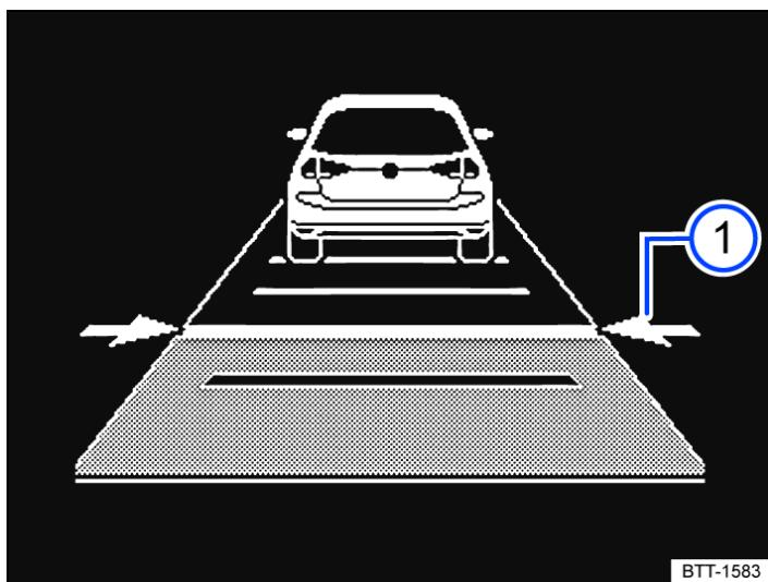
Fig. 1 On the instrument cluster display: setting the distance (illustration, the ACC is active).
