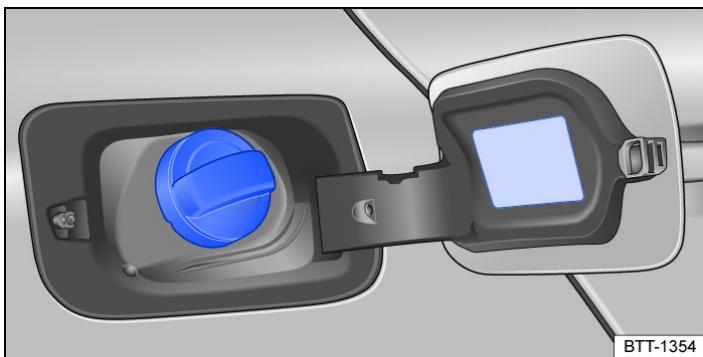
Fig. 1 Behind the tank flap: tank cap (illustration).
