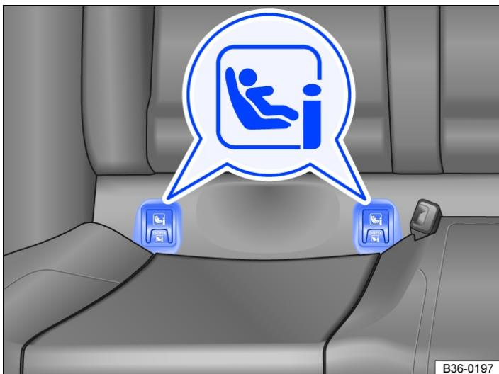
Fig. 1 Markings identifying the ISOFIX anchor points for child seats.
