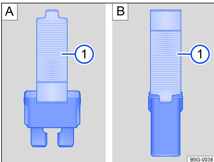
Fig. 2 Removing or inserting a fuse with plastic pliers: **A**: flat blade fuse, **B**: cartridge fuse.
