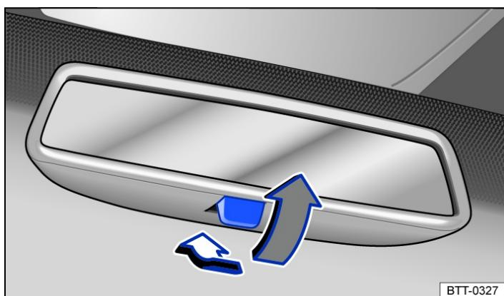
Fig. 2 On the windscreen: manual anti-dazzle interior mirror.
