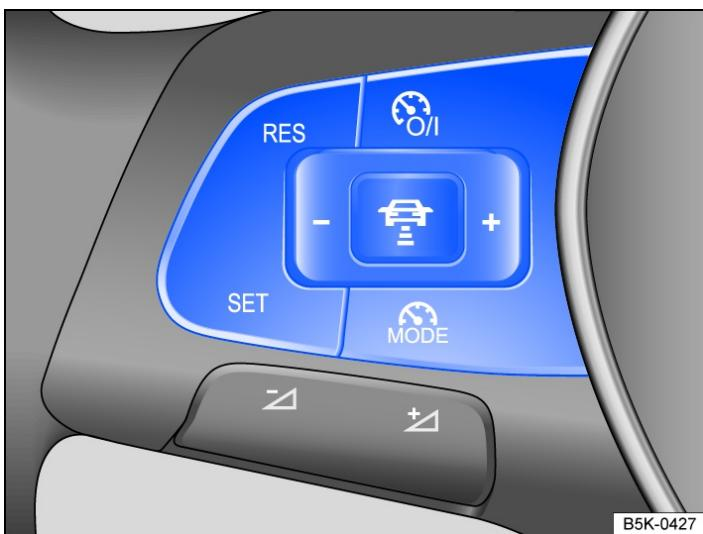
Fig. 1 Left-hand side of the multifunction steering wheel: buttons for operating the ACC.
