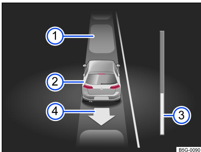
Fig. 1 On the instrument cluster display: driving out of a parallel parking space.
