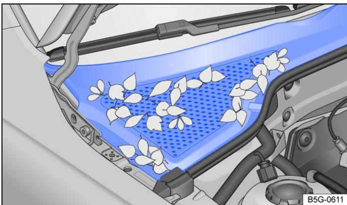
Fig. 1 Between the engine compartment and the windscreens: plenum chamber (illustration).
