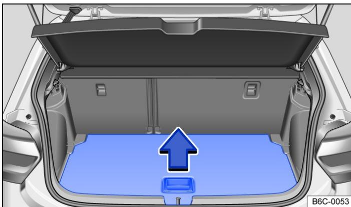
Fig. 1 In the luggage compartment: opening the luggage compartment floor.
