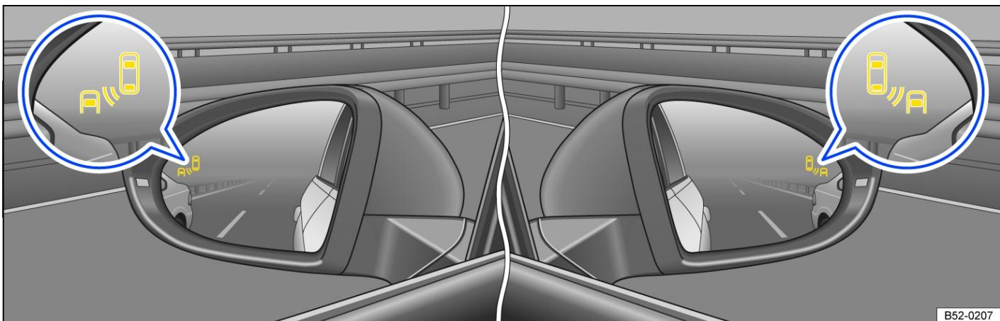
Fig. 1 In the wing mirrors: Blind Spot Monitor display.
