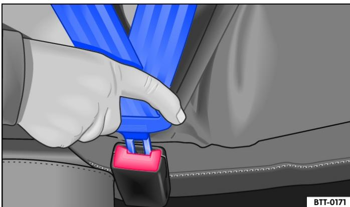
Fig. 1 Inserting the seat belt latch plate into the buckle.
