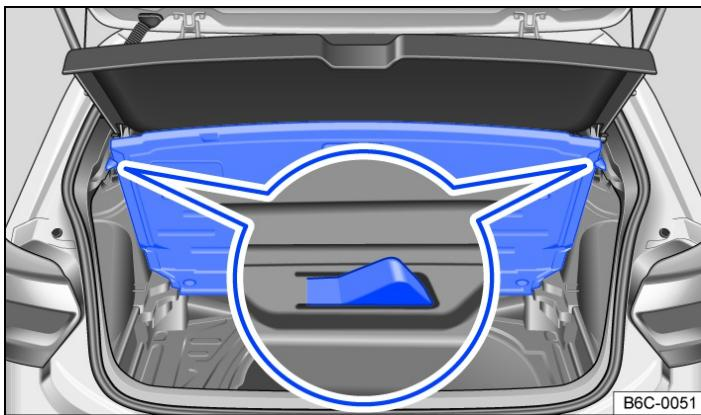
Fig. 2 In the luggage compartment: locking the luggage compartment floor in position.
