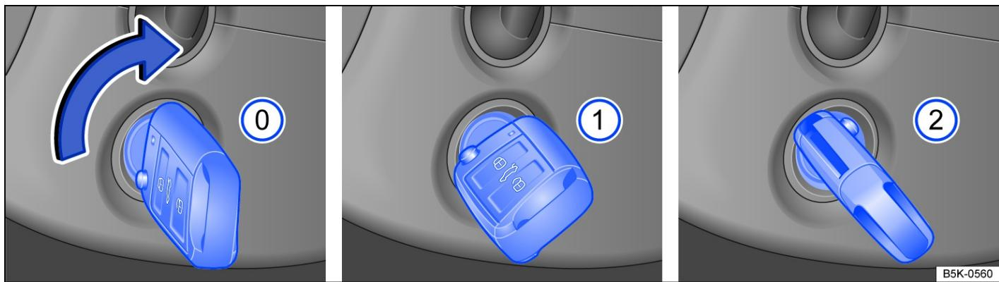
Fig. 1 To the right of the steering wheel: positions of the vehicle key in the ignition lock.
