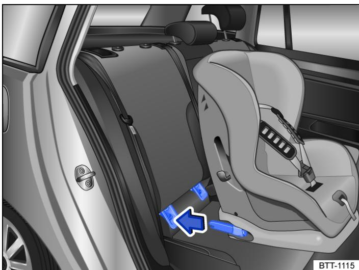
Fig. 2 Illustration: fitting an ISOFIX child seat with the attachment arms.
