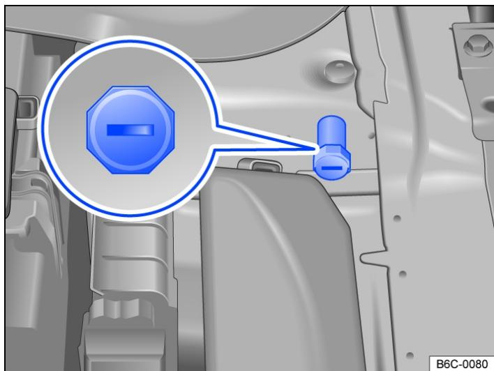
Fig. 1 In the engine compartment: jump lead connection point (earth connection).
