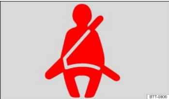
Fig. 55 Warning light in the instrument cluster.
