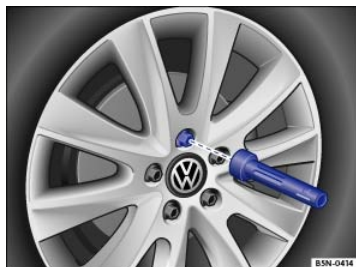
Fig. 199 Changing a wheel: remove previously loosened wheel bolts using the screwdriver handle.
