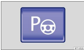
Fig. 155 In the lower center console: Button for switching on the Park Assist system.
