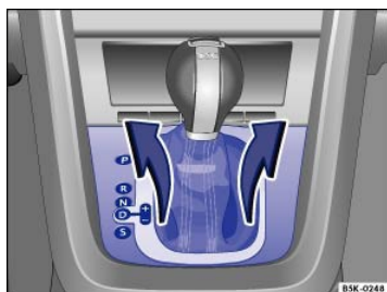
Fig. 189 Removing the selector gate cover.
