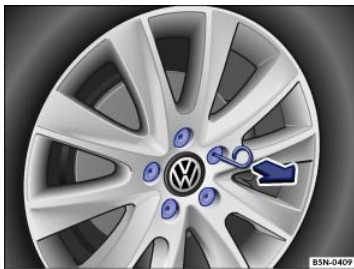
Fig. 193 Pulling cover caps off wheel bolts.
