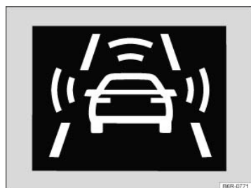
Fig. 143 In the instrument cluster display: Advance warning (symbol displayed in color on an instrument cluster with color display).
