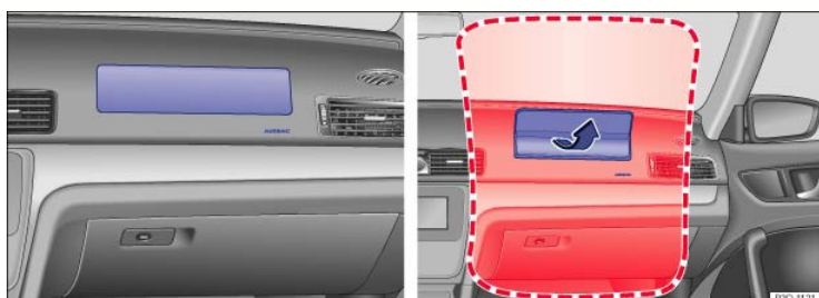
Fig. 70 Location and deployment zone of the front passenger front airbag.
