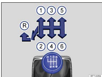
Fig. 125 Gearshift pattern of a 6-speed manual transmission.
