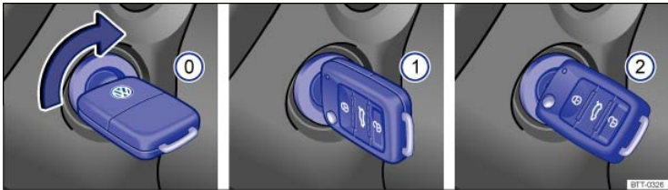
Fig. 118 In the ignition switch: Vehicle key positions.
