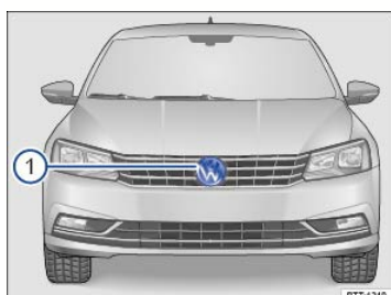
Fig. 144 In the front bumper: Radar sensor.
