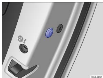
Fig. 183 On the front side of the right rear door: Emergency lock, covered by a rubber seal.
