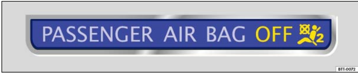
Fig. 68 PASSENGER AIR BAG light on the instrument panel.
