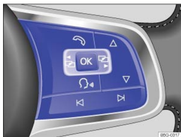
Fig. 11 Premium version (vehicles with menu control multi-function steering wheel): Buttons on the right side of the steering wheel.
