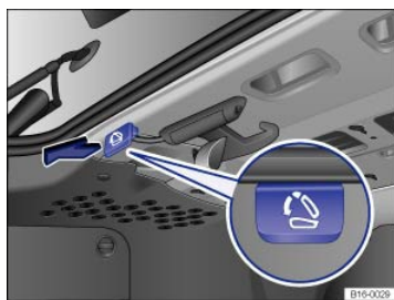
Fig. 93 On the left side of the luggage compartment: Release lever for the left-side rear seat backrest. The release lever for the right-side rear seat backrest is on the right side of the luggage compartment.
