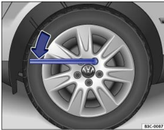
Fig. 195 Changing a wheel: Loosening wheel bolts.
