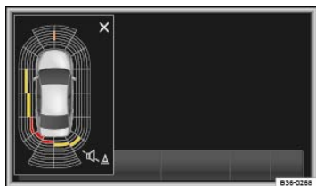
Fig. 154 Mini PDC display of the area surrounding the vehicle.
