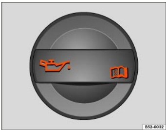
Fig. 172 In the engine compartment: Engine oil filler cap.
