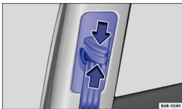
Fig. 65 Next to the front seats: Safety belt height adjuster.
