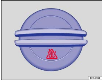
Fig. 175 Coolant expansion tank cap in the engine compartment.
