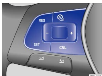
Fig. 134 Left-hand side of the multi-function steering wheel: Buttons for operating the cruise control.
