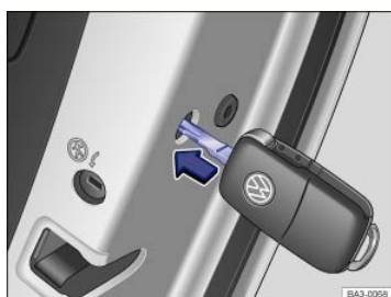
Fig. 184 On the front side of the right rear door: Manual vehicle locking with the key bit in the vehicle key.
