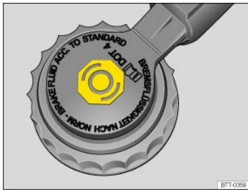
Fig. 130 In engine compartment: Brake fluid reservoir cap.
