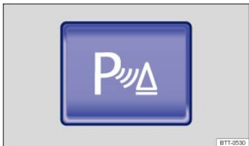
Fig. 152 In the lower center console: Button to switch the Park Distance Control system on or off.
