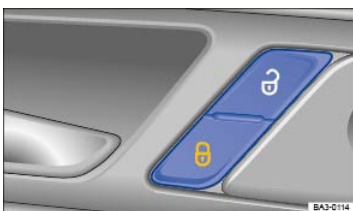
Fig. 26 In the driver and front passenger doors: power locking button.
