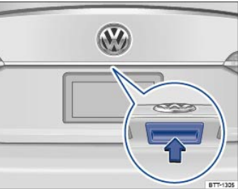
Fig. 32 Opening trunk lid from the outside.
