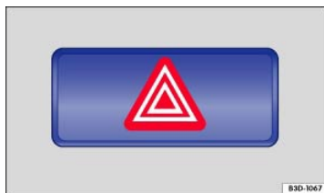
Fig. 181 In the center of the instrument panel: Switch for emergency flashers.
