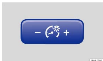
Fig. 82 To the left of the steering wheel: Control for instrument panel lighting.
