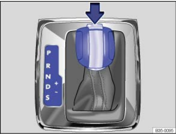
Fig. 126 Automatic transmission selector lever with shift lever release button (arrow).
