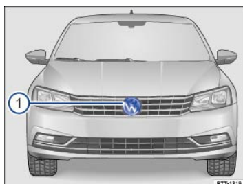
Fig. 137 Behind the Volkswagen emblem: Radar sensor.
