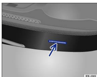
Fig. 15 Vehicle identification number (VIN).
