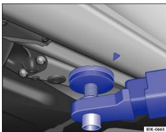
Fig. 180 Rear lift point for workshop hoist or floor jack.
