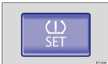
Fig. 105 In the glove compartment: SET button for the Tire Pressure Monitoring System.
