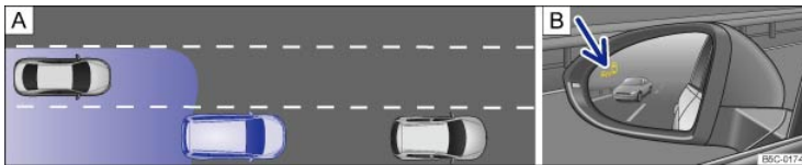
Fig. 160 : Driving situation when passing with traffic behind your vehicle. : Blind Spot Monitor indicator light in the driver side mirror.
