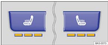
Fig. 52 In the center console: Seat heating control for front seats.
