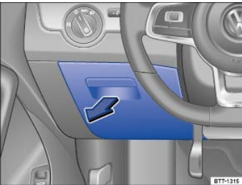
Fig. 200 On the driver side in the instrument panel: Fuse box behind the storage compartment.
