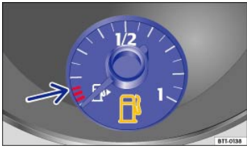
Fig. 167 In the instrument cluster: Fuel gauge.
