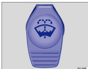
Fig. 89 In the engine compartment: Cap of the windshield washer fluid reservoir.
