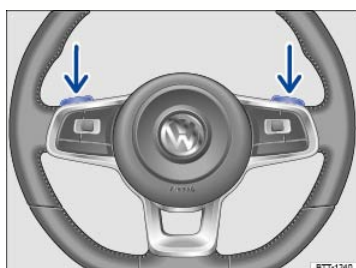
Fig. 128 Steering wheel with optional Tiptronic shift paddles.
