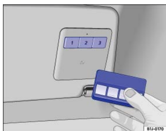
Fig. 37 In the driver side sun visor: The remote control and buttons for the HomeLink Universal Transmitter.
