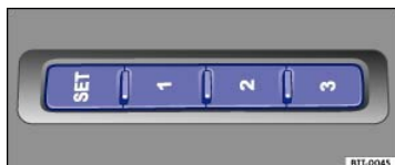
Fig. 54 Memory buttons on the outer side of the driver seat.
