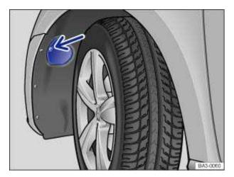
Fig. 217 In the wheel housing: Removing cover.
