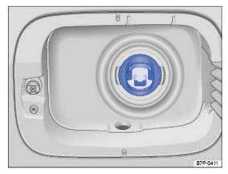
Fig. 163 With open fuel cap: Misfueling guard in the fuel filler neck.
