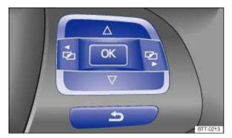
Fig. 15 Premium version (vehicles with menu control multi-function steering wheel): buttons on the right side of the steering wheel.
