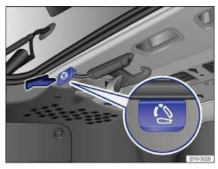
Fig. 110 On the left side of the luggage compartment: Release lever for the left-side rear seat backrest. The release lever for the right-side rear seat backrest is on the right side of the luggage compartment.
