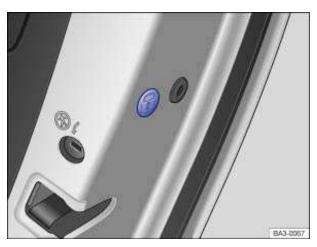
Fig. 195 On the front side of the right rear door: Emergency lock, covered by a rubber seal.
