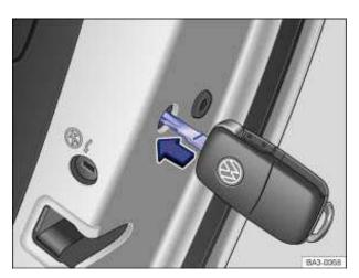
Fig. 196 On the front side of the right rear door: Manual vehicle locking with the key bit in the vehicle key.
