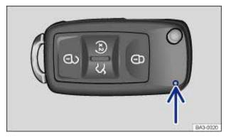
Fig. 26 Indicator light in the remote control vehicle key (version 2).
