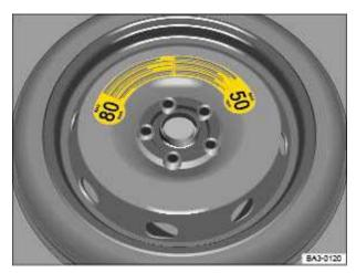
Fig. 183 In the luggage compartment: Compact spare wheel.
