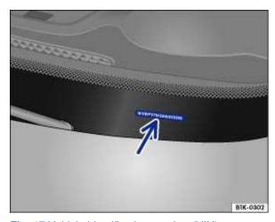
Fig. 17 Vehicle identification number (VIN).
