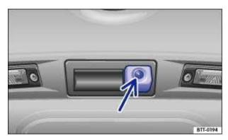
Fig. 149 In the luggage compartment lid: Location of the Rear Assist camera.
