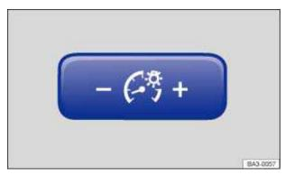
Fig. 98 To the left of the steering wheel: Control for instrument panel lighting.
