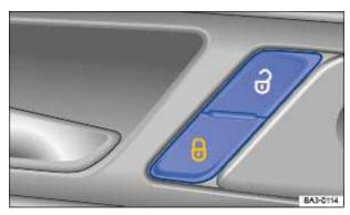
Fig. 35 In the driver and front passenger doors: power locking button.
