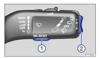
**Fig. 14** Basic version (Vehicles without menu control multi-function steering wheel): control buttons 1 and 2 on the windshield wiper lever.
