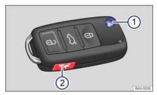
Fig. 20 Remote control vehicle key without remote start feature.
