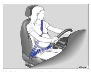
Fig. 76 Proper safety belt positioning for expectant mothers.
