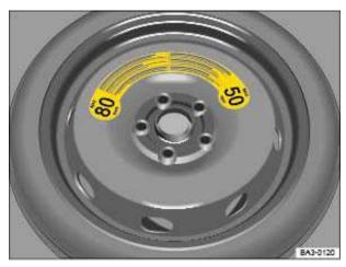
Fig. 182 In the luggage compartment: Compact spare wheel.
