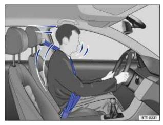
Fig. 72 Belted driver secured by the correctly worn safety belt in the event of a sudden braking maneuver.
