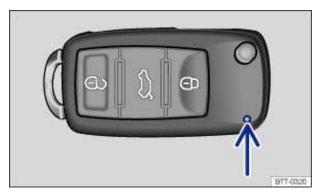
Fig. 25 Indicator light in the remote control vehicle key (version 1).
