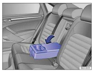
Fig. 64 Folded down rear center armrest with storage compartment (arrow).
