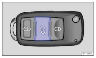
Fig. 42 In the remote control vehicle key: Button to unlock and open the luggage compartment lid.
