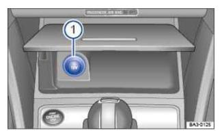
Fig. 131 12 Volt socket in the front center console.
