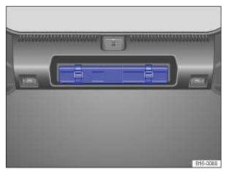
Fig. 190 In the luggage compartment: holder for the warning triangle (version 1).
