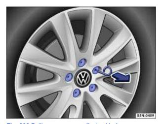
Fig. 206 Pulling cover caps off wheel bolts.
