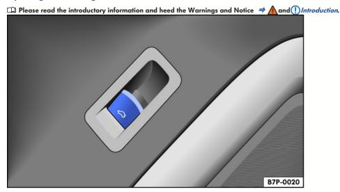
Fig. 61 In the driver's door: unlock button for the trunk lid.
