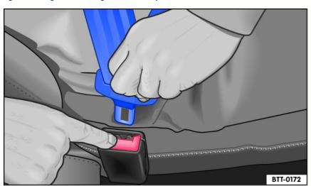
Fig. 29 Releasing the buckle tongue from the safety belt buckle.
