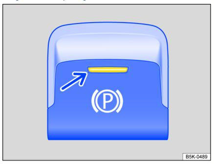
Fig. 116 In the center console: button for the electronic parking brake (general example).
