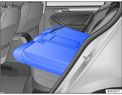
Fig. 72 Rear bench seat: Rear seat backrest folded forwards.
