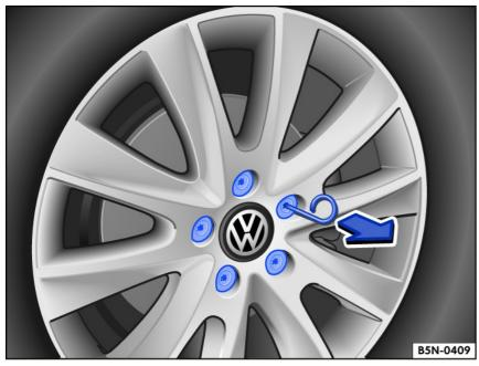
Fig. 173 Remove the caps from the wheel bolts.
