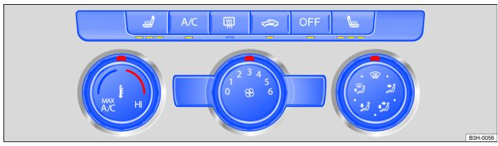
Fig. 89 In the upper section of the center console: climate control toolbar for the manual climate control system.
