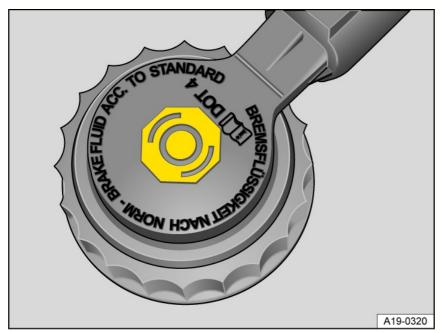
Fig. 162 In the engine compartment: cap on the brake fluid reservoir variant A.
