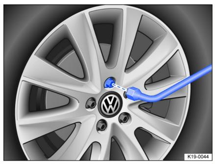
Fig. 182 Wheel change: removing wheel bolts with the lug wrench.
