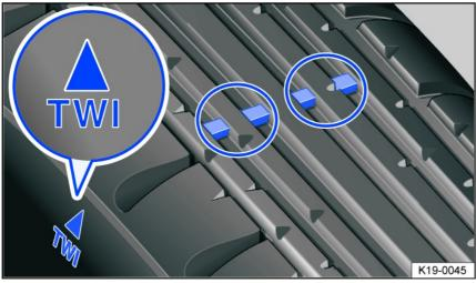
Fig. 168 Tire tread: tread wear indicator.
