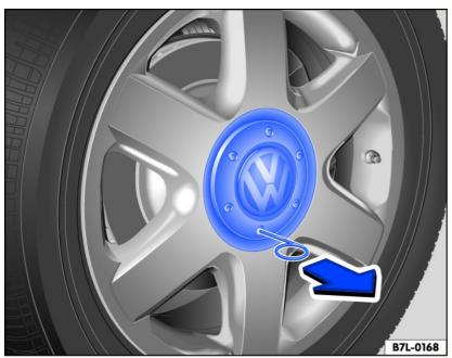
Fig. 170 Remove the wheel center trim.
