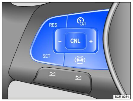
Fig. 109 Left side of the multifunction steering wheel: buttons for cruise control system operation.
