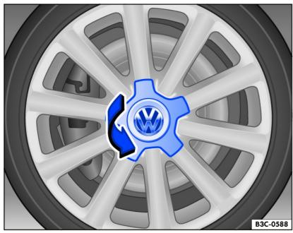
Fig. 171 Twist off the hubcap.
