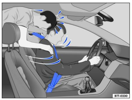
Fig. 26 A passenger in the rear seat who is not wearing a safety belt will be propelled forward toward the driver who has their own safety belt fastened.
