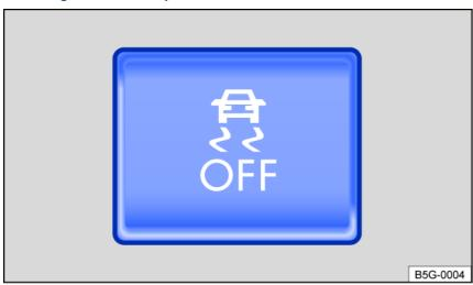
Fig. 120 Located on the center console: Button to manually switch ASR or ESC Sport on and off (depending on how your vehicle is equipped).
