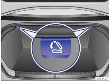
Fig. 90 In the luggage compartment: Release levers for the rear seat backrest.
