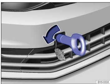
Fig. 206 In the right front bumper: Installing the towing eye.
