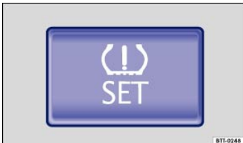
Fig. 102 In the glove compartment: SET button for the Tire Pressure Monitoring System.
