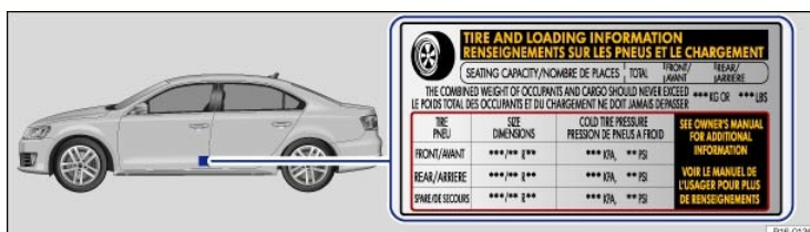
Fig. 98 On the driver door jamb: Location of the tire inflation pressure label.
