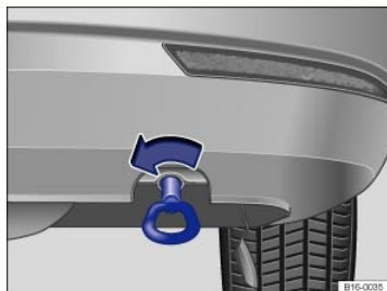
Fig. 208 In the right rear bumper: Installing the towing eye.
