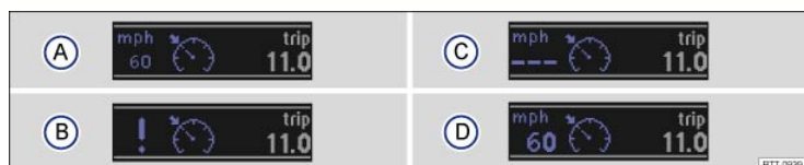
Fig. 133 In the instrument cluster display (depending on vehicle equipment): Cruise control status indications.
