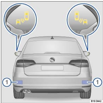
Fig. 155 In the outside mirrors: Indicator lights for the Blind Spot Monitor.
