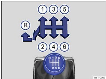
Fig. 124 Gearshift pattern of a 6-speed manual transmission.
