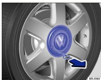
Fig. 191 Pulling the hubcap off.
