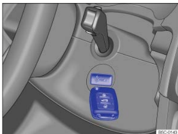
Fig. 120 Hold the remote control vehicle key to the right of the steering column: Emergency starting feature.
