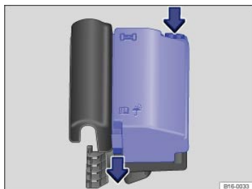
Fig. 200 In the engine compartment: Fuse box cover.
