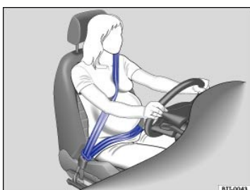
Fig. 58 Proper safety belt positioning for expectant mothers.
