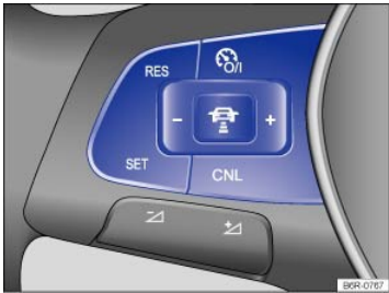
Fig. 139 Left-hand side of the multifunction steering wheel: Buttons for operating the Adaptive Cruise Control (ACC).
