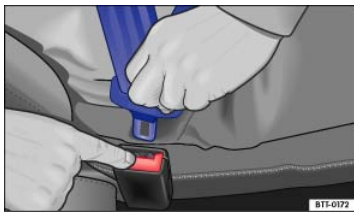
Fig. 56 Releasing the buckle tongue from the belt buckle.
