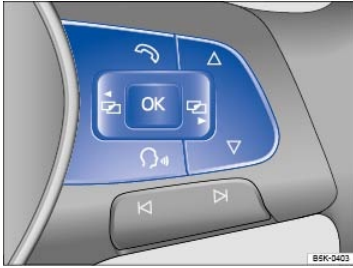
Fig. 14 Right side of the multi-function steering wheel: Controls for the menus and information in the instrument cluster display.
