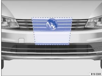
Fig. 145 Area around the radar sensor to be kept clean and free of obstructions.
