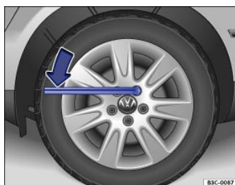
Fig. 195 Changing a wheel: Loosening the wheel bolts.
