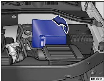
Fig. 175 In the engine compartment: Open the sleeve covering of the vehicle battery.
