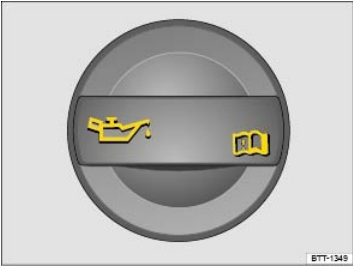
Fig. 170 In the engine compartment: Engine oil filler cap (cap design may vary depending on vehicle equipment).
