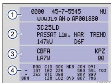
Fig. 19 Vehicle identification label: Shown in the example with engine identification code CBFA ③.
