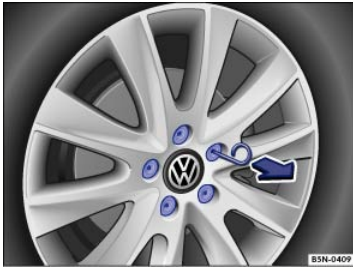
Fig. 193 Pulling cover caps off wheel bolts.
