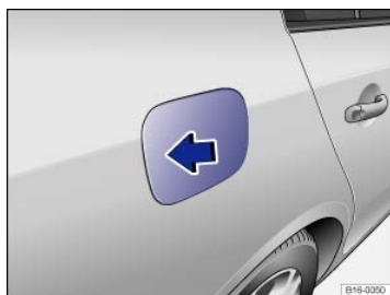
Fig. 165 Right rear side of vehicle: Opening the fuel filler flap.
