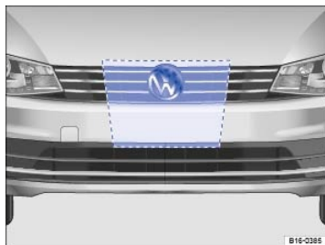
Fig. 138 Area around the radar sensor to be kept clean and free of obstructions.
