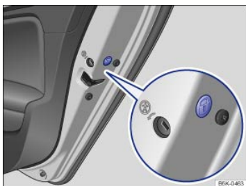
Fig. 181 On the front side of the passenger side rear door: Manual lock, covered by a rubber seal.
