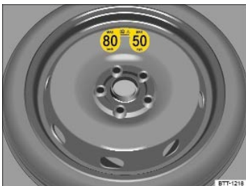
Fig. 100 In the luggage compartment: Compact spare wheel (label design may vary).
