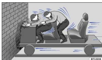
Fig. 51 A vehicle with passengers not wearing safety belts hits a wall.
