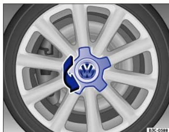
Fig. 192 Twisting the hubcap off.
