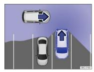
Fig. 161 Rear Traffic Alert: Monitored area around the vehicle that is backing out of a parking space.
