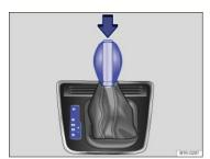
Fig. 128 Automatic transmission selector lever with shift lever release button (arrow).
