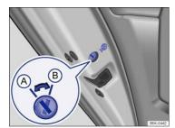
Fig. 28 In the driver side rear door: Child safety lock (A) deactivated, (B) activated.
