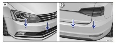
Fig. 152 In the front and rear bumpers: Park Distance Control system sensors.
