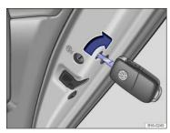
Fig. 185 On the front side of the passenger side rear door: Locking the vehicle with the key bit in the vehicle key.
