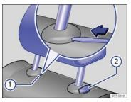
Fig. 45 Removing the rear head restraints.
