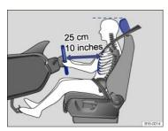
Fig. 38 The driver should never sit closer than 10 inches (25 cm) from the steering wheel.
