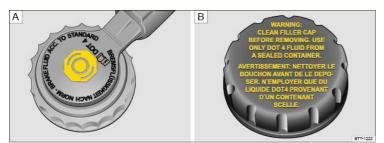
Fig. 133 In the engine compartment: Brake fluid reservoir cap (cap design may vary depending on vehicle equipment).
