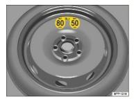
Fig. 103 In the luggage compartment: Compact spare wheel (label design may vary).
