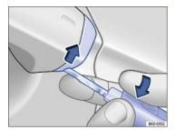
Fig. 183 Door handle on driver door: Removing the lock cylinder cover (if applicable).
