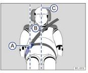
Fig. 64 Positioning of the safety belt extender.
