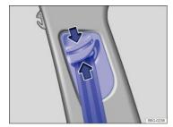
Fig. 62 Next to the front seats: Safety belt height adjuster.
