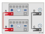
Fig. 207 Diagram for attaching the jumper cables: Dead battery 1 and booster battery 2.
