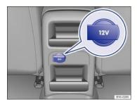
Fig. 120 In the rear center console (vehicles with a front center armrest): 12 Volt socket.
