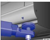
Fig. 180 Front lift point for workshop hoist or floor jack.
