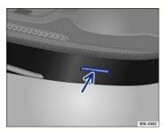
Fig. 20 Vehicle identification number (VIN).
