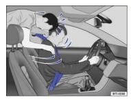
Fig. 56 Unbelted passengers in the rear seats are thrown forward on top of the belted driver.
