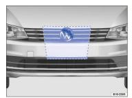
Fig. 148 Area around the radar sensor to be kept clean and free of obstructions.
