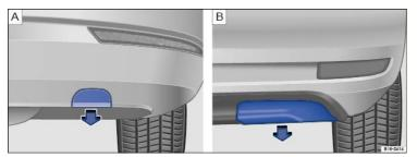
Fig. 210 In the right rear bumper: Removing the cover: Jetta models: Jetta GLI models.
