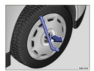
Fig. 197 Pulling the wheel cover off.
