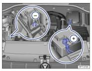
Fig. 206 In the engine compartment (1.8 liter engine): Positive jump-start terminal  $\oplus$  and negative jump-start terminal  $\ominus$ .
