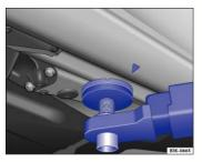
Fig. 181 Rear lift point for workshop hoist or floor jack.
