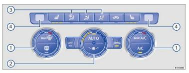
Fig. 164 In the center console: Climatronic controls.
