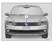
Fig. 140 Behind the Volkswagen emblem: Radar sensor.
