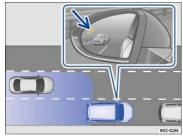
Fig. 159 Driving situation when passing with traffic behind your vehicle. Arrow: Blind Spot Monitor indicator light in the driver side mirror.
