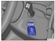
Fig. 123 Hold the remote control vehicle key to the right of the steering column: Emergency starting feature.
