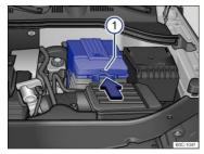
Fig. 177 In the engine compartment: Remove the hard cover from the vehicle battery.
