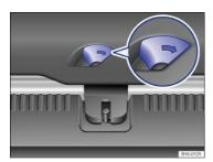
Fig. 187 Opening the trunk lid from inside the luggage compartment.
