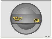
Fig. 173 In the engine compartment: Engine oil filler cap (cap design may vary depending on vehicle equipment).
