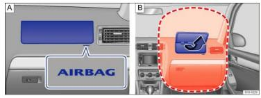
Fig. 67 Location and deployment zone of the front passenger front airbag.
