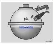
Fig. 175 Coolant expansion tank in the engine compartment.
