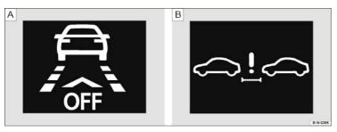
Fig. 145 In the instrument cluster display. : Front Assist switched off, : Distance warning.
