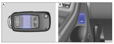
Fig. 30: On the remote control vehicle key: Button to unlock and open the trunk lid.: In the driver door: Switch to unlock and open the trunk lid.
