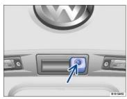
Fig. 149 In the trunk lid: Location of the camera.
