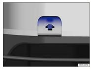
Fig. 208 In the right front bumper: Removing the cover.
