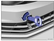
Fig. 209 In the right front bumper: Installing the towing eye.
