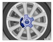
Fig. 195 Twisting the hubcap off.
