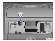
Fig. 189 Hexagonal head screw for closing the power sunroof.
