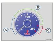
Fig. 174 Engine coolant temperature gauge in the instrument cluster: (A) Engine cold; (B) Normal temperature range; (C) Warning zone.
