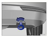
Fig. 211 In the right rear bumper: Installing the towing eye.
