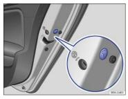
Fig. 184 On the front side of the passenger side rear door: Manual lock, covered by a rubber seal.
