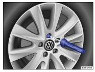
Fig. 201 Changing a wheel: Remove previously loosened wheel bolts using the screwdriver handle.
