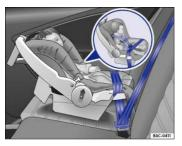
Fig. 73 Rearward-facing infant seat properly installed on the rear seat.
