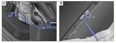
Fig. 171: In the engine compartment: Bracket for hood support.: Hood propped open.
