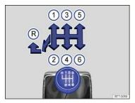
Fig. 127 Gearshift pattern of a 6-speed manual transmission.
