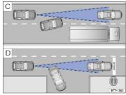
Fig. 144 Vehicle changing lanes. A turning and a stationary vehicle ahead.
