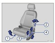
Fig. 41 Driver seat: Manual seat adjustment controls (version 2).
