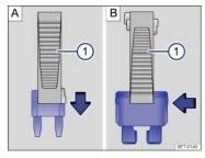
Fig. 205 Removing or installing a blade fuse with the plastic tweezers: : MINI. : ATO.
