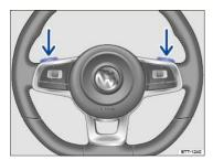
Fig. 130 Steering wheel with Tiptronic shift paddles (if equipped).
