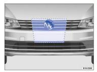
Fig. 141 Area around the radar sensor to be kept clean and free of obstructions.
