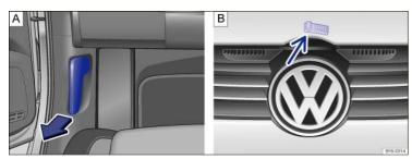
Fig. 170: In the footwell on the driver side: Inside engine hood release lever.: Above the radiator grille: Outside engine hood release.
