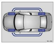
Fig. 100 Tire rotation diagram.
