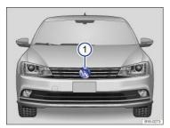
Fig. 147 Behind the Volkswagen emblem: Radar sensor.
