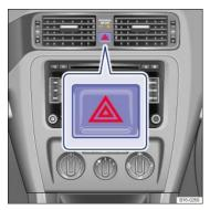
Fig. 182 In the center of the instrument panel: Button for the emergency flashers.
