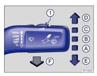
Fig. 85 Operating the front windshield wipers.
