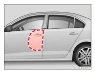
Fig. 68 Deployment zone of the side airbag.
