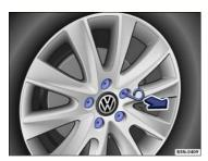
Fig. 196 Pulling cover caps off wheel bolts.
