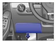
Fig. 202 On the driver side in the instrument panel: Fuse box cover.
