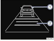
Fig. 138 In the instrument cluster display: ACC deactivated temporarily; vehicle detected ahead, time interval set.
