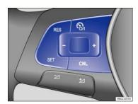
Fig. 137 On the left side of the multi-function steering wheel: Buttons for operating the cruise control.
