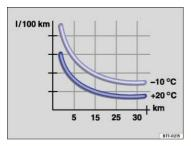
Fig. 135 Fuel consumption in I/100 km at 2 different outside air temperatures.
