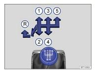
Fig. 126 Gearshift pattern of a 5-speed manual transmission.
