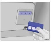
Fig. 36 In the driver side sun visor: The remote control and buttons for the HomeLink Universal Transmitter.
