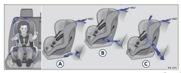
Fig. 74 Some child restraints have lower anchors and a top tether. Figures (a) and (b) show how to correctly install a LATCH/UCRA seat. Figure (c) shows the set up of a seat using the vehicle's safety belt system.
