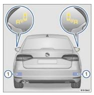
Fig. 158 In the outside mirrors: Indicator lights for the Blind Spot Monitor.
