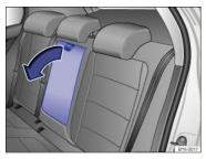
Fig. 49 Folding down the rear center armrest (arrow).
