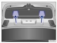
Fig. 32 Opened trunk lid: Recessed grips for closing.
