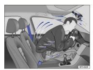
Fig. 55 The unbelted driver is thrown forward.
