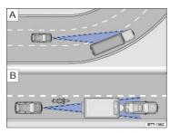
Fig. 143 Driving in a curve. Motorcycle traveling ahead outside of the sensor range.
