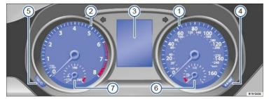
Fig. 11 Instrument cluster in the instrument panel (version 2).
