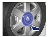
Fig. 194 Pulling the hubcap off.
