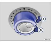
Fig. 35 In the headliner: Rotary switch for the power sunroof: Press or pull the switch to tilt open or to close
