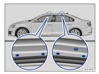
Fig. 97 Attachment points for the base carrier and roof rack.
