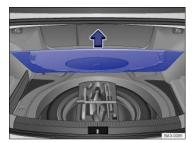
Fig. 192 In the luggage compartment under the floor panel: Compact spare wheel and vehicle tool kit.
