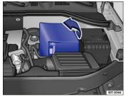
Fig. 178 In the engine compartment: Open the sleeve covering of the vehicle battery.
