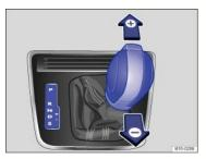
Fig. 129 Selector lever in Tiptronic position.
