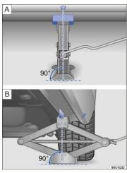
Fig. 200 Jack in position at the left rear lift point.
