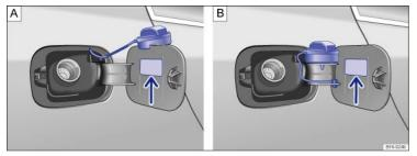
Fig. 169 Fuel cap placed on the open fuel filler flap: Versions and .
