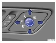
Fig. 92 In the driver door: Adjusting knob for the outside mirrors.
