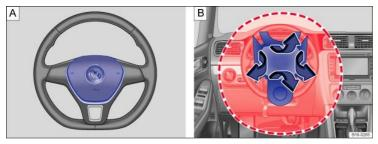
Fig. 66 Location and deployment zone of the driver front airbag.
