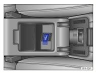
Fig. 112 Inside the front center armrest storage compartment: MDI (MEDIA-IN) jack (if equipped).
