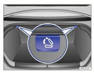
Fig. 93 In the luggage compartment: Release levers for the rear seat backrest.
