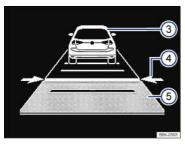
Fig. 139 In the instrument cluster display: ACC active, vehicle detected ahead, time interval is being set.
