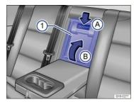
Fig. 95 In the rear seat backrest: Opening the luggage compartment pass-through (if equipped).
