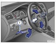
Fig. 46 Manual adjustment for the steering wheel position.
