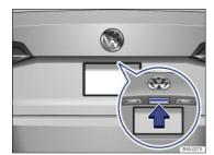
Fig. 31 Opening the trunk lid from the outside.
