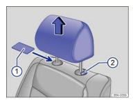
Fig. 44 Removing the front head restraints.
