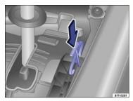
Fig. 191 Releasing the selector lever lock.
