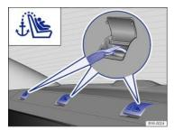
Fig. 77 Behind the rear seat backrest: Top tether anchorages.
