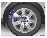
Fig. 198 Changing a wheel: Loosening the wheel bolts.
