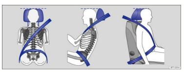
Fig. 60 Proper safety belt positioning and head restraint adjustment.
