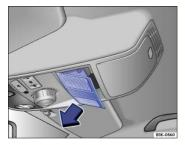
Fig. 188 In headliner: Removing cover
