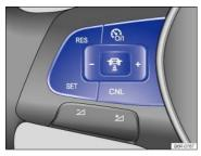
Fig. 142 Left-hand side of the multifunction steering wheel: Buttons for operating the Adaptive Cruise Control (ACC).
