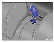
Fig. 186 Behind the rear seat backrest: Release of the rear seat back.
