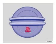
Fig. 176 Coolant expansion tank cap in the engine compartment.
