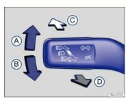
Fig. 79 On the left side of the steering column: Turn signal lever and high beam switch (version 2).
