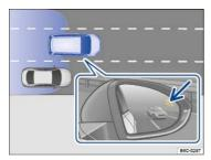
Fig. 160 Driving situation when passing and merging into the lane. Arrow: Blind Spot Monitor indicator light in the passenger side mirror.
