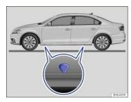
Fig. 199 Lift points for the jack.
