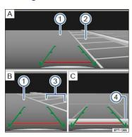
Fig. 151 On the screen: Orientation lines for the parking space behind the vehicle.: Searching for a parking space,: Backing into the parking space,: Maneuvering.
