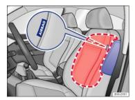
Fig. 69 In the padding on the outboard side of the front seat backrests: Location and deployment zone of the side airbags.
