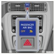
Fig. 65 In the instrument panel: PASSENGER AIR BAG light.
