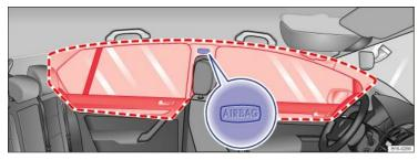
Fig. 70 On the left vehicle side: Installation location and deployment zone of the Side Curtain Protection airbag.
