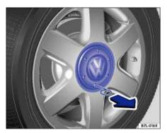
Fig. 186 Pulling the hubcap off.
