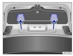
Fig. 33 Opened luggage compartment lid: Recessed grips for closing.
