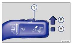
Fig. 86 Windshield wiper lever: Adjusting the rain sensor 1 (if equipped).
