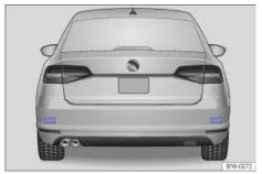
Fig. 143 Rear of the vehicle: Radar sensor areas.
