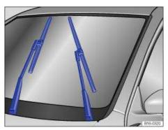
Fig. 85 Windshield wiper in service position
