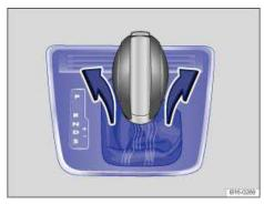
Fig. 182 Removing the selector gate cover.
