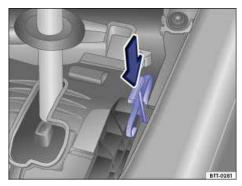
Fig. 183 Releasing the selector lever lock.
