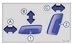
**Fig. 43** Driver seat: Electrical controls to move the seat backward or forward, and adjust seat cushion height and backrest angle (if equipped).
