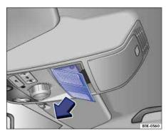
Fig. 180 In headliner: Removing cover.
