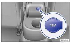
Fig. 121 In the rear center console (vehicles without a front center armrest): 12 Volt socket.
