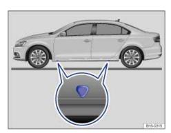
Fig. 191 Lift points for the jack.
