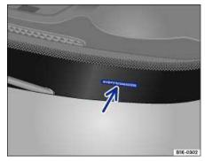
Fig. 20 Vehicle identification number (VIN).
