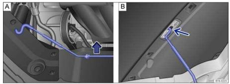
Fig. 163 A: In the engine compartment: Bracket for hood support. B: Hood propped open.
