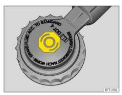
Fig. 134 In the engine compartment: Brake fluid reservoir cap.
