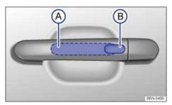
Fig. 28 Keyless Access system: Sensor for unlocking A on the inside of the front door handles. Sensor for locking B on the outside of the front door handles.
