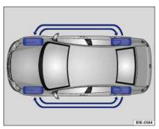
Fig. 100 Tire rotation diagram.
