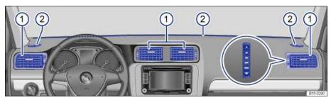
Fig. 154 In the instrument panel: Air vents.
