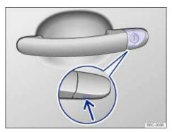
Fig. 175 Door handle on driver door: Concealed lock cylinder (if applicable).
