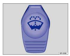
Fig. 88 In the engine compartment: Cap of the windshield washer fluid reservoir.
