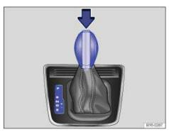
Fig. 131 Automatic transmission selector lever with shift lever release button (arrow).
