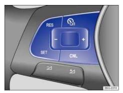
Fig. 138 Left-hand side of the multi-function steering wheel: Buttons for operating the cruise control .
