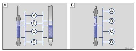
Fig. 164 Engine oil dipstick with oil level marks. A: For vehicles with gasoline engines. B: For vehicles with diesel engines.
