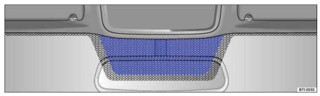
Fig. 83 Heat-reflective windshield with communications window (blue shaded area).
