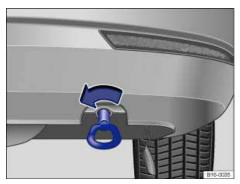
Fig. 203 In the rear right bumper: Installing the towing eye.
