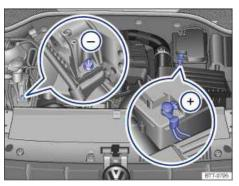
Fig. 198 In the engine compartment (1.8 liter engine): Positive jump-start terminal + and negative jump-start
