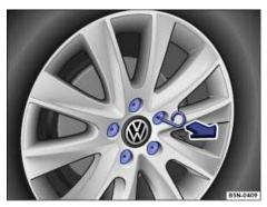
Fig. 188 Pulling cover caps off wheel bolts.
