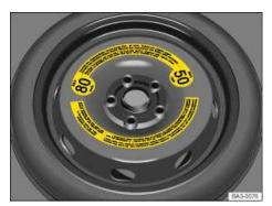
Fig. 103 In the luggage compartment: Compact spare wheel.
