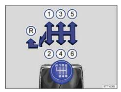
Fig. 130 Gearshift pattern of a 6-speed manual transmission.
