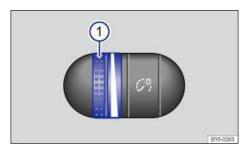
Fig. 81 To the left of the steering wheel: Thumbwheel to adjust instrument panel lighting 1.
