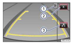
Fig. 140 Rear View Camera system display (may vary depending on vehicle equipment).
