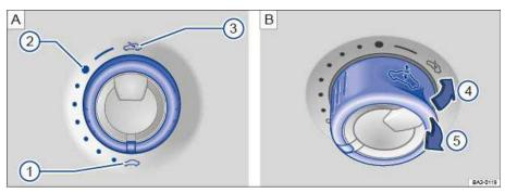
Fig. 35 In the headliner: Rotary switch for the power sunroof.
