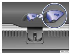
Fig. 179 Opening the luggage compartment lid from inside the luggage compartment.
