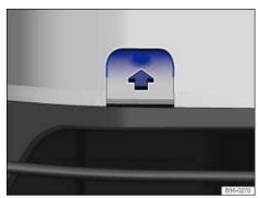
Fig. 200 In the right front bumper: Removing the cover.
