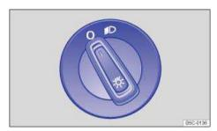
Fig. 79 Headlight switch next to the steering wheel.
