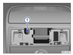
Fig. 181 Hexagonal head screw for closing the power sunroof.
