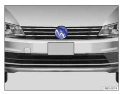
Fig. 150 Area around the radar sensor to be kept clean and free of obstructions.
