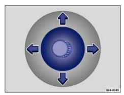
Fig. 91 In the front doors: Rotary knob for the mechanically adjustable outside mirrors.
