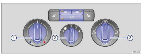
Fig. 151 In the center console: Manual air conditioning controls.
