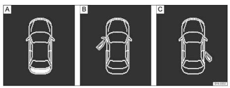
Fig. 13 In the instrument cluster display (depending on vehicle equipment): A: Open luggage compartment lid, B: Open front driver side door, C: Open rear passenger side door.
