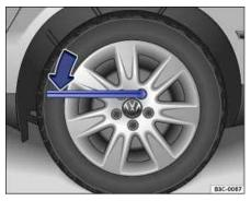
Fig. 190 Changing a wheel: Loosening the wheel bolts.
