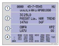
Fig. 19 Vehicle identification label: Shown in the example with engine identification code CBFA 3.
