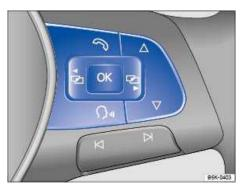
Fig. 16 Right side of the multi-function steering wheel (if equipped): Controls for the menus in the instrument
