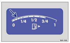
Fig. 155 In the instrument cluster display: Fuel gauge (version 1).
