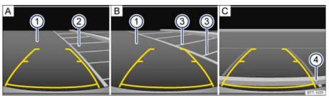
Fig. 141 On the screen: Static orientation lines for the parking space behind the vehicle.
