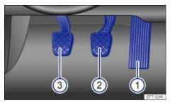
Fig. 127 Pedals in vehicles with manual transmission: 1 Accelerator pedal, 2 Brake pedal, 3 Clutch pedal.
