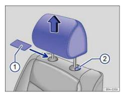
Fig. 45 Removing the front head restraints.
