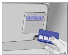
Fig. 37 In the driver side sun visor: The remote control and buttons for the HomeLink Universal Transmitter.
