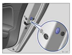
Fig. 176 On the front side of the right rear door: Manual lock, covered by a rubber seal.
