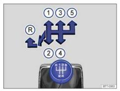
Fig. 129 Gearshift pattern of a 5-speed manual transmission.
