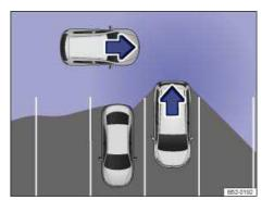
Fig. 146 Rear Traffic Alert: Monitored area around the vehicle that is backing out of a parking space.
