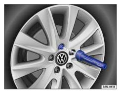
Fig. 193 Changing a wheel: Remove previously loosened wheel bolts using the screwdriver handle.
