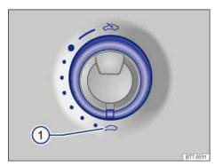
Fig. 36 In the headliner: Sunroof rotary switch.
