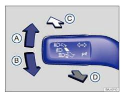
Fig. 78 On the left side of the steering column: Turn signal lever and high beam switch.
