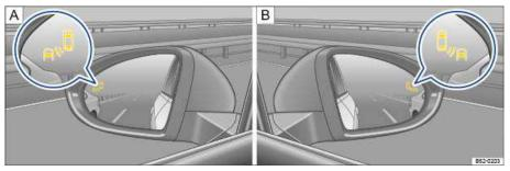
Fig. 142 In the outside mirrors: Indicator lights for the Blind Spot Monitor.
