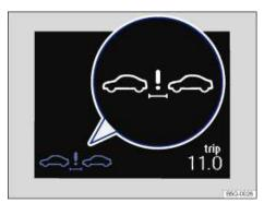
Fig. 147 In the instrument cluster display: Distance warning.
