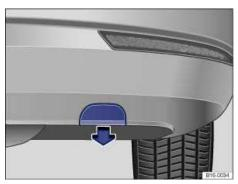
Fig. 202 In the right rear bumper: Removing the cover.
