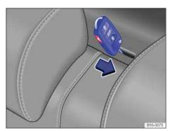
Fig. 178 Behind the rear seat backrest: Release of the rear seat back.
