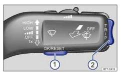
Fig. 15 On the right side of the steering column (vehicles without a multi-function steering wheel): Windshield wiper lever with controls for instrument cluster menus and displays.
