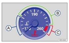
**Fig. 166** Engine coolant temperature gauge in the instrument cluster: A Engine cold; B Normal temperature range; C Warning zone.
