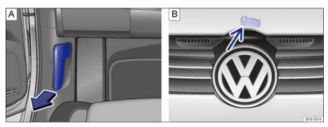
Fig. 162 A: In the footwell on the driver side: Inside engine hood release lever. B: Above the radiator grille: Outside engine hood release.
