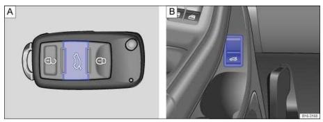
Fig. 31 A: In the remote control vehicle key: Button to unlock and open the luggage compartment lid. B: In the driver door: Switch to unlock and open the luggage compartment lid.
