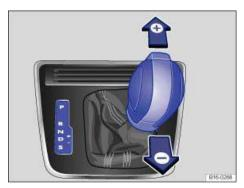
Fig. 132 Selector lever in Tiptronic position.
