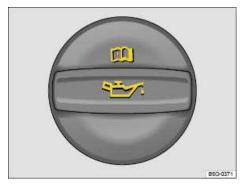
Fig. 165 In the engine compartment: Engine oil filler cap.
