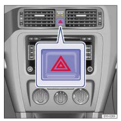
Fig. 174 In the center of the instrument panel: Button for the emergency flashers.
