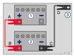
Fig. 199 Diagram for attaching the jumper cables: Dead battery 1 and booster battery 2.
