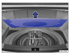
Fig. 184 In the luggage compartment under the floor panel: Compact spare wheel and vehicle tool kit.
