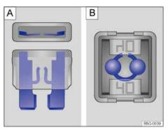
Fig. 196 Blown fuse: A: Blade fuse. B: Cartridge fuse.
