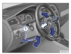
Fig. 47 Manual adjustment for the steering wheel position.
