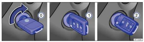
Fig. 123 In the ignition switch: Vehicle key positions.
