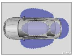
Fig. 27 Ranges of the Keyless Access system. Outside the vehicle: Unlocking range. Inside the vehicle:
