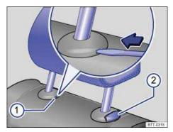
Fig. 46 Removing the rear head restraints.
