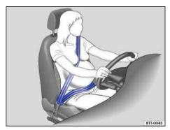
Fig. 61 Proper safety belt positioning for expectant mothers.
