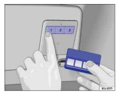
Fig. 38 To program: Simultaneously press the buttons for the HomeLink Universal Transmitter and the remote
