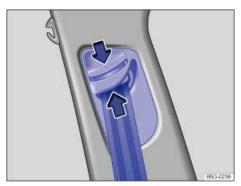
Fig. 62 Next to the front seats: Safety belt height adjuster.
