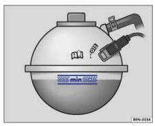
Fig. 167 Coolant expansion tank in the engine compartment.
