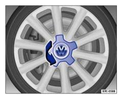
Fig. 187 Twisting the hubcap off.
