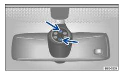
Fig. 87 Inside the front windshield above the inside mirror: Sensitive rain sensor surface.
