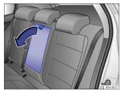
Fig. 49 Folding down the rear center armrest (arrow).
