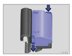
Fig. 195 In the engine compartment: Fuse box cover.
