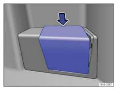
Fig. 160 At the right rear of the luggage compartment: AdBlue tank underneath a cover.
