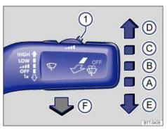
Fig. 84 Operating the front windshield wipers.
