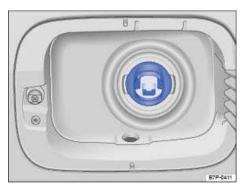
Fig. 159 With open fuel cap: Misfueling guard in the fuel filler neck.
