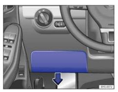
Fig. 194 On the driver side in the instrument panel: Fuse box cover.
