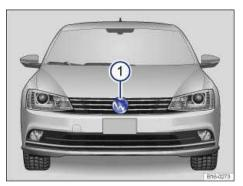
Fig. 149 Behind the Volkswagen emblem: Radar sensor.
