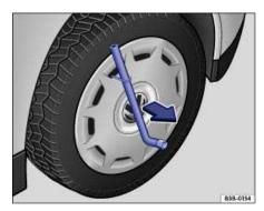
Fig. 189 Pulling the wheel cover off.
