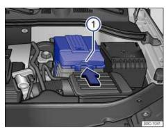
Fig. 169 In the engine compartment: Remove the hard cover from the vehicle battery.
