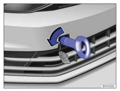
Fig. 201 In the right front bumper: Installing the towing eye.
