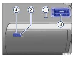
Fig. 9 Overview of the front passenger side.
