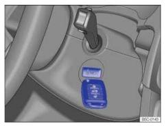
Fig. 125 Hold the remote control vehicle key to the right of the steering column: Emergency starting feature.
