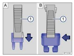
Fig. 197 Removing or installing a blade fuse with the plastic tweezers: A: MINI. B: ATO.
