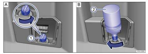
Fig. 161 AdBlue tank with filler neck cap 1 and refill bottle 2.
