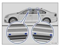
Fig. 97 Attachment points for the base carrier and roof rack.
