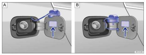
Fig. 158 Fuel cap placed on the open fuel filler flap: Versions A and B.
