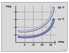
Fig. 135 Fuel consumption in miles per gallon (mpg) at 2 different outside air temperatures.
