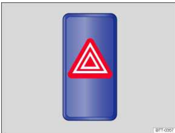
Fig. 147 In the center of the instrument panel: Switch for emergency flashers.
