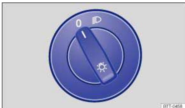
Fig. 71 Headlight switch next to the steering wheel.
