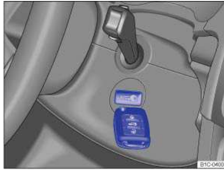
Fig. 105 Emergency starting feature on vehicles with Keyless Access.
