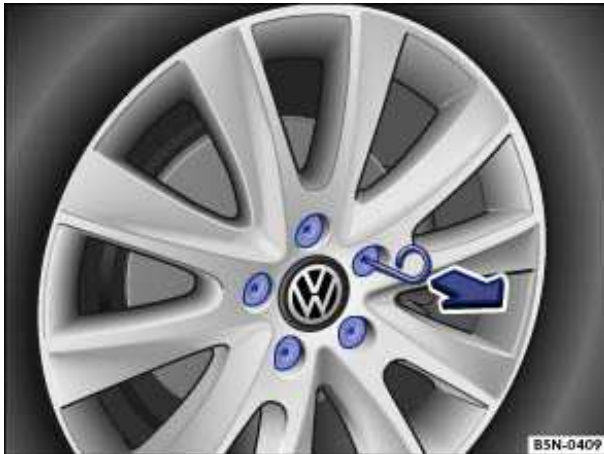
Fig. 162 Pulling cover caps off wheel bolts.
