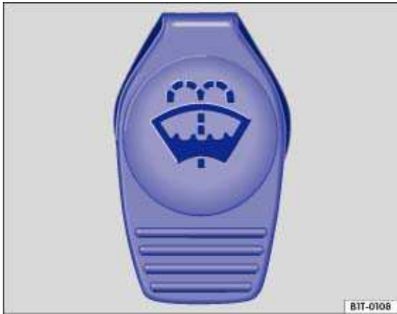
Fig. 78 In the engine compartment: Cap of the windshield washer fluid reservoir.
