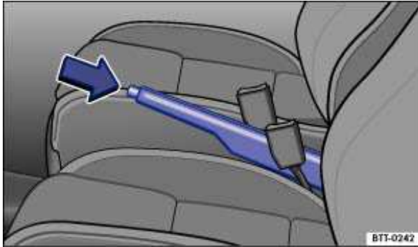
Fig. 114 Between the front seats: Parking brake.
