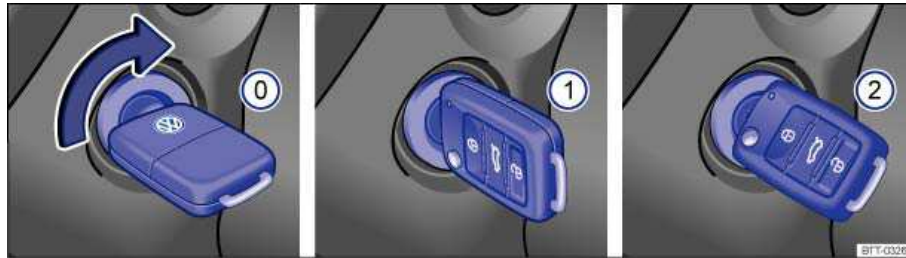
Fig. 103 In the ignition switch: Vehicle key positions.
