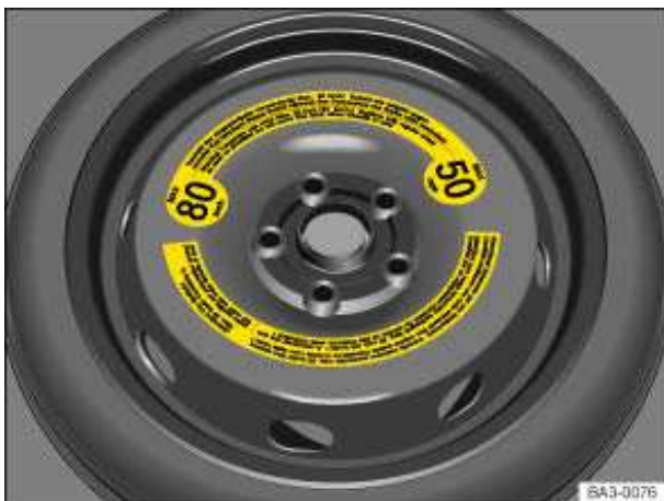
Fig. 143 In the luggage compartment: Compact spare wheel.
