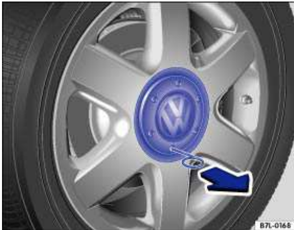
Fig. 159 Pulling the hubcap off.
