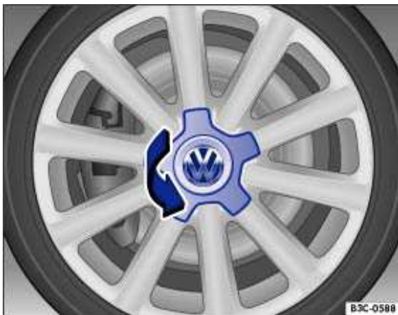
Fig. 160 Twisting the hubcap off.
