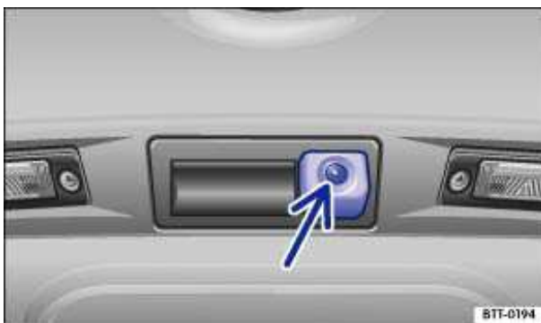
Fig. 118 In the luggage compartment lid: Location of the Rear Assist camera.
