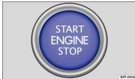
Fig. 104 In the center console: Starter button of the Keyless Access locking and starting system.
