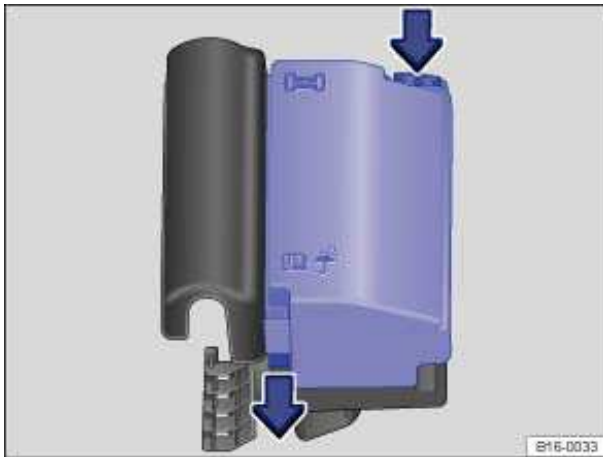
Fig. 169 In the engine compartment: Fuse box cover.
