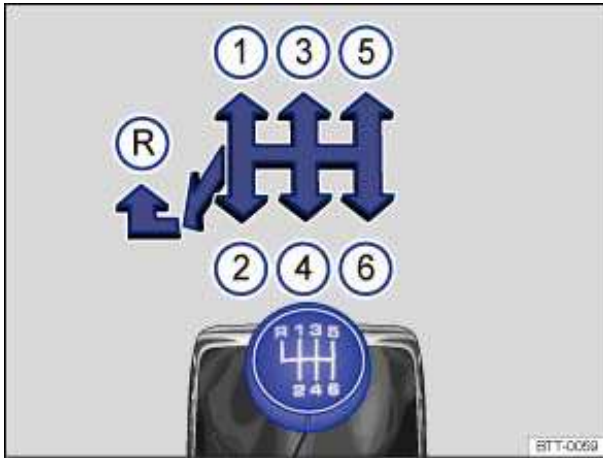
Fig. 110 Gearshift pattern of a 6-speed manual transmission.
