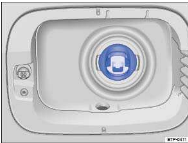
Fig. 129 With open fuel cap: Misfueling guard in the fuel filler neck.
