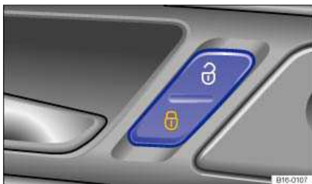
Fig. 21 In the driver and front passenger doors: Power locking button.
