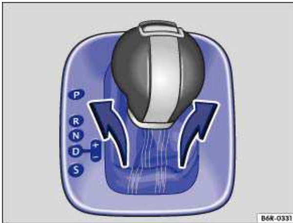
Fig. 155 Removing the selector gate cover.
