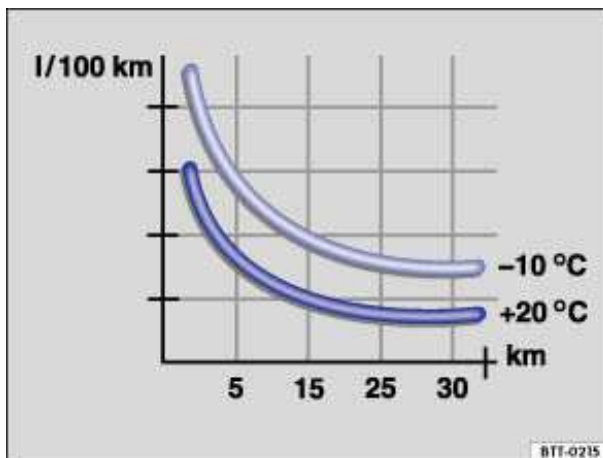
Fig. 117 Fuel consumption in l/100 km at 2 different outside air temperatures.
