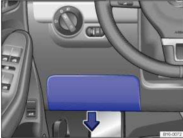
Fig. 168 On the driver side in the instrument panel: Fuse box cover.
