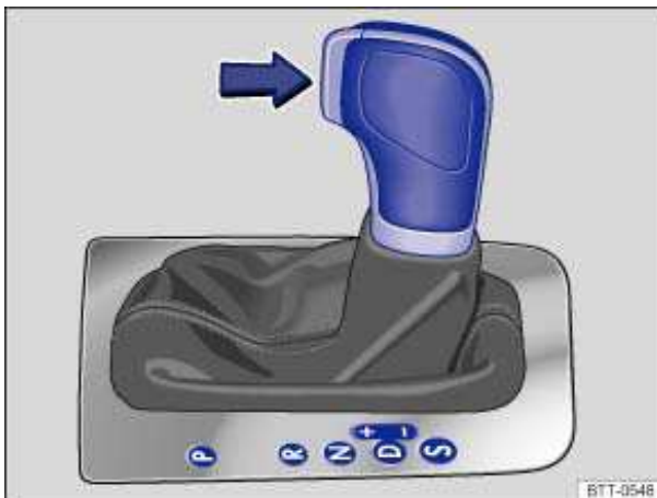
Fig. 111 Side view: Automatic transmission selector lever with shift lever release button (arrow).
