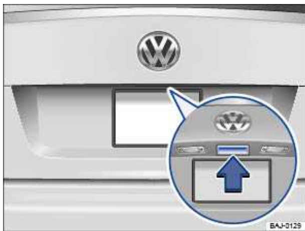
Fig. 28 Opening luggage compartment lid from the outside.
