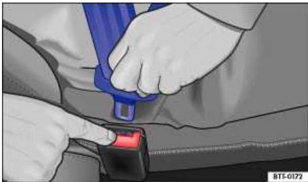
Fig. 51 Releasing the buckle tongue from the belt buckle.
