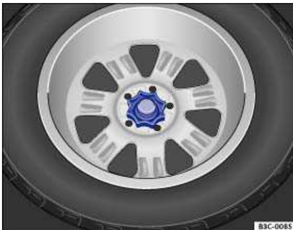
Fig. 142 In the luggage compartment: Handwheel holding the spare wheel in place.
