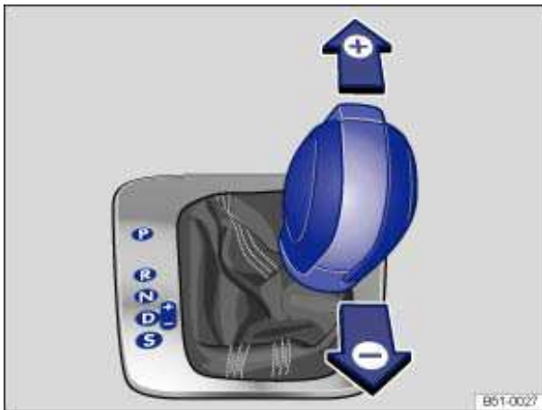
Fig. 113 Selector lever in Tiptronic position.
