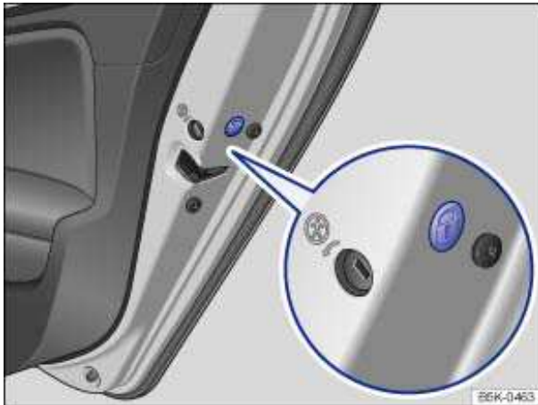
Fig. 149 On the front side of the right rear door: Emergency lock, covered by a rubber seal.
