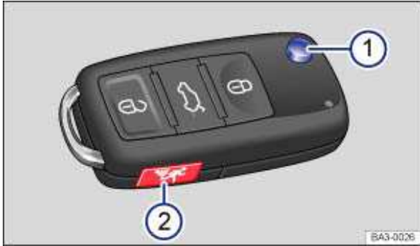
Fig. 16 Remote control vehicle key with panic button.
