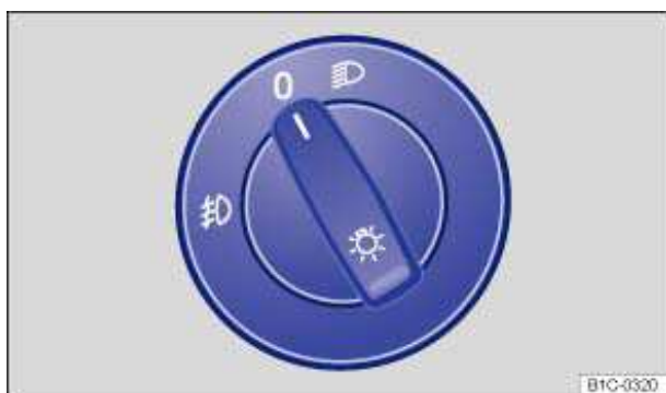
Fig. 72 Headlight switch next to the steering wheel (with fog lights).
