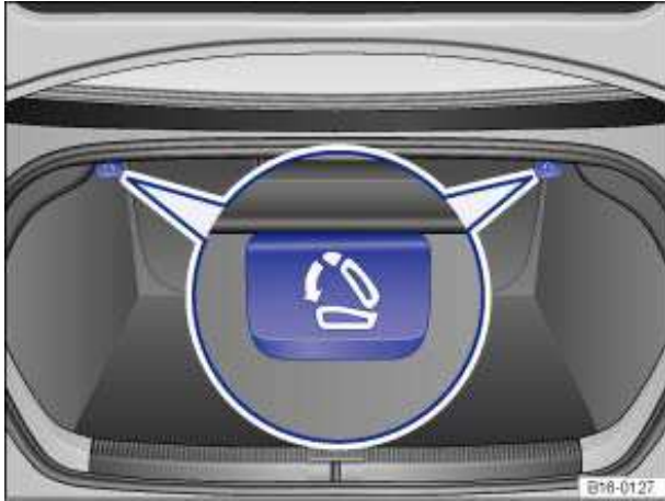
Fig. 82 On the left side of the luggage compartment: Release lever for the left-side rear seat backrest. The release lever for the right-side rear seat backrest is on the right side of the luggage compartment.
