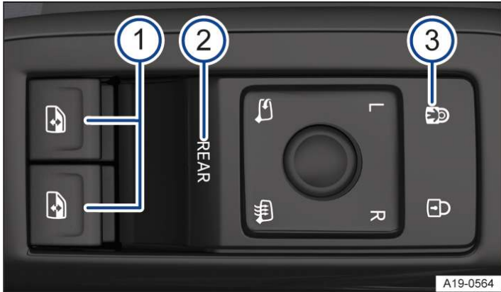
Fig. 1 In the driver door: buttons for the front and rear electric windows (illustration).
