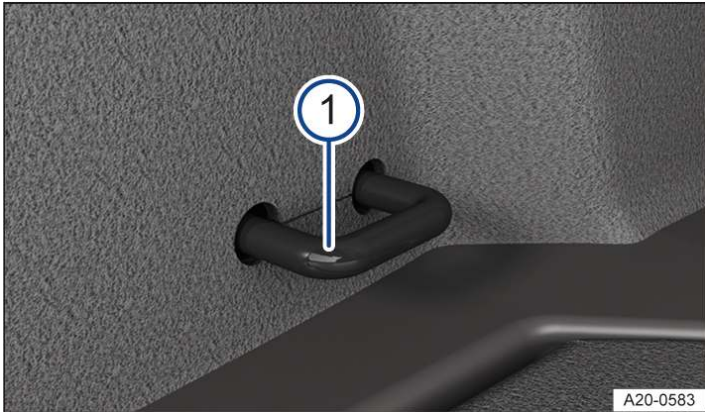
Fig. 1 In the luggage compartment: fastening ring (illustration).
