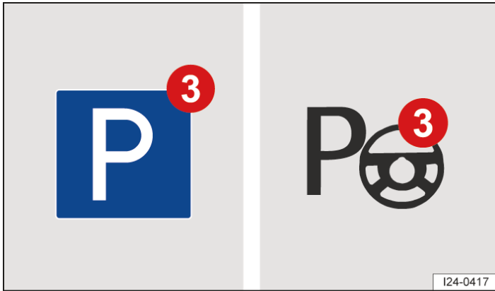
Fig. 2 Infotainment system: parking spaces detected (red number).
