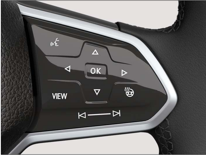
Fig. 1 Right side of the multifunction steering wheel: selecting displays (illustration)
