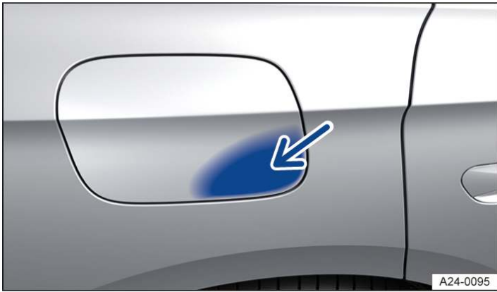
Fig. 1 At the rear right of the vehicle: opening the charging socket flap.
