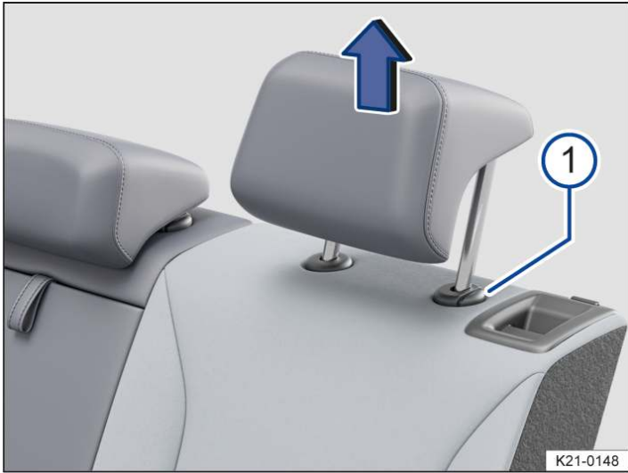
Fig. 2 Removing a rear head restraint (illustration).
