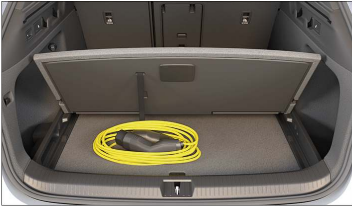
Fig. 1 Under the upper luggage compartment floor in the upper position: stowage space for the charging cable (illustration).
