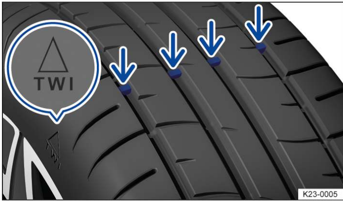
Fig. 1 In the tread grooves: tread wear indicator.
