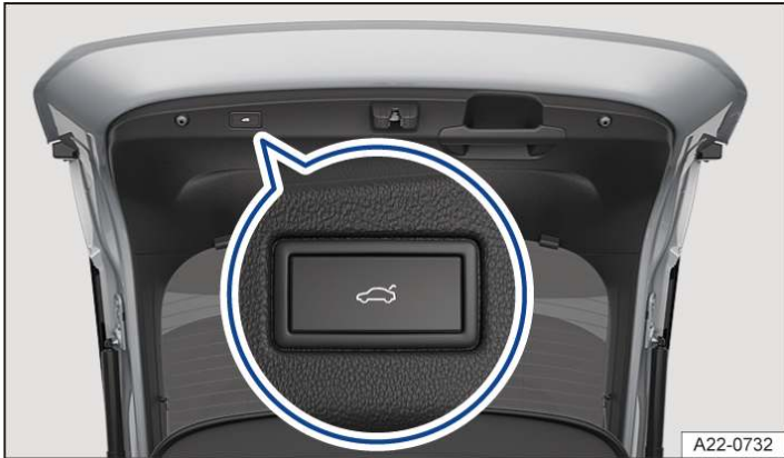
Fig. 1 In the open boot lid: button for electrically closing the boot lid (illustration).
