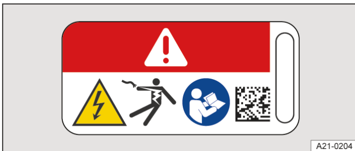
Fig. 1 Warning sign on high-voltage components.
