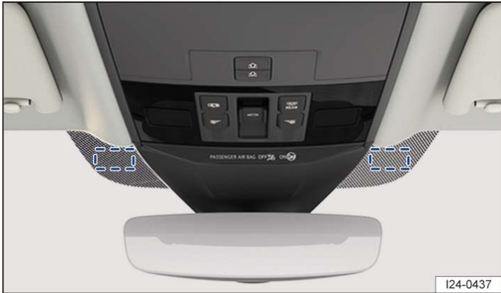
Fig. 1 Next to the mirror base: communication window (illustration).
