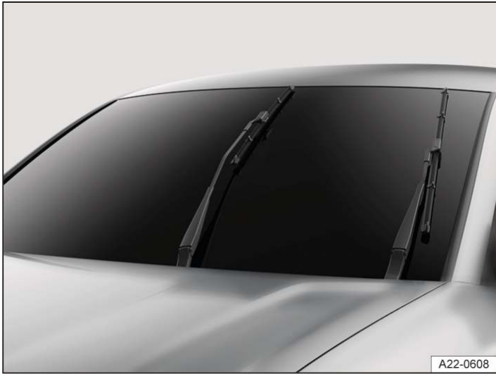
Fig. 1 Wipers in service position (illustration).
