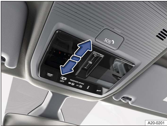
Fig. 1 In the roof: function button for controlling the panoramic sunroof with smart glass.
