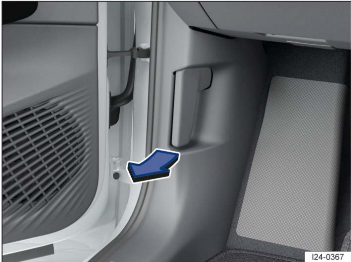
Fig. 1 In the footwell on the driver side: bonnet release lever (illustration).
