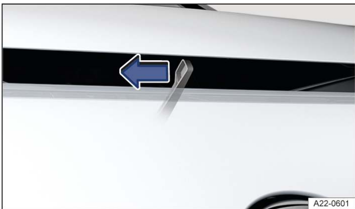
Fig. 2 On the bonnet: control lever. (illustration)
