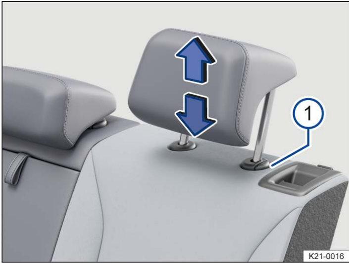
Fig. 2 Adjusting a rear head restraint (illustration).
