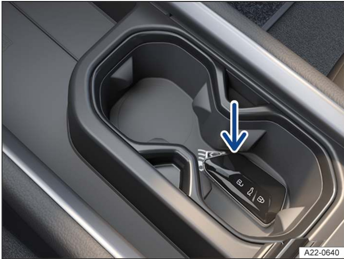
Fig. 1 In the centre console: emergency start function.
