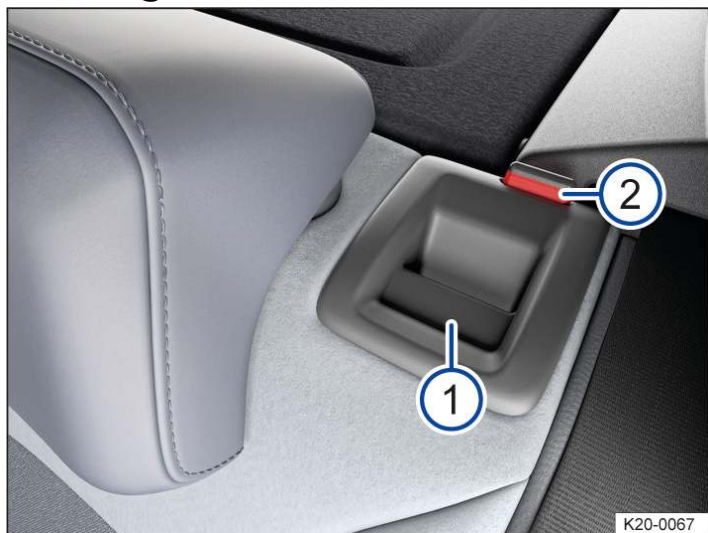
Fig. 1 In the rear seat backrest: release button.
