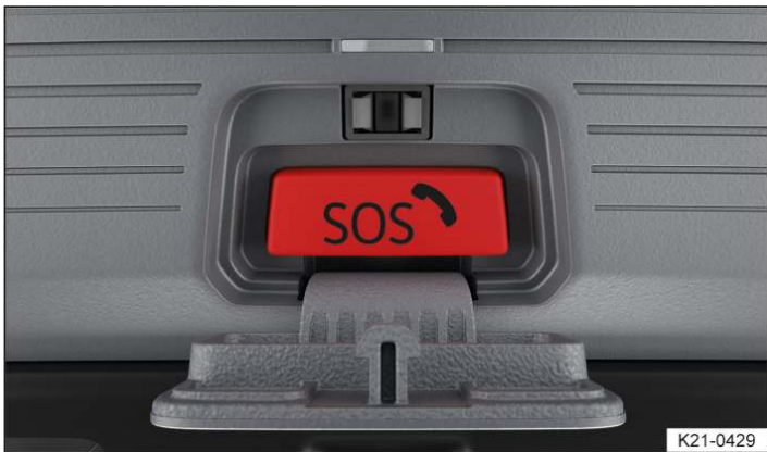
Fig. 2 In the roof console: button for the legally required eCall Emergency System.
