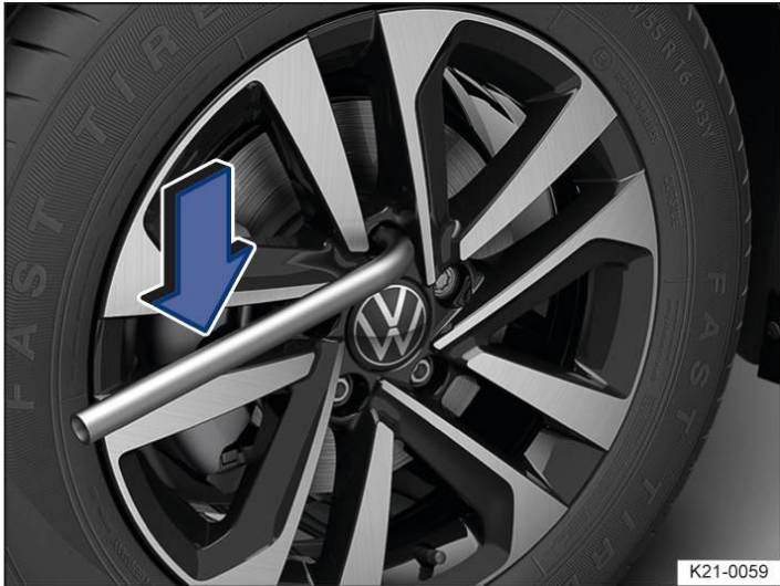
Fig. 1 Loosening wheel bolts.
