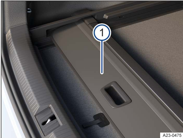
Fig. 1 Under the luggage compartment floor: stowing the luggage compartment cover.
