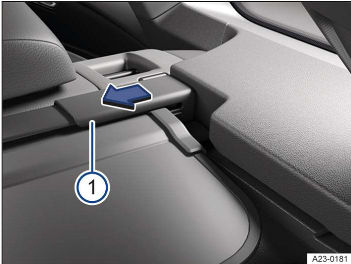
Fig. 1 In the luggage compartment: removing the luggage compartment cover.
