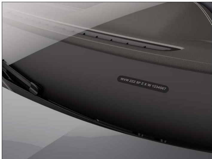
Fig. 1 In the windscreen: vehicle identification number.
