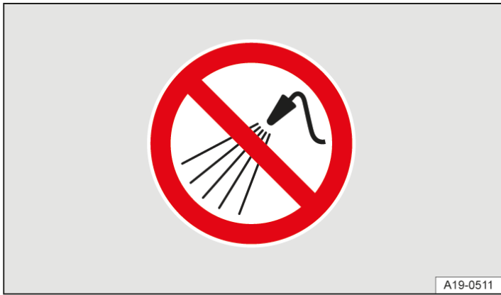
Fig. 1 In the bonnet space: do not use a high-pressure cleaner.
