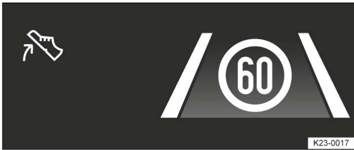
Fig. 1 In the head-up display: Eco Assistance display (illustration).
