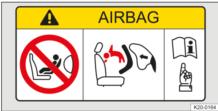
Fig. 1 On the sun visor: airbag label(illustration).
