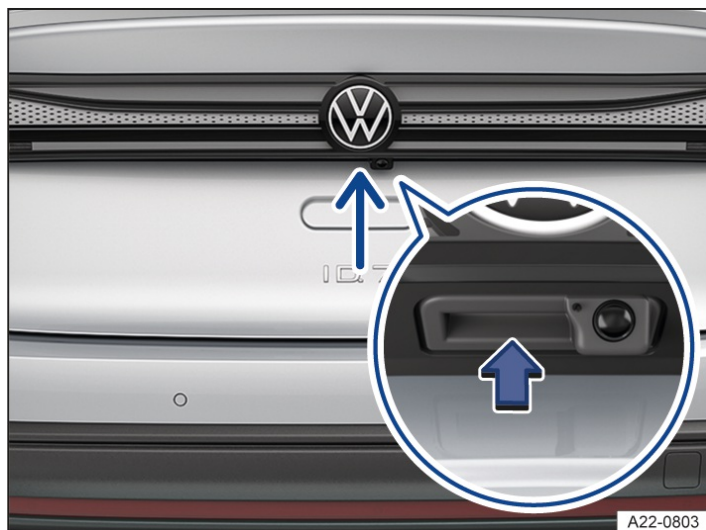
Fig. 1 In the boot lid: button for opening the boot lid.
