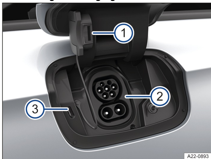
Fig. 1 Behind the charging socket flap at the rear right: charging socket.
