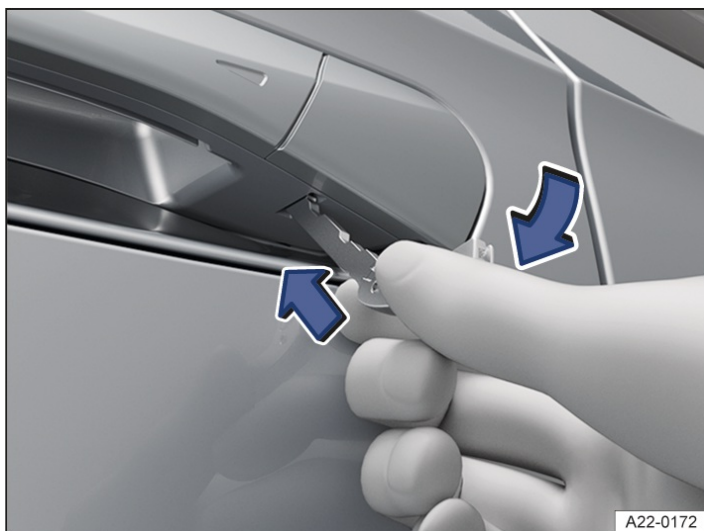
Fig. 1 Handle on the driver door: levering off the cover.
