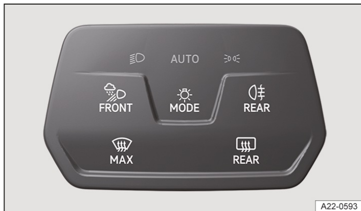
Fig. 1 Next to the steering wheel: touch panel for switching on the exterior lighting.
