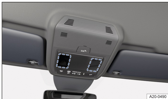
Fig. 1 In the roof console: touch-sensitive reading lights.
