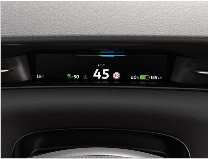
Fig. 1 In the dash panel: digital instrument cluster (illustration).
