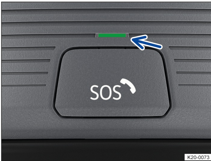
Fig. 1 In the roof console: button for Emergency Call Service (behind button cover) and indicator lamp.
