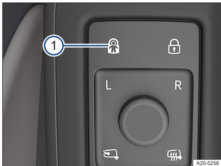
Fig. 1 In the driver door: touch panel for electric childproof lock.
