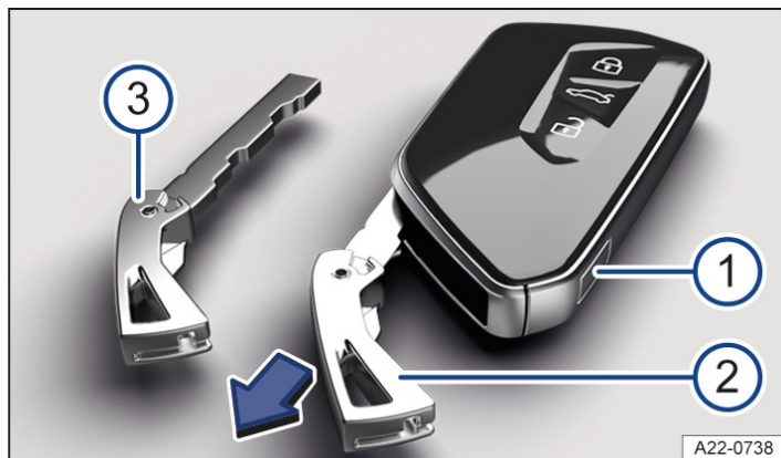
Fig. 1 Vehicle key: releasing the manual key.
