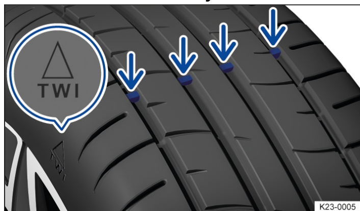
Fig. 1 In the tread grooves: tread wear indicator.
