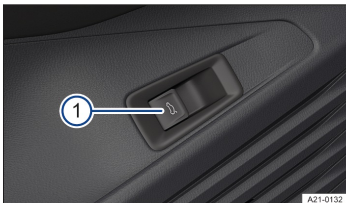
Fig. 1 In the driver door: release button for the boot lid.
