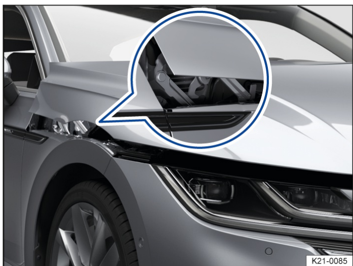
Fig. 1 Triggered re-active bonnet (illustration).
