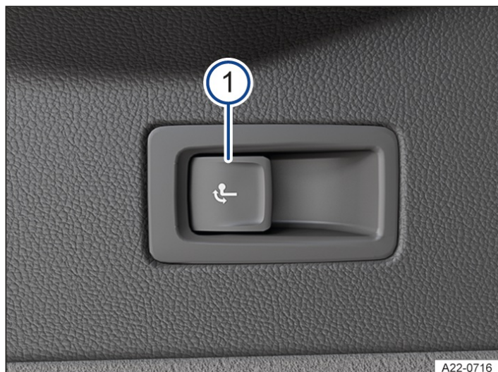
Fig. 1 On the left of the luggage compartment: button for releasing the ball coupling.
