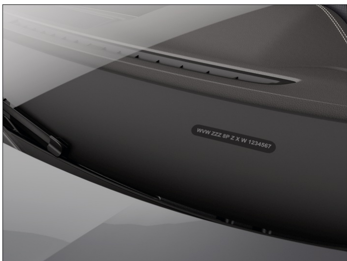
Fig. 1 In the windscreen: vehicle identification number.
