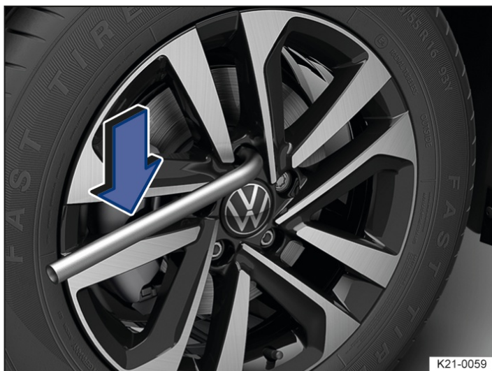
Fig. 1 Loosening wheel bolts.
