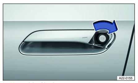
Fig. 47 Emergency locking of driver door.
