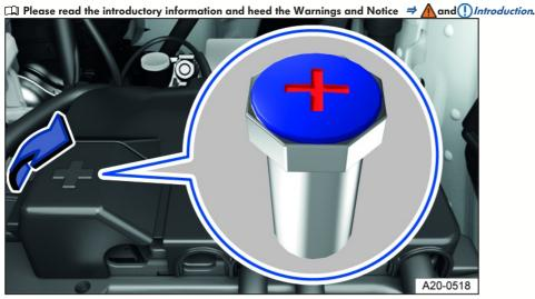
Fig. 153 Under a cover in the hood space: Positive jump-start point.
