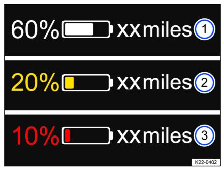
Fig. 11 In the digital instrument cluster: Range and reserve display.
