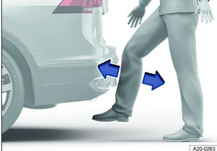
Fig. 54 General example of the sensor-controlled luggage compartment opener (Easy Open).
