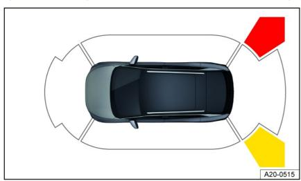
Fig. 109 Infotainment system: Rear Traffic Alert display.
