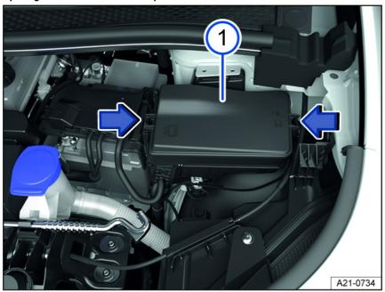
Fig. 145 In the hood space: fuse box.
