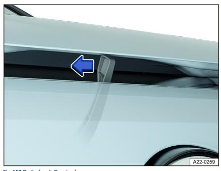
Fig. 157 On the hood: Opening lever.
