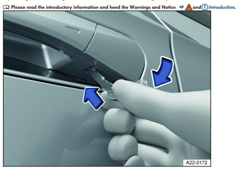
Fig. 46 Driver's door handle: prying off the cap.
