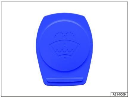
Fig. 160 In the hood space: Cap on the washer fluid reservoir (general example).
