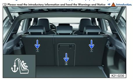
Fig. 31 On the rear side of the rear bench seat: Top tether anchorages for the top tether safety belt.
