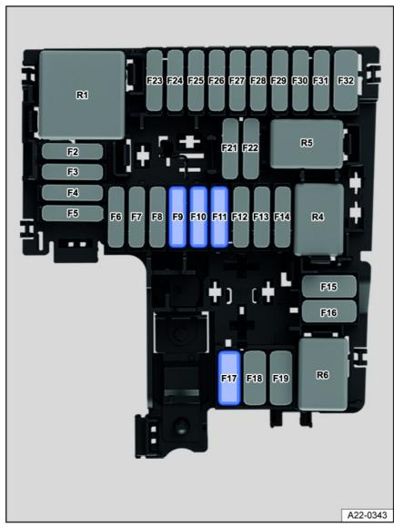
Fig. 146 In the hood space: Fuse locations.
