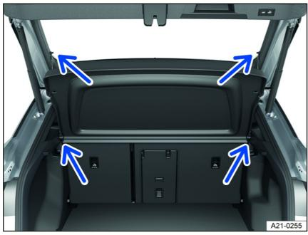
Fig. 115 In the luggage compartment: Installing and removing the luggage compartment cover.
