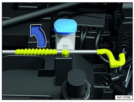
Fig. 158 In the hood space: Hood support in the bracket.
