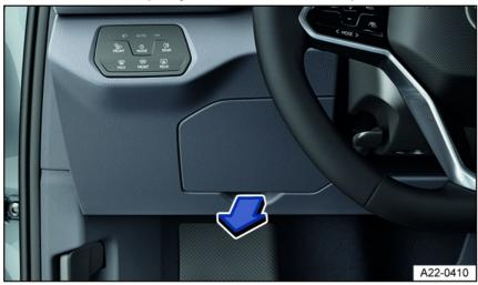
Fig. 147 Fuse box cover on the instrument panel on the driver's side (left-hand drive vehicles).
