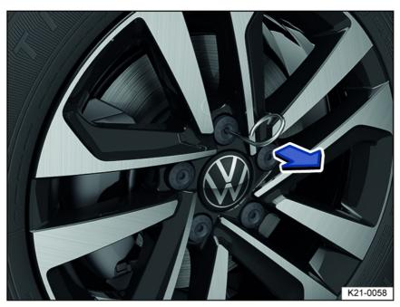
Fig. 169 Remove the caps from the wheel bolts.
