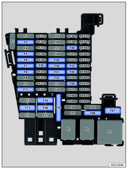
Fig. 149 Fuse assignment in the instrument panel.
