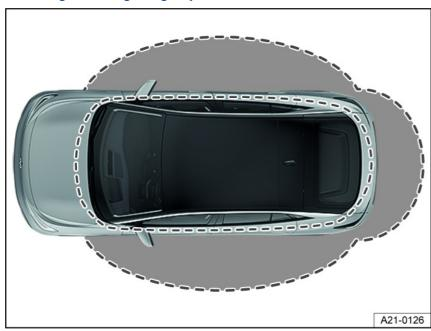
Fig. 43 Keyless Access: general example of the sensor ranges.
