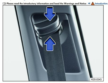
Fig. 20 Next to the front seats: safety belt height adjuster.
