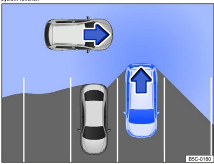
Fig. 108 Rear Traffic Alert, general example: monitored area around the vehicle that is exiting a parking space.
