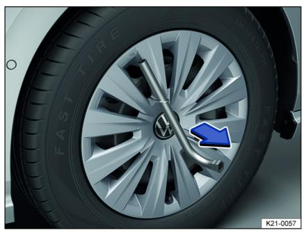
Fig. 168 Remove the wheel hub cover.
