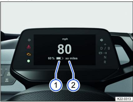
Fig. 10 In the Volkswagen Digital Cockpit: The high-voltage battery charge level (1) and vehicle range (2) (general example).
