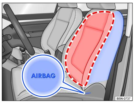
Fig. 26 On the side of the front seat: Side airbag installation location and deployment zone
