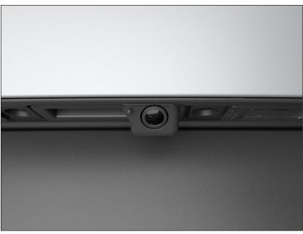
Fig. 180 In the rear of the vehicle: Rear View Camera system on the handle (general example).
