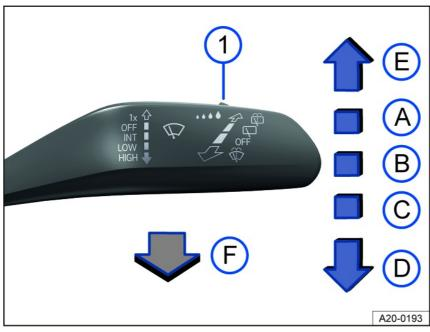
Fig. 75 On the right side of the steering column: operating the windshield wipers.
