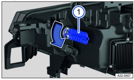
Fig. 144 In the right-side of the hood space: rear side of the headlights.
