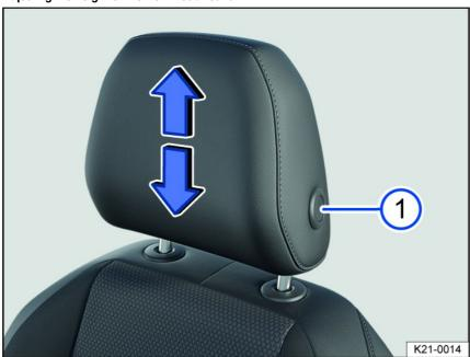
Fig. 63 Adjusting the front head restraint (general example).
