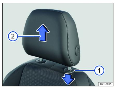
Fig. 65 Removing the front head restraint (general example).
