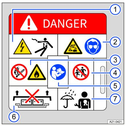
Fig. 128 Warning sign on the high-voltage battery.
