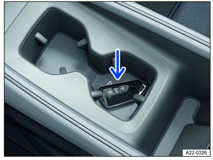
Fig. 84 In the center armrest: Emergency start function.
