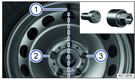
Fig. 175 Changing a tire: tire valve 1 and locations of the anti-theft wheel bolt 2 or 3.
