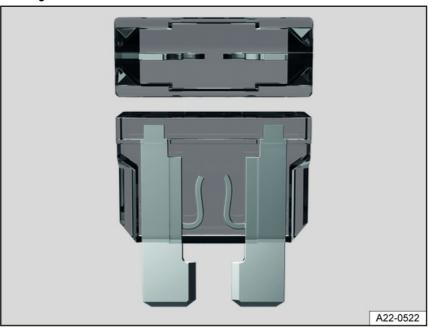
Fig. 150 Blown fuse (general example).
