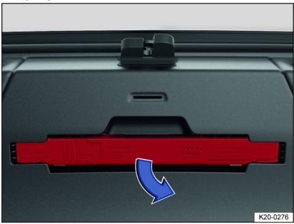
Fig. 35 In the trunk lid: Holder for the warning triangle.
