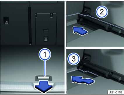
Fig. 118 In the luggage compartment: Adjusting the height of the second luggage compartment floor.
