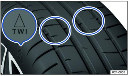
Fig. 166 Tire tread: tread wear indicator.
