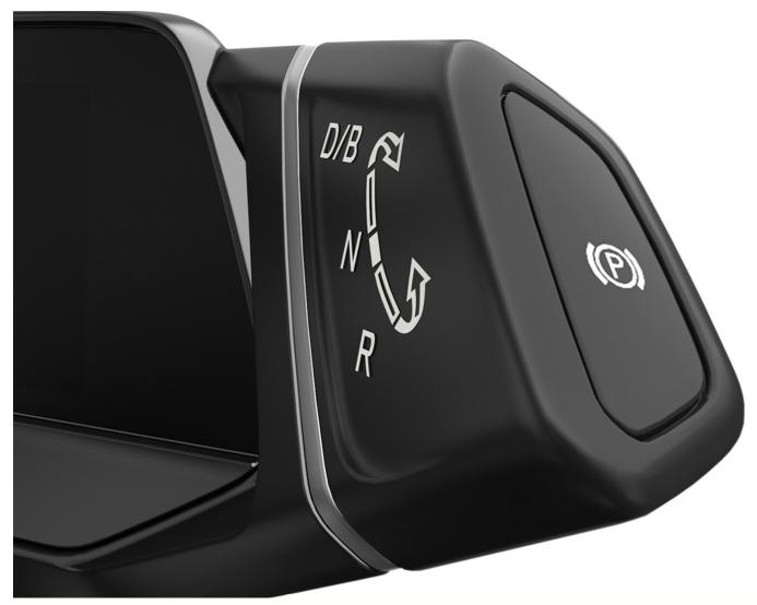
Fig. 98 On the driving mode selector: Button (2) for the electronic parking brake (general example).
