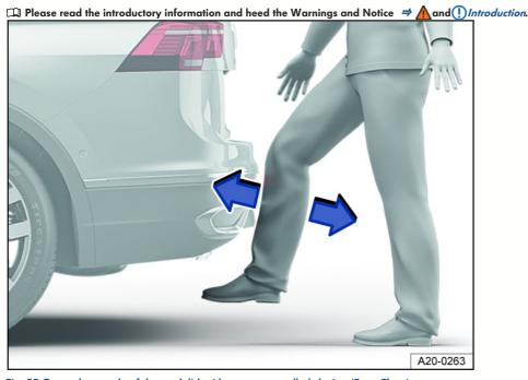
Fig. 55 General example of the trunk lid with sensor-controlled closing (Easy Close).
