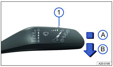
Fig. 77 On the right side of the steering column: windshield wiper lever.
