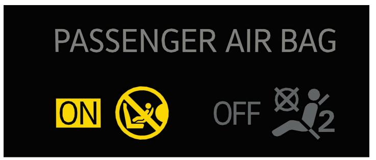
Fig. 22 In the roof console: Indicator light (general example) for the activated front passenger's front airbag.
