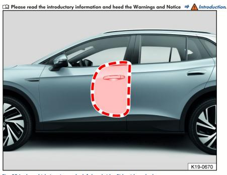
Fig. 25 In the vehicle interior on the left-hand side: Side airbag deployment zone.
