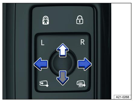
Fig. 79 In the driver door: knob for the outside mirrors.
