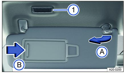
Fig. 80 In the front of the headliner: sun visor.
