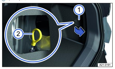
Fig. 134 In the bottom right luggage compartment trim: Emergency release of the charging connector.
