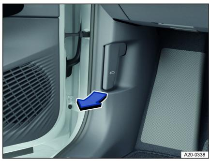
Fig. 156 In the driver's side footwell: Release lever for the hood (general example).
