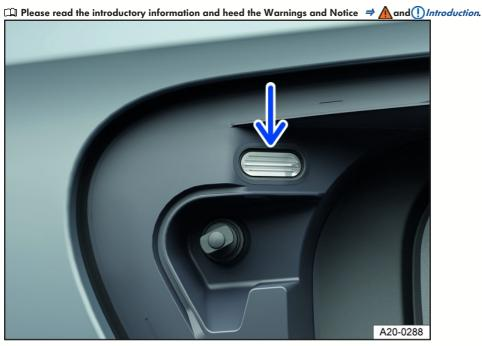
Fig. 131 Behind the charging socket flap: charging process indicator.
