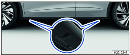
Fig. 171 Mounting points for the vehicle jack.
