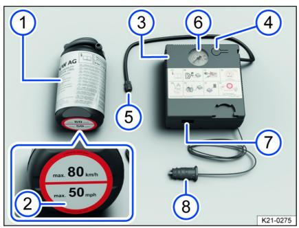
Fig. 176 Tire mobility set components (general example).
