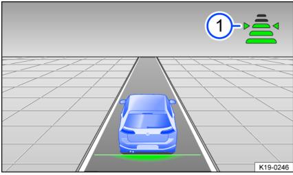
Fig. 92 In the instrument cluster display: set distance (1), ACC is regulating (general example).
