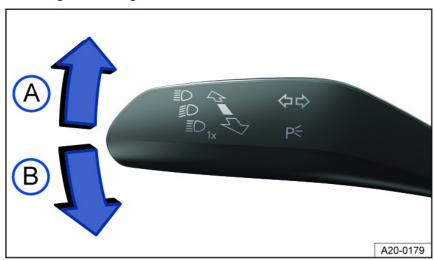
Fig. 71 On the left side of the steering column: turn signal and high beam lever.
