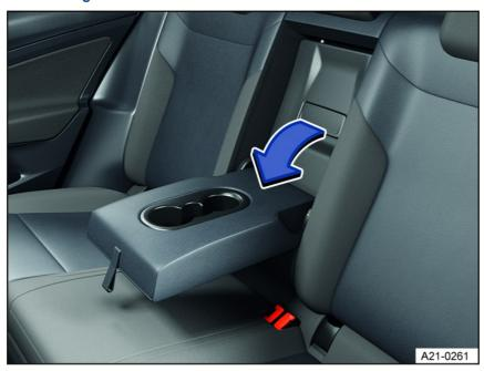
$\label{fig:prop:prop:prop:prop:seq} \textbf{Fig. 122 Pass-through in the rear seat backrest.}$
