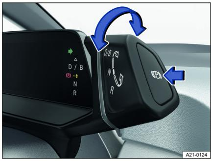
Fig. 85 Driving mode selector with the button for the electronic parking brake (arrow).
