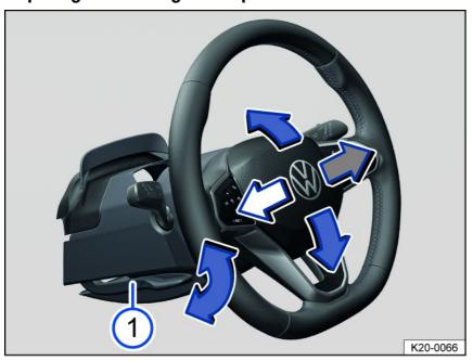
Fig. 57 Under the steering wheel in the steering column trim panel: lever to adjust the steering wheel position manually (general example).
