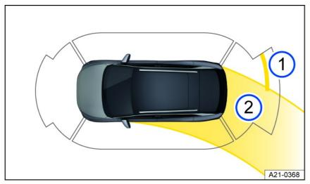
Fig. 99 Infotainment system: Display of Park Distance Control (general example).
