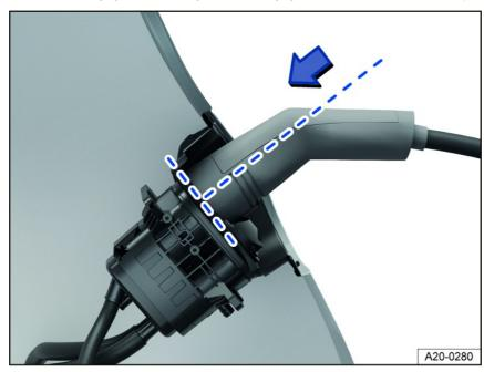
Fig. 130 Fully inserted charging connector (general example).
