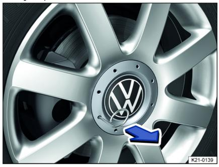
Fig. 167 Remove the hubcap.
