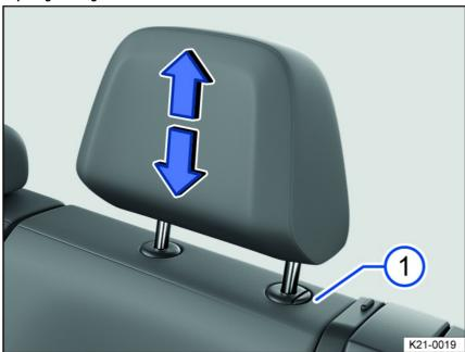
Fig. 64 Adjusting the rear head restraint (general example).
