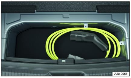
Fig. 137 Under the luggage compartment floor: Storage compartment for the charging cable (general example).
