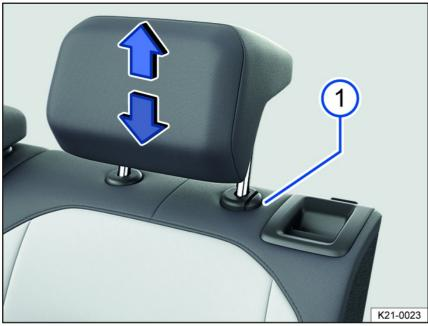
Fig. 66 Removing the rear head restraint (general example).
