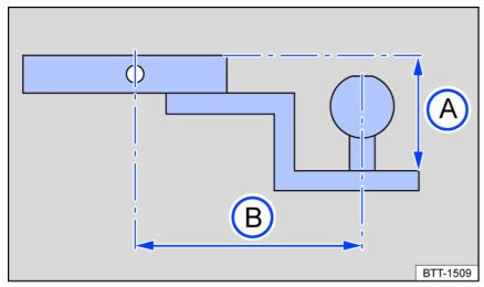
Fig. 124 Dimensions of the ball mount holder and receptacle.
