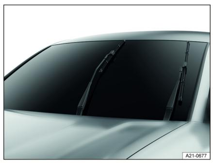
Fig. 141 Windshield wipers in service position (general example).
