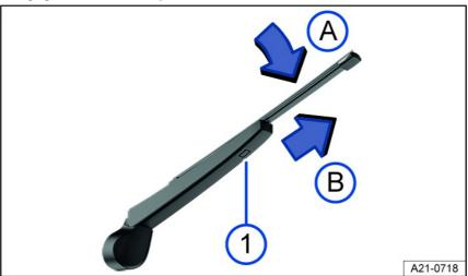
Fig. 143 Changing the rear window wiper blade.
