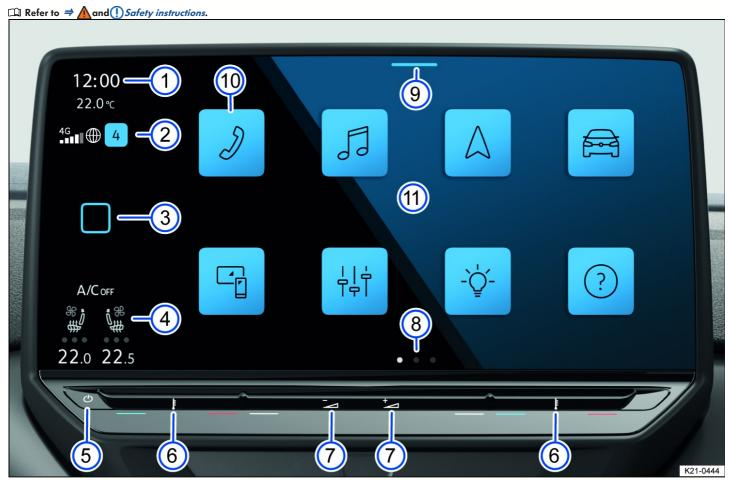
Fig. 113 Overview: display and control unit, 12" version.
