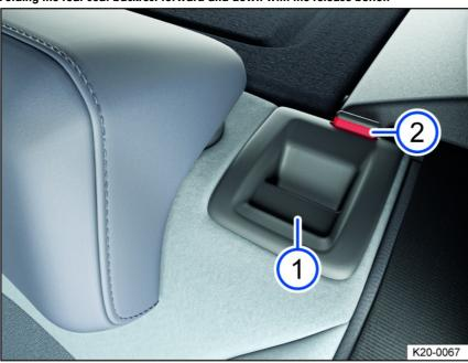
Fig. 62 In the rear seat backrest: release button.
