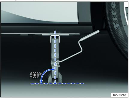
Fig. 172 Correct jack setup.
