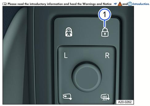
Fig. 45 In the driver door: Control for central locking.
