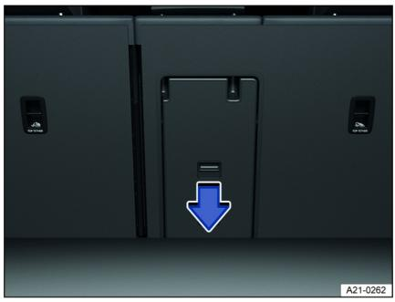
Fig. 117 Pass-through in the luggage compartment.
