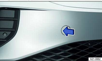
Fig. 151 In the right front bumper: Remove cover.
