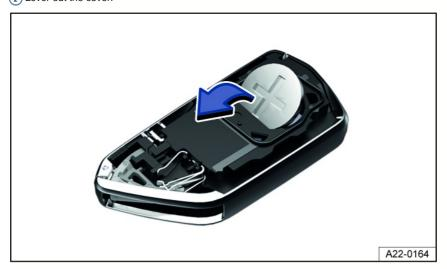
Fig. 42 Vehicle key: replacing the button cell battery
