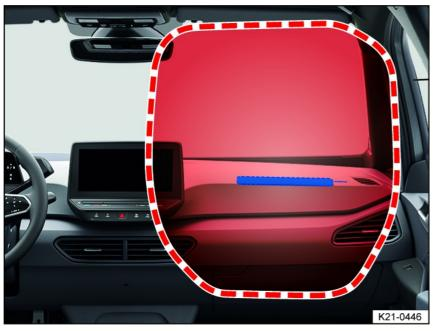
Fig. 24 Installation location and deployment zone of the front passenger's front airbag.
