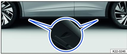
Fig. 172 Mounting points for the vehicle jack.
