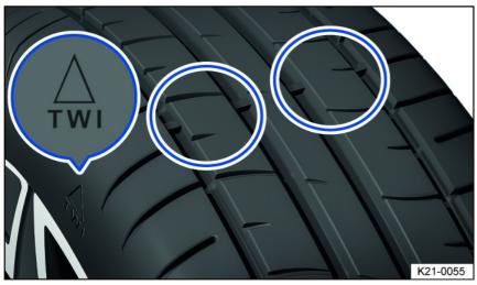
Fig. 166 Tire tread: tread wear indicator.
