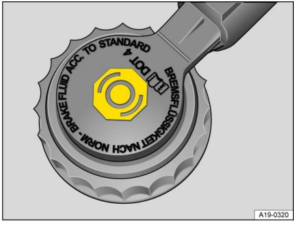
Fig. 162 In the hood space: Cap on the brake fluid reservoir (version 1).
