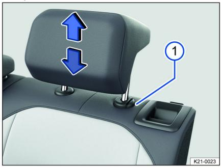
Fig. 66 General example: removing the rear head restraint.
