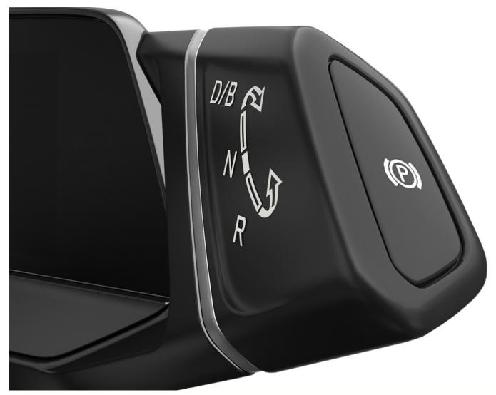
Fig. 97 On the selector lever: Button (P) for the electronic parking brake (general example).
