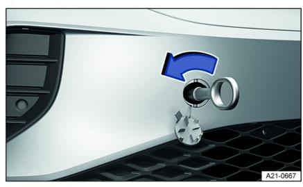
Fig. 152 In the right front bumper: Screw in towing eye.
