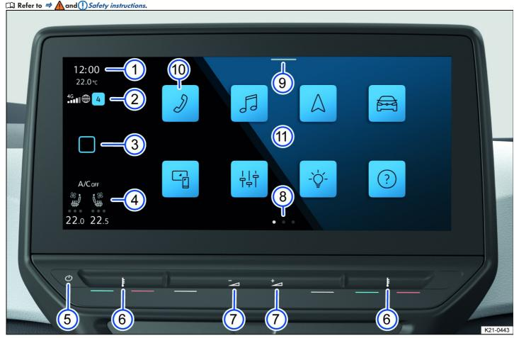
Fig. 106 Overview: display and control unit, 10" version.
