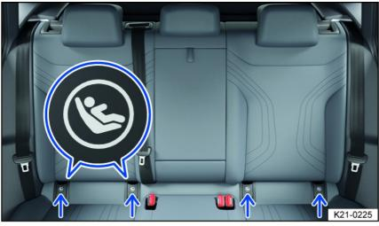
Fig. 29 On the outer seats in the rear bench seat: Designation of the ISOFIX/lower LATCH anchorage points for child restraints.
