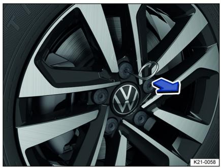
Fig. 169 Remove the caps from the wheel bolts.
