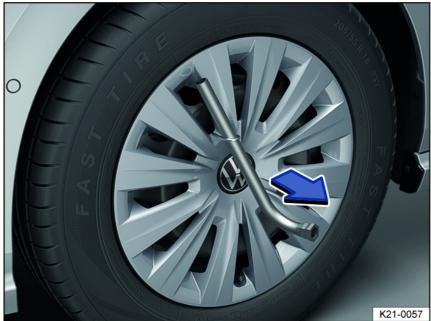
Fig. 168 Remove the wheel hub cover.
