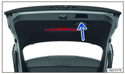
Fig. 51 In the open trunk lid: handle for closing the trunk lid (general example).
