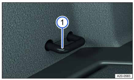
Fig. 113 In the luggage compartment: Tie-down (general example).
