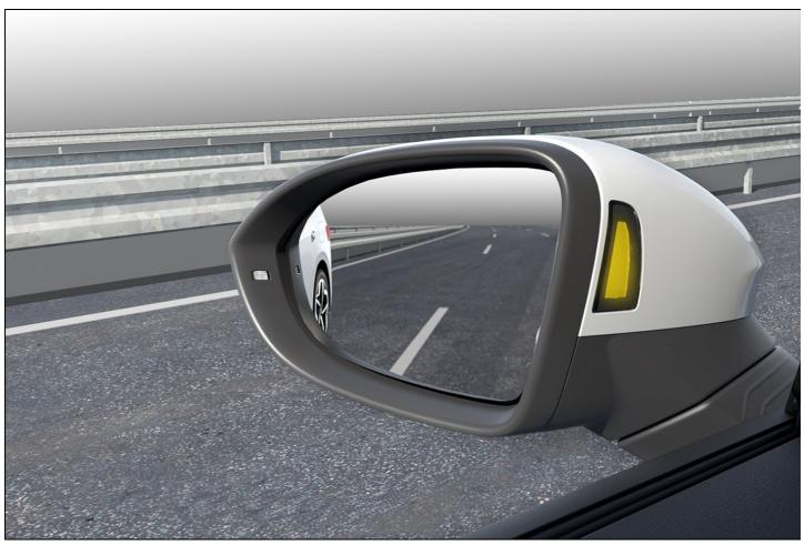
Fig. 96 In the outside mirror housing: Visual indicators for Side Assist.
