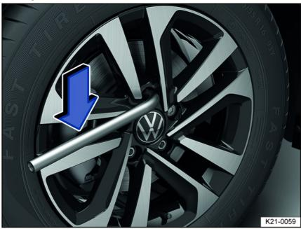
Fig. 175 Wheel change: removing wheel bolts with the lug wrench.
