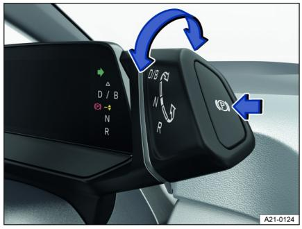
Fig. 85 Selector lever with the button for the electronic parking brake (arrow).
