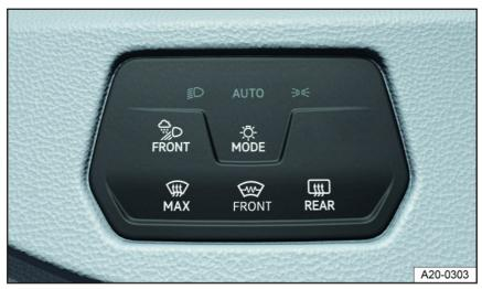
Fig. 71 Next to the steering wheel: Button to switch on the exterior lighting.
