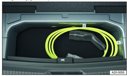
Fig. 133 Under the luggage compartment floor: Storage compartment for the charging cable (general example).
