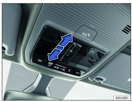
Fig. 81 In the headliner: Function keys for controlling the sunshade.
