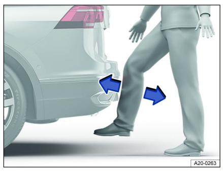
Fig. 55 General example of the trunk lid with sensor-controlled closing (Easy Close).
