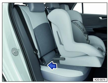
Fig. 30 General example: fitting a child restraint with attachment arms.
