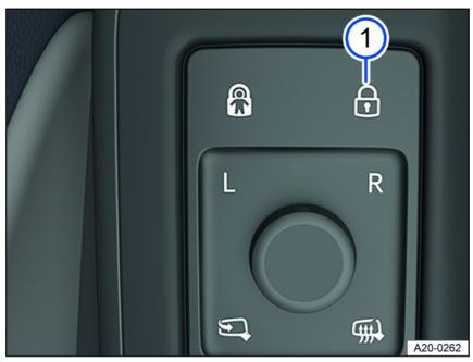
Fig. 45 In the driver door: Control for central locking.
