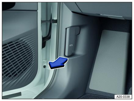
Fig. 154 In the driver's side footwell: Release lever for the hood (general example).
