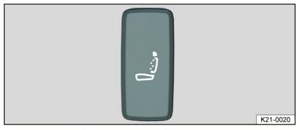
Fig. 69 In the lower part of the driver seat: Massage function button.
