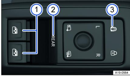
Fig. 56 In the driver door: Buttons for the front and rear power windows.
