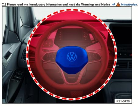
Fig. 23 Installation location and deployment zone of the driver's front airbag.
