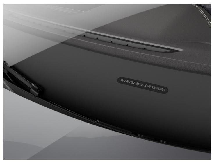
Fig. 184 In the windshield: vehicle identification number (VIN)
