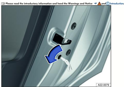
Fig. 48 In the front edge of the rear right-hand door: vehicle emergency lock for using the emergency key (general example).
