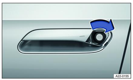
Fig. 47 Emergency locking of driver door.
