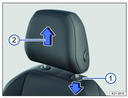
Fig. 65 General example: removing the front head restraint.
