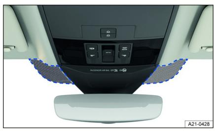
Fig. 82 Next to the mirror base: Communication window (general example).
