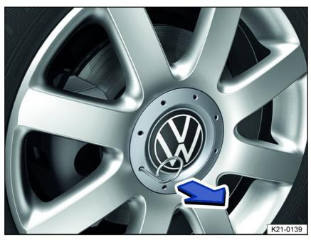
Fig. 167 Remove the hubcap.
