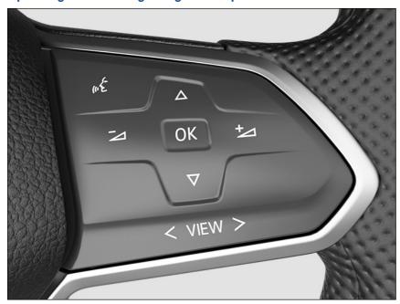
Fig. 9 Right side of the multi-function steering wheel: operating the Volkswagen Digital Cockpit.
