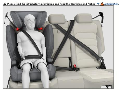
Fig. 34 Correctly fastened child on a booster seat.
