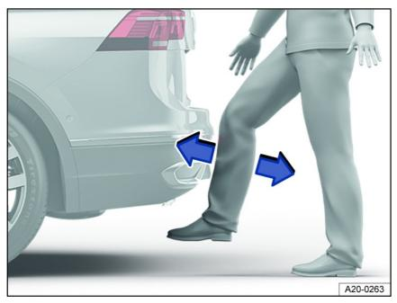
Fig. 54 General example of the sensor-controlled luggage compartment opener (Easy Open).
