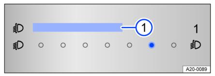
Fig. 73 In the Infotainment system: Touch control for headlight range control.
