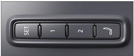
Fig. 68 On the outer side of the driver's seat: memory buttons.
