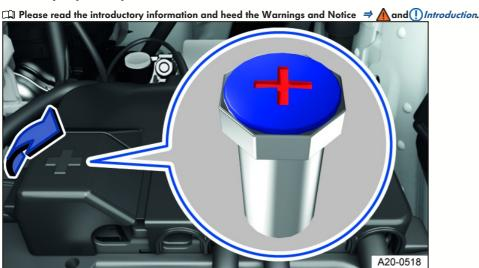
Fig. 149 Under a cover in the hood space: Positive jump-start point.
