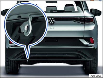
Fig. 153 At the rear of the vehicle: fixed towing eye installation location for a tow truck.
