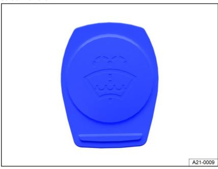
Fig. 159 In the hood space: Cap on the washer fluid reservoir (general example).
