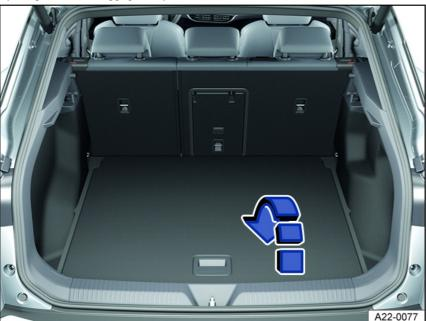
Fig. 111 In the luggage compartment: Opening the second luggage compartment floor.
