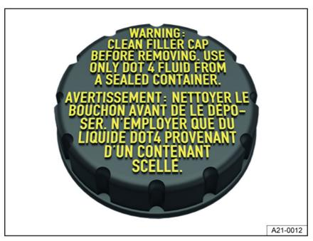
Fig. 163 In the hood space: Cap on the brake fluid reservoir (version 2).
