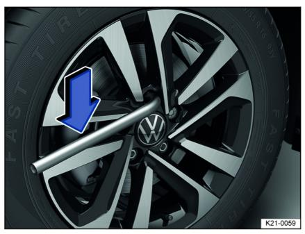
Fig. 170 Changing a tire: loosening the wheel bolts.
