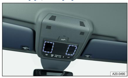
Fig. 74 On the overhead console: touch-sensitive reading lights.
