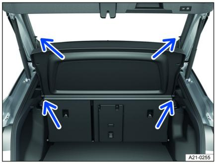
Fig. 109 In the luggage compartment: Installing and removing the luggage compartment cover.
