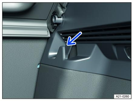
Fig. 115 Shopping bag hooks on the left and right of the luggage compartment.
