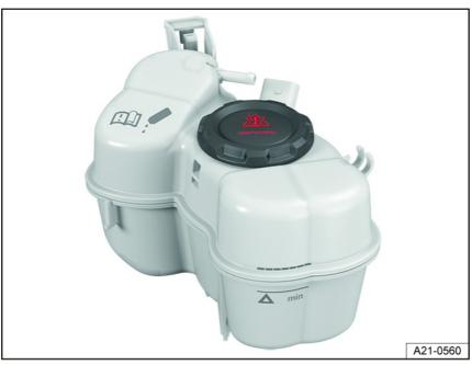
Fig. 161 In the hood space: markings on the engine coolant expansion tank (general example).
