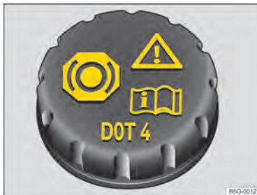
Fig. 181 In the bonnet space: cap of the brake fluid reservoir.
