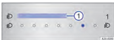
Fig. 89 In the Infotainment system: touch slider for headlight range control.
