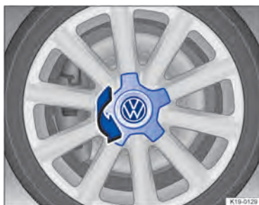
Fig. 188 Removing the centre wheel trim by turning.
