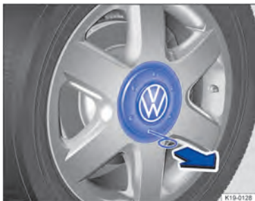
Fig. 187 Removing the centre wheel trim by pulling off.
