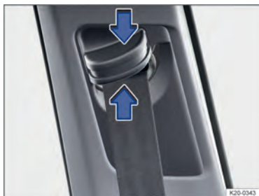
Fig. 30 Next to the front seats: belt height adjuster.
