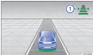
Fig. 109 On the instrument cluster display: set distance ①, ACC regulating (illustration).
