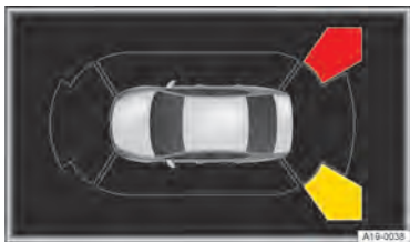
Fig. 120 On the Infotainment system: Rear Traffic Alert display.
