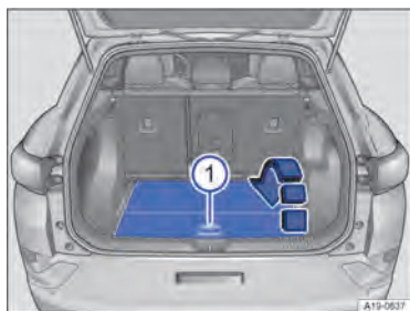
Fig. 127 In the luggage compartment: opening the second luggage compartment floor.
