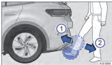
Fig. 69 Sensor-controlled luggage compartment opener (Easy Open).
