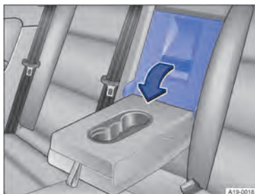
Fig. 134 In the rear seat backrest: opening the load-through hatch.
