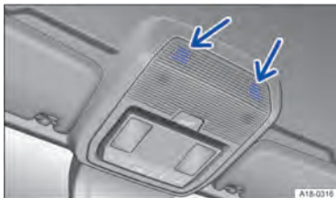
Fig. 64 In the roof console: sensors for the interior monitoring system (arrows).
