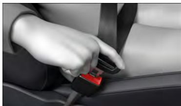
Fig. 26 Inserting the seat belt latch plate into the buckle.
