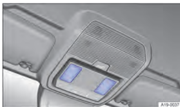
Fig. 90 In the roof console: touch-sensitive reading lights.
