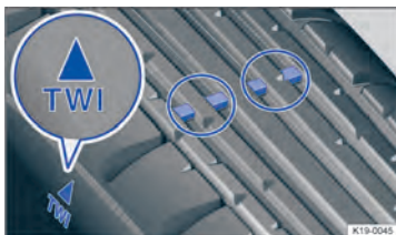
Fig. 185 Tyre tread: tread wear indicators.
