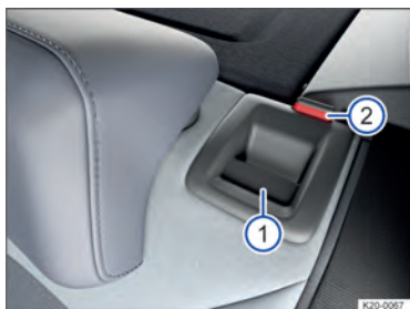
Fig. 77 In the rear seat backrest: release button.
