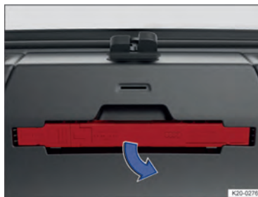
Fig. 50 In the boot lid: holder for the warning triangle.
