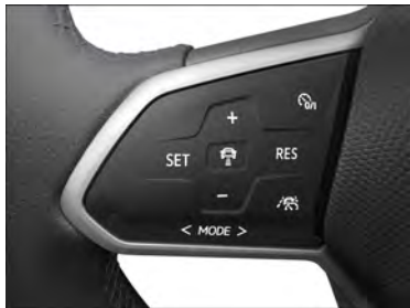
Fig. 112 Lefthand side of the multifunction steering wheel.
