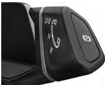
Fig. 114 On the driving mode selector: button for the electronic parking brake.
