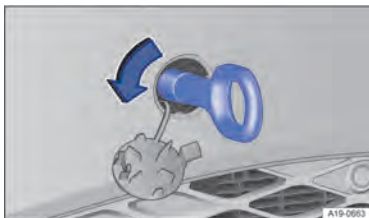
Fig. 170 In the front bumper on the right: screwing in the towing eye.
