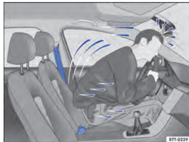
Fig. 23 An unbelted driver is thrown forwards.
