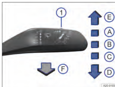
Fig. 91 On the right-hand side of the steering column: operating the windscreen wipers.
