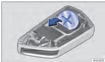
Fig. 56 Vehicle key: replacing the button cell.
