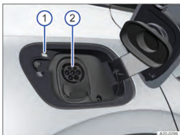
Fig. 145 Behind the charging socket flap at the rear right: charging socket.
