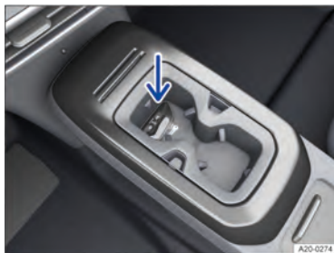
Fig. 99 In the centre console: emergency start function.
