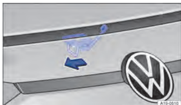
Fig. 174 On the bonnet: control lever.
