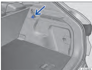
Fig. 133 On the left and right in the luggage compartment: bag hooks.
