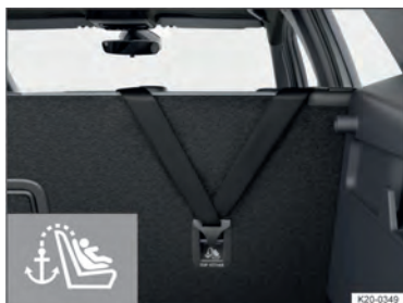
Fig. 47 In the luggage compartment: attached top tether.
