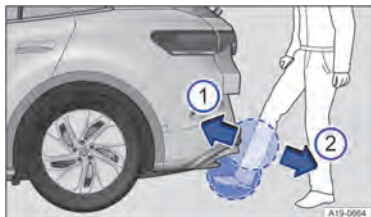
Fig. 70 Boot lid with sensor-controlled closing (Easy Close).
