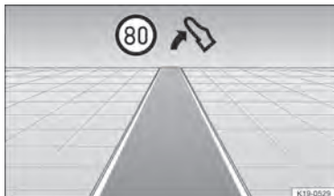
Fig. 17 Eco Assistance display (illustration).
