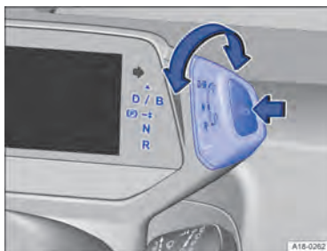
Fig. 100 Position switch with button for the electronic parking brake (arrow).
