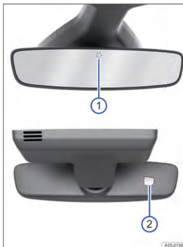
Fig. 94 On the windscreen: automatic anti-dazzle interior mirror.
