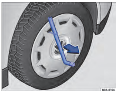
Fig. 189 Removing the wheel cover.
