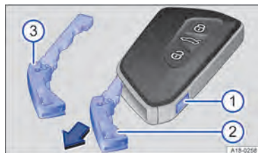
Fig. 54 Vehicle key: releasing the spare key.
