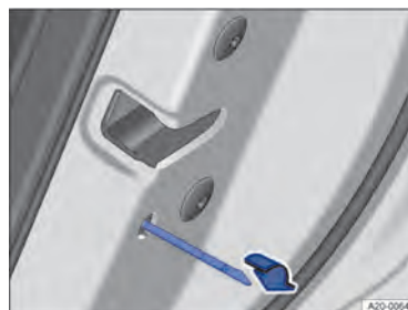
Fig. 62 In the end face of the right-hand door: locking the vehicle manually with the spare key.
