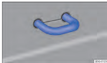
Fig. 131 In the luggage compartment: fastening ring.
