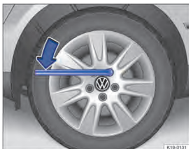
Fig. 191 Changing a wheel: loosening the wheel bolts.
