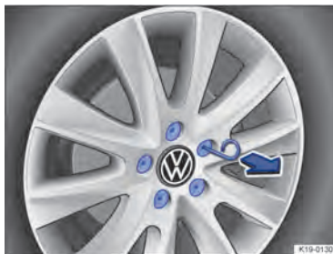
Fig. 190 Removing the wheel bolt caps.
