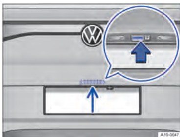
Fig. 65 In the boot lid: button for opening the boot lid.
