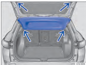
Fig. 125 In the luggage compartment: removing and installing the luggage compartment cover.
