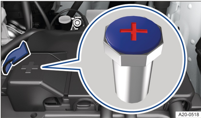
Fig. 1 In the bonnet space underneath a cover: jump-start connection point (positive battery terminal).
