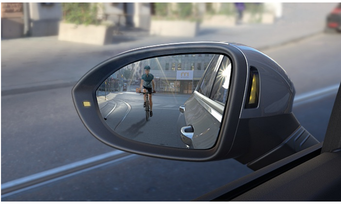
Fig. 2 In the exterior mirror housing: visual display of the exit warning system.
