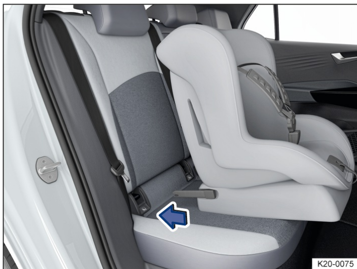
Fig. 1 Illustration: fitting a child seat with the attachment arms.
