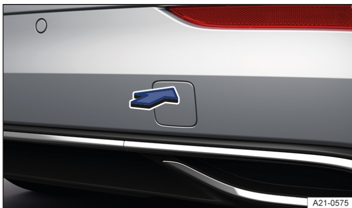
Fig. 1 In the rear bumper on the right: removing the cover, variant 1.
