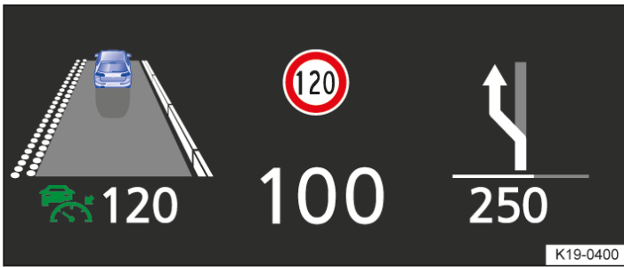
Fig. 1 In the driver's field of vision: example displays in the head-up display
