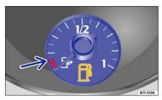
Fig. 147 In the instrument cluster: Fuel gauge.
