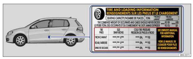
Fig. 162 Location of the tire inflation pressure label.
