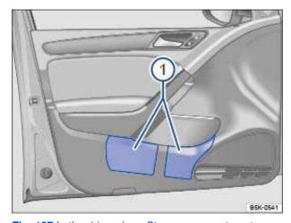
Fig. 107 In the driver door: Storage compartment.
