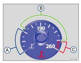
Fig. 154 Engine coolant temperature gauge in the instrument cluster: A Engine cold; B Normal temperature range; C Warning zone.
