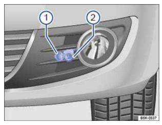
Fig. 124 In the front left bumper: Connection socket 2 for the engine preheating system.
