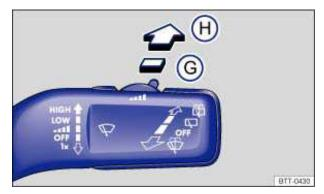
Fig. 91 Operating the rear wiper.
