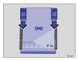
Fig. 190 In the engine compartment: Fuse box cover.
