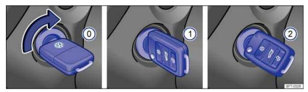
Fig. 121 In the ignition switch: Vehicle key positions.
