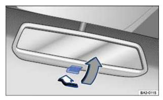
Fig. 94 Manually adjustable inside mirror.
