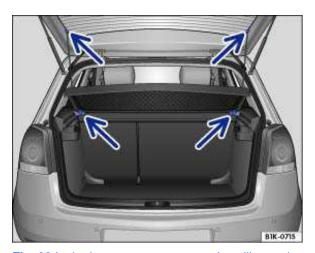
Fig. 98 In the luggage compartment: Installing and removing the luggage compartment cover.
