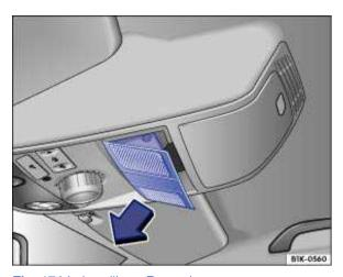
Fig. 174 In headliner: Removing cover.
