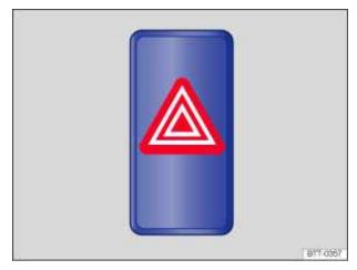
Fig. 169 In the center of the instrument panel: Switch for emergency flashers.
