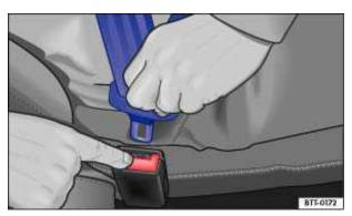
Fig. 55 Releasing the buckle tongue from the belt buckle.
