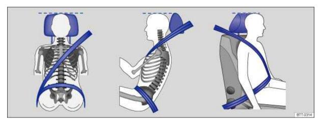
Fig. 56 Proper safety belt positioning and head restraint adjustment.
