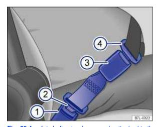
Fig. 59 A safety belt extender properly attached to the factory-installed safety belt.
