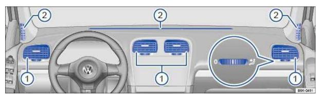
Fig. 146 In the instrument panel: Air vents.
