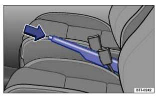
Fig. 133 Between the front seats: Parking brake.
