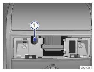
Fig. 175 Hexagonal head screw for closing the power sunroof.
