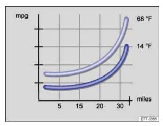
Fig. 136 Fuel consumption in mpg at 2 different outside air temperatures.
