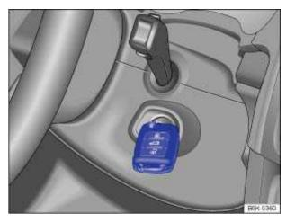
Fig. 123 Emergency starting feature on vehicles with Keyless Access.
