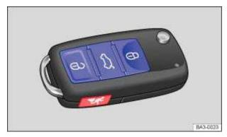
Fig. 24 Remote control vehicle key with panic button.
