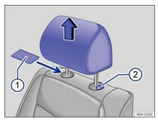
Fig. 41 Removing the front head restraints.
