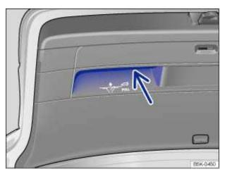
Fig. 32 Opened rear hatch: Recessed grips for closing.
