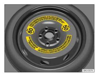
Fig. 165 In the luggage compartment: Compact spare wheel.
