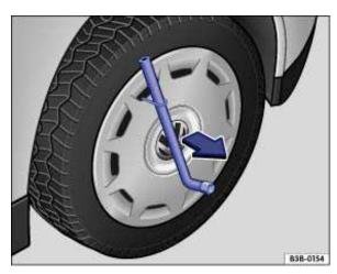
Fig. 182 Pulling the wheel cover off.
