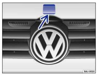
Fig. 151 Above the radiator grille: Outside engine hood release.
