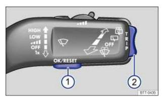
**Fig. 15** In vehicles without a multi-function steering wheel: Use button 1 in the windshield wiper lever to confirm menu items and rocker switch 2 to switch menus.
