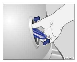
Fig. 31 Opening rear hatch from the outside.
