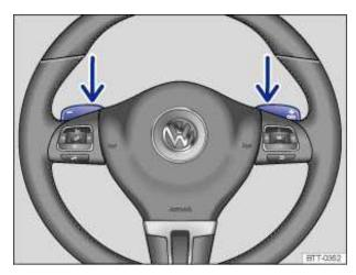
Fig. 132 Steering wheel with optional Tiptronic shift paddles.
