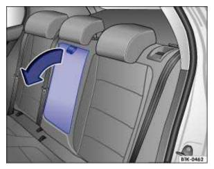
Fig. 45 Folding down the rear center armrest.
