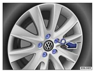
Fig. 183 Pulling cover caps off wheel bolts.
