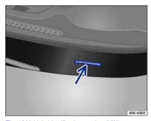
Fig. 18 Vehicle identification number (VIN).
