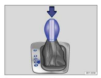
Fig. 130 Automatic transmission selector lever with shift lever release button (arrow).
