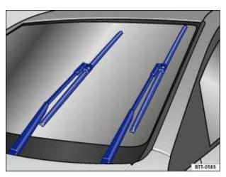
Fig. 92 Windshield wiper in service position.
