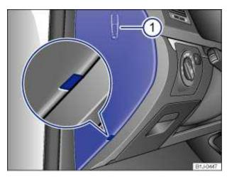
Fig. 189 On the driver side in the instrument panel: Fuse box cover with plastic tweezers 1 on the inside of the cover.
