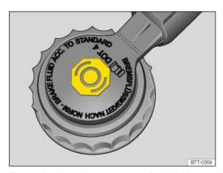
Fig. 135 In the engine compartment: Brake fluid reservoir cap.
