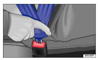
Fig. 54 Inserting the safety belt buckle tongue into the belt buckle.
