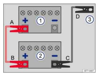
Fig. 202 Diagram for attaching the jumper cables: Dead battery 1 and booster battery 2.
