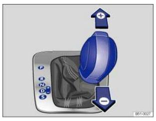
Fig. 131 Selector lever in Tiptronic position.
