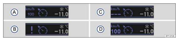
Fig. 139 In the instrument cluster display: Cruise control status indications.
