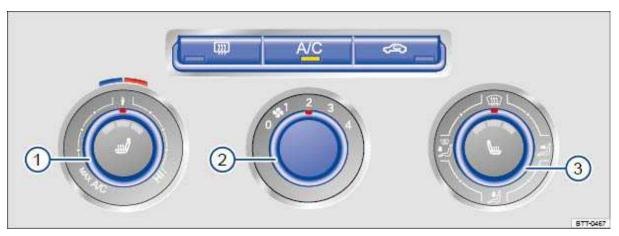
Fig. 144 In the center console: Manual AC controls.
