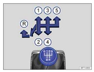
Fig. 127 Gearshift pattern of a 5-speed manual transmission.
