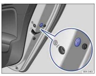
Fig. 171 On the front side of the right rear door: Emergency lock, covered by a rubber seal.
