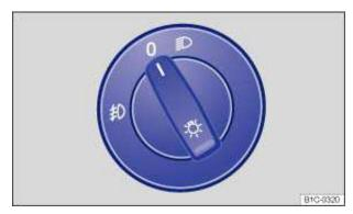
Fig. 86 Headlight switch next to the steering wheel (with fog lights).
