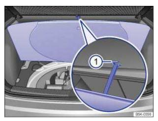
Fig. 178 In the luggage compartment: Floor covering raised and 1 secured.
