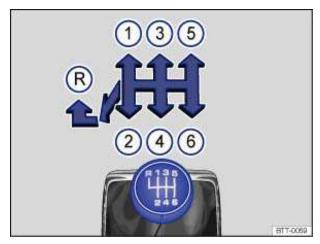
Fig. 128 Gearshift pattern of a 6-speed manual transmission.
