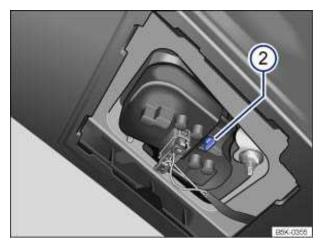
Fig. 197 In the rear hatch: Removing the bulb holder.
