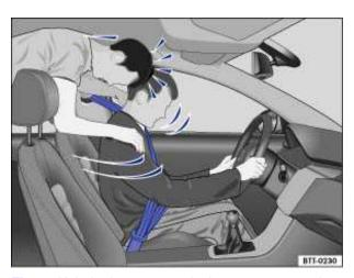
Fig. 52 Unbelted passengers in the rear seats are thrown forward on top of the belted driver.
