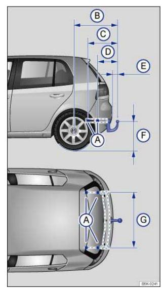
Fig. 106 Dimensions and attachment points for retrofitting a trailer hitch.
