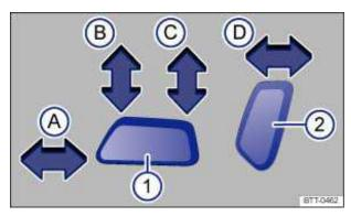
Fig. 38 Driver seat: Controls to adjust the seat backward and forward, adjust seat cushion height and angle, and backrest angle (if applicable).
