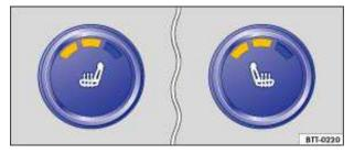
Fig. 46 In the center console: Seat heating buttons for the front seats.
