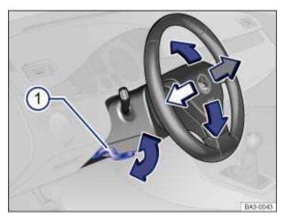
Fig. 43 Manual adjustment for the steering wheel position.
