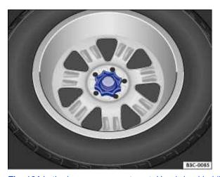
Fig. 164 In the luggage compartment: Handwheel holding the spare wheel in place.
