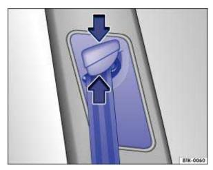
Fig. 58 Next to the front seats: Safety belt height adjuster.
