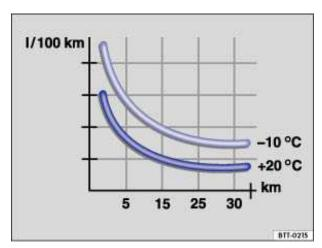
Fig. 137 Fuel consumption in I/100 km at 2 different outside air temperatures.
