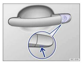
Fig. 170 Door handle on driver door: Concealed lock cylinder.
