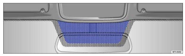
Fig. 89 Heat-reflective windshield with communications window (blue shaded area).
