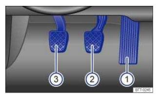
Fig. 125 Pedals in vehicles with manual transmission: 1 Accelerator pedal, 2 Brake pedal, 3 Clutch pedal.
