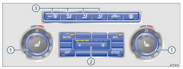
Fig. 145 In the center console: Climatronic controls.
