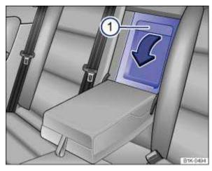
Fig. 99 In the rear seat backrest: Opening the luggage compartment pass-through.
