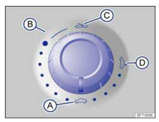
Fig. 34 In the headliner: Rotary switch for the power sunroof.
