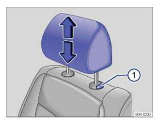
Fig. 40 Adjusting the head restraints.
