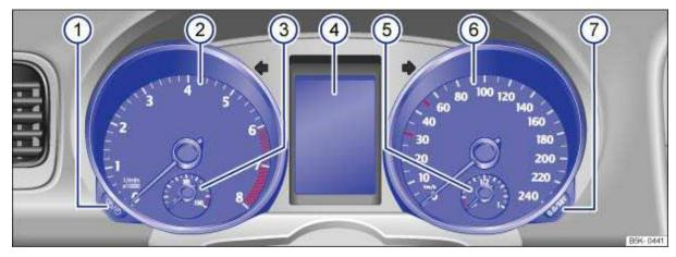
Fig. 12 Instrument cluster in the instrument panel.
