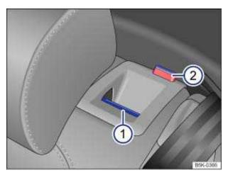
Fig. 97 Rear seat backrest: release button 1; red mark 2.
