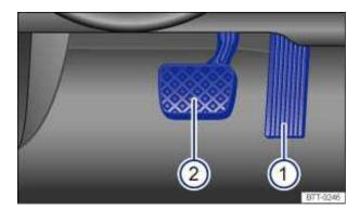
Fig. 126 Pedals in vehicles with automatic transmission: 1 Accelerator pedal, 2 Brake pedal.
