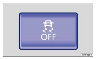
Fig. 134 In the center console: Button for switching ASR on and off manually.
