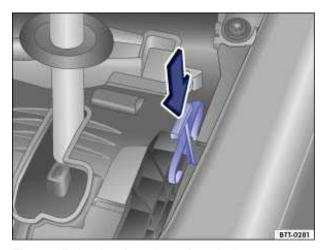
Fig. 177 Releasing the selector lever lock.
