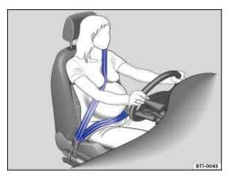
Fig. 57 Proper safety belt positioning for expectant mothers.
