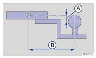
Fig. 105 Dimensions of the ball mount support.
