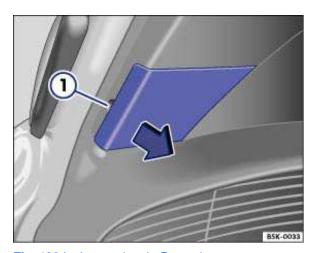
Fig. 196 In the rear hatch: Removing cover.
