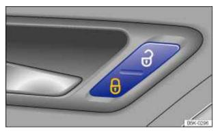
Fig. 25 In the driver and front passenger doors: Power locking button.
