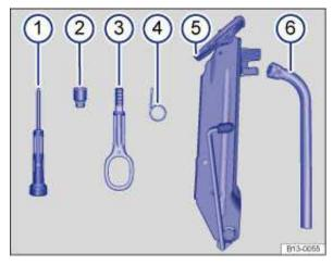
Fig. 179 Contents of the vehicle tool kit.
