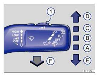
Fig. 90 Operating the front windshield wipers.
