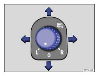
Fig. 96 In the driver door: Adjusting knob for the outside mirrors.
