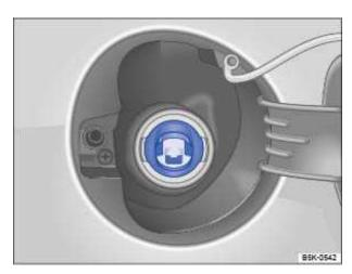
Fig. 149 With open fuel cap: Misfueling guard in the fuel filler neck.
