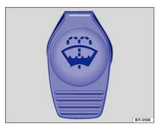
Fig. 93 In the engine compartment: Cap of the windshield washer fluid reservoir.
