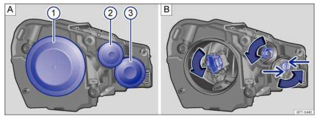
Fig. 193 In the engine compartment: Covers in the left headlight assembly. 1 Low beam, 2 Turn signal indicator, 3 High beam and parking light as well as daytime running light.
