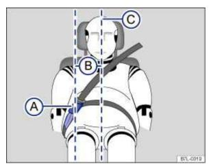
Fig. 60 Positioning of the safety belt extender.
