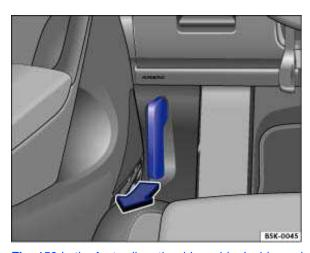
Fig. 150 In the footwell on the driver side: Inside engine hood release lever.
