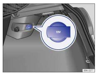
Fig. 120 In the luggage compartment: 12 Volt socket.
