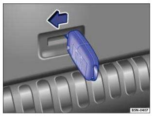
Fig. 173 Inside the luggage compartment: Opening the rear hatch.
