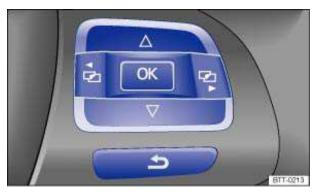
Fig. 16 Right side of the multi-function steering wheel (if applicable): Controls for the menus in the instrument cluster.
