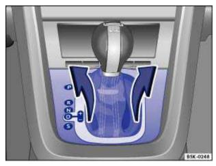
Fig. 176 Removing the selector gate cover.
