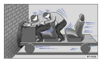
Fig. 50 A vehicle with passengers not wearing safety belts hits a wall.
