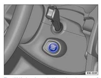
Fig. 122 Keyless Access locking and starting system: Starter button.
