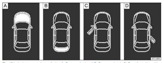
Fig. 13 In the instrument cluster display: A: Open engine hood, B: Open rear hatch, C: Open front driver side door, D: Open rear passenger side door.
