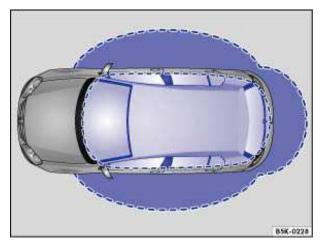
Fig. 26 Ranges of the Keyless Access locking and starting system. Outside the vehicle: Unlocking range. Inside the vehicle: Starting range.
