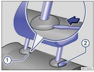
Fig. 42 Removing the rear head restraints.
