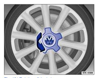
Fig. 181 Twisting off the hubcap.
