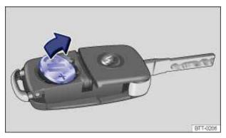
Fig. 23 Remote control vehicle key: Remove old battery.
