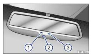
Fig. 95 Auto-dimming inside mirror (if applicable): Version A and Version B.
