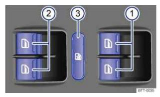
Fig. 33 In the driver door: Switches for front and rear power windows (4-door version shown).
