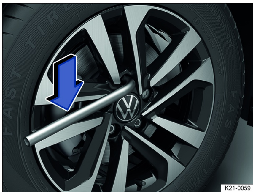
Fig. 201 Changing a tire: loosening the wheel bolts.
