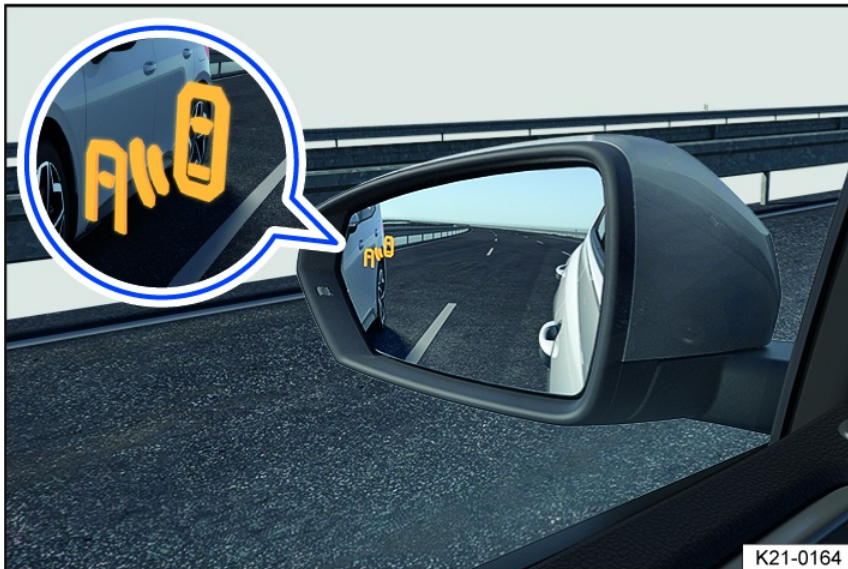
Fig. 135 In the outside mirror: Visual indicators for Side Assist.
