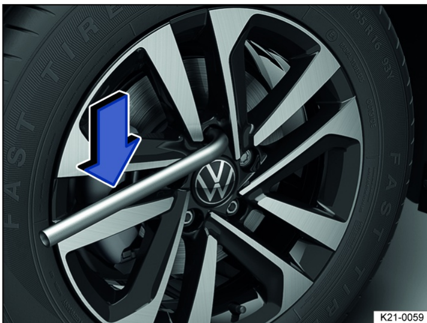
Fig. 207 Wheel change: removing wheel bolts with the lug wrench.
