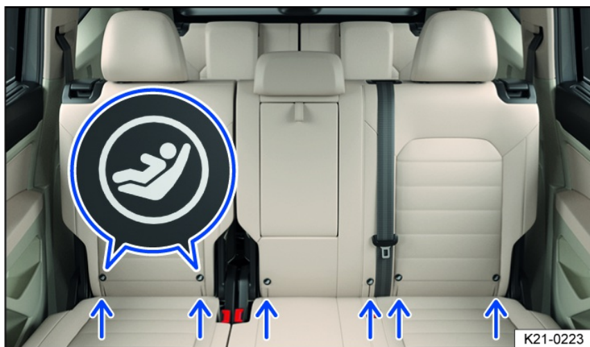
Fig. 34 On the second-row seats: Designation and symbol showing the ISOFIX/lower LATCH anchorage points for child restraints.
