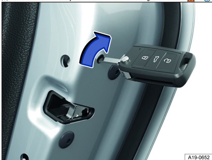
Fig. 56 On the front of the right rear door: emergency locking the vehicle with the vehicle key (general example).
