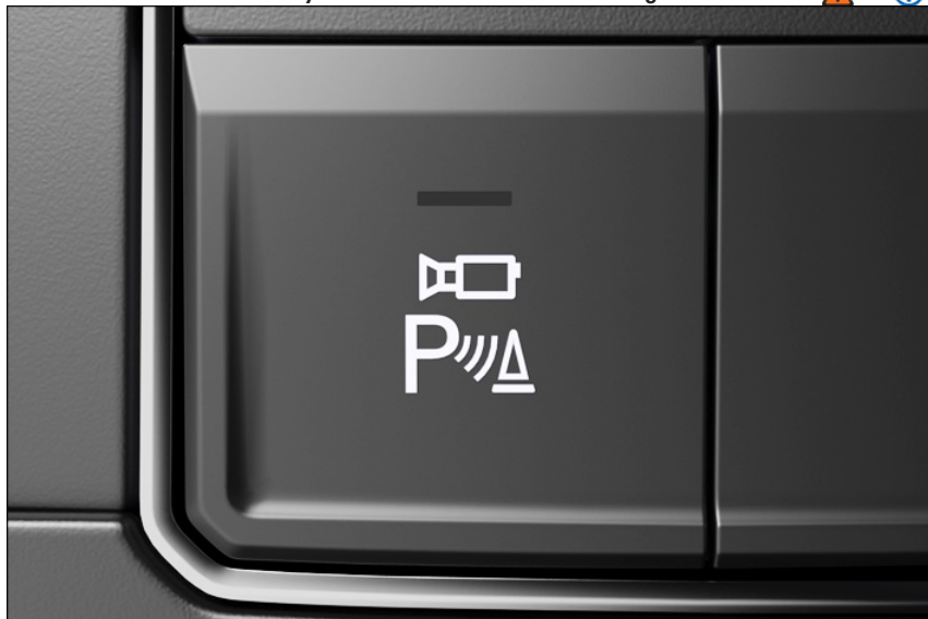
Fig. 146 In the center console: Button for switching the Area View on and off.
