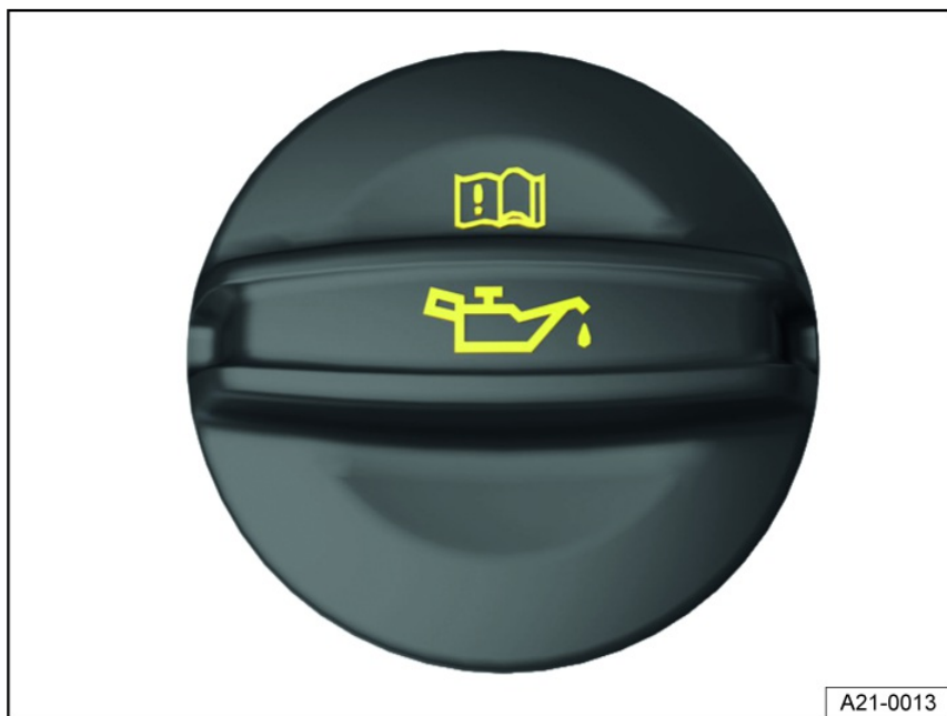
Fig. 187 In the engine compartment: engine oil filler cap (general example).
