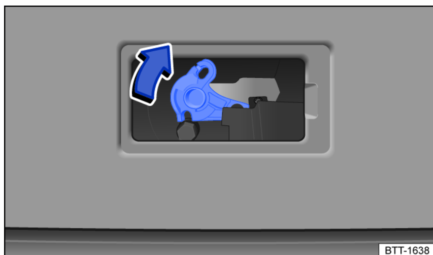
Fig. 65 In the luggage compartment: trunk lid emergency release.
