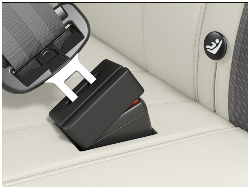
Fig. 41 Protective cap for belt buckles: Remove the protective cap.
