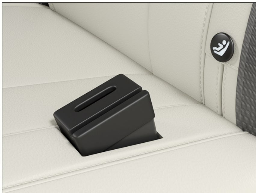
Fig. 40 Protective cap for belt buckles: Fitted protective cap.
