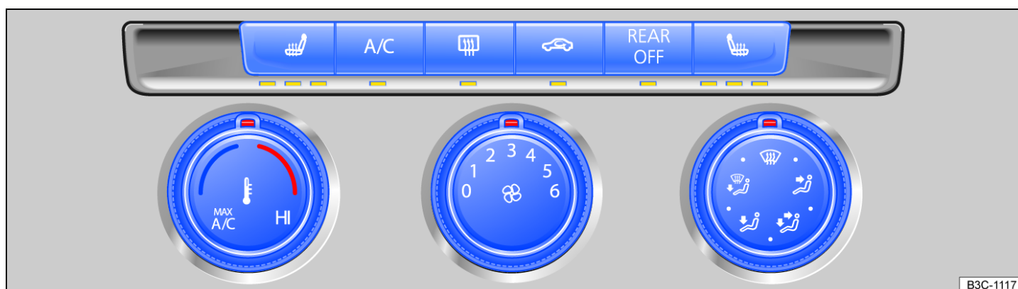
Fig. 103 In the upper section of the center console: Climate control bar for the manual climate control system.
