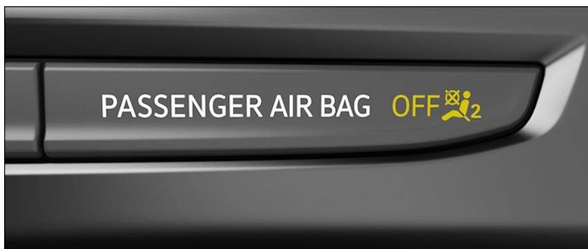
Fig. 27 In the center console: indicator light for the deactivated passenger front airbag.
