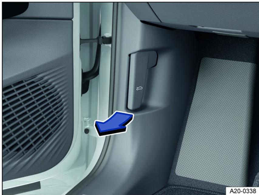
Fig. 183 In the driver's side footwell: Release lever for the hood (general example).
