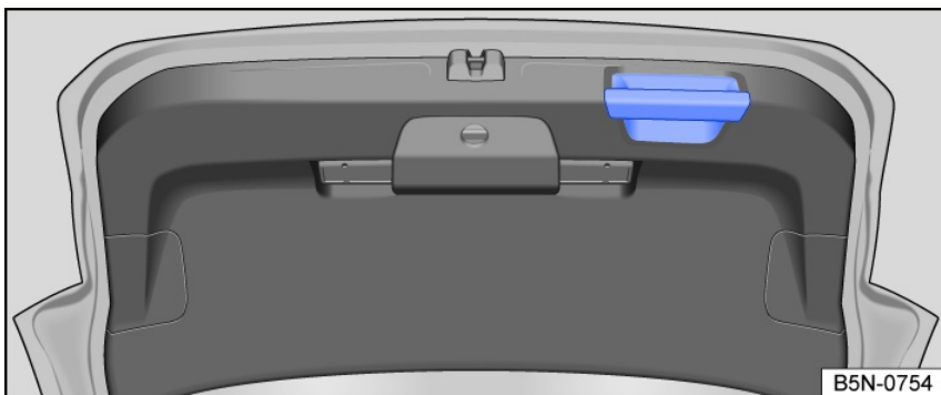
Fig. 59 In the open trunk lid: handle for closing the trunk lid.
