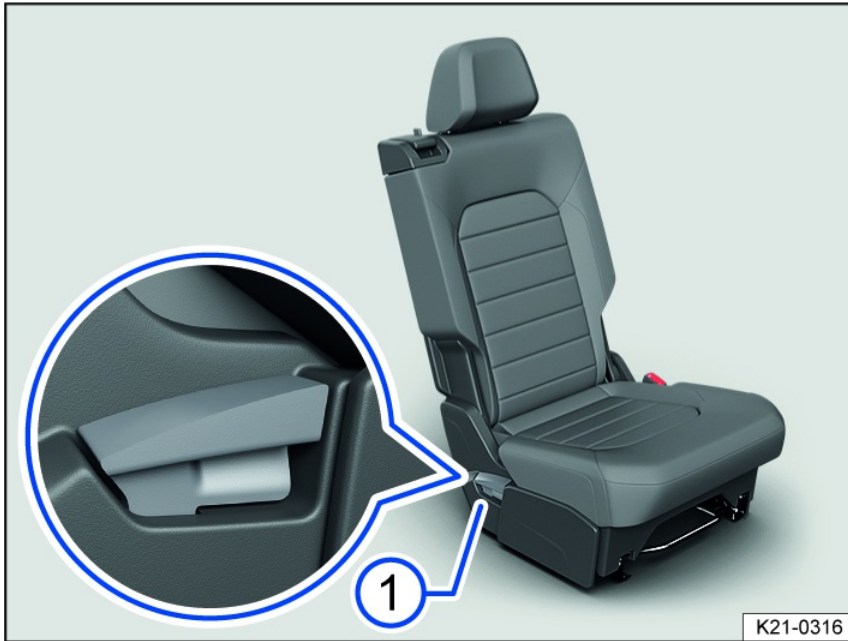
Fig. 76 Second row seats: folding the outer rear seats forward into the cargo floor position.
