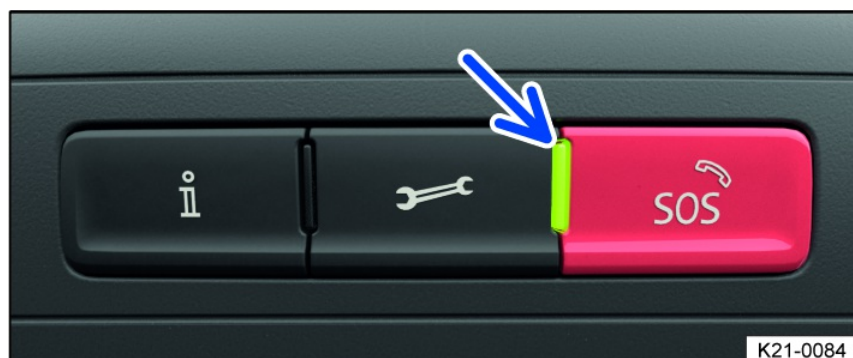
Fig. 43 In the roof console: controls for call services.
