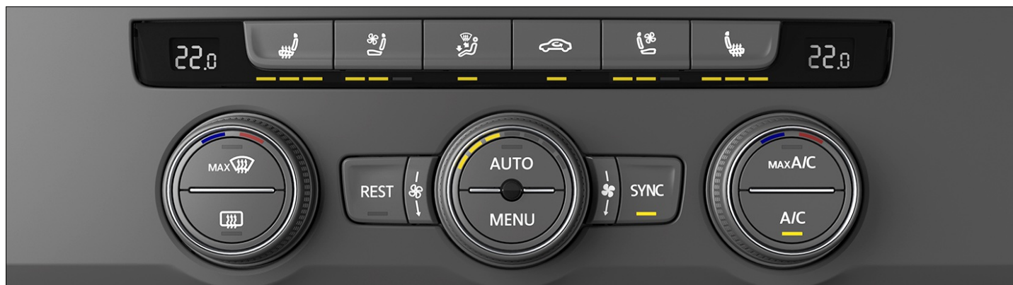
Fig. 102 In the upper section of the center console: Climate control bar for the Climatronic system.
