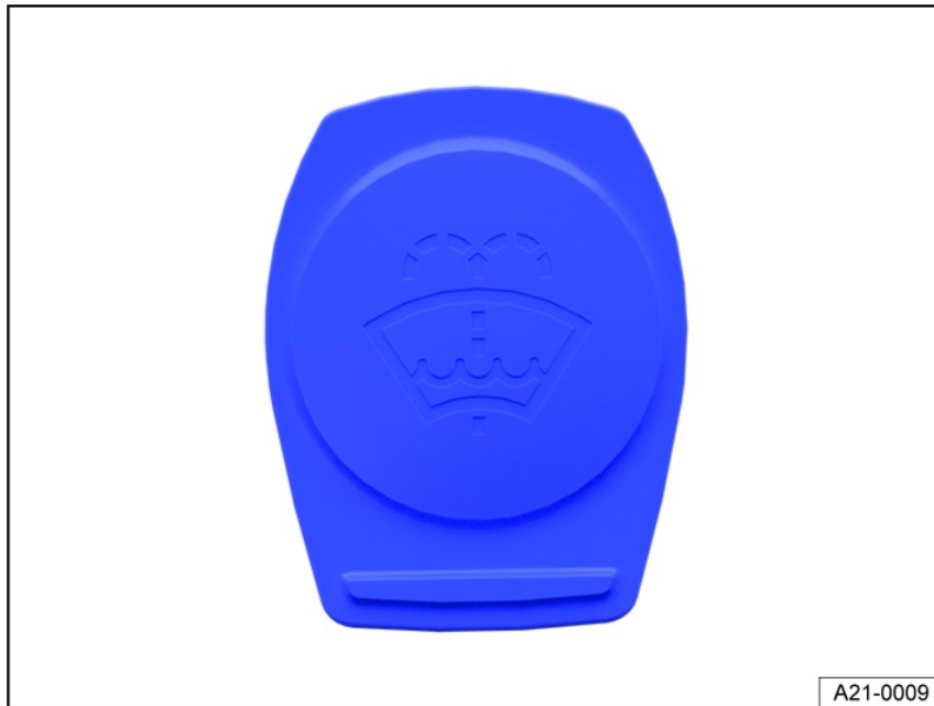
Fig. 186 In the engine compartment: Cap on the washer fluid reservoir (general example).
