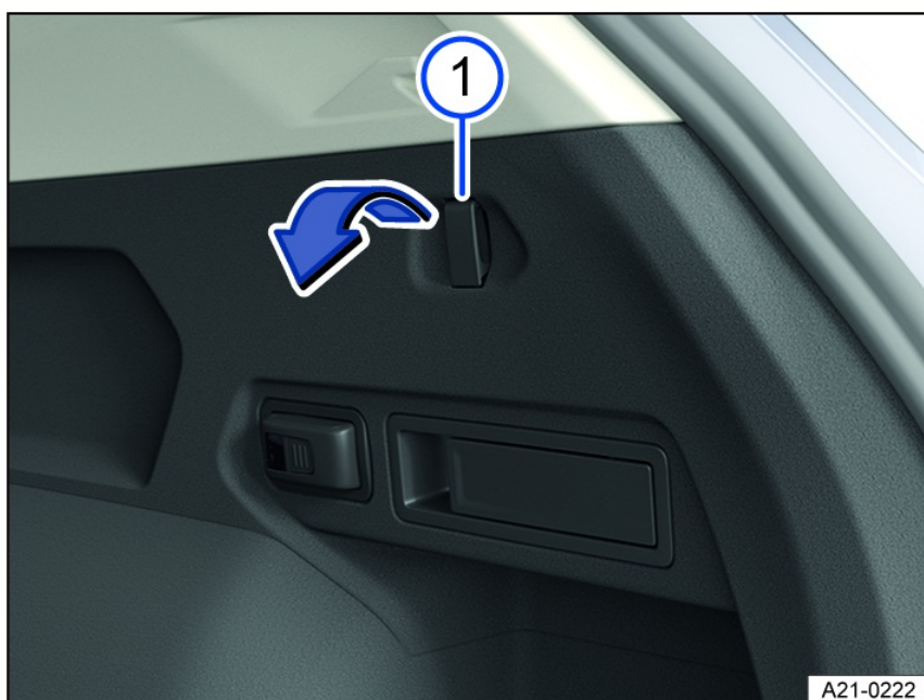
Fig. 163 In the luggage compartment: fold-out shopping bag hooks.
