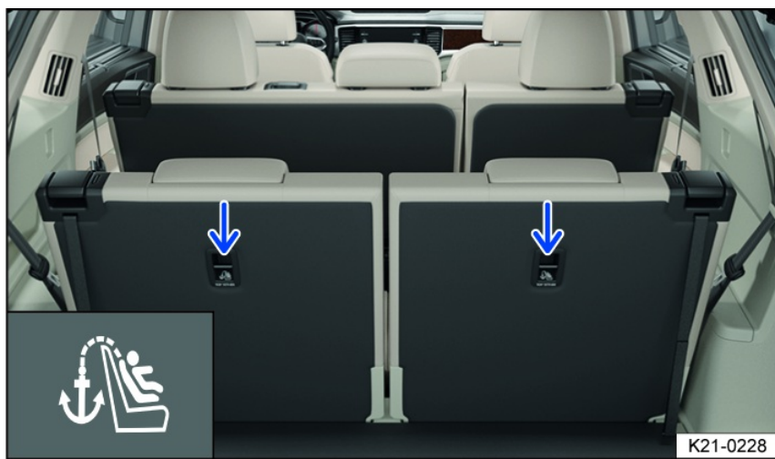
Fig. 37 On the back of the third-row seats: Top tether anchorages for the top tether safety belt.
