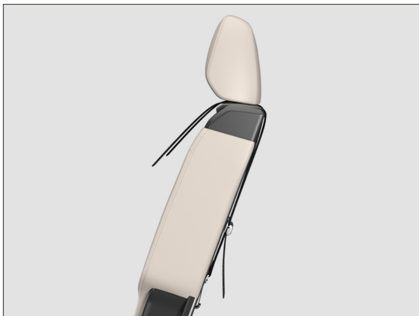
Fig. 38 On the rear side of the rear bench seat: Attached top tether safety belt.
