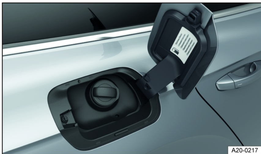
Fig. 166 Behind the fuel filler flap: fuel tank cap (general example)
