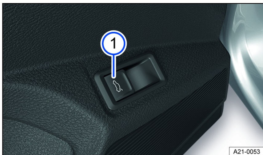
Fig. 54 In the driver's door: Button for powered opening of the trunk lid (general example).
