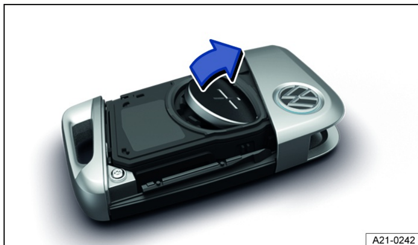
Fig. 50 Vehicle key: replacing the button cell battery
