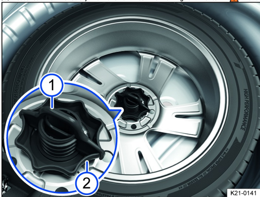
Fig. 203 In the luggage compartment: handle to secure the compact spare wheel.
