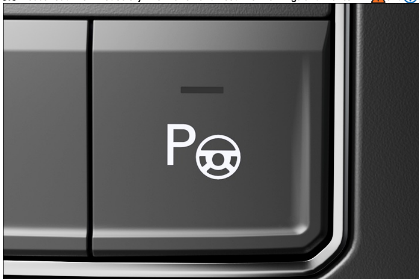
Fig. 142 In the center console: Park Assist button.
