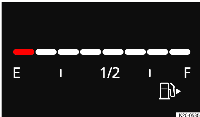
Fig. 16 Fuel gauge on the Volkswagen Digital Cockpit Basic version (general example).
