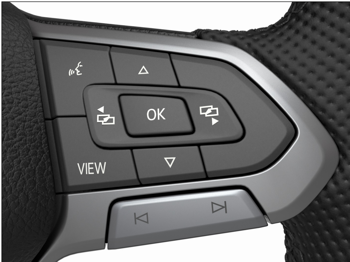
Fig. 13 Right side of the multi-function steering wheel: buttons for operating the menus and information displays in the Volkswagen Digital Cockpit Basic Version (version 1).
