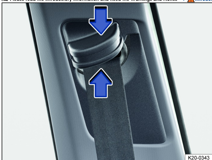
Fig. 26 Next to the front seats: safety belt height adjuster.
