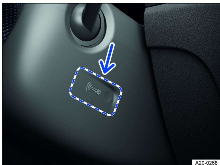
Fig. 110 On the right side of the steering column: emergency start function on vehicles with Keyless Access with push-button start.
