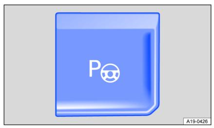
Fig. 145 In the center armrest: button to manually switch on Park Assist.
