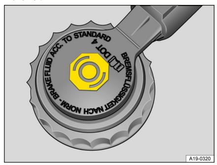
Fig. 196 In the engine compartment: cap on the brake fluid reservoir variant A.
