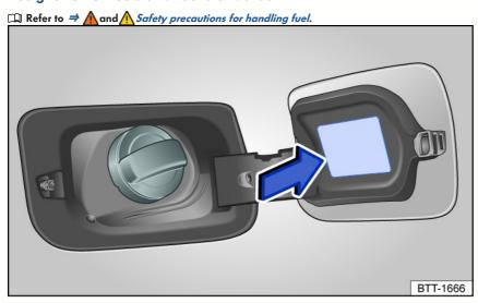
Fig. 170 On the inside of the fuel filler flap: fuel label (general example)
