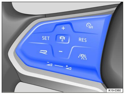
Fig. 131 Left side of the multi-function steering wheel: buttons for ACC operation (variant 2).
