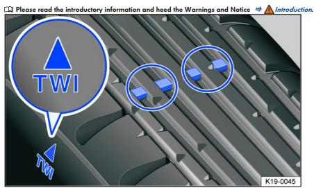
Fig. 201 Tire tread: tread wear indicator.
