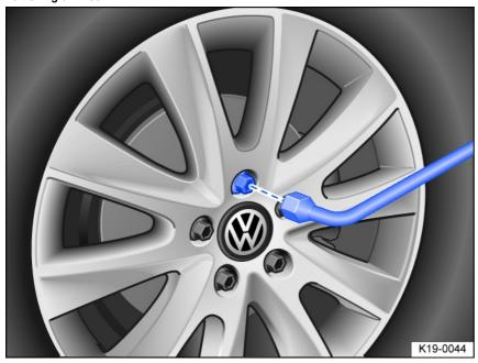
Fig. 211 Wheel change: removing wheel bolts with the lug wrench.
