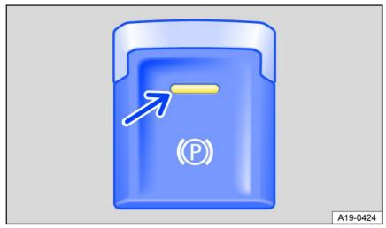
Fig. 138 In the center console: button for the electronic parking brake.
