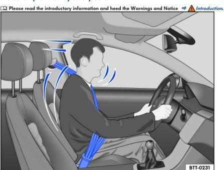
Fig. 26 Driver that is restrained during a braking maneuver by a safety belt that is fastened correctly.
