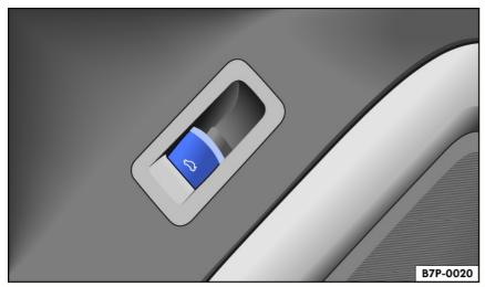
Fig. 64 In the driver door: Button for power opening the trunk lid.
