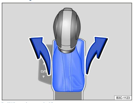
Fig. 116 Remove the cover on the shift gate.
