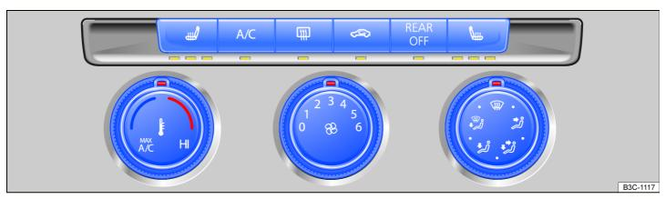
Fig. 104 In the upper section of the center console: Climate control bar for the manual climate control system.
