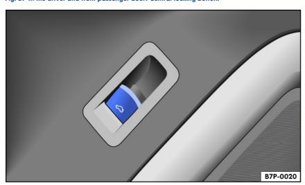
Fig. 58 In the driver door: Button for power opening the trunk lid.
