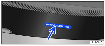
Fig. 214 In the windshield: vehicle identification number (VIN)
