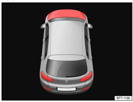
Fig. 190 In the instrument cluster display: the hood is open or not closed correctly (general example).
