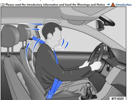
Fig. 24 Driver that is restrained during a braking maneuver by a safety belt that is fastened correctly.
