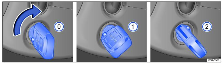
Fig. 106 Next to the steering wheel on the right side: positions of the vehicle key in the ignition lock.
