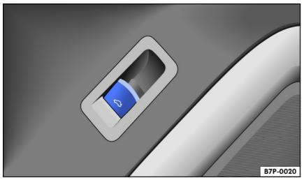
Fig. 62 In the driver door: button for powered opening of the trunk lid.
