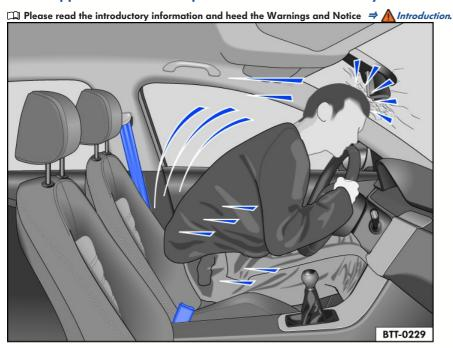
Fig. 22 A driver not wearing a safety belt is propelled forward.
