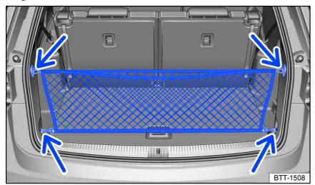
Fig. 151 In the luggage compartment: cargo net secured on the loading edge.
