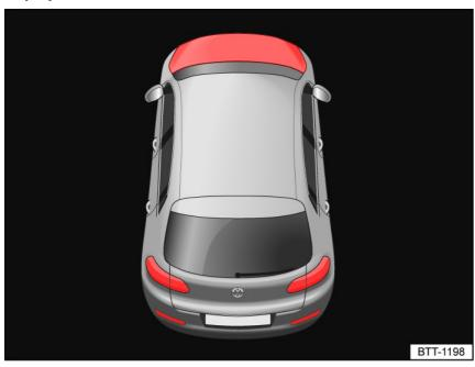
Fig. 176 In the instrument cluster display: the hood is open or not closed correctly (general example).
