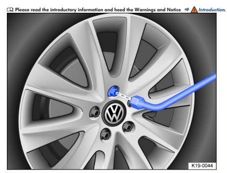
Fig. 198 Wheel change: removing wheel bolts with the lug wrench.
