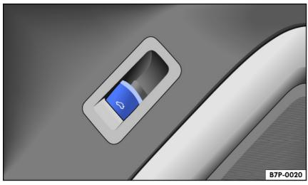
Fig. 55 In the driver door: Button for electrically opening the trunk lid.
