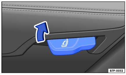
Fig. 75 Left side area in the rear bench seat: adjusting lever.
