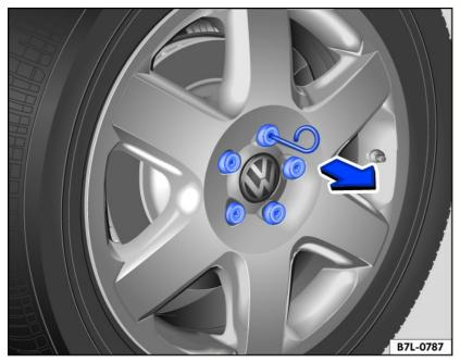
Fig. 191 Remove the caps from the wheel bolts.
