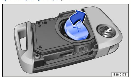
Fig. 51 Vehicle key: replacing the button cell battery.
