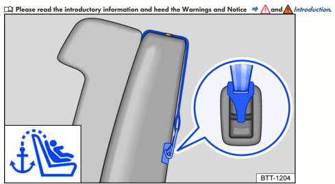
Fig. 38 On the back side of the second seat row: anchorages for the top tether.
