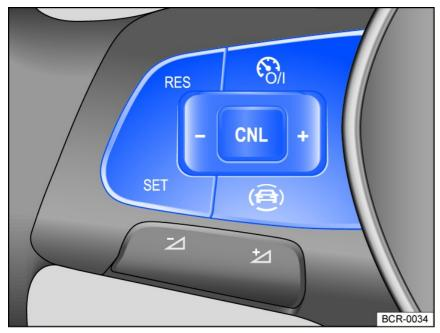
Fig. 121 Left side of the multifunction steering wheel: buttons for cruise control system operation.
