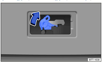
Fig. 66 In the luggage compartment: luggage compartment lid emergency release
