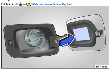
Fig. 155 On the inside of the fuel filler flap: fuel label (general example)
