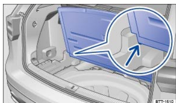
Fig. 190 In the luggage compartment: Holding the luggage compartment floor in place.
