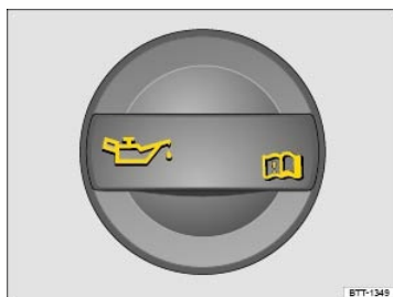
Fig. 218 In the engine compartment: Engine oil filler cap (cap design may vary depending on vehicle equipment).
