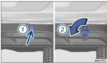
Fig. 212 In the right rear bumper: Installing the towing eye.
