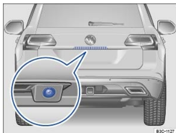
Fig. 159 In the trunk lid: Location of the camera.
