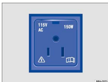
Fig. 183 Rear center console: Open cover for access to the 115 Volt outlet (if equipped).
