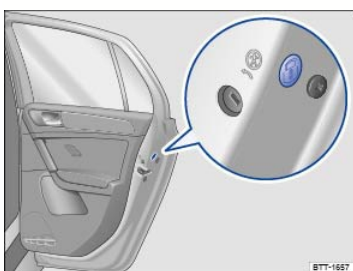
Fig. 68 on the rear passenger door: Manual lock, covered by a rubber seal.
