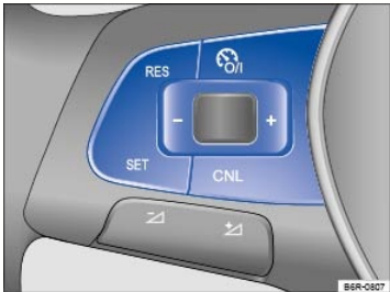
Fig. 136 Left-hand side of the multi-function steering wheel: Buttons for operating the cruise control.
