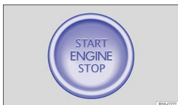
Fig. 121 In the lower center console: Starter button for the Keyless Access system.
