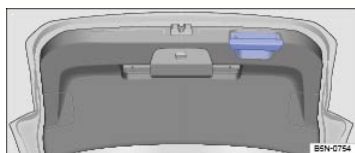
Fig. 73 Open trunk lid: Handle for closing the trunk lid.
