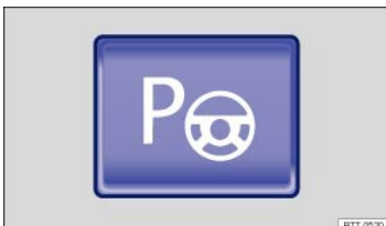
Fig. 166 In the lower center console: Button for switching on the Park Assist system.
