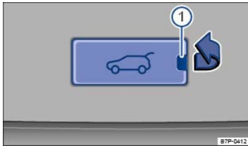
Fig. 76 Inside the luggage compartment: Cover for manually unlocking the trunk lid.
