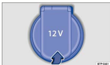
Fig. 182 In the lower center console, in the rear center console, or on the left side of the luggage compartment: 12 Volt socket with cover.
