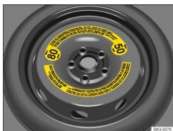
Fig. 227 In the luggage compartment: Compact spare wheel.
