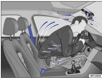
Fig. 27 The unbelted driver is thrown forward.
