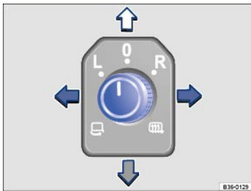
Fig. 108 In the driver door: Adjusting knob for the outside mirrors.
