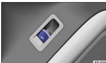
Fig. 61 In the driver door: Switch to open the trunk lid.
