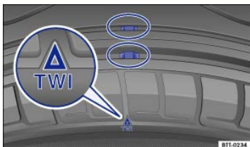
Fig. 225 Tread pattern: Wear indicator.
