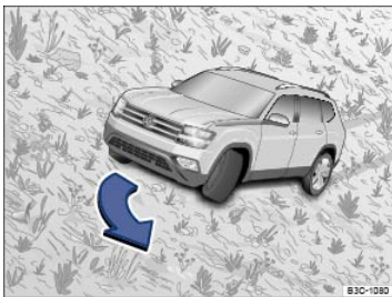
Fig. 133 Steer downhill along the fall line.
