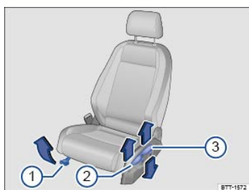
Fig. 84 Driver seat: Manual seat adjustment controls.
