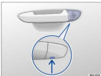
Fig. 66 Driver door: Concealed lock cylinder.
