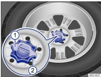
Fig. 226 In the luggage compartment: Handwheel holding the compact spare wheel in place.
