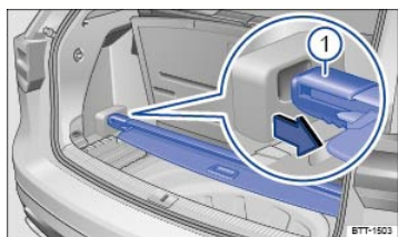
Fig. 191 Under the luggage compartment floor: Stowing the luggage compartment cover.
