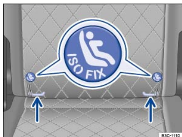
Fig. 48 On the second row seat backrests: Markings indicating the location of the LATCH/UCRA lower universal anchorages.
