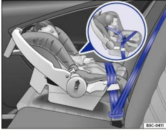
Fig. 44 Rearward-facing infant seat properly installed on the rear seat.
