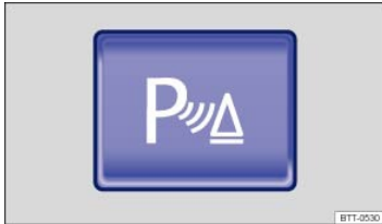
Fig. 150 In the lower center console: Button to switch the Park Distance Control system on or off (Vehicles without Area View).
