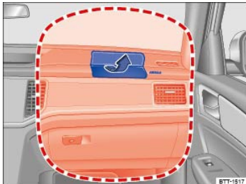
Fig. 39 Location and deployment zone of the front passenger front airbag.
