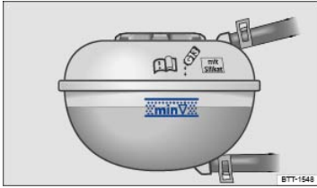
Fig. 219 Coolant expansion tank in the engine compartment.
