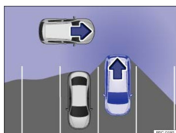
Fig. 157 Rear Traffic Alert: Monitored area around the vehicle that is backing out of a parking space.
