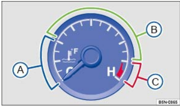
Fig. 17 Engine coolant temperature gauge in the instrument cluster: A Engine cold; B Normal temperature range; C Warning zone.
