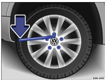
Fig. 232 Changing a wheel: Loosening the wheel bolts.
