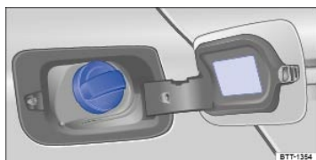
Fig. 199 Right rear side of vehicle: Fuel cap placed on the open fuel filler flap.
