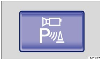
Fig. 151 In the lower center console: Button to switch the Park Distance Control system on or off (vehicles with Area View).
