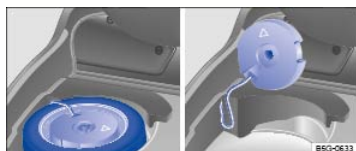
Fig. 184 Under the luggage compartment floor: Subwoofer (if equipped)
