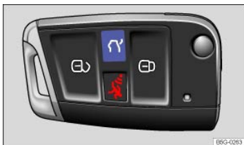
Fig. 71 On the remote control vehicle key: Button to unlock the trunk lid.
