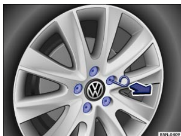
Fig. 231 Pulling cover caps off wheel bolts.
