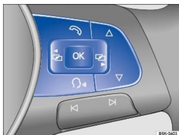
Fig. 21 Right side of the multi-function steering wheel: Controls for the menus and information in the instrument cluster display.
