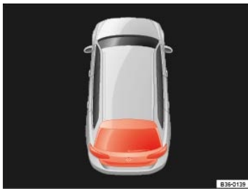
Fig. 70 In the instrument cluster display: Trunk lid open or improperly closed.
