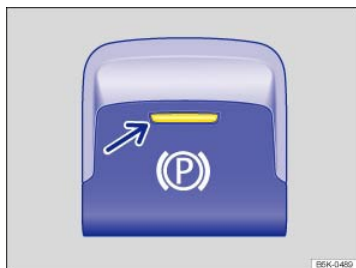
Fig. 149 In the lower center console: Electronic parking brake switch.
