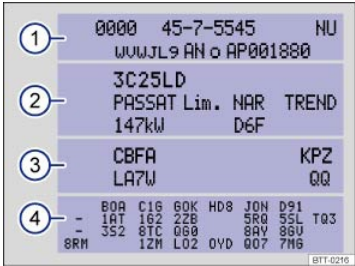
Fig. 236 Vehicle identification label: Shown in the example with engine identification code CBFA ③.
