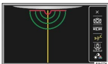
Fig. 164 Trailer support display (vehicles with a factory-installed trailer hitch).
