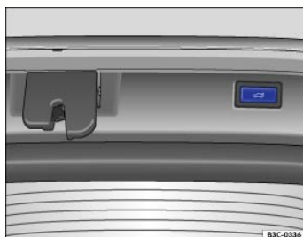
Fig. 74 Button in the open trunk lid.
