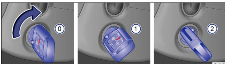
Fig. 120 In the ignition switch: Vehicle key positions for vehicles without Keyless Access.
