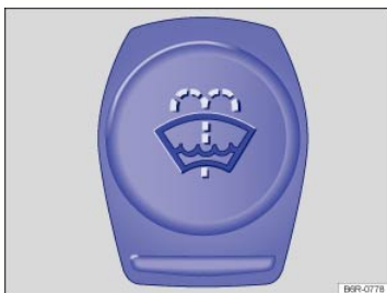
Fig. 216 In the engine compartment: Cap of the windshield washer fluid reservoir
