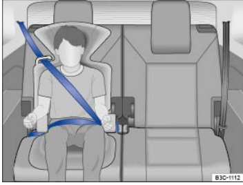
Fig. 47 Child properly restrained in a booster seat in the third row.
