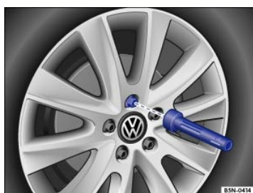
Fig. 235 Changing a wheel: Remove previously loosened wheel bolts using the screwdriver handle.
