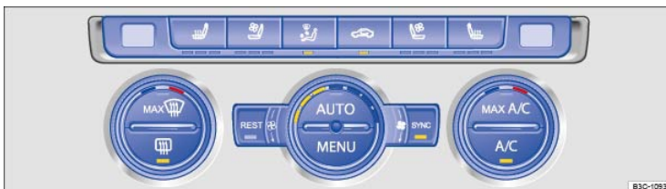
Fig. 114 In the center console: Climatronic controls.
