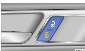
Fig. 60 In the driver and front passenger doors: Power locking button.
