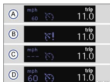
Fig. 135 In the instrument cluster display: Cruise control status indications.
