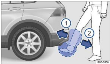
Fig. 75 Keyless Access locking and starting system: Opening the sensor-controlled trunk lid (Easy Open).
