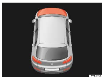
Fig. 215 In the instrument cluster display: Engine hood open or not properly closed.
