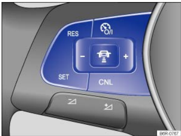
Fig. 140 Left-hand side of the multi-function steering wheel: Buttons for operating the Adaptive Cruise Control (ACC).
