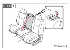
Pull the lever up and fold down the seatback.
