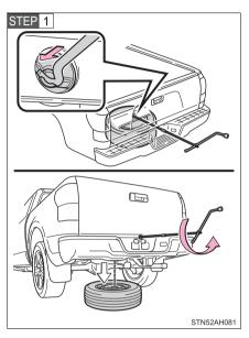
Insert the end of the jack handle extension into the lowering screw and turn it counterclockwise.
