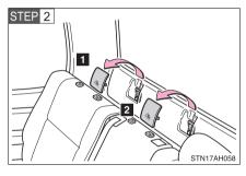
Remove the anchor bracket cover.
