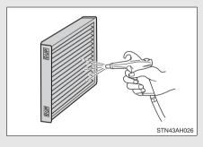
If the filter is dirty, clean by blowing compressed air through the filter from the downward side.
