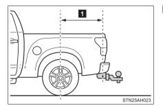
■ Hitch receiver pin hole position: 46.4 in. (1179 mm)
