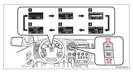
1 Zoom display of odometer and trip meters
