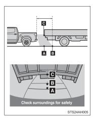
The distance that appears on the screen between three-dimensional objects (such as vehicles) and flat surfaces (such as the road) and the actual distance differ as follows.
