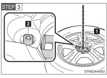
Fasten the claws of the holding bracket into the wheel holes as shown in the illustration.
