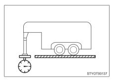
The load placed on the 5th wheel mount or the gooseneck ball.  $(\rightarrow P. 282)$
