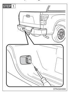
Remove the screw and light unit.
