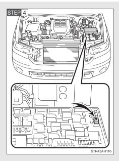
Remove the fuse with the pullout tool.
