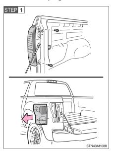
Remove the bolts and rear combination assembly.
