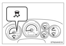
If the vehicle is in danger of slipping, or if the rear wheels (2WD models and 2WD mode on 4WD models) or all wheels (4WD mode on 4WD models) spin, the slip indicator flashes to indicate that VSC/Trailer Sway Control/TRAC/A-TRAC have been engaged.
