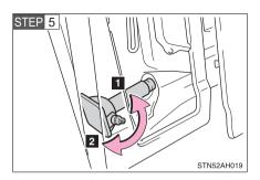
Loosen and remove the jack.
