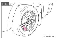
Slightly loosen the wheel nuts (one turn).
