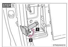
Loosen and remove the jack.
