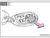
Remove the discharged transmitter battery.
