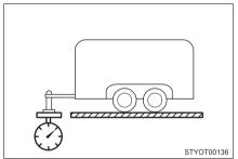
The load placed on the trailer hitch ball. ( $\rightarrow$ P. 282)
