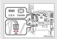
Sets the parking brake\*. (Depressing the pedal again releases the parking brake.)
