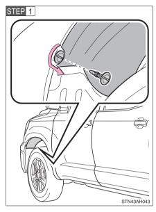
Remove the fender liner clip.
