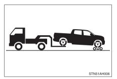
We recommend the use of a towing dolly under the front wheels.
