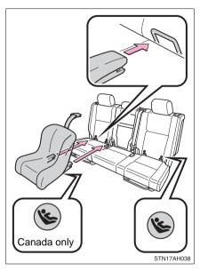
STEP 3 Widen the gap between the seat cushion and seatback slightly.
