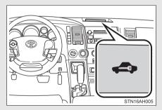
Close the doors and hood, and lock all the doors. The system will be set automatically after 30 seconds.
