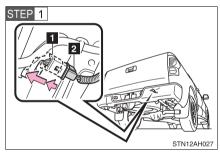
To disconnect the wire harness connectors (1 and 2), depress small plastic tab on connector 1 and pull apart from connector 2.
