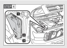
The coolant level is satisfactory if it is between the "FULL" and "LOW" line on the reservoir.
