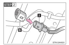
Attach the connector cover (White) to the frame wire harness connector (Gray).
