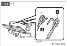
Open the tailgate to the angle where you can release the brackets on the support cables from the lugs on both sides.
