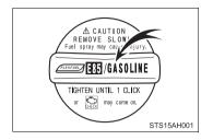
Flex-fuel vehicles can be identified by the fuel tank cap, which is marked "FLEXFUEL E85/GASOLINE".
