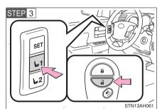
Push the "1" or "2" button and the putton on the wireless remote control at the same time for about 1 second until you hear a beep.
