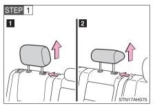
Remove the head restraint.
