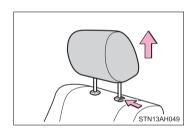
Pull the head restraint up while pushing the lock release button.
