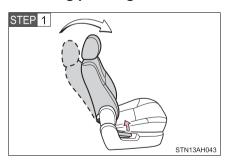
Pull the seatback angle adjusting lever and raise the seatback to its upright position.
