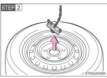
After the tire is lowered completely to the ground, remove the holding bracket.
