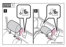
Remove the head restraint.
