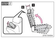
Fold down the seatback and back to the 1st lock position (most upright position) until it locks into place. Adjust the seatback to the 8th lock position.  $(\rightarrow P. 65)$
