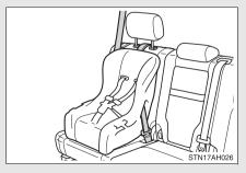
Seat belts equipped with a child restraint locking mechanism (ALR/ELR belts except driver's seat belt) (→P. 81)
