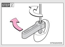
Using the wrench, tighten the antenna an additional 1/8th turn (20 to 45 degrees) to secure it in place.
