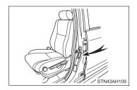
For the GAWR, see the Certification Label. For the maximum load of the tire, see the load limit at maximum cold tire inflation pressure mentioned on the sidewall of the tire. ( $\rightarrow$  P. 685)
