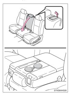
Pull the lever up and fold down the seatback.
