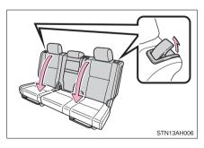
Pull the lever to unlock the seatback and fold the seatback down until it locks.
