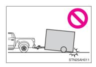
No matter which class of tow hitch applies, for a safe trailer hookup, the trailer ball setup on must be the proper height for the coupler on the trailer.
