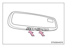
Press and hold down the 2 outside buttons for 20 seconds until the indicator flashes.
