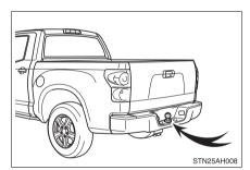
The rear bumper of your vehicle is equipped with a hole to install a trailer ball.
