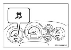
If the rear wheels spin, the slip indicator flashes to indicate that the AUTO LSD system have been controlled the spinning of the rear wheels.
