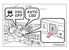
Stop the vehicle completely, and press the VSC OFF switch for more than 3 seconds, when the system is in the TRAC OFF mode.
