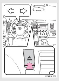
Press the switch to flash all the turn signal lights. To turn them off, push the switch once again.
