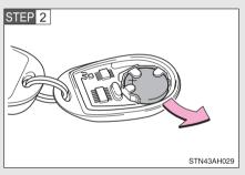
Remove the discharged transmitter battery.
