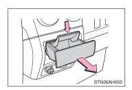
Push down on the lock spring plate and pull out.
