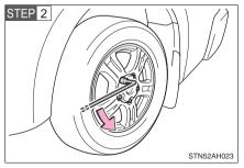
Slightly loosen the wheel nuts (one turn).
