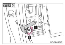
Loosen and remove the jack.
