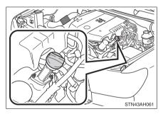
If the oil level is below or near the low level mark, add engine oil of the same type as already in the engine.
