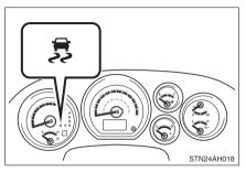
If the vehicle is in danger of slipping, or if the rear wheels (2WD models and 2WD mode on 4WD models) or all wheels (4WD mode on 4WD models) spin, the slip indicator flashes to indicate that VSC/TRAC/A-TRAC have been engaged.
