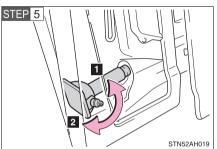
Loosen and remove the jack.
