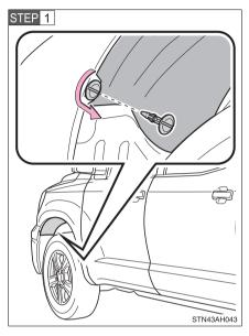
Remove the fender liner clip.
