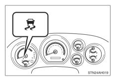
If the vehicle is in danger of slipping, or if the rear wheels (2WD models and 2WD mode on 4WD models) or all wheels (4WD mode on 4WD models) spin, the slip indicator flashes to indicate that VSC/TRAC/A-TRAC have been engaged.
