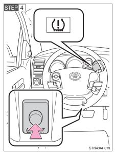
Push and hold the tire pressure warning reset switch about 3 seconds. After releasing the switch, check that the tire pressure warning light blinks slowly three times.
