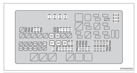
Fuse Ampere Circuit Multiport fuel injection system/ 1 A/F 15 A sequential multiport fuel injection system **HORN** 10 A Horn 2 Multiport fuel injection system/ 3 EFI NO.1 25 A sequential multiport fuel injection system 4 **IG2 MAIN** 30 A INJ, MET, IGN fuses 5 **DEICER** 20 A Front windshield wiper de-icer **TOW TAIL** 30 A Trailer lights (tail lights) 6 7 POWER NO.2 Power back windows 30 A 8 FOG 15 A Front fog lights
