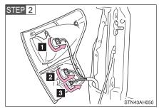
Turn the bulb bases counter-clockwise.
