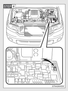
Remove the fuse with the pullout tool.
