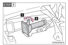
Loosen and remove the jack.
