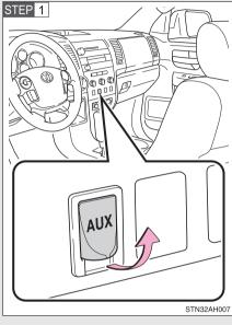
Connect the portable audio device.
