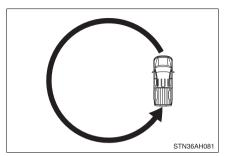
When "CAL" appears on the display, drive the vehicle at 5 mph (8 km/h) or less in a circle until a direction is displayed.
