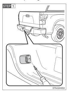
Remove the screw and light unit.
