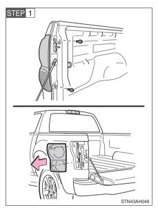
Remove the bolts and rear combination assembly.
