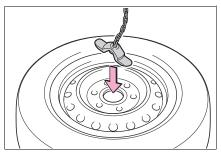
3 Check to ensure the holding bracket is centered in the wheel hub.
