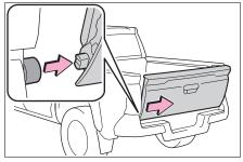
To attach the tailgate, follow the removal procedure in reverse order.
