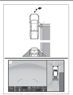
The pillar that is diagonal to the parking spot may be displayed perpendicular on the screen. Even if it seems like there will not be a collision, the pillar is diagonal, so there may be collision with the upper part of the pillar.
