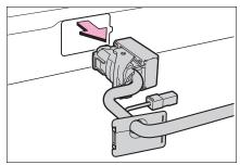
7 Install the connector cover (Type A and B) to the wire harness connector of the tailgate.
