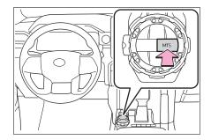
2 Select the Multi-terrain Select modes on the multi-information display while turning the mode select switch left and right.
