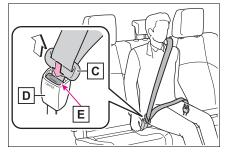
2 To release plate A, insert the mechanical key (→P.124) or plate C into the hole on buckle B.
