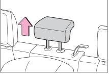
2 Place the child restraint system on the seat facing the front of the vehicle. **3** Latch the hook onto the anchor bracket.
