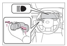
1 With the headlights on, push the lever away from you to turn on the high beams.
