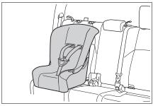
4 Run the seat belt through the child restraint system and insert the plate into the buckle. Make sure that the belt is not twisted.
