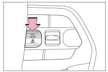
2 Using the accelerator pedal, accelerate or decelerate to the desired vehicle speed (approximately 20 mph [30 km/h] or more), and press the driving assist switch to set the set vehicle speed.
