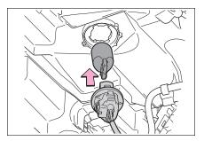
4 Install a new light bulb and turn the bulb base clockwise.
