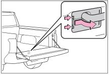
6 Pull out the wire harness from the vehicle bed.
