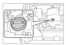
1 Remove the oil filler cap by turning it counterclockwise.
