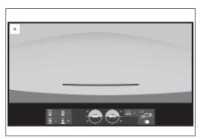
The rear view & dual side view and the wide rear displays can be switched by touching the screen.
