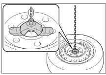
4 While raising, secure the tire, taking care that the tire goes straight up without catching on any surrounding parts, to prevent it from flying forward during a collision or sudden braking.
