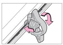
3 Slide the cleat to the closest detent in the rail system. You will feel that the locking plate snaps into a detent.
