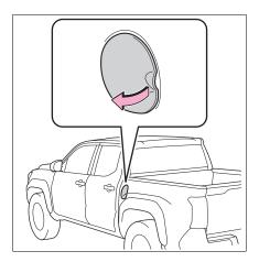
2 Turn the fuel tank cap slowly to open it and put it into the holder on the fuel filler door.
