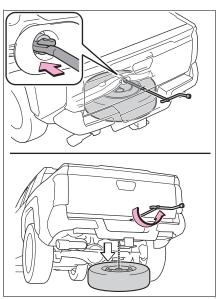
3 After the tire is lowered completely to the ground, remove the holding bracket.
