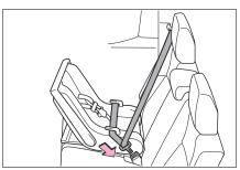
3 Fully extend the shoulder belt and allow it to retract to put it
