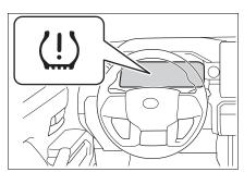
After 2 minutes, registration of a second wheel set is being performed. The tire pressure warning light will turn off and "--" will be displayed for the inflation pressure of each tire on the multi-information display.
