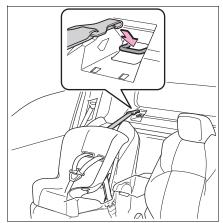
6 If the head restraint does not interfere with the child restraint system installation, install the head restraint.
