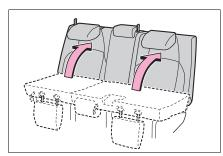
2 Returning the head restraints on the rear outboard seats to the original position. (→P.158)
