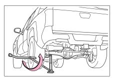
4 Securely tighten the wheel nuts two or three times in the order shown in the illustration using a wheel nut wrench. Tightening torque:
