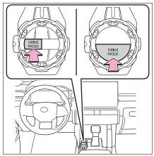
2 Select the driving modes on the multi-information display while turning the mode select switch left and right.
