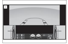
When the under vehicle terrain view and side view screens are touched, each of the display sizes can be changed.
