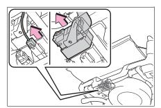
4 Install the connector cover (Type C and D) to the wire harness connector of the vehicle body frame.
