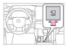
The Multi-terrain Monitor is displayed by operating □ when vehicle speed is approximately 10 mph (16 km/h) or less. If the vehicle speed exceeds approximately 10 mph (16 km/h), the Multi-terrain Monitor display is canceled.
