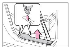
After removing the clips, pull the rear seat undercover forward in the order A, B and remove it.
