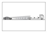
When a detectable vehicle has extremely high ground clearance
