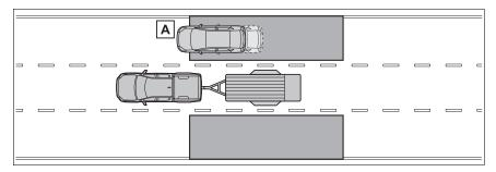
A Vehicles approaching in adjacent lanes that may not be visible using the outside rear view mirrors (the blind spots)
