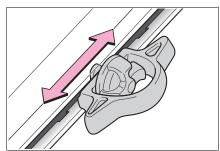
**4** Tighten the thumb wheel in a clockwise motion until the clutch mechanism ratchets.
