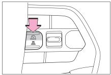
2 Using the accelerator pedal, accelerate to the desired vehicle speed (approximately 20 mph [30 km/h] or more), and press the driving assist switch to set the set vehicle speed.
