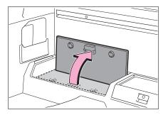
3 Unhook the tightening strap and take out the tool bag.
