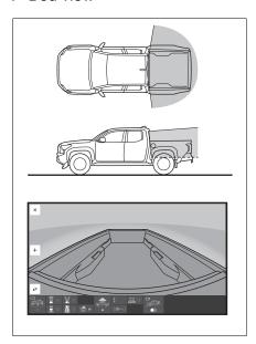
The area covered by the camera is limited. Objects which are close to either corner of the bumper or under the bumper cannot be seen on the screen.
