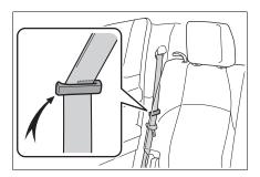
**4** Lift the seat cushion and secure the strap button **A** to the seat back.
