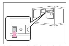
Press and hold the desired HomeLink® button (inside the vehicle) for 2 seconds and release it. Repeat this sequence (press/hold/release) up to 3 times to complete programmina. If the garage door opener motor operates when the HomeLink® button is pressed, the garage door opener motor recognizes the HomeLink® signal.
