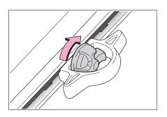
5 Check the tie-down cleat to confirm that it is locked into a detent and securely mounted to the deck rail system.
