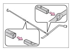
2 Insert the end of the jack handle extension into the lowering screw and turn it counterclockwise.
