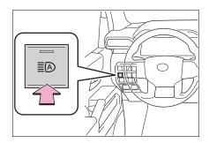
When the headlight switch lever is in the low beam position, the AHB system will be enabled and the AHB indicator will illuminate.
