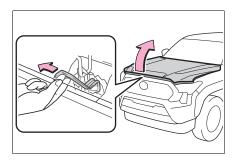
3 Hold the hood open by inserting the supporting rod into the slot or .
