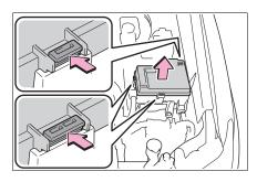
Engine compartment: type B fuse box
