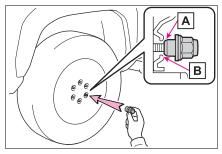
When replacing an aluminum wheel with a spare aluminum wheel, tighten the nuts until the washer of the nut A comes into loose contact with the disc wheel B.
