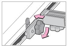
3 Slide the Thumb wheel to the closest detent in the rail system.
