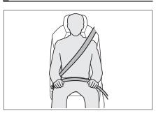
Extend the shoulder belt so that it comes fully over the shoulder, but does not come into contact with the neck or slide off the shoulder.
