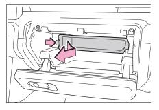
4 Unlock the filter cover (A), pull the filter cover out of the claws (B), and remove the filter cover.
