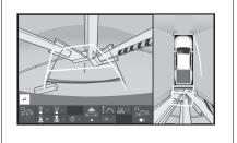
Visually check the surroundings and the area behind the vehicle. In the case shown below, the truck appears to be outside of the estimated course lines and the vehicle does not look as if it hits the truck. However, the rear body of the truck may actually cross over the estimated course lines. In reality if you back up as guided by the estimated course lines, the vehicle may hit the truck.
