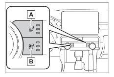
Adjust the front seat heater temperature level
