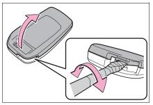
3 Remove the depleted battery.
