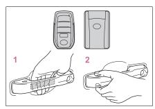
1 Grip the driver's door handle to unlock the door. Holding the driver's door handle for approximately 2 seconds unlocks all the doors. Grip front passenger door handle to unlock all the doors. \*1, 2
