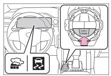
2 Turn the mode select switch left or right to select a mode on the multi-information display.
