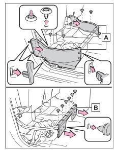
After removing the clips, lift up the near corner of the storage box.
