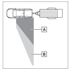
The area able to be seen changes depending on the camera angle adjustments.
