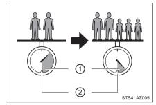
When 2 people with the combined weight of A lb. (kg) are riding in your vehicle, which has a total load capacity (vehicle capacity weight) of B lb. (kg), the available amount of cargo and luggage load capacity will be C lb. (kg) as follows:
