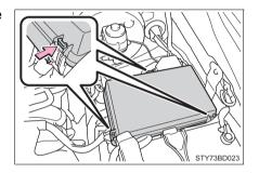
Under the instrument panel Remove the cover.
