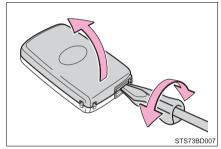
Remove the depleted battery.
