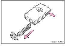
After using the mechanical key, store it in the electronic key. Carry the mechanical key together with the electronic key. If the electronic key battery is depleted or the entry function does not operate properly, you will need the mechanical key. (→P. 522)
