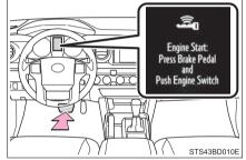
4 Press the engine switch shortly and firmly.
