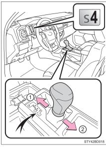
The initial shift range in S mode is set automatically to 5 or 4 according to vehicle speed. However, the initial shift range may be set to 3 if the AI-SHIFT has operated while the shift lever was in the D position.  $(\rightarrow P. 212)$
