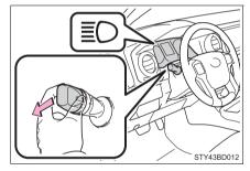
2 Press the Automatic High Beam switch.
