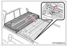
4 Secure by using the storage straps.
