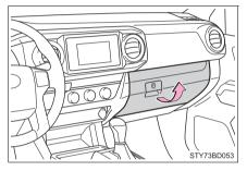
Remove the cover by sliding up and then pull the cover toward you.
