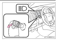
2 Press the Automatic High Beam switch.
