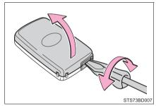
Remove the depleted battery.
