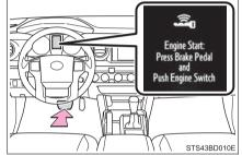
Press the engine switch shortly and firmly.
