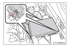
Under the instrument panel Remove the cover.
