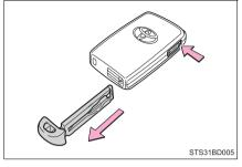
After using the mechanical key, store it in the electronic key. Carry the mechanical key together with the electronic key. If the electronic key battery is depleted or the entry function does not operate properly, you will need the mechanical key.  $(\rightarrow P. 614)$
