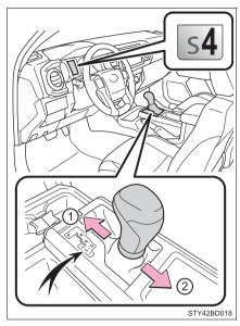
The initial shift range in S mode is set automatically to 5 or 4 according to vehicle speed. However, the initial shift range may be set to 3 if the AI-SHIFT has operated while the shift lever was in the D position.  $(\rightarrow P. 204)$
