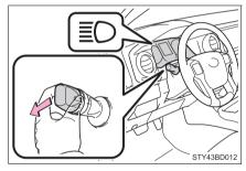
2 Press the Automatic High Beam switch.
