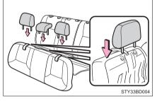
Center head restraint: The front of the head restraint facing forward.
