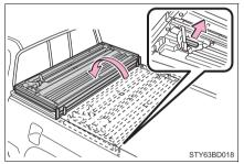
4 Secure by using the storage straps.
