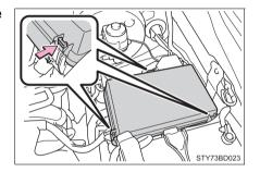
Under the instrument panel Remove the cover.
