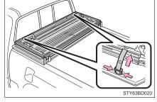
Close the tonneau cover and push down on the top surface (latch position) until it clicks.
