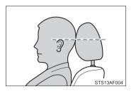
Adjusting the rear center seat head restraint (Double Cab models only)
