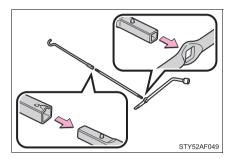
2 Insert the end of the jack handle extension into the lowering screw and turn it counterclockwise.
