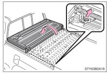
4 Secure by using the storage straps.
