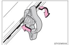
3 Slide the cleat to the closest detent in the rail system. You will feel that the locking plate snaps into a detent.
