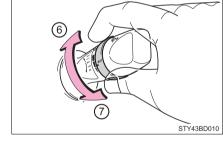
Washer/wiper dual operation Wipers will automatically operate a couple of times after the washer squirts.
