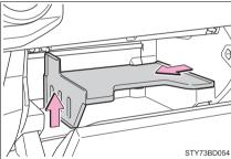
A Remove the cover by sliding up and then pull the cover toward you.
