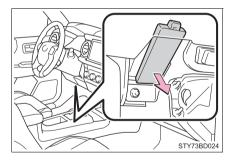
Remove the fuse with the pullout tool.
