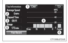
Average fuel consumption for the past 15 minutes is divided by color into past averages and averages attained since the engine switch was last turned to the "ON" position (vehicles without a smart key system) or IGNITION ON mode (vehicles with a smart key system). Use the displayed average fuel consumption as a reference.
