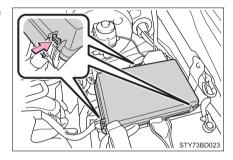
Under the instrument panel Remove the cover.
