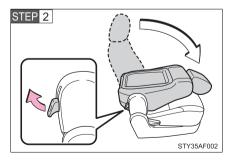
Pull the seatback folding lever and fold the seatback down.
