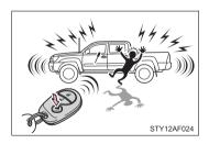
When will is pushed for longer than about 1 second, an alarm will sound for about 60 seconds and the vehicle lights will flash to deter any person from trying to break into or damage your vehicle.
