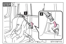
■ Route the top tether strap through the routing device as shown in the illustration.
