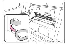
Cargo net hooks are designed to hang the factory-supplied cargo net.
