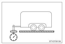
The load placed on the trailer hitch ball. ( $\rightarrow$ P. 221)
