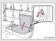
Push the bottom cushion down while pulling the lever until the bottom cushion locks into the seat position.
