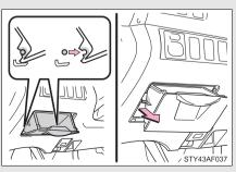
2.Pull up the box and disengage the claws. Remove the stoppers from the cutouts and remove the box. STEP 3 After a system failure, see "Fuse layout and amperage ratings" (→P. 447) for details about which fuse to check.
