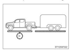
The maximum allowable gross vehicle weight. The gross vehicle weight is the total weight of the vehicle. When towing a trailer, it is the sum of the vehicle weight (including the occupants, cargo and any optional equipment installed on the vehicle) and the tongue weight.
