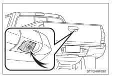
The camera for the rear view monitor system is located as shown in the illustration.
