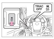
Press and hold the VSC OFF switch for more than 3 seconds while the vehicle is stopped to turn off TRAC, VSC and Trailer Sway Control.
