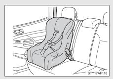
Seat belts equipped with a child restraint locking mechanism (ALR/ELR belts except driver's seat belt) (→P. 57)
