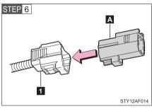
Attach the connector cover (Gray) to the tailgate wire harness connector (White).
