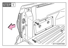
Remove the bolts and rear combination assembly.
