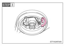
Release the bulb retaining spring.
