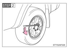
Slightly loosen the wheel nuts (one turn).
