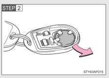
Remove the discharged transmitter battery.
