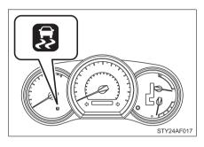
The slip indicator will flash while the VSC/Trailer Sway Control/TRAC/hill-start assist control systems are operating.
