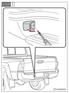
Remove the screw and light unit.
