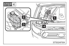
The coolant level is satisfactory if the reservoir level is between the "FULL" and "LOW" lines on the reservoir.
