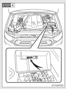
Remove the fuse with the pullout tool.
