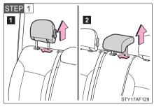
Remove the head restraint.
