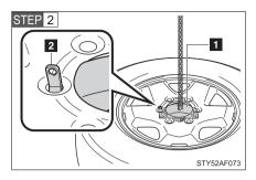
4WD models only: Fasten the claws of the holding bracket into the wheel holes as shown in the illustration.
