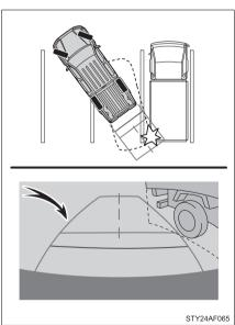
Visually check the surroundings and the area behind the vehicle. In the case shown below, the truck appears to be outside of the vehicle width guide lines and the vehicle does not look as if it hits the truck. However, the rear body of the truck may actually cross over the vehicle width guide lines. In reality if you back up as guided by the vehicle width guide lines, the vehicle may hit the truck.
