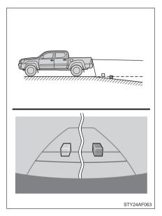
The distance guide lines will appear to be further from the vehicle than the actual distance. Because of this, objects will appear to be closer than they actually are. In the same way, there will be a margin of error between the guidelines and the actual distance/course on the road.
