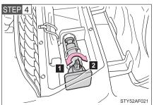
Loosen and remove the jack.
