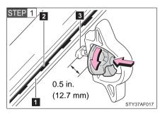
Loosen the thumb wheel in a counterclockwise motion, and depress the wheel so that the locking plate maintains 0.5 in. (12.7 mm) gap.
