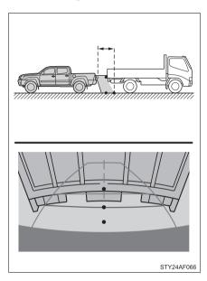
Visually check the surroundings and the area behind the vehicle. On the screen, it appears that a truck is parked at point 2. However, in reality if you back up to point 1, you will hit the truck. On the screen, it appears that 1 is closest and 3 is furthest away. However, in reality, the distance to 1 and 3 is the same, and 2 is farther than 1 and 3.
