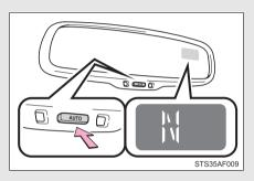
To turn the compass on or off, press the button.
