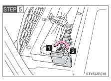
Loosen and remove the jack.
