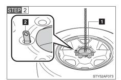
4WD models only: Fasten the claws of the holding bracket into the wheel holes as shown in the illustration.
