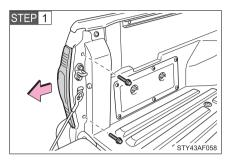
Remove the bolts and rear combination assembly.
