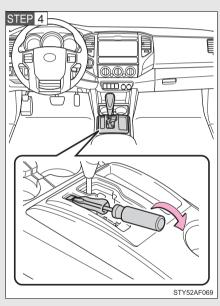
Pry the cover up with a flathead screwdriver or equivalent.
