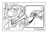
Your vehicle is equipped with a service connector for the trailer brake controller as shown.
