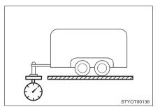
The load placed on the trailer hitch ball.  $(\rightarrow P. 232)$
