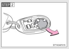
Remove the discharged transmitter battery.
