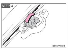
Tighten the thumb wheel in a clockwise motion until the clutch mechanism ratchets.
