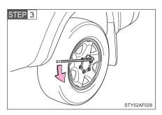
Slightly loosen the wheel nuts (one turn).
