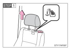
Remove the head restraint.
