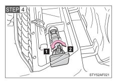
Loosen and remove the jack.
