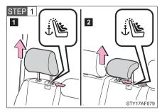
Remove the head restraint.
