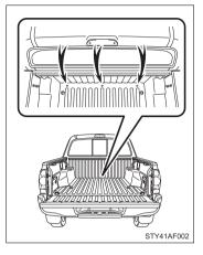
Clean the drainage hole of the deck regularly.
