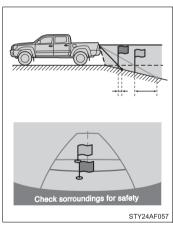
When the grade behind the vehicle slopes down sharply, objects appear to be closer than they actually are.
