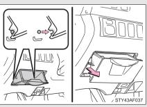
2.Pull up the box and disengage the claws. Remove the stoppers from the cutouts and remove the box. STEP 3 After a system failure, see "Fuse layout and amperage ratings" (→P. 477) for details about which fuse to check.
