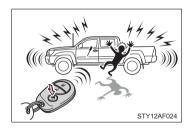
When will is pushed for longer than about 1 second, an alarm will sound for about 60 seconds and the vehicle lights will flash to deter any person from trying to break into or damage your vehicle.
