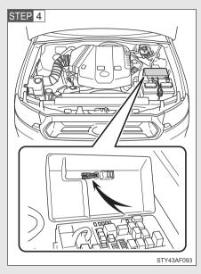
Remove the fuse with the pullout tool.
