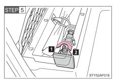
Loosen and remove the jack.
