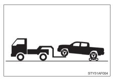
Vehicles with an automatic transmission: Use a towing dolly under the rear wheels.
