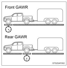
The maximum allowable gross axle weight. The gross axle weight is the load placed on each axle (front and rear).
