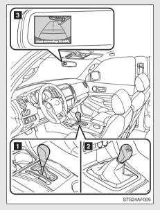
The rear view image is displayed on the inside rear view mirror
