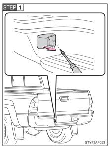
Remove the screw and light unit.
