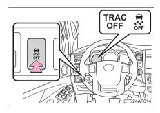
Press and hold the VSC OFF switch for more than 3 seconds while the vehicle is stopped to turn off TRAC, VSC and Trailer Sway Control.
