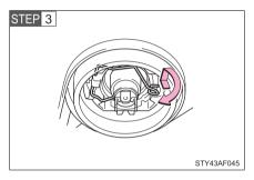
Release the bulb retaining spring.
