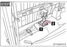
Loosen and remove the jack.
