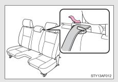
Make sure the shoulder belt pass through the guide when using the center seat belt.
