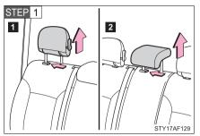
Remove the head restraint.
