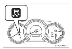
If the vehicle is in danger of slipping or rolling backward when starting on an incline, or if any of the drive wheels spins, the slip indicator light flashes to indicate that the VSC/Trailer Sway Control/TRAC/hill-start assist control systems are operating.
