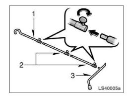
Put a wheel nut wrench, jack handle extension and jack handle end together as shown in the illustration.
