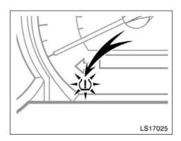
If the tire pressure warning light does not blink slowly three times when you push and hold the tire pressure warning reset switch, initialization has failed and the tire pressure warning system may not work properly. In this case, initialize the system again. If initialization cannot be performed, have the system checked at your Toyota dealer.
