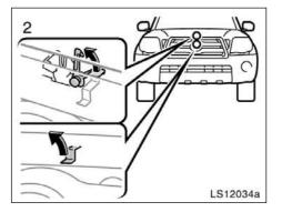
2. Pull up the auxiliary catch lever inside the engine compartment, and lift the hood. (by inserting your finger through either the opening between the hood and grille or through the grille.)
