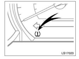
The tire pressure warning light comes on when the engine switch is turned to the "ON" position and goes off after a few seconds. This means the tire pressure warning system is operating properly. If the tire inflation pressure becomes low, the light comes on again. In this case, adjusting the tire inflation pressure will turn off the light after a few minutes. If the light comes on after blinking for 1 minute, the tire pressure warning system is not working properly.
