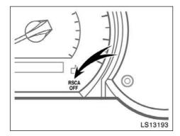
• Make sure the "RSCA OFF" indicator light is off. The curtain shield airbags will not inflate in a vehicle rollover if this indicator light is on and you may be killed or seriously injured. For details, see "Roll sensing of curtain shield airbags off switch" on page 92 in this Section.
