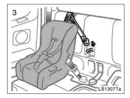
3. Latch the hook onto the rear lower anchor bracket and tighten the top strap.
