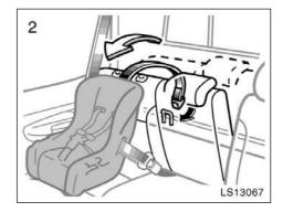
Pull the seatback release strap and swing the seatback forward slightly, then latch the hook onto the anchor bracket.
