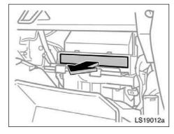
4. Remove the filter from the filter outlet. Inspect the filter on the surface.
