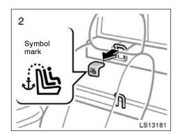
Lightly push down on the top surface of the routing device cover with the symbol mark shown in the illustration, then pull it forward to remove.
