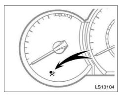
This indicator comes on when the engine switch is turned to the "ON" position. It goes off after about 6 seconds. This means the SRS airbags are operating properly.
