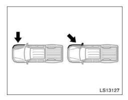
The SRS side airbags may not activate if the vehicle is subjected to a collision from the side at certain angles, or a collision to the side of the vehicle body other than the passenger compartment as shown in the illustration.
