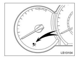
This indicator comes on when the engine switch is turned to the "ON" position. It goes off after about 6 seconds. This means the seat belt pretensioners are operating properly.
