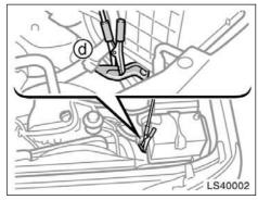
Connecting point for 2.7 L 4-cylinder (2TR-FE) engine
