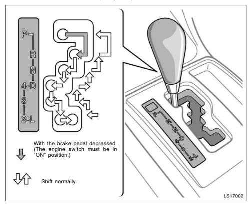
Your automatic transmission has a shift lock system to minimize the possibility of incorrect operation. This means you can only shift out of "P" position when the brake pedal is depressed (with the engine switch in "ON" position).
