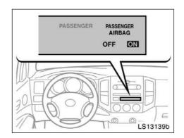
The front passenger occupant classification indicator light indicates the actuation of the front passenger airbag, side airbag on the front passenger seat and front passenger seat belt pretensioner.
