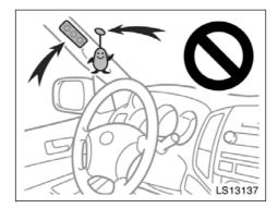
• Do not attach a microphone or any other device or object around the area where the curtain shield airbag activates such as on the windshield glass, side door glass, front and rear pillars, roof side rail and assist grips. When the curtain shield airbags inflate, the microphone or other device or object will be thrown away with great force or the curtain shield airbags may not activate correctly, resulting in death or serious injury.
