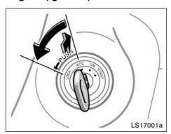
"START"—Starter motor on. The engine switch will return to the "ON" position when released.
