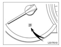
If there is any abnormality in the system, the "VSC OFF" warning light will flash. When the "DAC" switch is pushed, the downhill assist control system indicator light also flash.
