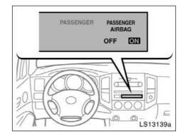
The front passenger occupant classification indicator light indicates the actuation of the front passenger airbag and front passenger seat belt pretensioner.
