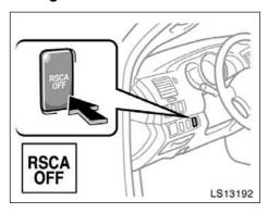
The roll sensing of curtain shield airbags off switch ("RSCA OFF" switch) can turn off the curtain shield airbags and seat belt pretensioners in a vehicle rollover. This switch should only be used if inflation is not desired (such as extreme off-road driving).
