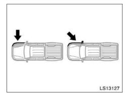
The SRS curtain shield airbags may not activate if the vehicle is subjected to a collision from the side at certain angles, or a collision to the side of the vehicle body other than the passenger compartment as shown in the illustration.
