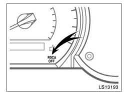
The seat belt pretensioners will not operate in a vehicle rollover if the "RSCA OFF" indicator light is on. For details, see "Roll sensing of curtain shield airbags off switch" on page 92 in this Section.
