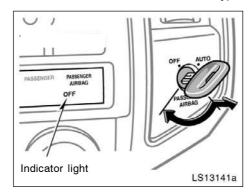
This off switch is designed to disable the front passenger airbag in order to allow usage, if necessary, of a member of a passenger risk group identified in TABLE 1 is occupying the front passenger seating position. (For details, see "SRS driver airbag and front passenger airbag" on page 53 in this Section.)
