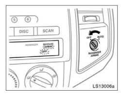
When you install a rear-facing child restraint system which belongs to a passenger risk group on the front passenger seat, turn the passenger airbag off switch counterclockwise to the "OFF" position and remove the key. (For details, see "SRS driver airbag and front passenger airbag" on page 53 in this Section.)
