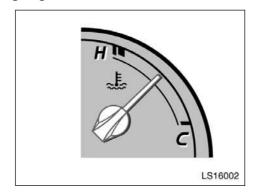
The gauge indicates the engine coolant temperature when the engine switch is on. The engine operating temperature will vary with changes in weather and engine load.
