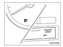
The SRS warning light and the passenger airbag on-off indicator light will indicate "OFF" if there is a malfunction in the passenger airbag off switch.
