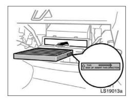
When installing the filter in the filter outlet, follow the instructions indicated on the label.
