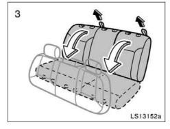
3. Fold down the seatback by pulling the lock release strap.
