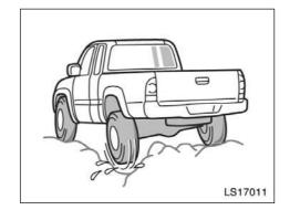
The rear differential lock system is provided for use only when wheel spinning occurs in a ditch or on a slippery or ragged surface.
