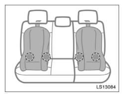
Lower anchorages for Child Restraint Systems equipped with hook or buckle type attachments are installed in the rear seat.
