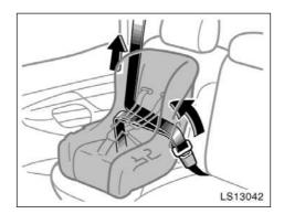
While pressing the convertible seat firmly against the seat cushion and seatback, let the shoulder belt retract as far as it will go to hold the convertible seat securely.
