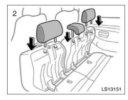
Attach the head restraints to the holders located on the back sides of the bottom cushions.
