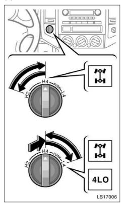
Use the front drive control switch knob to select the following transfer modes.
