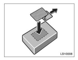
Remove the paper strip covering the adhesive on back side of square and adhere the square to back side of the transmitter near the center.
