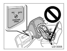
Never install a rear-facing child restraint system on the front seat with the passenger airbag off switch in the "AUTO" position. In the event of an accident, the force of the rapid inflation of the front passenger airbag can cause death or serious injury to the child if the rear-facing child restraint system is installed on the front passenger seat.
