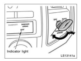
The passenger airbag system is equipped with a off switch and indicator light. Turning the passenger airbag off switch clockwise to the "AUTO" position makes the front passenger airbag system operational. To disable the front passenger airbag system, turn the off switch counterclockwise to the "OFF" position and remove the key. The "OFF" indicator light will come on when the front passenger airbag system has been disabled.
