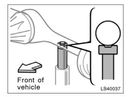
After making sure that no one is in the vehicle, as the jack touches the vehicle and begins to lift, double-check that it is properly positioned.
