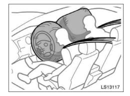
The SRS (Supplemental Restraint System) front airbags are designed to provide further protection for the driver and right front passenger (regular cab models with bench seat) or front passenger (double cab models) in addition to the primary safety protection provided by the seat belts.
