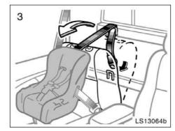
3. Pull the seatback release lever and swing the seatback forward slightly.
