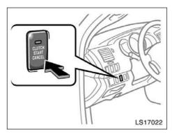
Never use the switch for normal engine starting. Be sure to follow the starting procedure instructed in "How to start the engine" on page 304 in Section 3.
