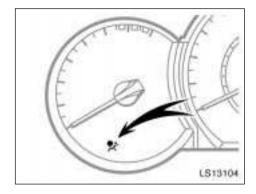
This indicator comes on when the ignition key is turned to the "ON" position. It goes off after about 6 seconds. This means the SRS front airbags are operating properly.
