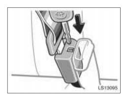
To release the concave end tab, insert the key into the hole on buckle 1 (with light gray buckle-release button) and allow the belt to retract.
