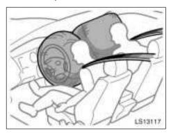
The SRS (Supplemental Restraint System) front airbags are designed to provide further protection for the driver and right front passenger (regular cab models with bench seat) or front passenger (double cab models) in addition to the primary safety protection provided by the seat belts.
