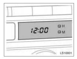
To reset the hour: Push the "H" button. To reset the minutes: Push the "M" button.
