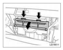
3. Push down on the tabs and open the filter door.
