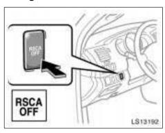
The roll sensing of curtain shield airbags off switch ("RSCA OFF" switch) can turn off the curtain shield airbags and seat belt pretensioners in a vehicle rollover. This switch should only be used if inflation is not desired (such as extreme off-road driving).
