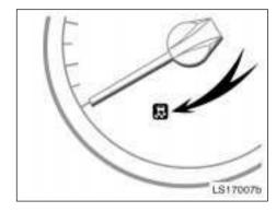
With the vehicle traveling at a speed of 25 km/h (15 mph) or less, release your foot from the accelerator or brake pedal to activate the system. The vehicle will descend the hill at a low speed. While the system is operating, the slip indicator light on the instrument panel will flash and the stop lights and high mounted stoplight will be lit.
