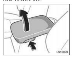
To use the rear console box, raise the console box lid while pushing the lock release button.
