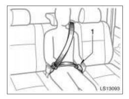
The center seat belt of the bench seat is a 3-point type restraint with 2 buckles. Both seat belt buckles must be correctly located and securely latched for proper operation.
