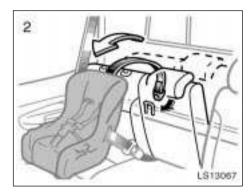
Pull the seatback release strap and swing the seatback forward slightly, then latch the hook onto the anchor bracket.
