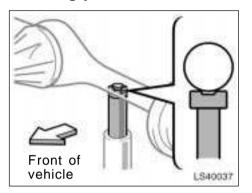
6. After making sure that no one is in the vehicle, as the jack touches the vehicle and begins to lift, double-check that it is properly positioned.
