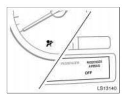
The SRS warning light and the passenger airbag on-off indicator light will indicate "OFF" if there is a malfunction in the passenger airbag off switch.
