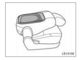
You should use the seatback as a temporary table only when the vehicle is stopped.
