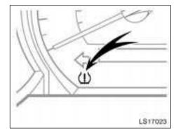
The tire pressure warning light comes on when the ignition key is turned to the "ON" position and goes off after a few seconds. This means the tire pressure warning light is operating properly. If the tire inflation pressure becomes low, the light comes on again. In this case, adjusting the tire inflation pressure will turn off the light after a few minutes. If the light blinks (comes on after blinking for 1 minute), the tire pressure warning system is not working properly.
