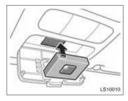
Place the transmitter with fastener square facing inside of box into the box. Make sure the transmitter button is located above button pins.
