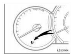
This indicator comes on when the ignition key is turned to the "ON" position. It goes off after about 6 seconds. This means the SRS airbags are operating properly.
