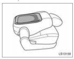
You should use the front passenger's seatback as a temporary table only when the vehicle is stopped.
