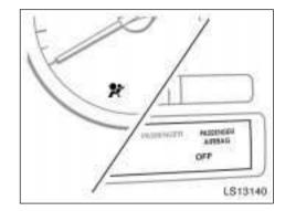
The SRS warning light will come on and the front passenger occupant classification indicator light will indicate "OFF" if there is a malfunction in the front passenger occupant classification system. Contact your Toyota dealer as soon as possible.
