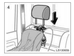
Fix the child restraint system with the seat belt and tighten the top strap.
