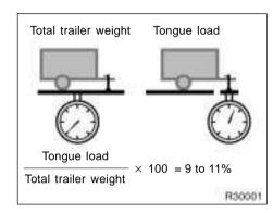
• The trailer cargo load should be distributed so that the tongue load is 9 to 11% of the total trailer weight, not exceeding the maximum load of the following.
