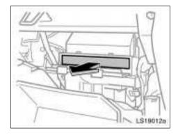
Remove the filter from the filter outlet. Inspect the filter on the surface.
