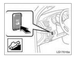
Push the "DAC" switch to turn the system on. The downhill assist control system indicator light on the instrument panel will come on.
