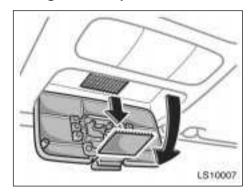
The box is designed to store a garage door opener transmitter.
