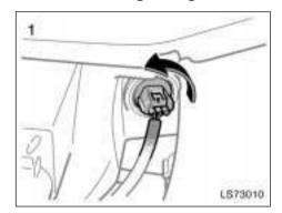
3. Install the bulb base into the mounting hole by turning it clockwise.
