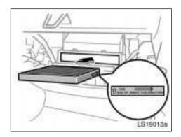
When installing the filter in the filter outlet, follow the instructions indicated on the label.
