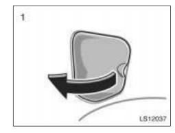
To open the fuel filler door, pull the door toward out as shown.
