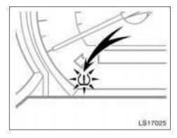
IF THE TIRE PRESSURE WARNING LIGHT BLINKS (COMES ON AFTER BLINKING FOR 1 MINUTE)...
