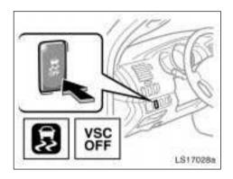
When getting the vehicle out of mud or newly fallen snow, etc., turn off the vehicle stability control system. This system that controls engine performance interferes with the process of freeing rear wheels (two-wheel drive models) or 4 wheels (four-wheel drive models).
