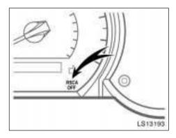
The seat belt pretensioners will not operate in a vehicle rollover if the "RSCA OFF" indicator light is on. For details, see "Roll sensing of curtain shield airbags off switch" on page 94 in this Section.
