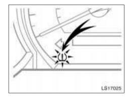
If the tire pressure warning light does not blink slowly three times when you push and hold the reset switch, initialization has failed and the tire pressure warning system may not work properly. In this case, initialize the system again. If initialization cannot be performed, have the system checked at your Toyota dealer.
