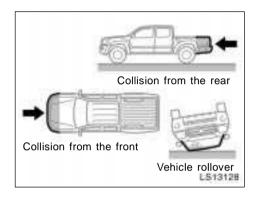
The SRS side airbags are not generally designed to inflate if the vehicle is involved in a front or rear collision, if it rolls over, or if it is involved in a low-speed side collision.
