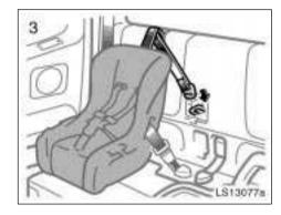
3. Latch the hook onto the rear lower anchor bracket and tighten the top strap.
