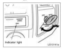
This off switch is designed to disable the front passenger airbag in order to allow usage, if necessary, of a member of a passenger risk group identified in TABLE 1 is occupying the front passenger seating position. (For details, see "SRS driver airbag and front passenger airbag" on page 55 in this Section.)
