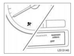
The SRS warning light will come on and the front passenger occupant classification indicator light will indicate "OFF" if there is a malfunction in the front passenger occupant classification system. Contact your Toyota dealer as soon as possible.
