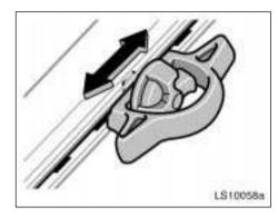
Slide the cleat to the closest detent in the rail system. You will feel that the locking plate snaps into a detent.
