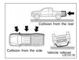
The SRS front airbags are not generally designed to inflate if the vehicle is involved in a side or rear collision, if it rolls over, or if it is involved in a low-speed frontal collision. But, whenever a collision of any type causes sufficient forward deceleration of the vehicle, deployment of the SRS front airbags may occur.
