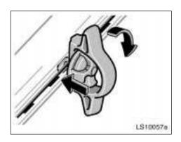
Insert the locking plate into the deck rail, rotate the tie-down cleat 90°, and release the thumb wheel.
