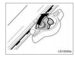
Tighten the thumb wheel in a clockwise motion until the clutch mechanism ratchets.
