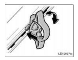
2. Insert the locking plate into the deck rail, rotate the tie-down cleat  $90^{\circ}$ , and release the thumb wheel.
