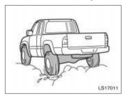
The rear differential lock system is provided for use only when wheel spinning occurs in a ditch or on a slippery or ragged surface.
