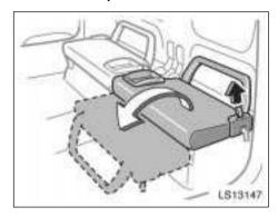
To flip over the bottom cushion, pull the lock release strap.
