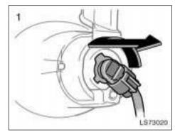
1. Turn the bulb base counterclockwise and remove it.
