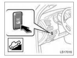
Push the "DAC" switch to turn the system on. The downhill assist control system indicator light on the instrument panel will come on.
