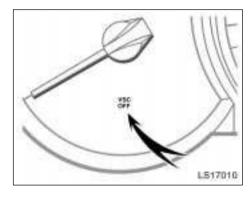
The vehicle stability control system automatically turns off, and the "VSC OFF" indicator light is illuminated, when either one of the following conditions applies:
