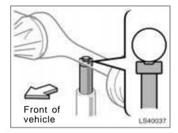
6. After making sure that no one is in the vehicle, as the jack touches the vehicle and begins to fit, double-check that it is properly positioned.
