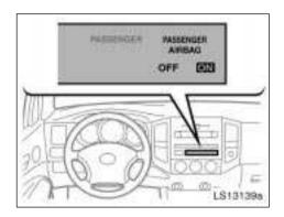
The front passenger occupant classification indicator light indicates the actuation of the front passenger airbag and side airbag on the front passenger seat.
