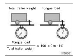
However, if towing with a fifth wheel trailer, the cargo load must be distributed so that the tongue load is 19 to 21% of the total trailer weight. Never load the trailer with more weight in the back than in the front. About 60% of the trailer load should be in the front half of the trailer and the remaining 40% in the rear.
