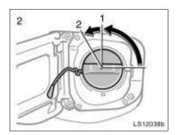
To remove the fuel tank cap, turn the cap counterclockwise by 90 degrees (to the pressure point 1), and then turn it an additional 30 degrees (to point 2). Pause slightly before removing it.
