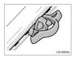
Check the tie-down cleat to confirm that it is locked into a detent and securely mounted to the deck rail system.
