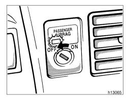
Only when you put a rear-facing child restraint system on the front seat unavoidably, turn the passenger airbag switch to the "OFF" position.
