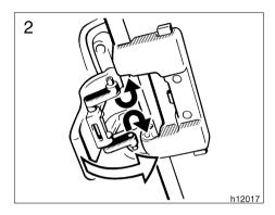
2. Press in the retaining spring arms and insert them into the holes. Then push the handle up with the palm of your hand and lock the roof.
