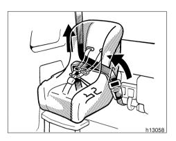
While pressing the convertible seat firmly against the seat cushion and seatback, let the shoulder belt retract as far as it will go to hold the convertible seat securely.
