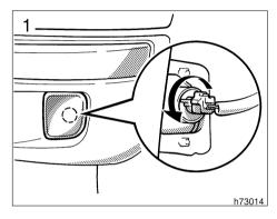
Rear turn signal, stop and tail, and back-up lights
