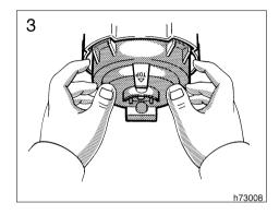
3. Install the rubber cover with the "TOP" mark upward and snuggle on the boss. Then insert the connector.
