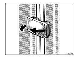
To unlock the rear window, pull the left end of the latch handle toward you and disengage the right end from the catch.
