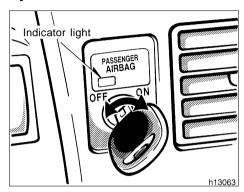
This system is designed to disable the passenger airbag in order to allow usage, if necessary, of a rear-facing child restraint system in the front seat. Disable the passenger airbag only when you put a rear facing child restraint system on the front seat unavoidably. Switch the system as follows:
