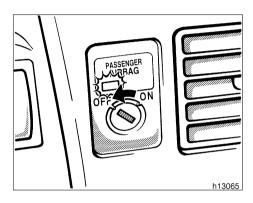
Only when you put a rear-facing child restraint system on the front seat unavoidably, turn the passenger airbag switch to the "OFF" position.
