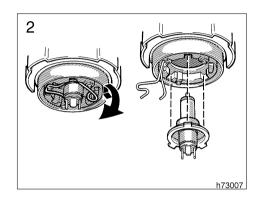
Release the bulb retaining spring and remove the bulb. Install a new bulb and the bulb retaining spring.
