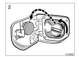
To open the fuel filler door, insert the key and turn it counterclockwise.
