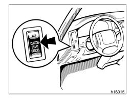
To crank the engine without depressing the clutch pedal, push the switch with the ignition on.
