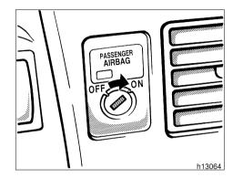
passenger airbag system is equipped with a cutoff switch and indicator light. Turning the passenger airbag switch to the "ON" position makes the passenger airbag system operational. Turning the passenger airbag switch to the "OFF" position disables the passenger airbag system. The indicator light on the passenger airbag switch will come on when the passenger airbag system has been disabled.
