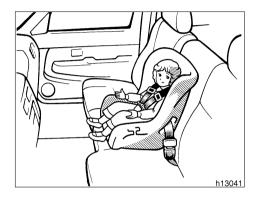
(B) CONVERTIBLE SEAT INSTALLATION A convertible seat is used in forward-facing and rear-facing position depending on the child's age and size. When installing, follow the manufacturer's instructions about the applicable child's age and size as well as direction for installing of a child restraint system.
