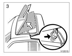
3. Push back the auxiliary catch to release it from the hook. Then lift the moon roof panel and pull it out.
