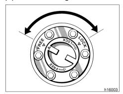
To engage the free-wheeling hubs, turn the hubs to "LOCK". To disengage, turn the hubs to "FREE".
