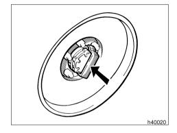
On steel wheel ornaments for free-wheeling hubs, place the wheel ornament replacer over the opening and tap on the replacer to snap the ornament into place. Be careful not to slip off the replacer.
