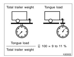
The trailer cargo load should be distributed so that the tongue load is 9 to 11 % of the total trailer weight, not exceeding 158 kg (350 lb.).
