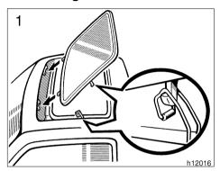
Insert the flat hinges of the moon roof panel into the cutouts on the body. Then slowly lower it while holding the roof with your hands.
