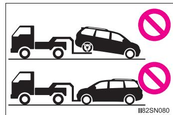
AWD models: Be sure to transport the vehicle with all four wheels raised off the ground. If the vehicle is towed with the tires contacting the ground, the drivetrain or related parts may be damaged, the vehicle may fly off the truck.
