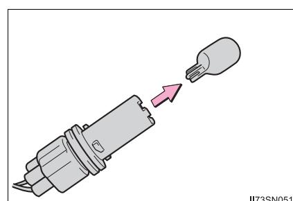
**■ Rear turn signal lights (vehicles with LED type stop/tail lights)**
