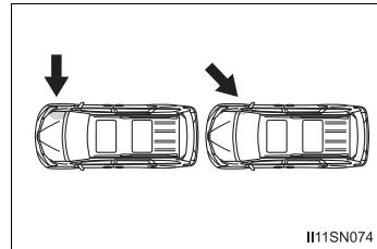
The SRS side airbags do not generally inflate if the vehicle is involved in a rear collision, if it rolls over, or if it is involved in a low-speed side collision or low-speed frontal collision.
