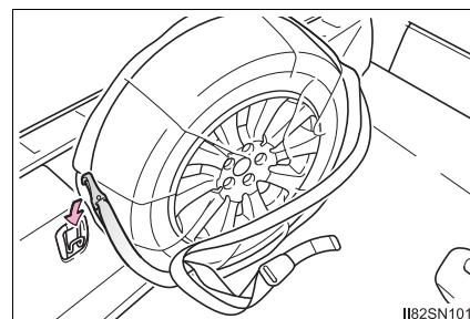
5 Pull strap to tighten and secure tire.
