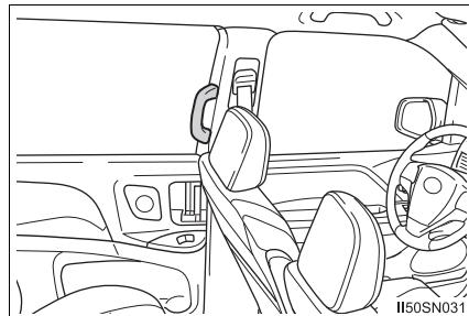
An assist grip installed on the ceiling can be used to support your body while sitting on the seat.
