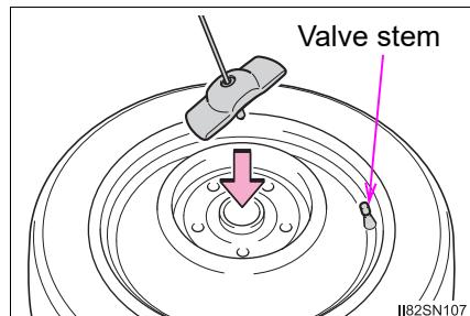
2 Turn the jack handle clockwise to raise the tire until the tire is in the correct position as the jack handle skips.
