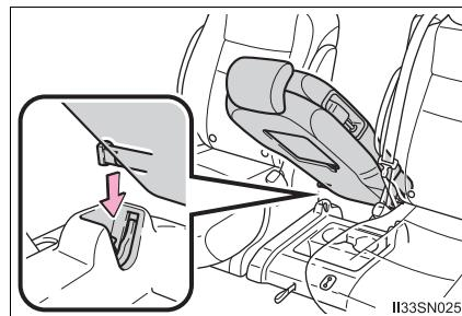
2 Unfold the cushion leg and push down on the seat to engage the front lock.
