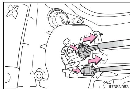
3 Turn the bulb base counter-clockwise.
