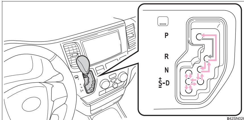
While the engine switch is in the "ON" position (vehicles without a smart key system) or IGNITION ON mode (vehicles with a smart key system), move the shift lever with the brake pedal depressed.
