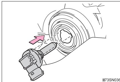
**5** Turn and secure the bulb base.
