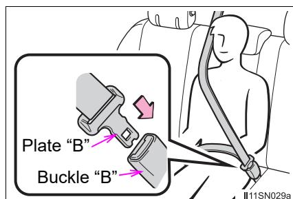
**Releasing and stowing the seat belt (for the third center seat)**
