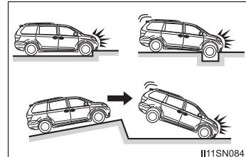
The SRS curtain shield airbags may also deploy under the situations shown in the illustration.
