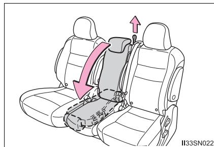
2 Pull the lock release strap under the seat to remove the seat.
