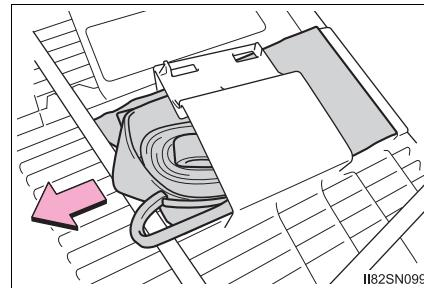
2 Place tire standing up in rear tub, after putting the tire in the tire bag.
