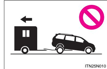
AWD models: Never tow this vehicle with any of the wheels on the ground. This may cause serious damage to the transaxle and Active Torque Control 4WD system.
