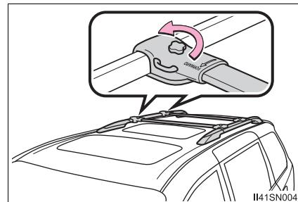
2 Slide the cross rails to the appropriate position for loading luggage and turn the knobs clockwise to tighten the cross rails securely.
