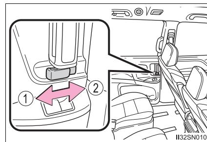
**Opening/closing the sliding door****◆ Sliding door handle****Open/close**
