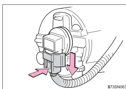
3 Turn the bulb base counter-clockwise.
