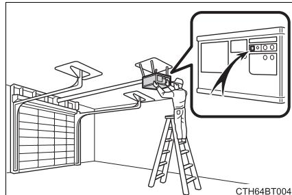
2 Press and release the “Learn” or “Smart” button. Perform 3 within 30 seconds after performing 2.
