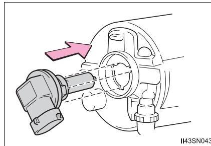
**5** Turn clockwise and secure the bulb base.
