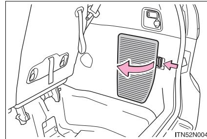
2 Remove the adapter socket.
