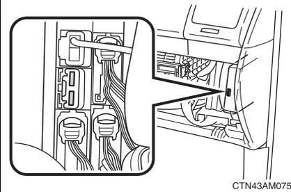
**STEP 3** After a system failure, see “Fuse layout and amperage ratings” (→P. 478) for details about which fuse to check.
