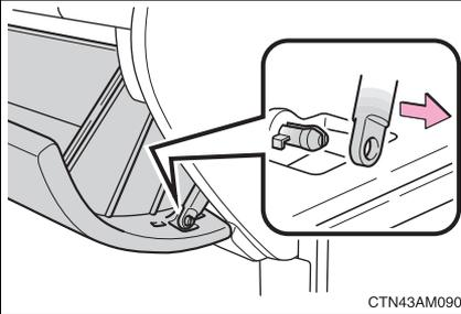
1. Open the glove box. Slide off the damper.
