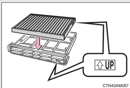
Install a new filter to the filter case.
