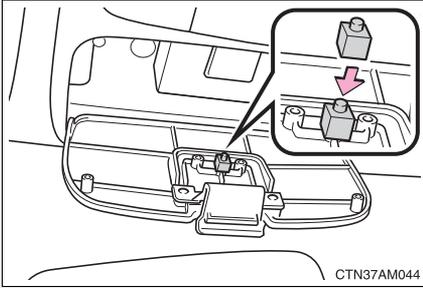
Check to see if the spacer is on the correct pin.
