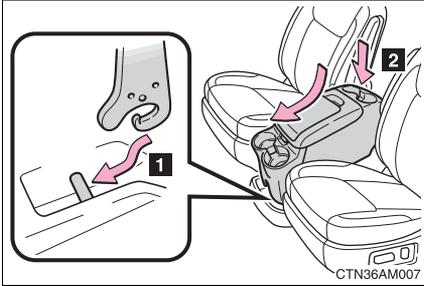
**1** Install the front hook in the front striker of the console box installation base.
