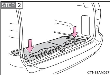
Push the seat against the floor and make sure it is locked securely.
