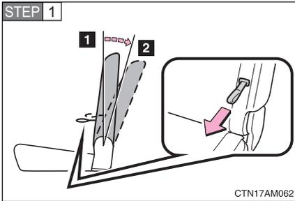
Fold the seatback while pulling the lever. Return the seatback and secure it at the 1st lock position (most upright position). Adjust the seatback to the 11th lock position. (→P. 61)
