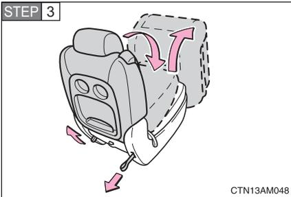
Center seat: Fold down the seatback while pulling the seatback angle adjustment strap.
