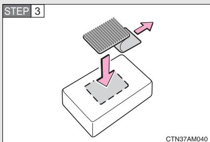
Remove the paper strip covering the adhesive on backside of loop and adhere loop to back side of the transmitter near its center.
