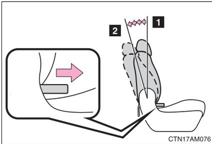
Fold the seatback while pulling the strap. Return the seatback and secure it at the 1st lock position (most upright position). Adjust the seatback to the 5th lock position. (→P. 59)
