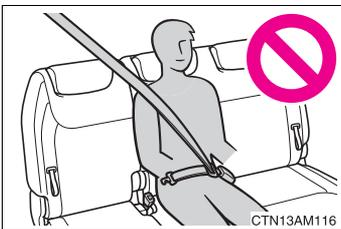
Do not use the center third seat belt with either buckle released. Fastening only one of the buckles may result in death or serious injury in case of sudden braking or a collision.
