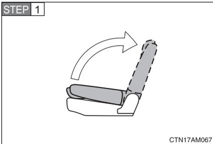
Fold down the seatback by pressing the folding/returning switch (→P. 72). Raise the seatback by pressing the same switch, the returning switch (→P. 76) or the seatback angle adjustment switch (→P. 61). (The seatback will automatically stop.) Do not touch the switch while the seatback is moving, because the operation will stop.
