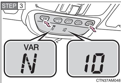
Press and hold both the “MODE” and “E/M” buttons simultaneously for 5 seconds until the “VAR” indication and a number (1 to 15) appears on the compass display.
