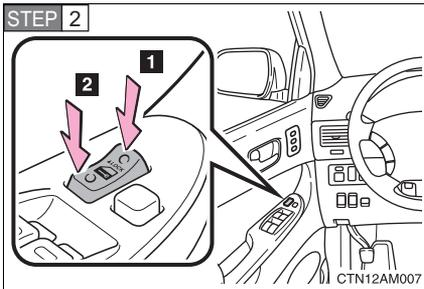
Shift the shift lever to P or N, and press and hold the driver's door lock switch (**1** or **2**) for approximately 5 seconds and then release.
