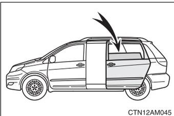
The sliding door will stop at half-opened position when the sliding door window is opened more than approximately 6 in. (15 cm).
