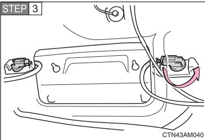
Turn the bulb bases counter-clockwise.
