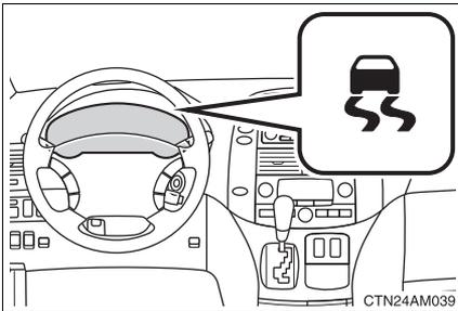
If the vehicle is in danger of slipping or the front wheels (2WD models), or 4 wheels (AWD models) spin, the indicator flashes to indicate that VSC/TRAC system have been engaged.
