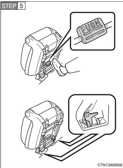
Push the foot pedal forward to securely latch the front leg locks.
