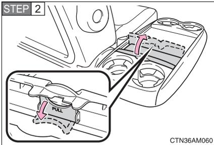
Open the lid and pull down the tab on the back of the lid.
