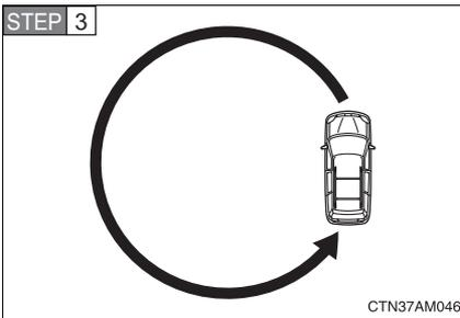
Drive the vehicle at 5 mph (8 km/h) or less in a circle until “CAL” indicator goes off and the compass returns to the normal mode.
