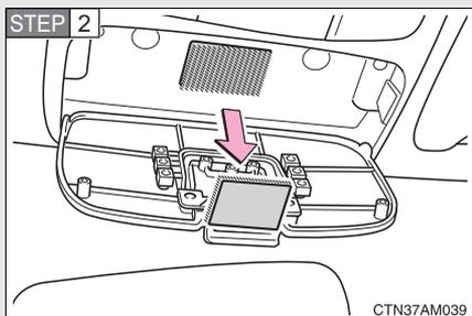
Remove the hook-and-loop fastener.
