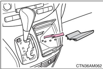
Pull out the partition and place it in the desired position as following illustration.
