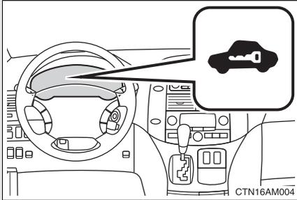
On some models: The indicator light flashes after the key has been removed from the engine switch to indicate that the system is operating.
