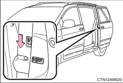
The sliding door cannot be opened from inside the vehicle when the child-protector lock is set.
