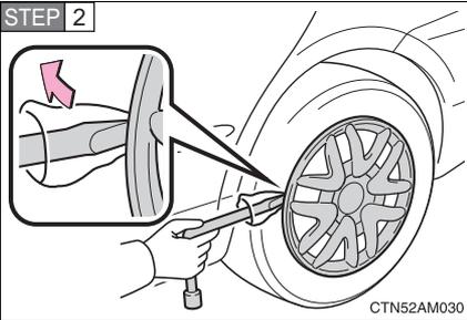
Vehicles with a steel wheel, remove the wheel ornament using the wheel nut wrench.
