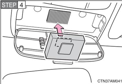
Place the transmitter with the fastener facing inside of box into the box.
