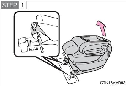
Align the front leg hooks with the rear strikers, then swing up the seat.
