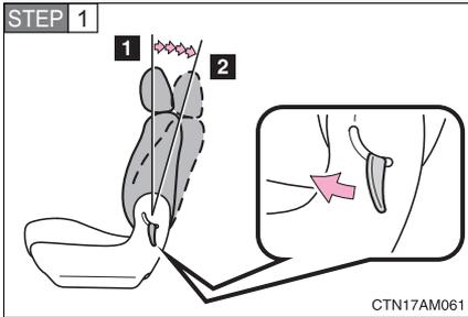
Fold the seatback while pulling the lever. Return the seatback and secure it at the 1st lock position (most upright position). Adjust the seatback to the 5th lock position. (→P. 59)
