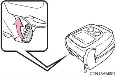
Center seat: Disengage the rear leg locks by pulling the rear leg release lever.
