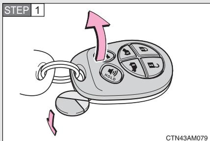
Remove the cover using a coin protected with tape etc.
