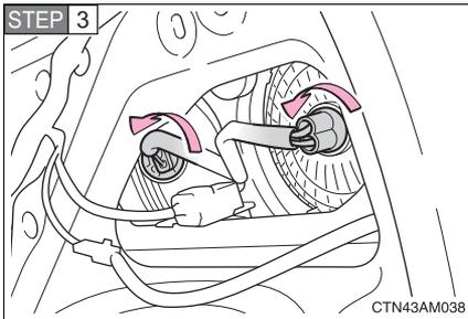
Turn the bulb bases counter-clockwise.
