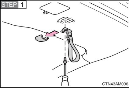
Open the back door and remove the strap.
