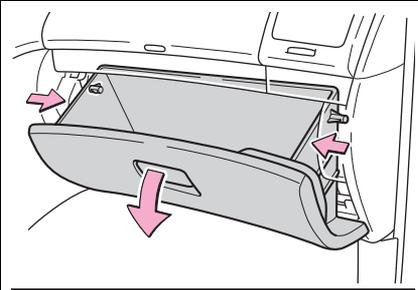
2. Push in each side of the glove box to disconnect the claws.
