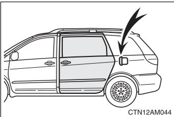
The left side sliding door (if equipped) does not open when the fuel filler door is opened.
