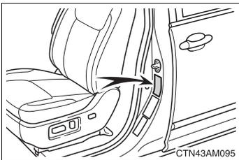
For the GAWR, see the Certification Label. For the maximum load of the tire, see the load limit at maximum cold tire inflation pressure mentioned on the sidewall of the tire. (→P. 553)
