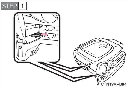
Outer seats: Disengage the rear leg locks by pushing the pins (red) inside each rear leg.
