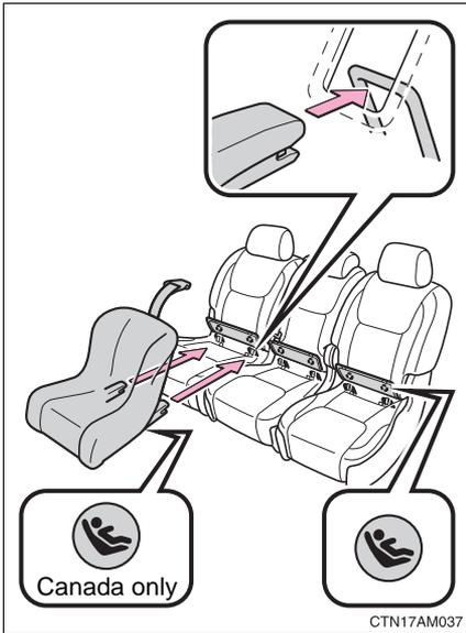
**STEP 2** LATCH anchors are behind the button. Open the cover and confirm the position of the LATCH anchors.
