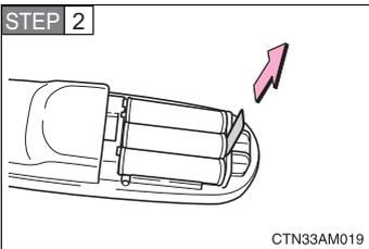
Remove the insulating sheet.
