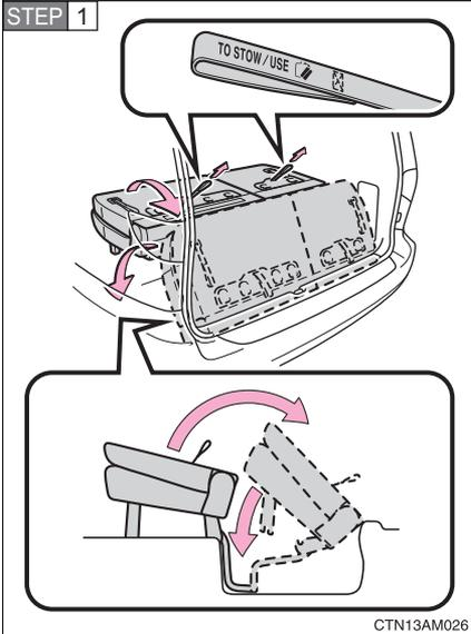
Pull and hold the “TO STOW/USE” strap and lift up the seat rearward. Then push the seat down.
