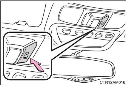
Push and hold the switch to open and close the right side sliding door.
