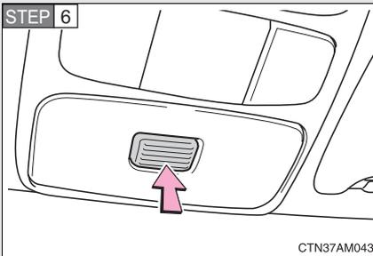
Test the operation of the transmitter by pressing the button.
