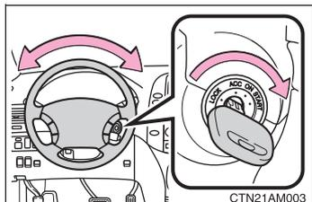
When starting the engine, the engine switch may seem stuck in the “LOCK” position. To free it, turn the key while turning the steering wheel slightly in either direction.
