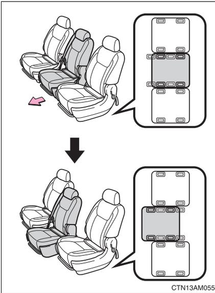
The second center seat can be used in the forward position.
