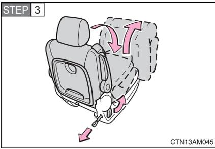
Outer seats: Fold down the seatback while pulling the seatback angle adjustment lever or strap and swing up the seat.
