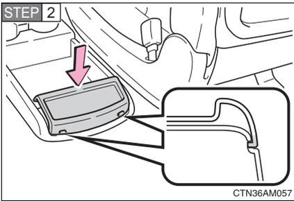
To install the tray (the tray is stored in the console box), hook it onto the outer edge of the console box installation base, then push down on the opposite end to secure it.
