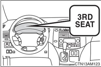
The warning light comes on if the third seat operation is not yet complete when the engine switch is in the “ON” position.
