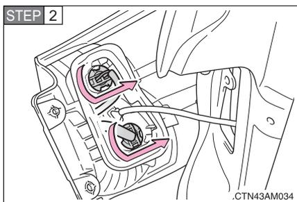
Turn the bulb bases counter-clockwise.
