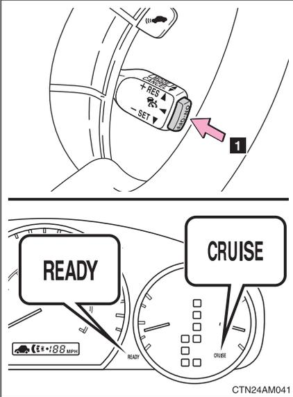
Selecting vehicle-to-vehicle distance control mode
