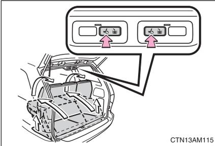
Push and hold the returning switch until the seat cushion is locked.
