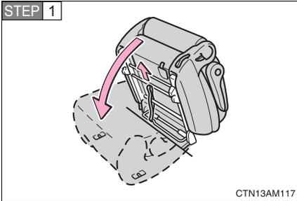
Pull and hold the front leg release strap and fold down the seat.
