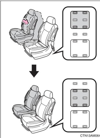
The right side second seat can be moved to the inside when the console box (if equipped) is not installed between the second seats.
