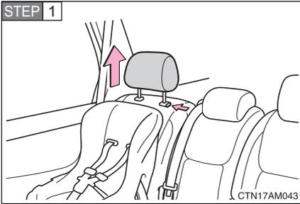
Secure the child restraint using the seat belt or LATCH anchors. Remove the head restraint.
