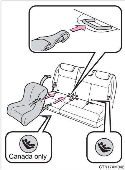
**STEP 2** Widen the gap between the seat cushion and seatback slightly and confirm the position of the LATCH anchors near the button on the seatback.
