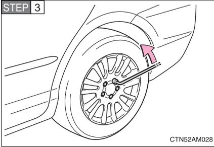
Slightly loosen the wheel nuts (one turn).
