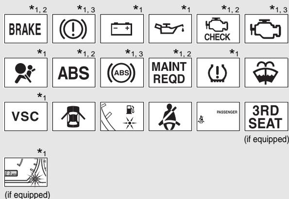
\*1: These lights turn on when the engine switch is turned to the “ON” position to indicate that a system check is being performed. They will turn off after the engine is started, or after a few seconds. There may be a malfunction in a system if a light does not come on, or if the lights do not turn off. Have the vehicle inspected by your Toyota dealer for details.
