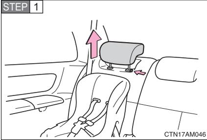
Secure the child restraint using the seat belt or LATCH anchors. Remove and safely stow the head restraint.
