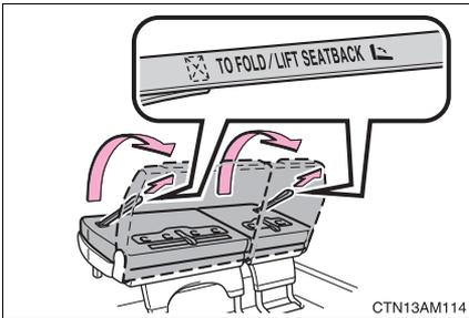
Pull the "TO FOLD/LIFT SEATBACK" strap and raise the seatback.
