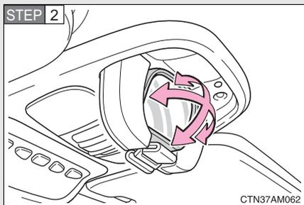
The mirror can be adjusted by pushing its edge.
