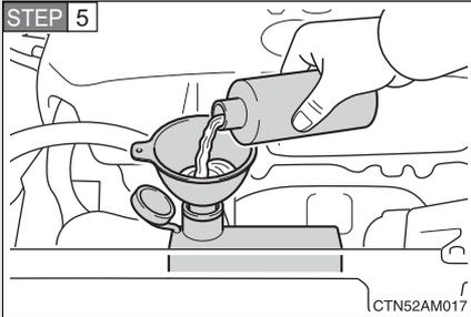
Add engine coolant if necessary.
