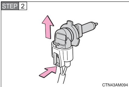
Pull out the light bulb while depressing the lock release.
