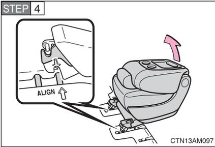
Align the front leg hooks with the rear strikers of the foremost pair. Then swing up the seat.
