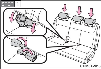
Lower the head restraints to the lowest position and stow the seat belt buckles.
