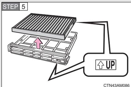
Remove the filter from the filter case.
