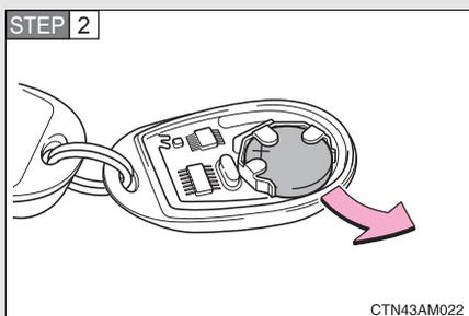
Remove the discharged transmitter battery.
