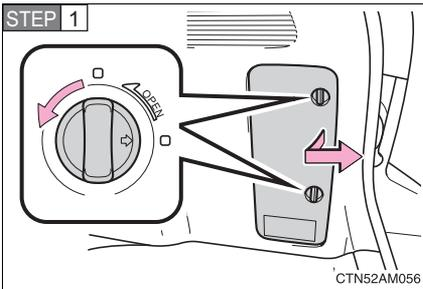
Turn the knobs to the "OPEN" position and remove the cover.
