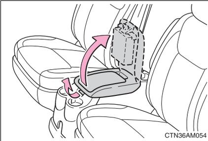
Pull up the knob to release the lock and lift the lid.
