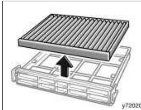
4. Remove the filter from the filter case.
