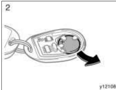
2. Remove the discharged transmitter battery.
