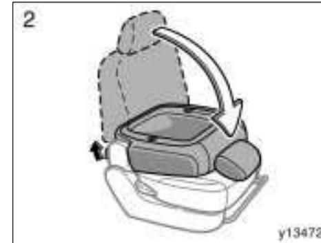
2. Pull the seatback folding lever and fold the seatback down.
