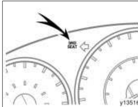
This "3RD SEAT" warning light warns the third seat operation is not yet complete when the ignition key is turned to the "ON" position.
