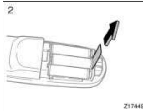
2. Remove the insulating sheet.
