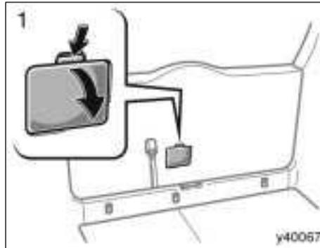
If the back door opener does not operate, you can open the back door from the inside.
