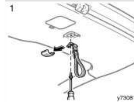
Remove the strap with a Phillips-head screwdriver.
