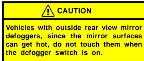
Make sure you turn the defoggers off when the surfaces are clear or the wiper blades have de-iced. Leaving the defoggers on for a long time could cause the battery to discharge, especially during stop-and-go driving. The defoggers are not designed for drying rain water or for melting snow.
