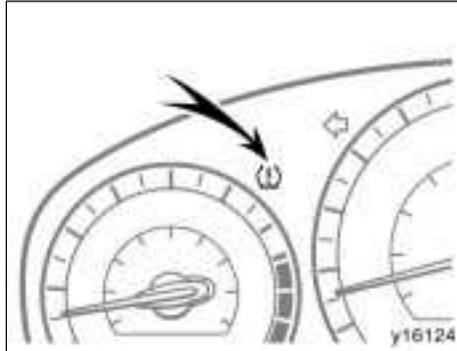
The tire pressure warning light comes on when the ignition key is turned to the "ON" position and goes off after a few seconds. This means the tire pressure warning light is operating properly. If the tire inflation pressure becomes low, the light comes on again. In this case, adjusting the tire inflation pressure will turn off the light after several minutes. If the light comes on after blinking for 1 minute, the tire pressure warning system is not working properly.
