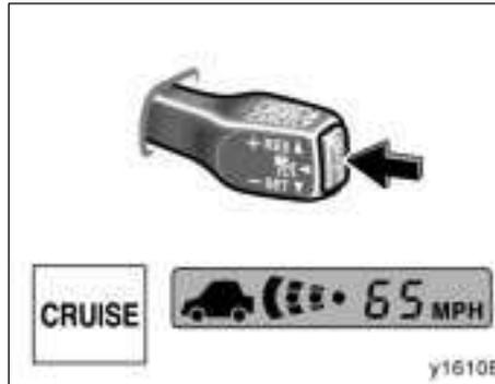
**Vehicle-to-vehicle distance control mode**
