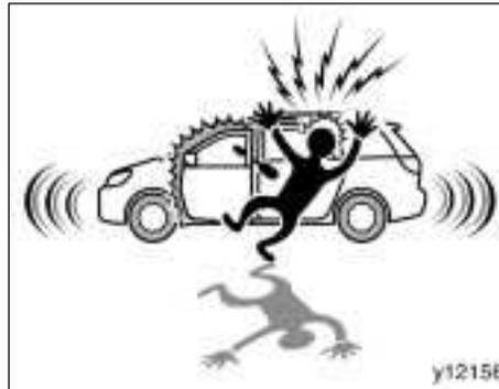
To deter the vehicle theft, the system is designed to sound an alarm if any of the side doors, back door or hood is forcibly unlocked or opened or the battery terminal is disconnected and then reconnected when the vehicle is locked. The alarm blows the horn intermittently and flashes the headlights, tail lights and turn signal lights, and turns on the front personal lights.
