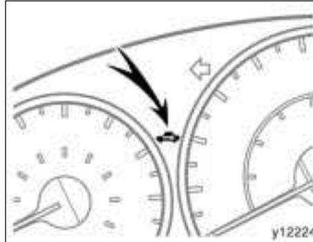
The system is automatically set when the key is removed from the ignition switch.
