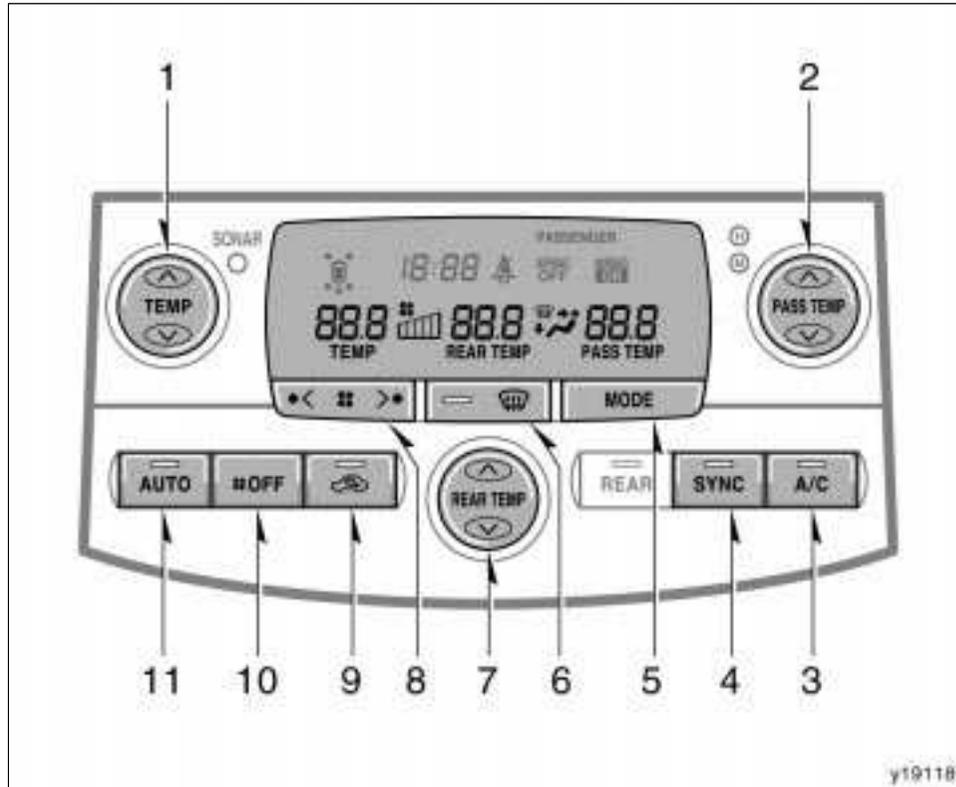
1. Temperature selector (“TEMP”) (with “SYNC” button indicator on—simultaneous setting on driver, front passenger and rear passenger sides) (with “SYNC” button indicator off—individual setting on driver side only)
