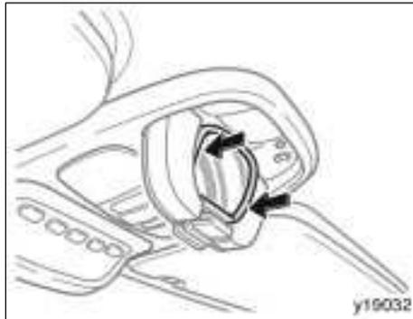
The mirror angle can be adjusted by pushing its edge.
