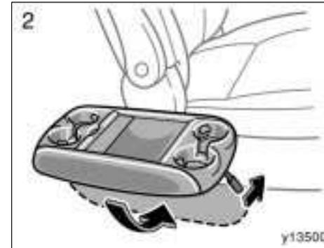
2. For vehicles equipped with the front seat side table, pull up the lock release lever and fold the table down.
