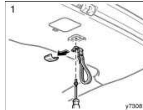
Remove the strap with a Phillips-head screwdriver.
