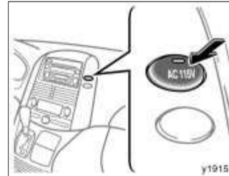
**To use the power outlet, push the main switch on the instrument panel.**
