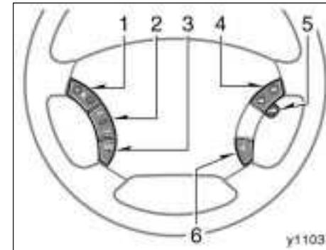
1. Volume control switches for audio system/hands-free system (For the hands-free system, see the separate "Navigation System Owner's Manual".)
