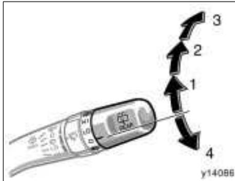
To turn on the rear window wiper, twist the lever knob upward.
