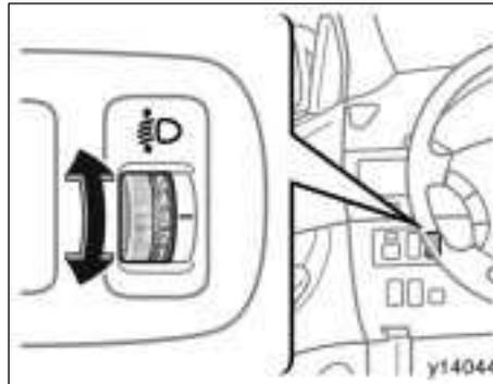
To adjust the headlight beam level, turn the dial.
