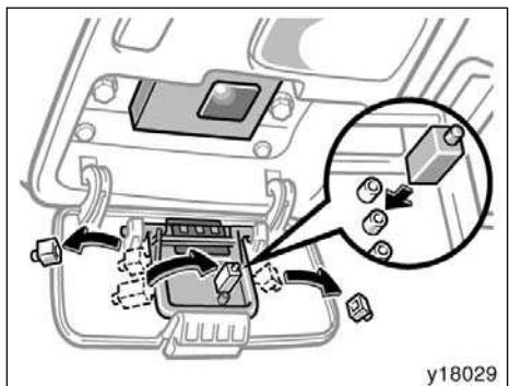
Remove spacers from the center panel. Place the largest spacer on the pin that would be below transmitter button when the cover is closed. Close the cover.
