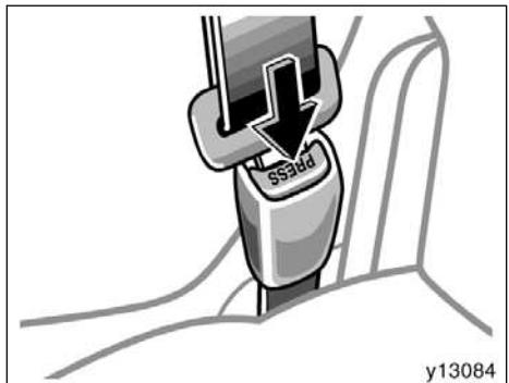
2. To remove the child restraint system, press the buckle-release button and allow the belt to retract.
