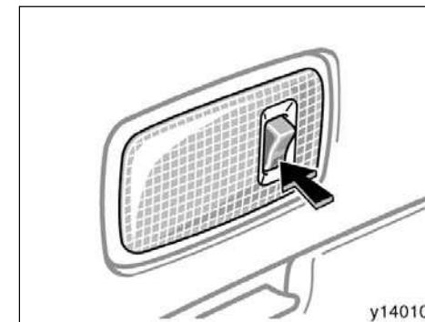
**To turn the luggage compartment light on, open the back door and push the switch downwards. To turn it off, push the switch upwards or close the back door.**
