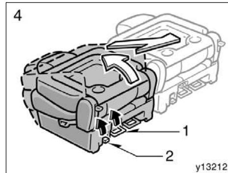
4. Pull the center handle (1) up while holding up the left side lever (2) under the seat, lift the seat and remove it toward you.
