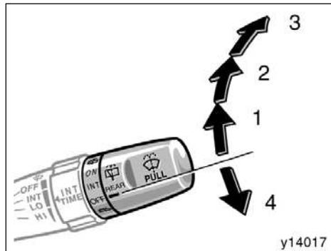
To turn on the rear window wiper, twist the lever knob upward.
