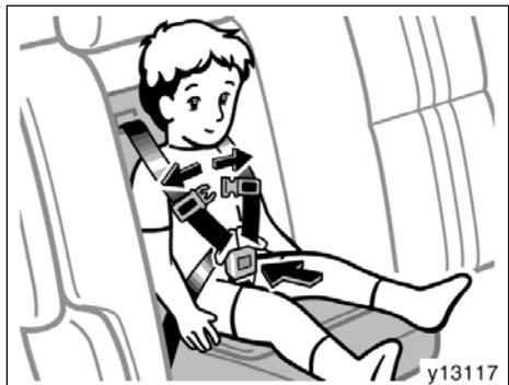
10. To release the child from the seat belts, separate the shoulder belts, then press the buckle release button.
