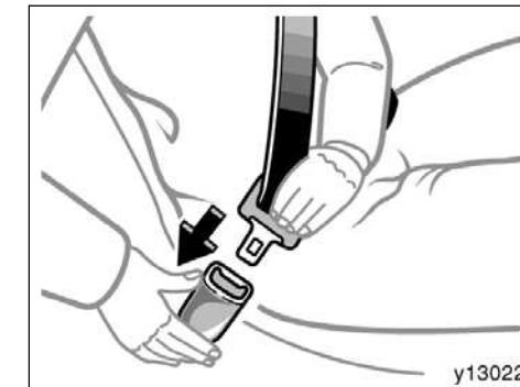
Adjust the seat as needed and sit up straight and well back in the seat. To fasten your belt, pull it out of the retractor and insert the tab into the buckle.
