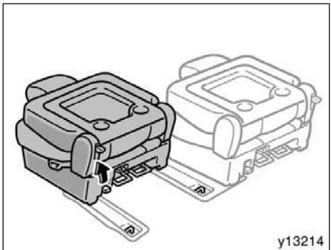
If the seat legs are locked in the wrong position, pull up the left side lever under the seat. Then lift and remove the seat.
