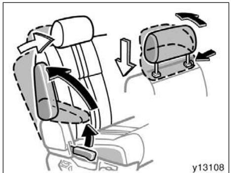
1. Bring the seat to the upright position and raise the armrest. Move the head restraint to the fully down and fully backward position.
