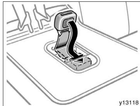
11. To store the built-in child restraint, fasten the shoulder belt clip and return the seat belt buckle. Raise the child seat cushion.
