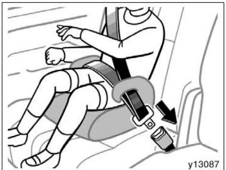
1. Sit the child on a booster seat. Run the lap and shoulder belt through or around the booster seat and child following the instructions provided by its manufacturer and insert the tab into the buckle taking care not to twist the belt.
