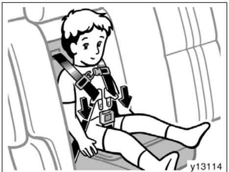
7. Sit the child on the child seat. Place a shoulder belt over each shoulder. Insert the tabs into the buckle.
