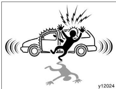
**To deter the vehicle theft, the system is designed to sound an alarm if any of the front, sliding or back doors or hood is forcibly unlocked or the battery terminal is disconnected and then reconnected when the vehicle is locked.**
