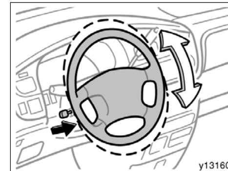
To change the steering wheel angle, hold the steering wheel, pull the lock release lever toward you, tilt the steering wheel to the desired angle and release the lever.
