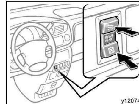
The rear quarter windows can be operated with the "REAR VENT" switch on the instrument panel.
