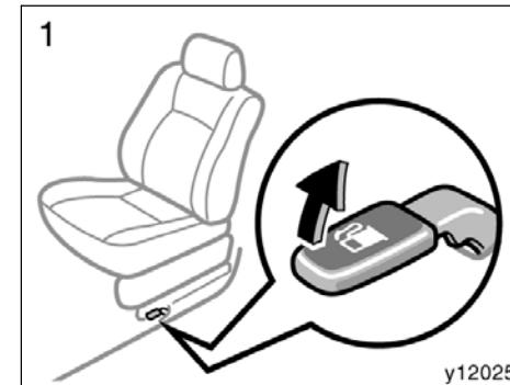
1. To open the fuel filler door, pull the lever up.
