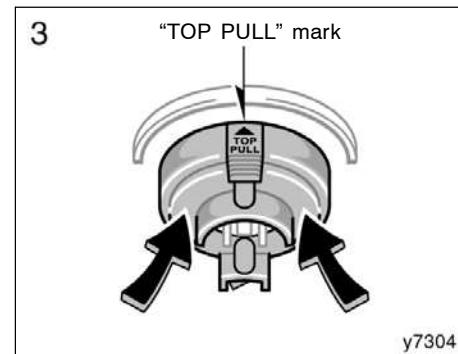
**3. Install the rubber cover with the "TOP PULL" mark upward, and fit it securely on the boss. Then plug in the connector.**
