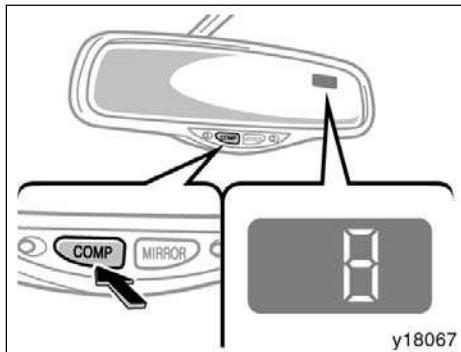
**CALIBRATING THE COMPASS (deviation calibration)**
