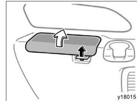
To use the box, pull up the lock release lever and open the lid.
