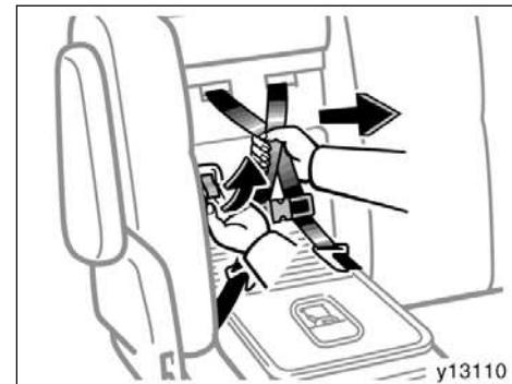
3. While lifting the seat belt adjustment lever in the child seat back panel, pull both shoulder belts together.
