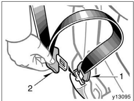
To release the concave end tab (1), press the buckle-release button with the round end tab (2).
