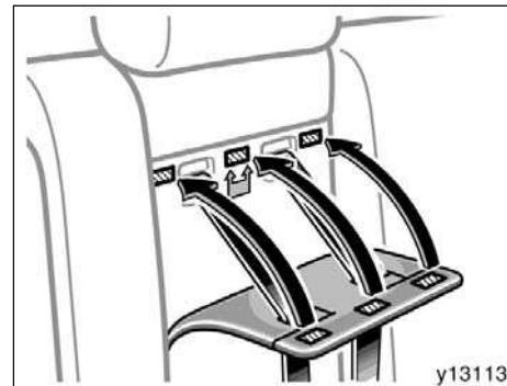
6. Press the removable pad against the Velcros and install the pad to the seatback. Make sure the belts go through the slots in the pad.
