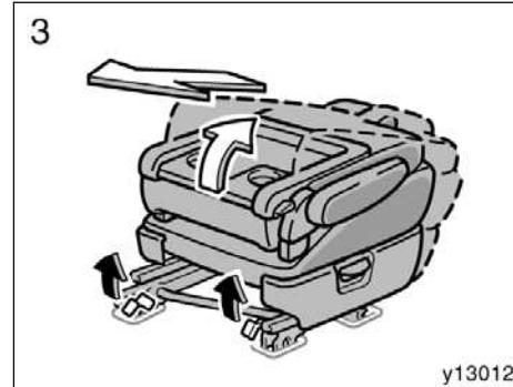
**3. Pull the seat lock release lever. Lift the seat cushion and remove the seat toward you.**
