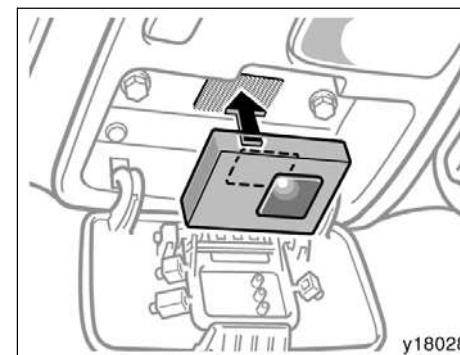
Place the transmitter with Velcro loop facing inside of box into the box. Make sure the transmitter button is located above button pins.
