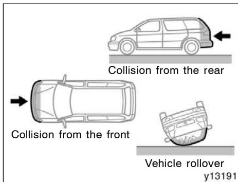
**The SRS side airbags are not designed to inflate if the vehicle is involved in a front or rear collision, if it rolls over, or if it is involved in a low-speed side collision.**
