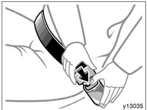
To release the belt, press the buckle-release button.
