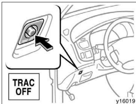
"TRAC OFF" indicator light comes on for a few seconds when the ignition key is turned to "ON". It will come on again when you push the "TRAC OFF" switch to turn off the system.
