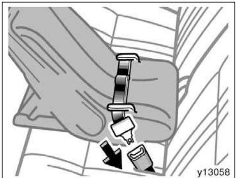
1. Run the center lap belt through or around the infant seat following the instructions provided by its manufacturer and insert the tab into the buckle taking care not to twist the belt.
