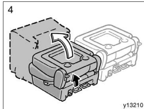
4. Unlock the seat legs by pulling up the center handle under the seat, and swing the whole seat up and forward.
