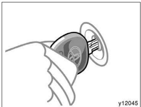
The engine immobiliser system is a theft prevention system. When you insert the key in the ignition switch, the transponder chip in the key's head transmits an electronic code to the vehicle. The engine will start, only when the electronic code in the chip corresponds to the registered ID code for the vehicle.
