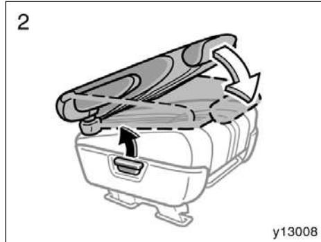
**2. Lift the seatback angle adjusting lever and fold the seatback down.**
