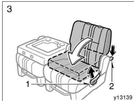
3. Lift the seatback angle adjusting lever (1) or press the lever (2) behind the seatback and fold the seatback down.
