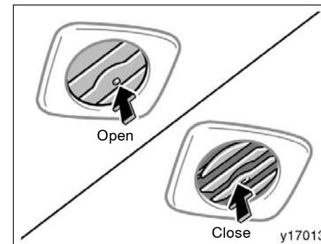
If air flow control is not satisfactory, check the roof vents. The roof vents may be opened or closed as shown.
