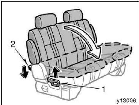
Lift the seatback angle adjusting lever (1) or press the lever (2) behind the seatback and fold the seatback down.
