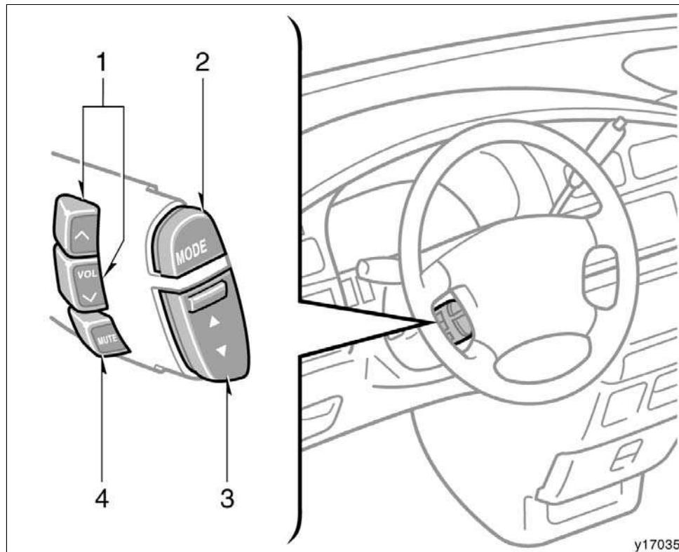
Some parts of the audio system can be adjusted with the buttons on the steering wheel.
