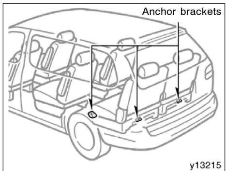
Second seat (left side only): Use the anchor bracket on the floor to attach the top strap.
