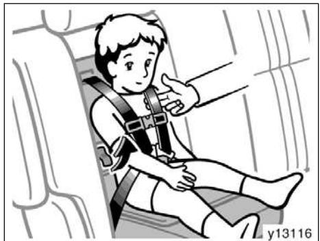
9. Lift the seat belt adjusting lever to allow the belts to retract until the shoulder belts are snugly adjusted around the child's shoulders.
