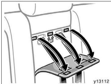
5. Pull down the seatback part of the removable pad. Make sure the child's shoulders are at or below the maximum shoulder height indicator label.
