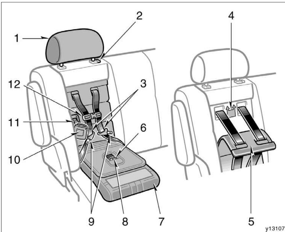
The built-in child restraint system mainly consists of two child seats integrated in the bench type second seat with 5-point seat belts. Refer to the illustration to become familiar with the parts of the system. This child restraint system conforms to U.S. Federal Motor Vehicle Safety Standard No.213 and Canada Motor Vehicle Safety Standard No.213.4.
