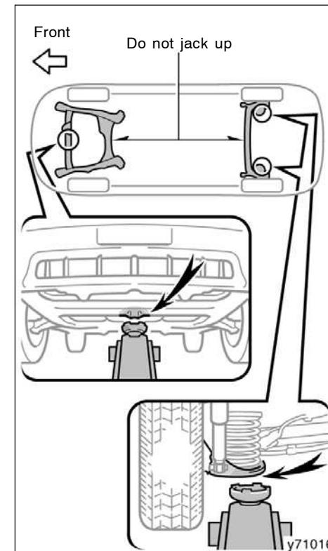
When jacking up your vehicle with the jack, position the jack correctly as shown in the illustrations.
