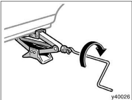
6. After making sure that no one is in the vehicle, raise it high enough so that the spare tire can be installed.
