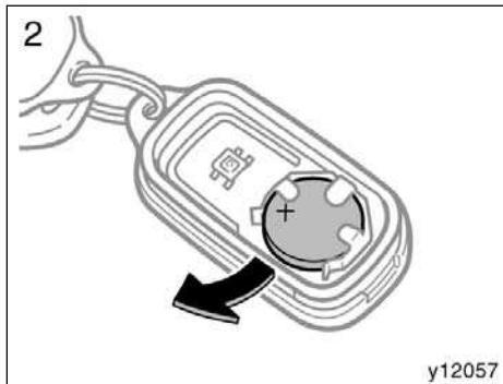
2. Remove the discharged transmitter battery.
