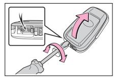
3 Remove the depleted battery using a small flathead screw-driver.
