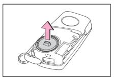
3 Remove the depleted battery.
