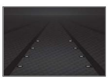
Indicates that the system is not able to recognize white (yellow) lines or a course\* or is temporarily can-
