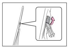
3 Slide the wiper blade to remove it from the wiper arm.
