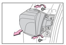
3 Turn the bulb base counter-clockwise.
