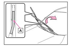
**2** Lift the stopper using a flathead screwdriver as shown in the illustration.
