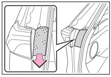
2 Remove the screws and remove the unit.
