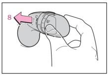
Pulling the lever operates the wipers and washer.
