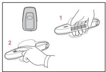
1 Grip the driver's door handle to unlock the door. Holding the driver's door handle for approximately 2 seconds unlocks all the doors.
