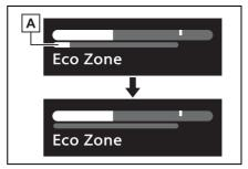
The engine braking force will be increased according to the driving conditions to more efficiently charge the hybrid battery (traction battery) after the accelerator pedal is released.
