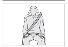
Extend the shoulder belt so that it comes fully over the shoulder, but does not come into contact with the neck or slide off the shoulder
