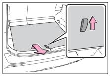
Place the deck board through the groove and move forward.
