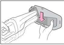
6 Hold the filter to the light and check if it is not clogged.
