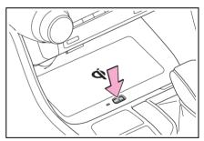
2 Place the portable device on the charging tray
