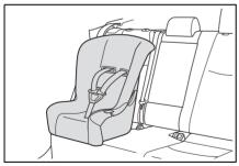
4 Run the seat belt through the child restraint system and insert the plate into the
