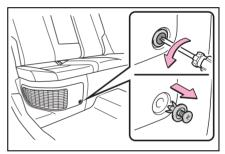
3 Remove the air intake vent cover.
