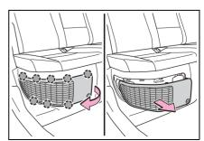
4 Remove the filter from the air intake vent cover.
