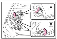
Engine compartment: Type B fuse box
