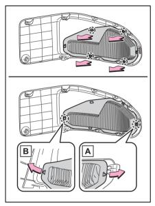
5 Remove the dust and sand from the filter.
