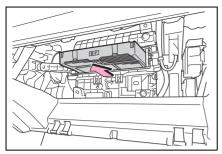
7 Remove the air conditioning filter from the filter case and replace it with a new one.
