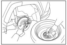
Install the spare tire and loosely tighten each wheel nut by hand by approximately the same amount.
