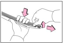
4 Remove the 2 metal plates from the old wiper insert and
