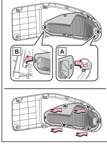
8 Install the air intake vent cover.
