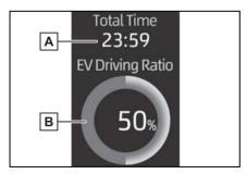
A Elapsed time after starting Displays the elapsed time since hybrid system was started.\*
