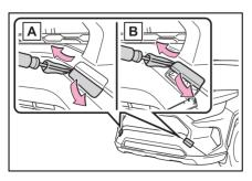
Insert the towing eyelet into the hole and tighten partially by hand.
