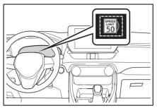
If signs other than speed limit signs are recognized, they will be displayed in an overlapping stack under the current speed limit sign.
