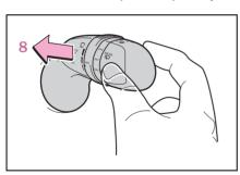
Pulling the lever operates the wipers and washer.
