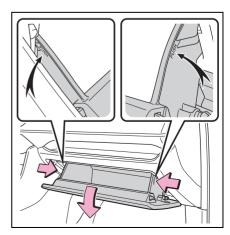
With the glove box fully open, slightly lift up the glove box and pull toward the seat to detach the bottom of the glove box.
