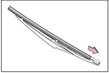
6 Check that the wiper blade claws are fitted in the grooves of the wiper insert.
