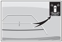
A simplified image is displayed on the upper corner of the screen when an obstacle is detected.
