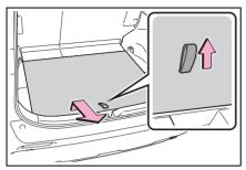
2 Place the deck board through the groove and move forward.
