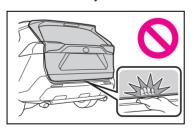
Use caution when using the back door closer as it still operates when the power back door system is canceled.
