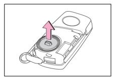
3 Remove the depleted battery.
