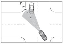
When you turn right/left, pedestrian is detected in the forward direction and estimated to enter your vehicle's path (bicyclists are not detected.)
