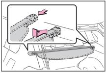
2 Pull out the luggage cover and hook it onto the anchors.
