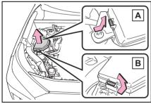
Engine compartment: Type B fuse box
