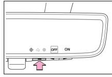
3 Press representation of to enable (ON)/disable (OFF) the automatic anti-glare function.
