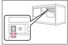
3 Press and hold the desired HomeLink<sup>®</sup> button (inside the vehicle) for 2 seconds and release it. Repeat this
