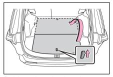
2 Place the edge into the groove (A), and with the deck board in a standing state, put the edge into the holes (B).
