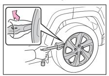
3 Slightly loosen the wheel nuts (one turn).
