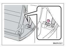
3 Push in each side of the glove box to disconnect the claws.
