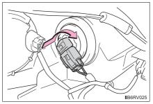
6 For the right side only: Move the washer tank inlet and install the securing clip.
