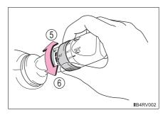
Washer/wiper dual operation The wipers will automatically operate a couple of times after the washer squirts.
