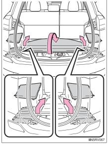
2 Insert the right end of the rear cargo net into the recess, then compress the left end of the rear cargo net and insert it into the recess.
