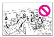
• Vehicles without a smart key system: Do not attach any heavy, sharp or hard objects such as keys and accessories to the key. The objects may restrict the SRS knee airbag inflation or be thrust into the driver's seat area by the force of the deploying airbag, thus causing a danger.
