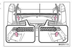
2 Insert the right end of the rear cargo net into the recess, then compress the left end of the rear cargo net and insert it into the recess.
