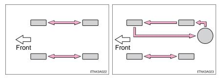
Do not fail to initialize the tire pressure warning system after tire rotation
