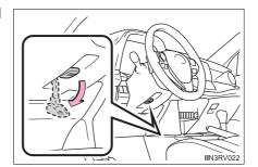
2 Adjust to the ideal position by moving the steering wheel horizontally and vertically.
