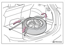
4 Hook one end of the forked belt to the cargo hook on the far right side, and the other end to the cargo hook on the near left side.
