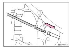
5 Holding a rag under the end, pull the dipstick out and check the
