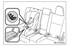
Seat belts equipped with a child restraint locking mechanism (ALR/ELR belts except driver's seat belt) (→P. 34)
