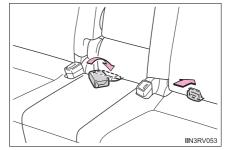
3 Lower the head restraint to the lowest position. ( $\rightarrow$ P. 146)
