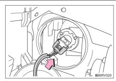
7 Set the connector and install the cover.
