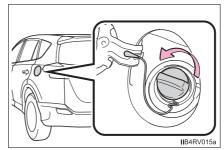
3 Hang the fuel tank cap on the back of the fuel filler door.
