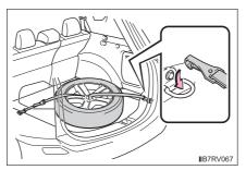
5 Pull the belt as shown in the illustration to secure the tire.
