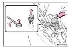
2 Disconnect the connector and turn the cover counter-clockwise.
