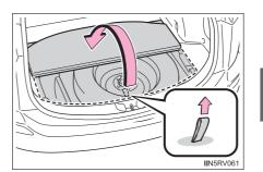
2 Fold up the deck board. The lid can be removed.
