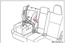
6 If the child restraint has a top tether strap, the top tether strap should be latched onto the top tether strap anchor.  $(\rightarrow P. 71)$
