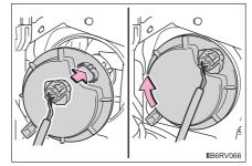
8 For the right side only: Move the washer tank inlet and install the securing clip.
