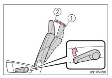
If your child restraint system interferes with a head restraint and cannot be installed properly, install the child restraint system after removing the head restraint. ( $\rightarrow$ P. 146)
