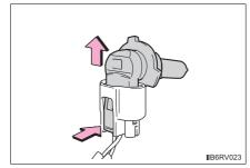
Align the 3 tabs on the light bulb with the mounting, and insert.
